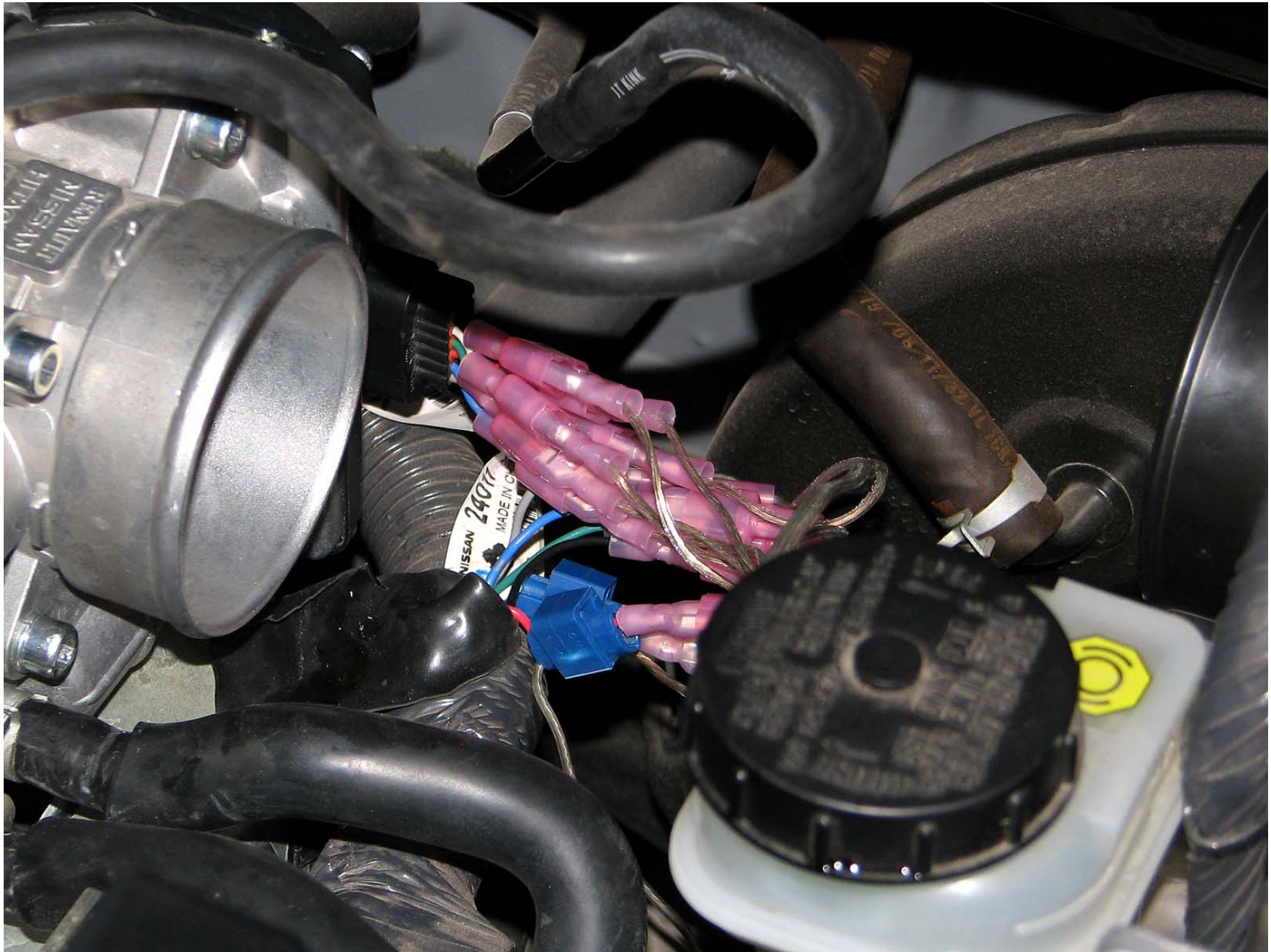
Figure A-9: Throttle Body Test Setup
