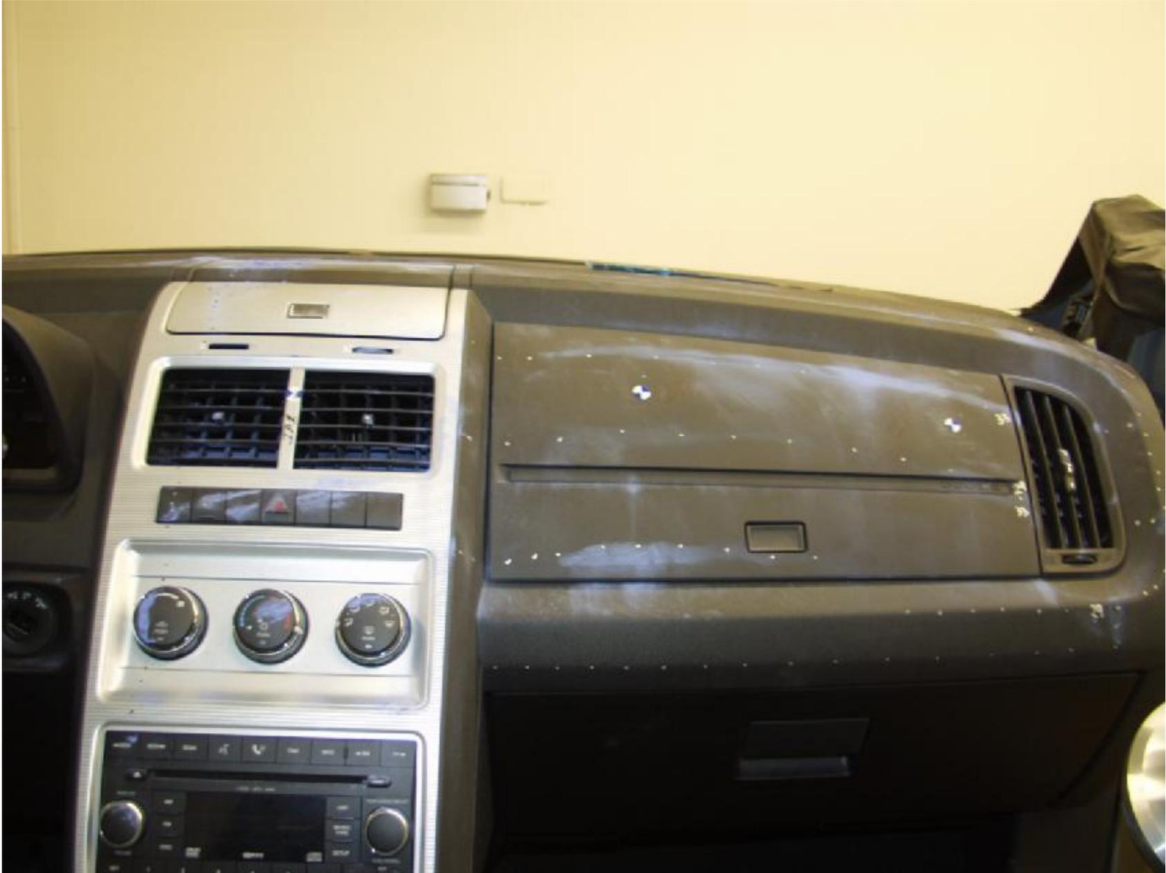
Figure A-14 : DELINEATED INSTRUMENT PANEL IMPACT ZONE POST-TEST
