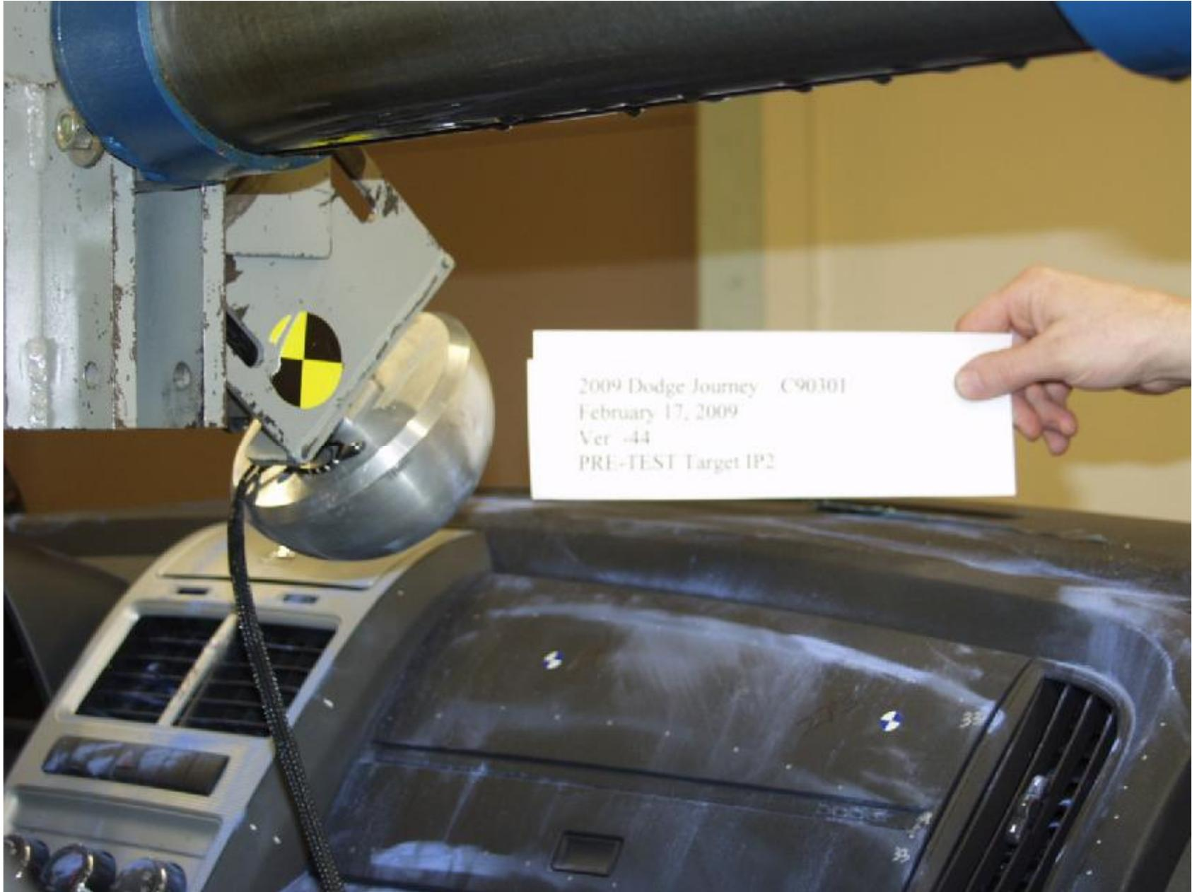
Figure A-17 : INSTRUMENT PANEL IMPACT #2 PRE-TEST
