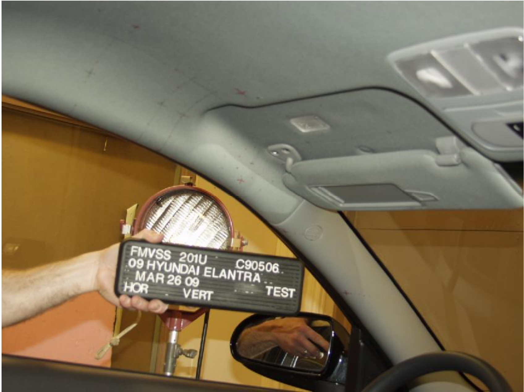
Figure A-7 : PRE-TEST DRIVER SIDE A-PILLAR
