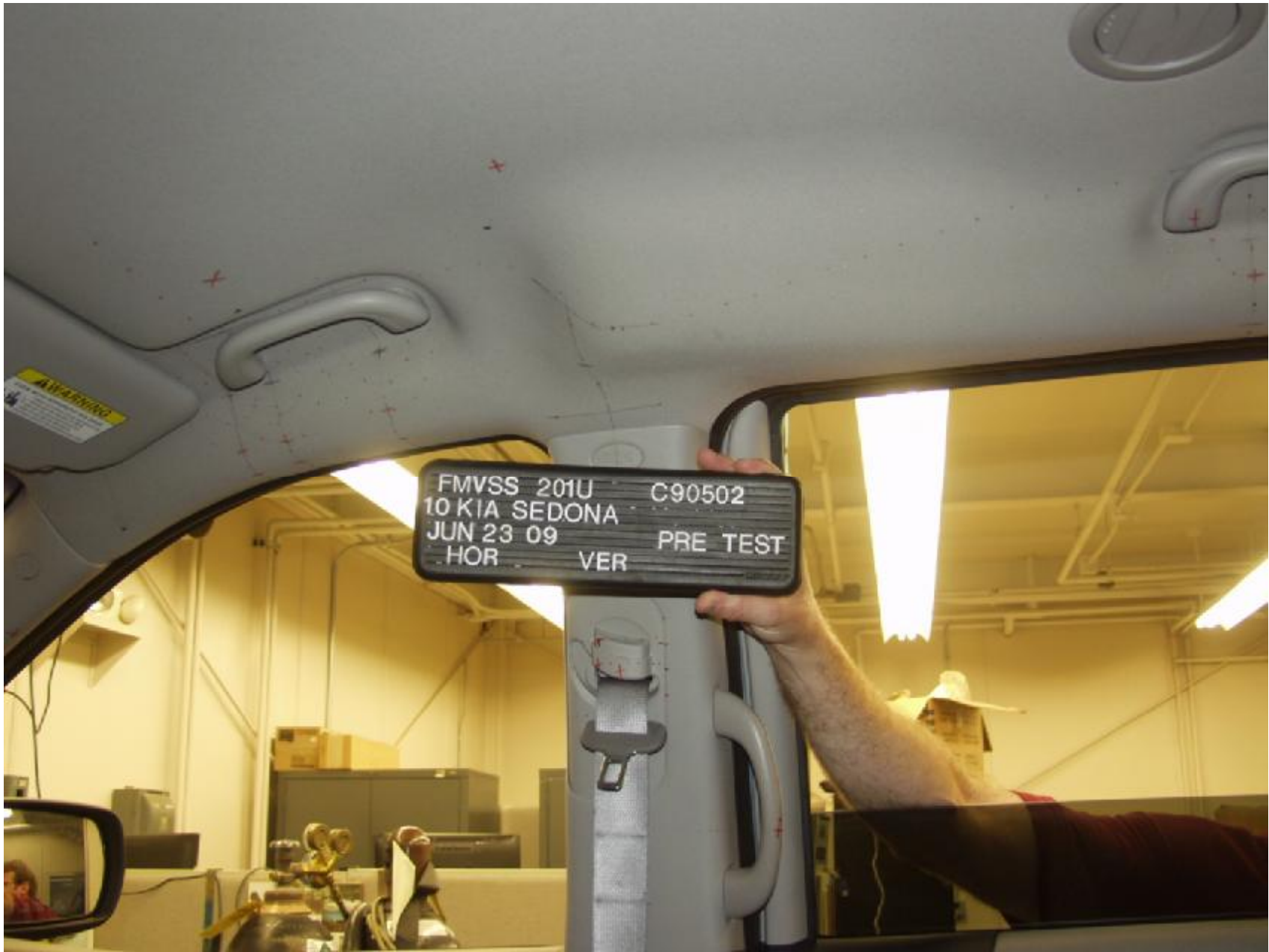
Figure A-17 : PRE-TEST PASSENGER SIDE B-PILLAR
