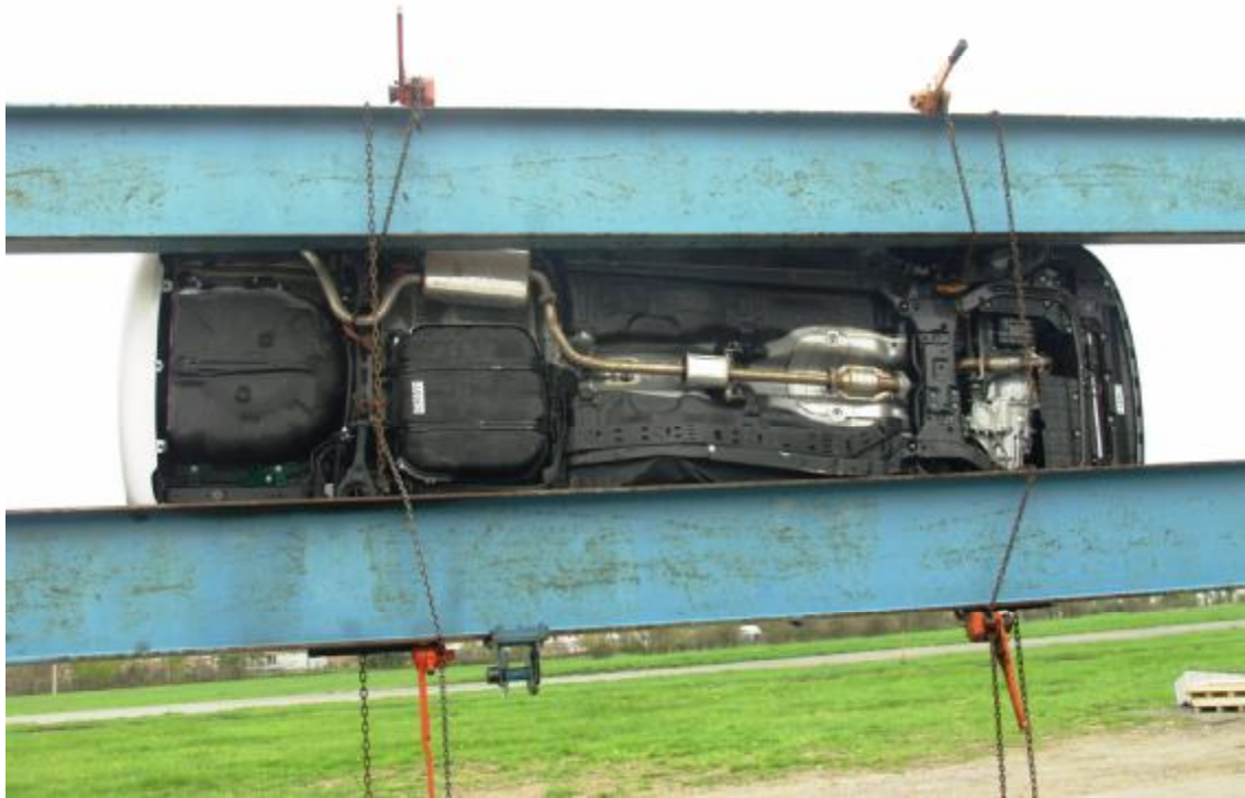
Figure A-40: Rollover 90 Degrees
