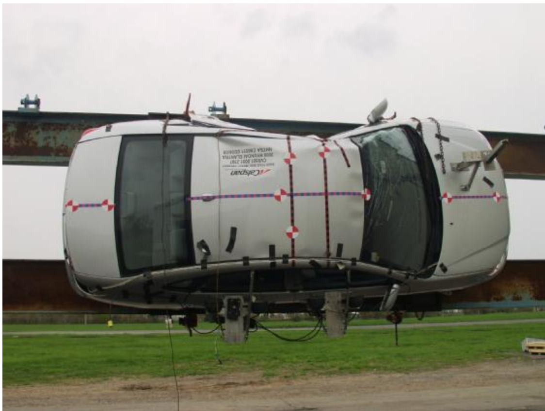
Figure A-42: Rollover 270 Degrees
