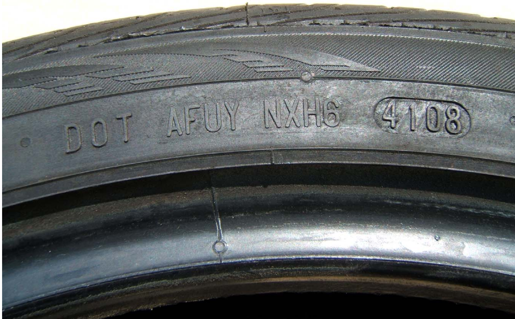
FIGURE 5.7 TIRE SHOWING DOT SERIAL NUMBER
