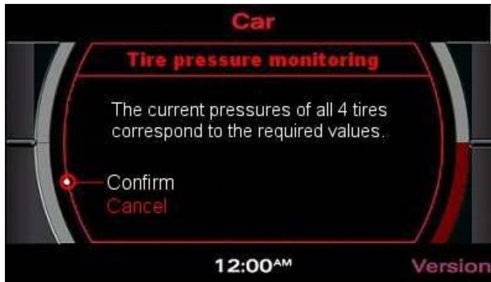
FIGURE 5.12 MULTI MEDIA INTERFACE CENTER CONSOLE DISPLAY SHOWING TPMS RESET
