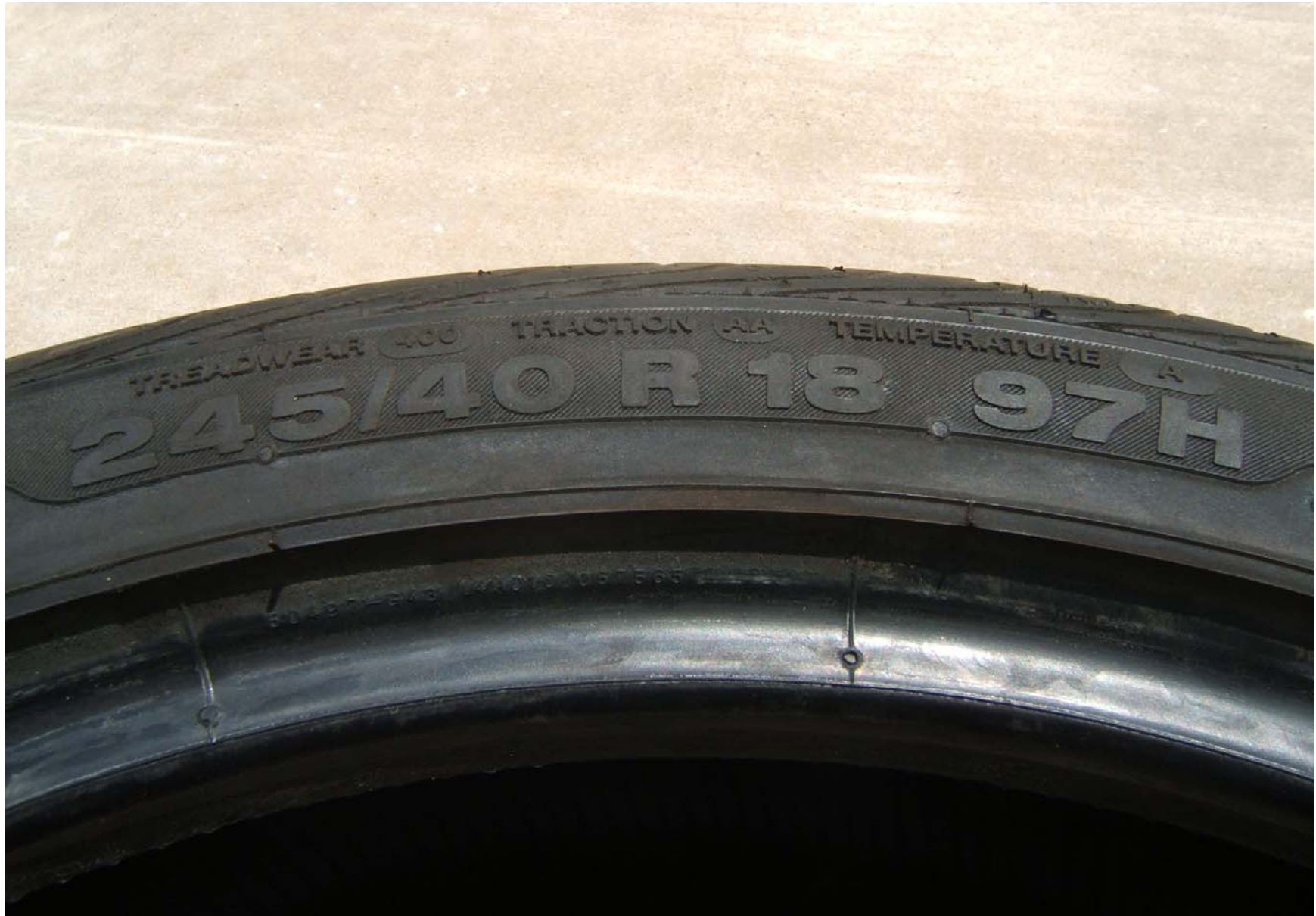
FIGURE 5.6 TIRE SHOWING SIZE AND LOAD INDEX / SPEED RATING
