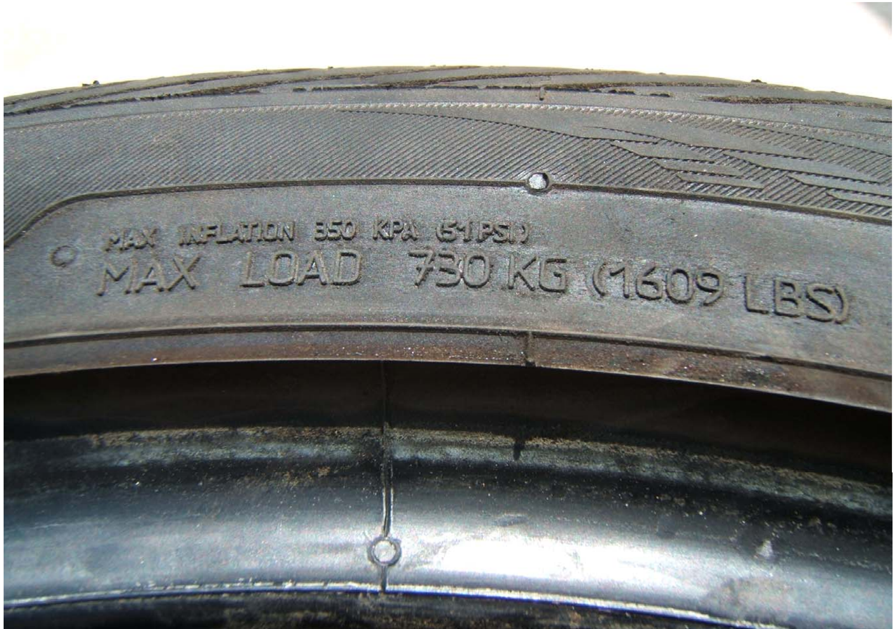
FIGURE 5.8 TIRE SHOWING MAX COLD INFLATION PRESSURE AND MAX LOAD RATING
