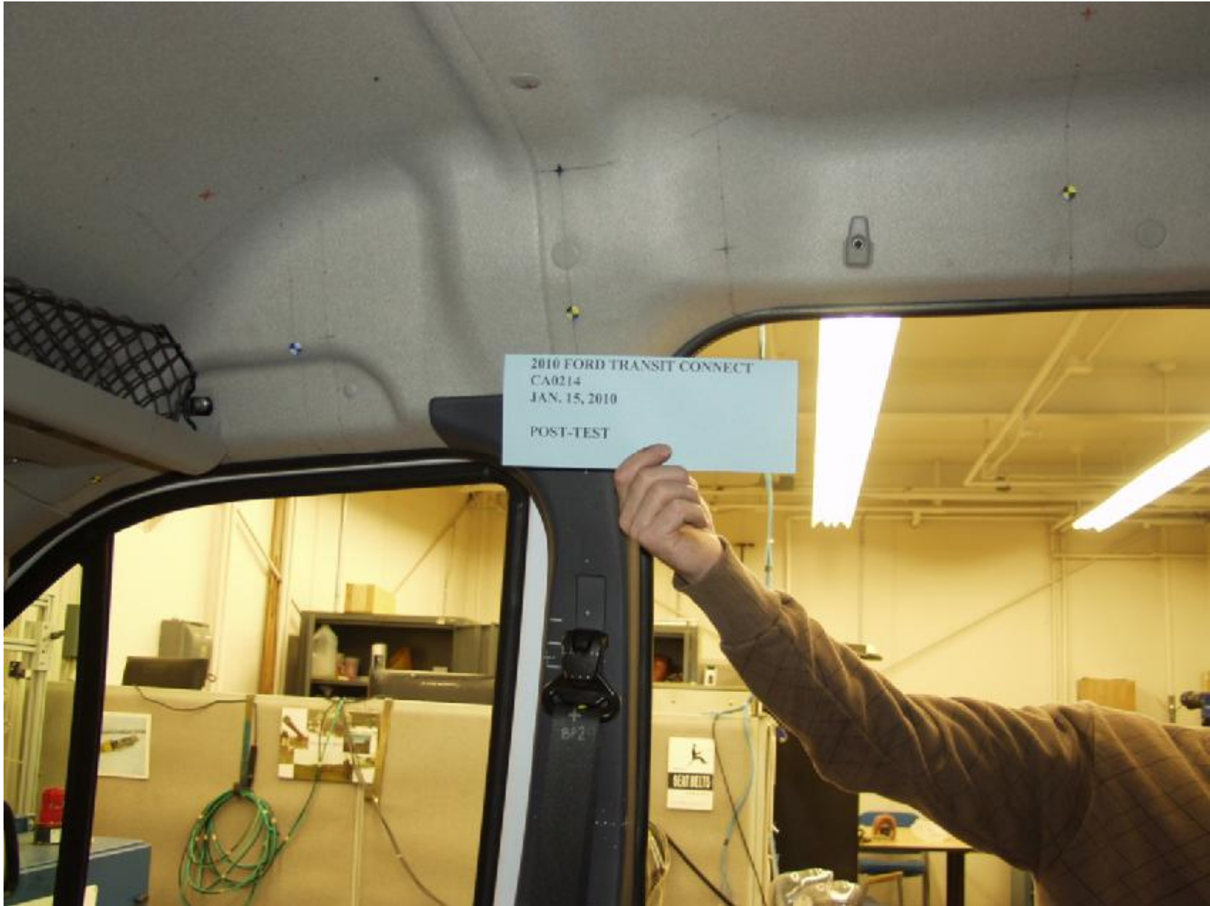
Figure A-28 : POST-TEST PASSENGER SIDE B-PILLAR
