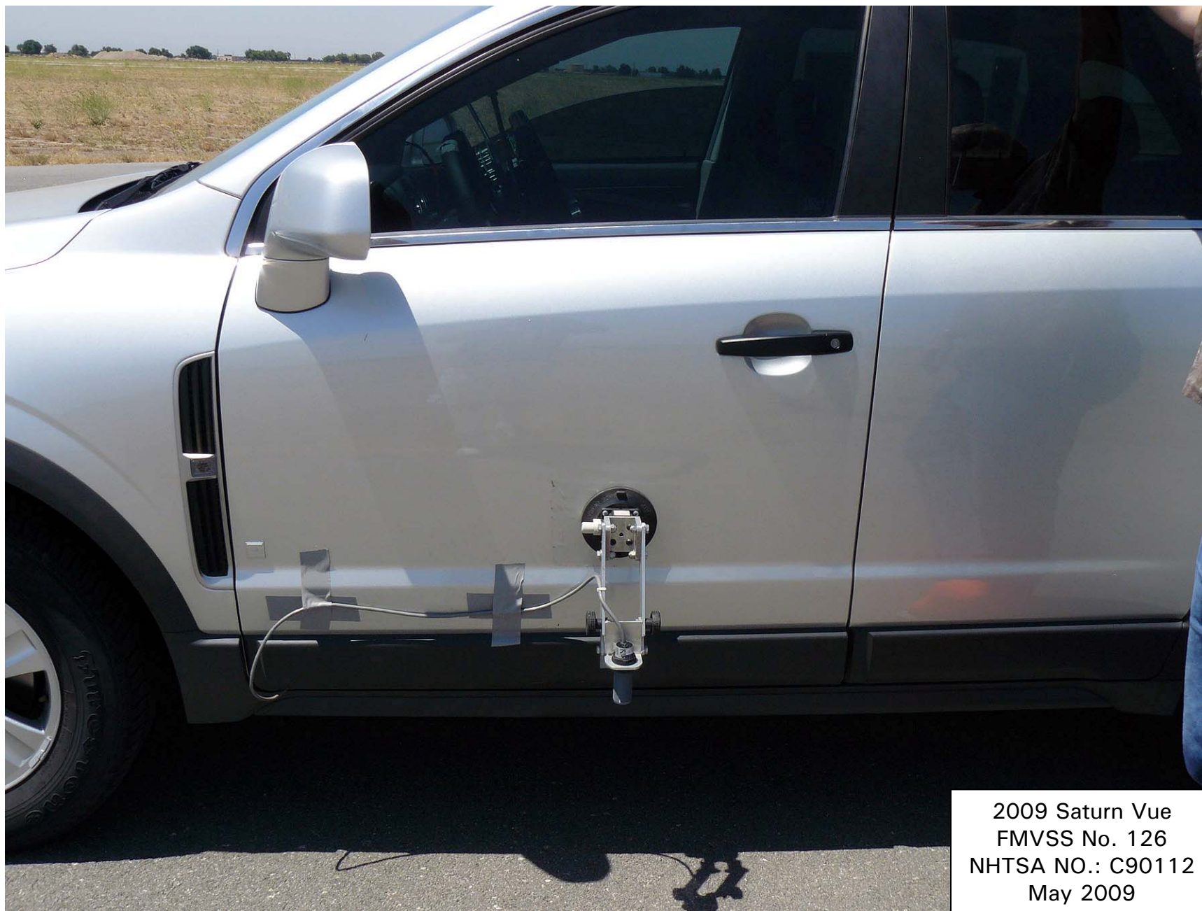
Figure 5.11. Ultrasonic Height Sensor Mounted on Left Side of Vehicle for Determining Body Roll Angle
