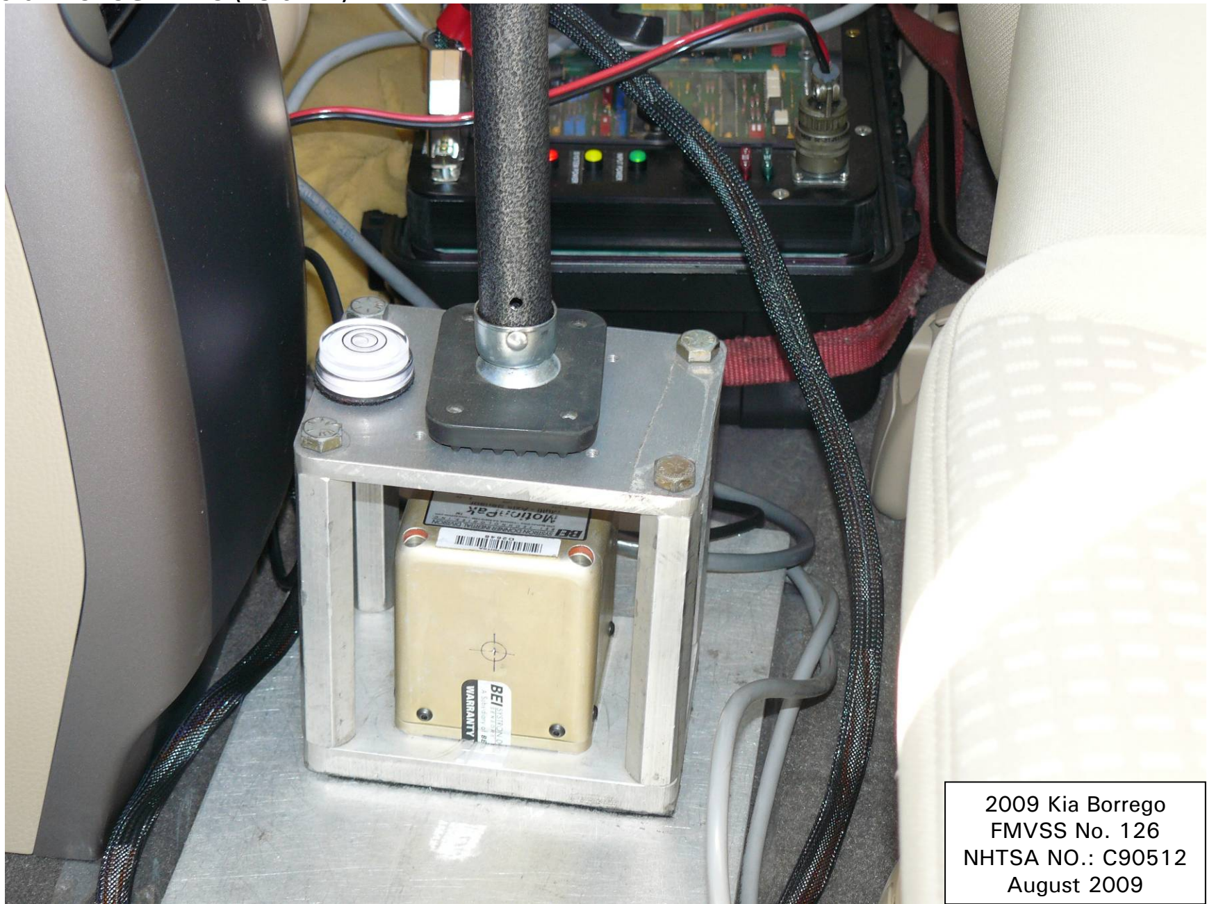
Figure 5.13. Inertial Measurement Unit Mounted in Vehicle
