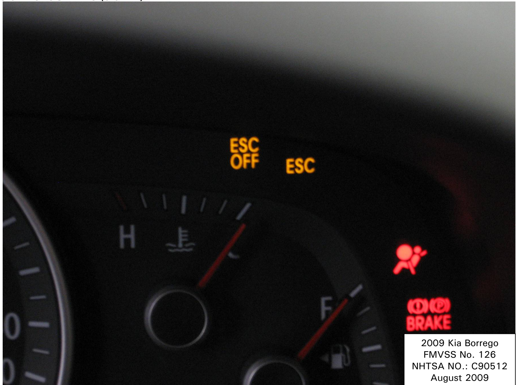
Figure 5.6. Telltales for ESC Actuation, Malfunction and ESC Off
