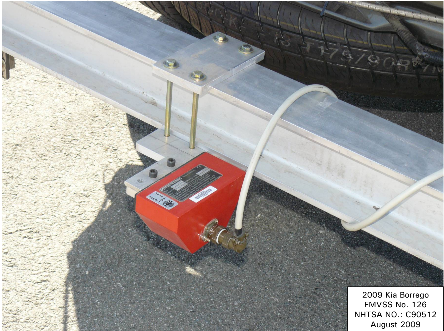
Figure 5.11. Rear Outrigger, Mount and Speed Sensor
