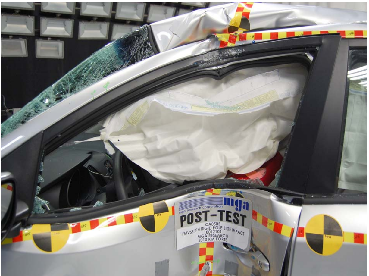
Post-Test Dummy with Door Closed (Impact Side)
