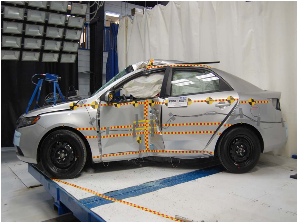
Post-Test Impacted Side View of Test Vehicle
