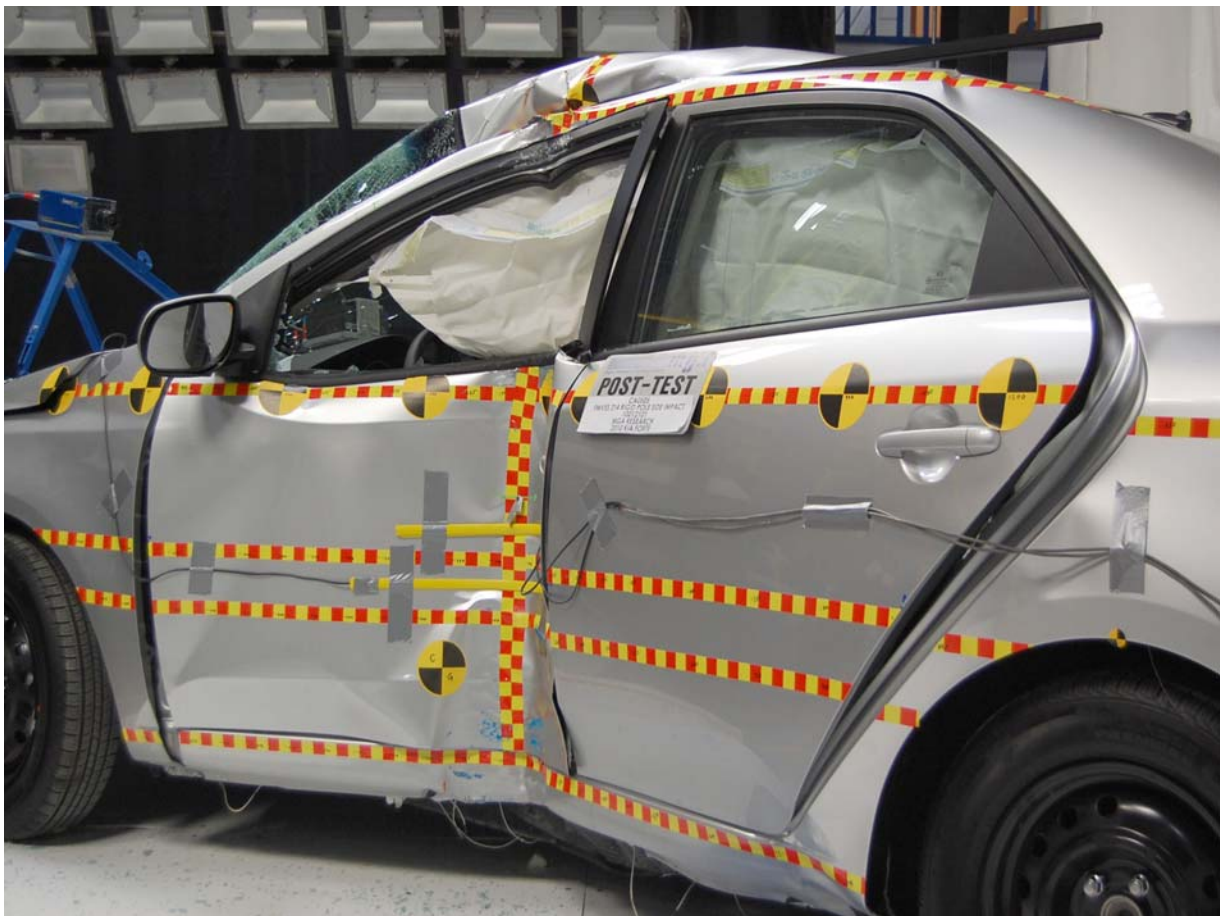
Post-Test \frac{3}{4} Rear View of Impact Zone
