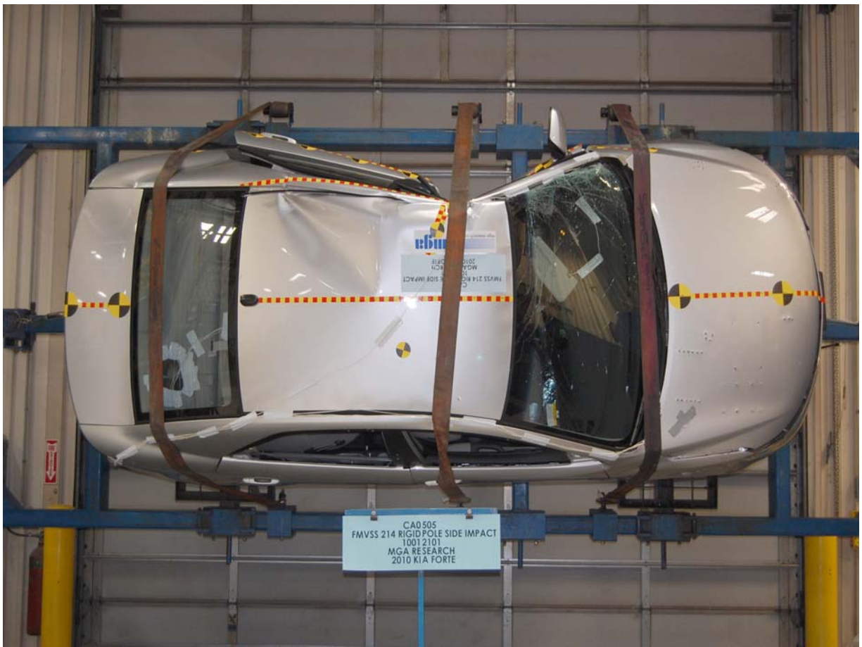
Post-Test Vehicle at 270 Degree Rollover
