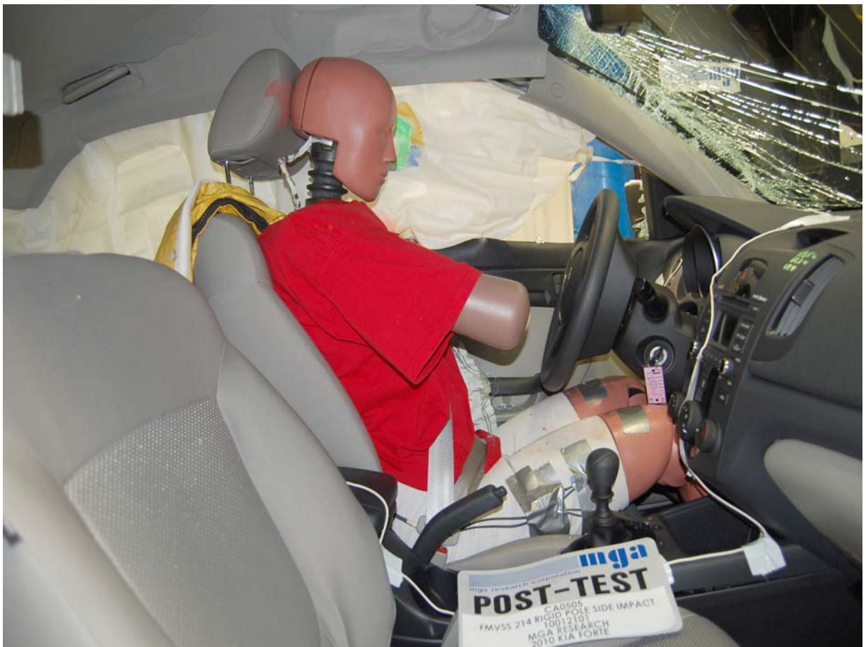
Post-Test Dummy Through Opposite Window
