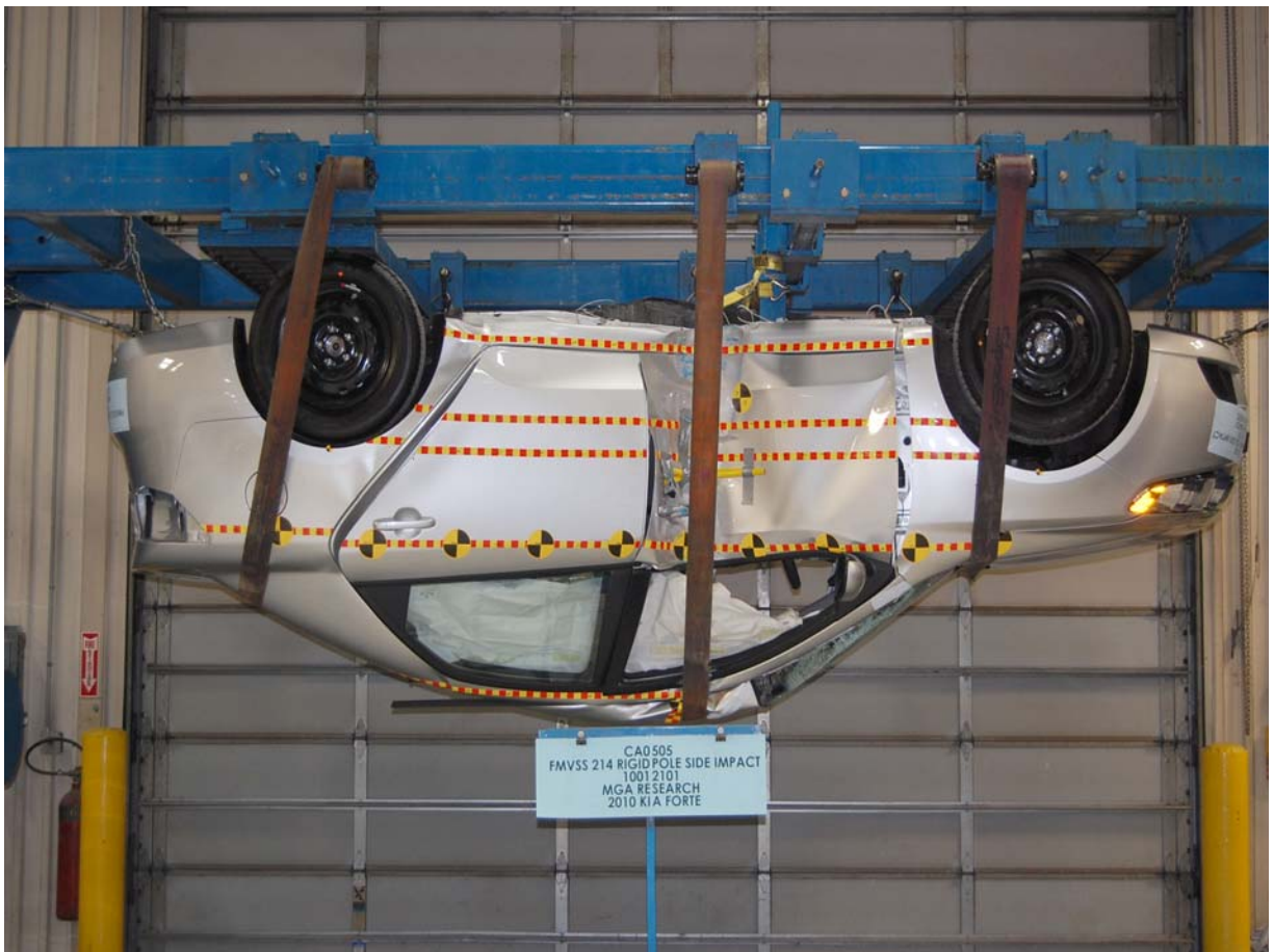
Post-Test Vehicle at 180 Degree Rollover
