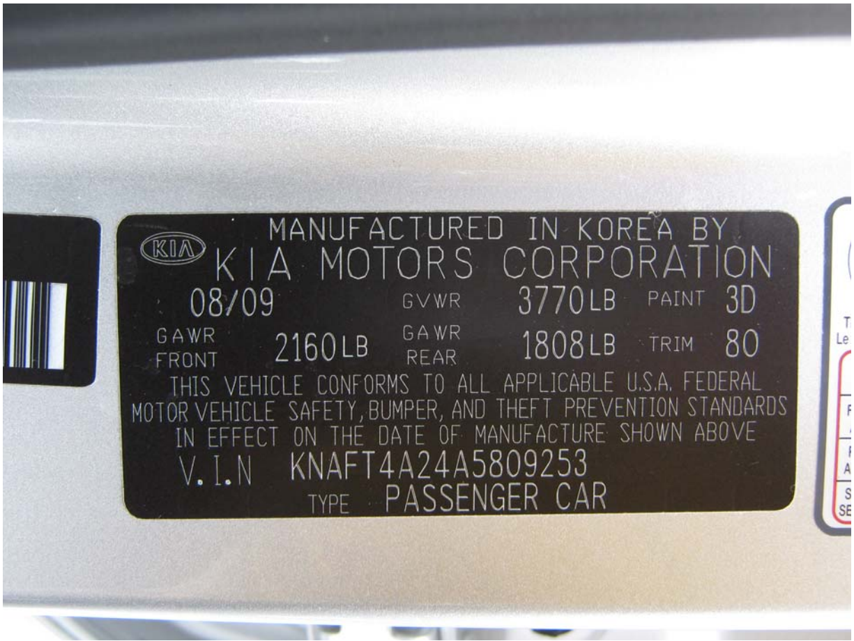
Close-up View of Vehicle's Certification Label
