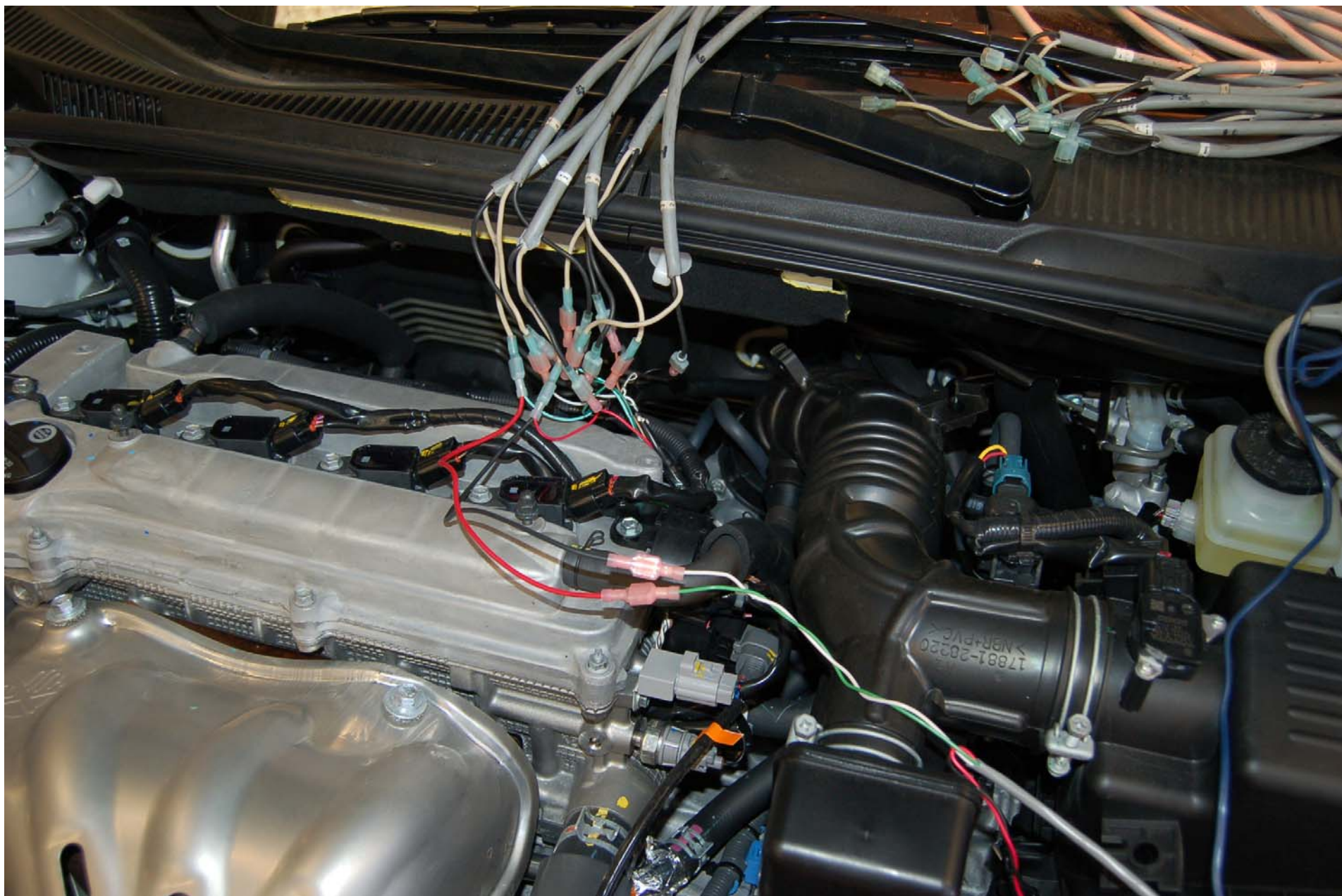
FIGURE 5.10 TEST SET-UP AT THROTTLE BODY
