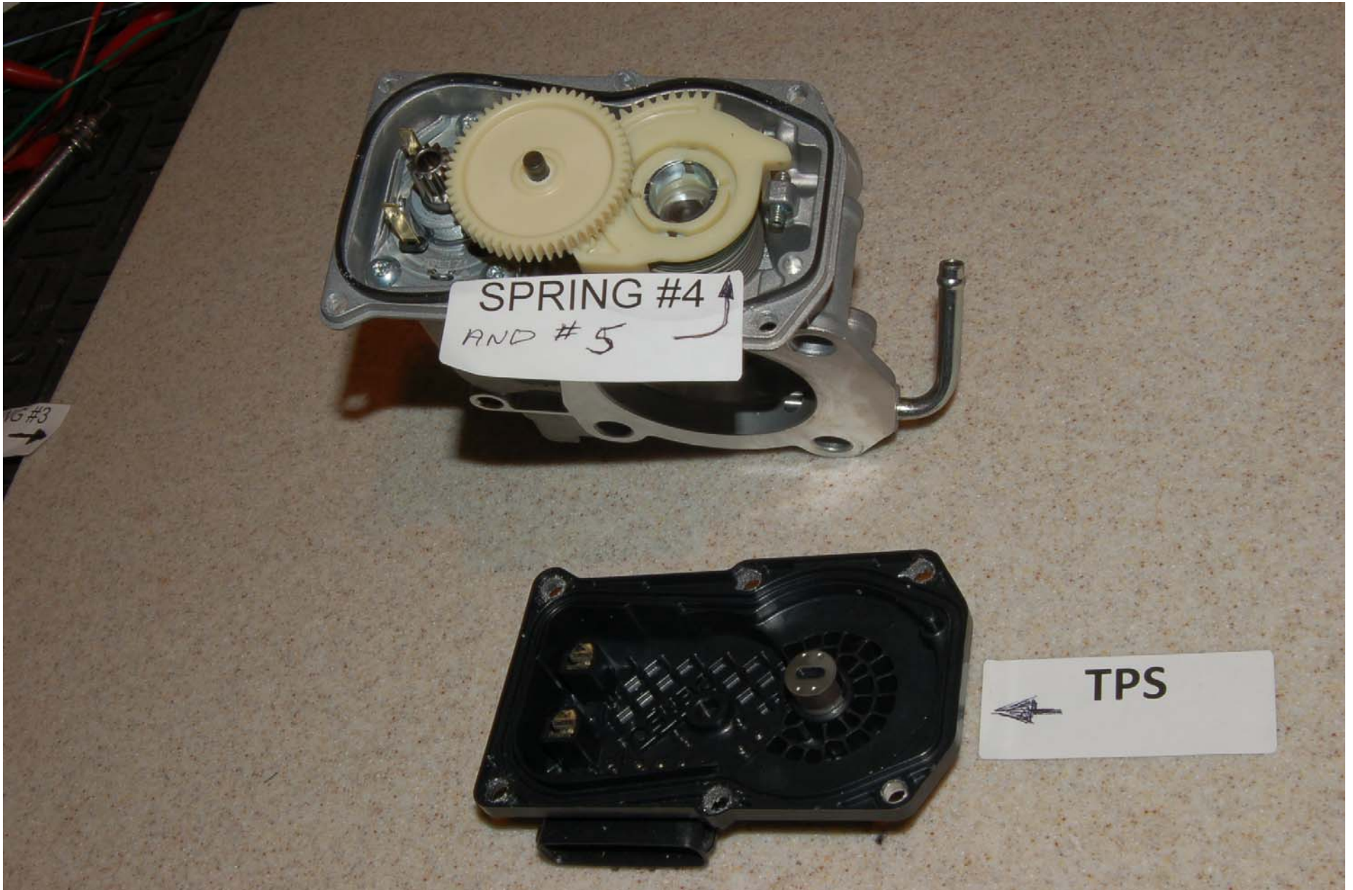
FIGURE 5.11 THROTTLE POSITION SENSOR WITH SPRINGS 4 & 5
