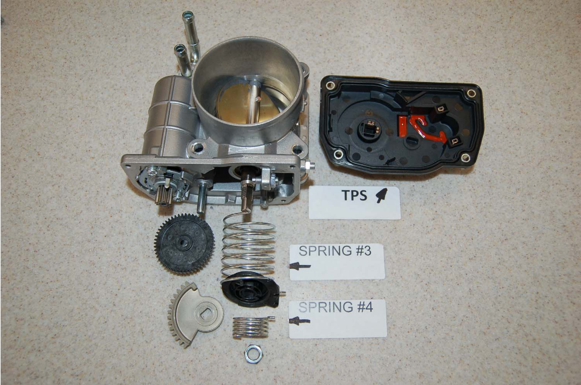
FIGURE 5.11 THROTTLE POSITION SENSOR WITH SPRINGS 3 & 4
