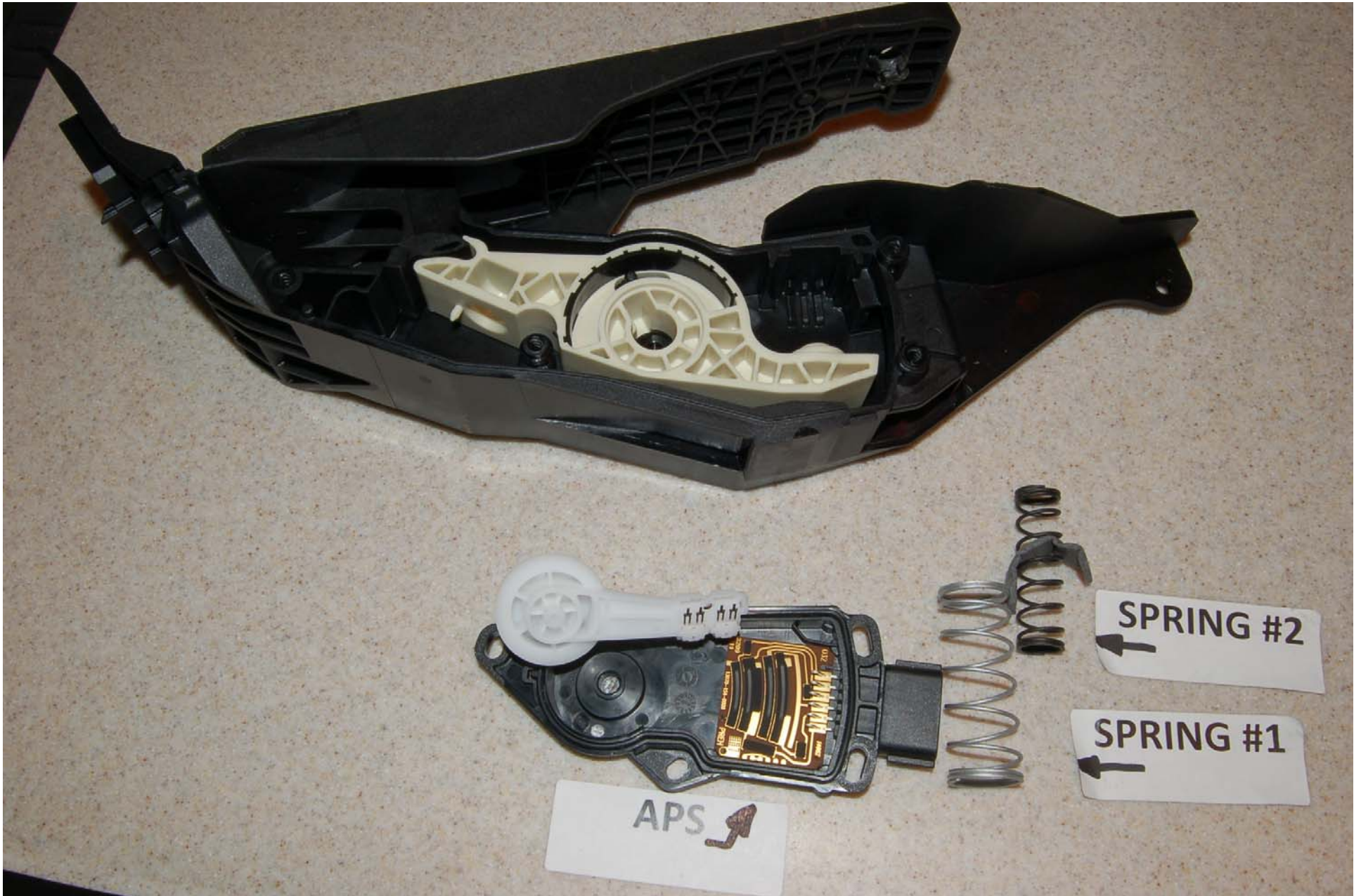
FIGURE 5.10 ACCELERATOR PEDAL SENSOR WITH SPRINGS 1 & 2
