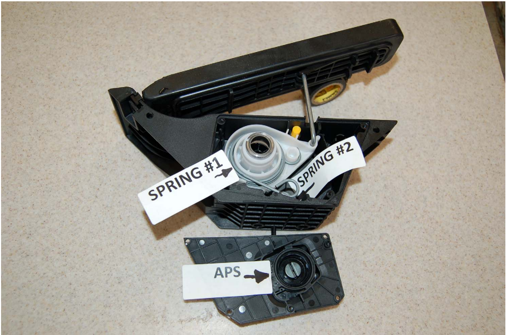
FIGURE 5.6 ACCELERATOR PEDAL ASSEMBLY SHOWING SPRING 1 & 2
