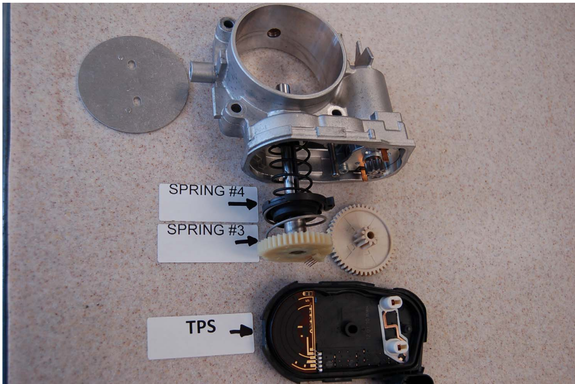
FIGURE 5.13 THROTTLE BODY SHOWING SPRINGS 3 & 4
