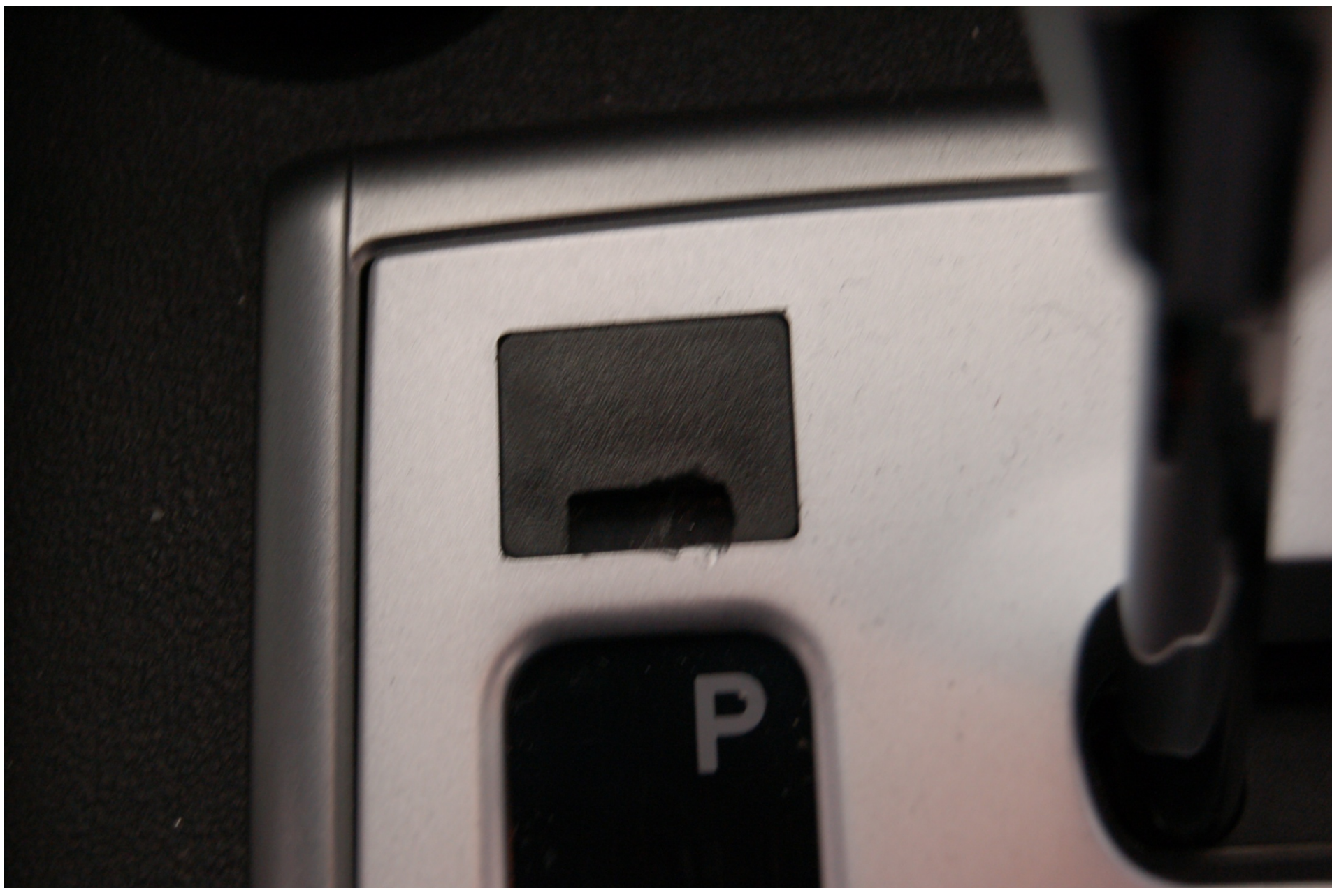
FIGURE 5.7 COVER OVER GEAR SELECTOR RELEASE
