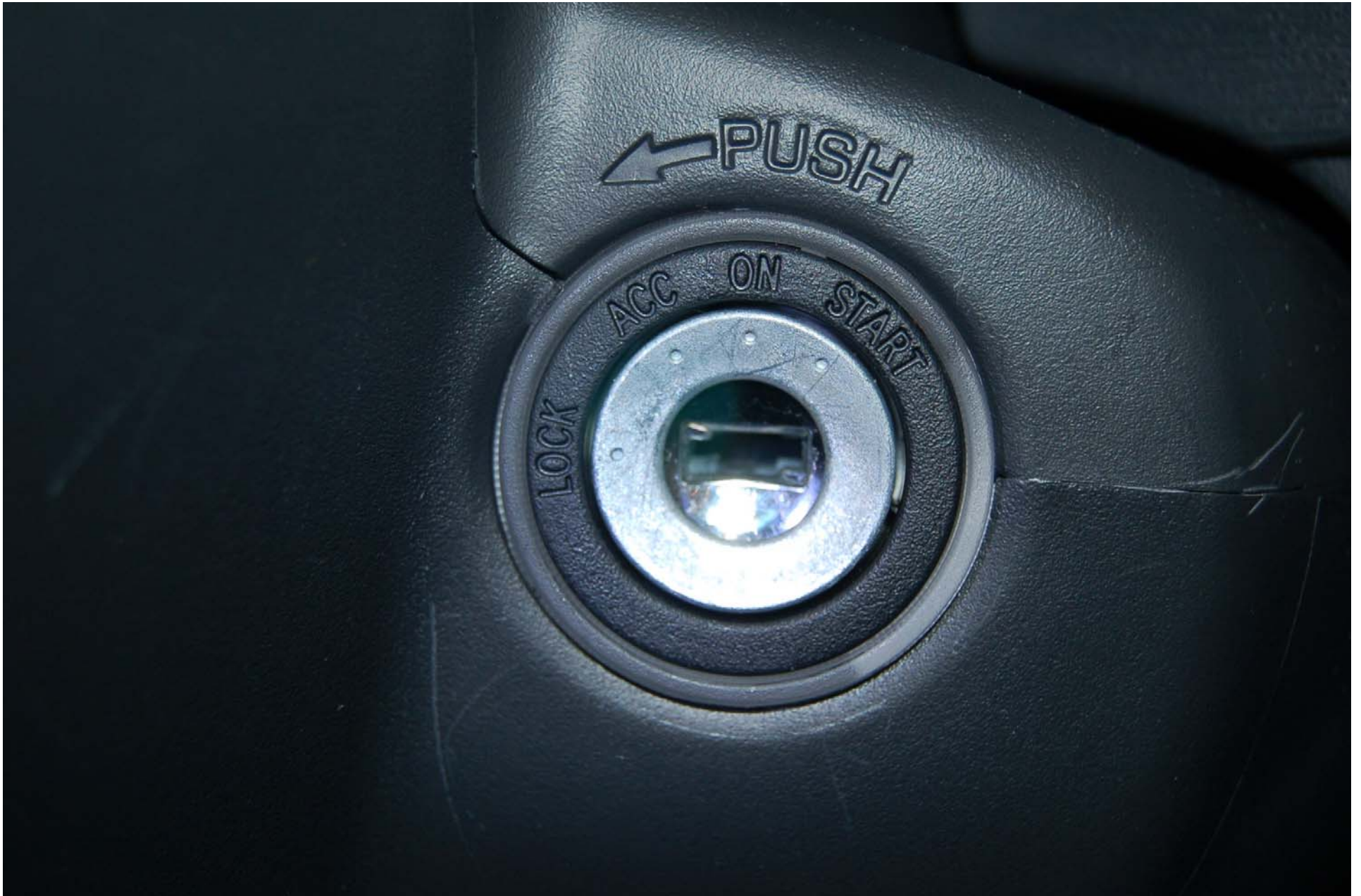
FIGURE 5.5 STARTING SYSTEM CONTROL
