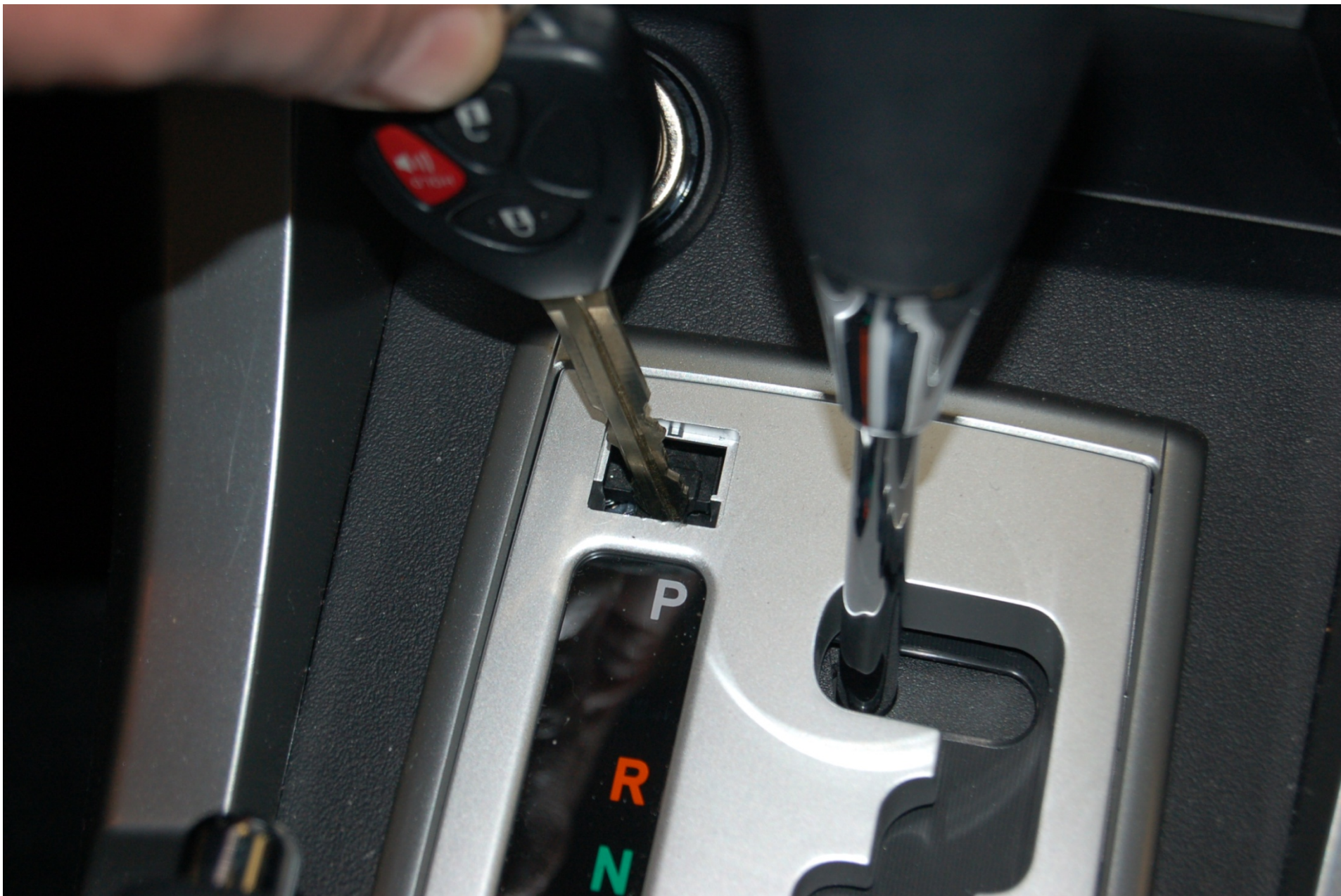
FIGURE 5.8 KEY INSERTED INTO GEAR SELECTOR RELEASE
