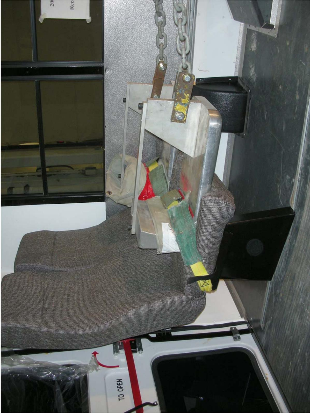
Post-Test of Seat S3 210 Test
