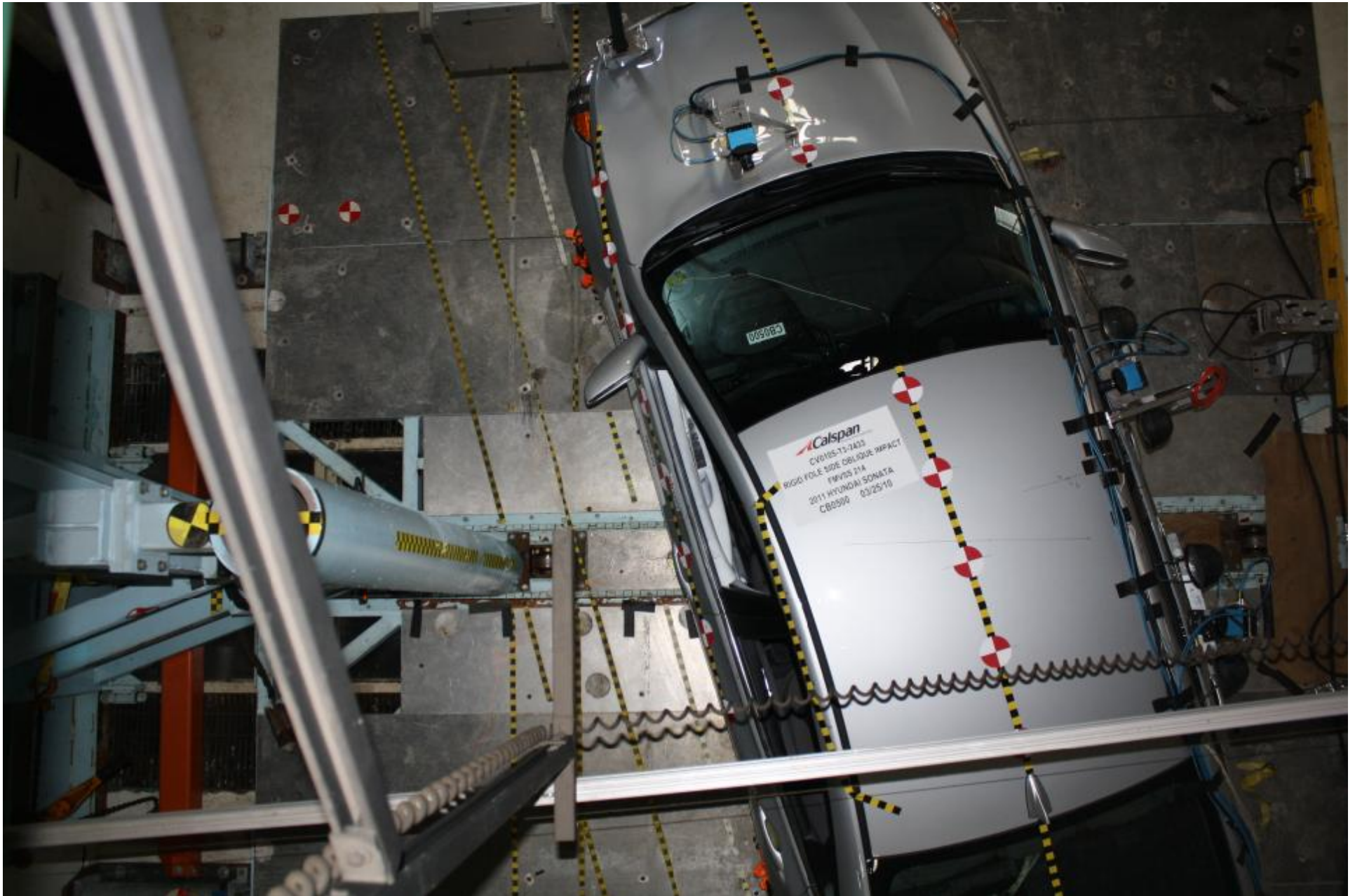
FIGURE A-9 : Pre-Test Overhead View of Aligned Vehicle and Pole
