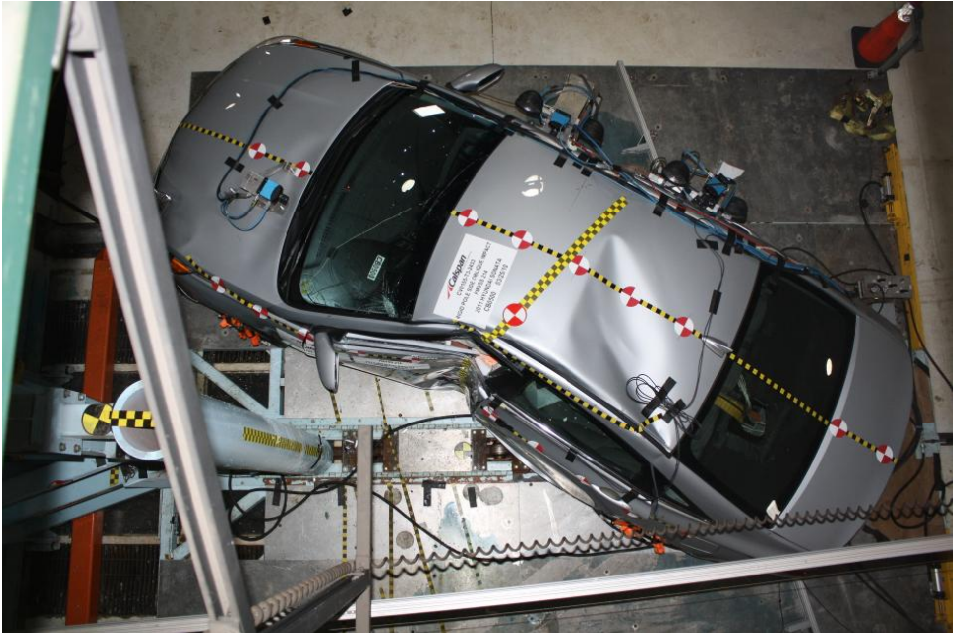
FIGURE A-10 : Post-Test Overhead View of Aligned Vehicle and Pole
