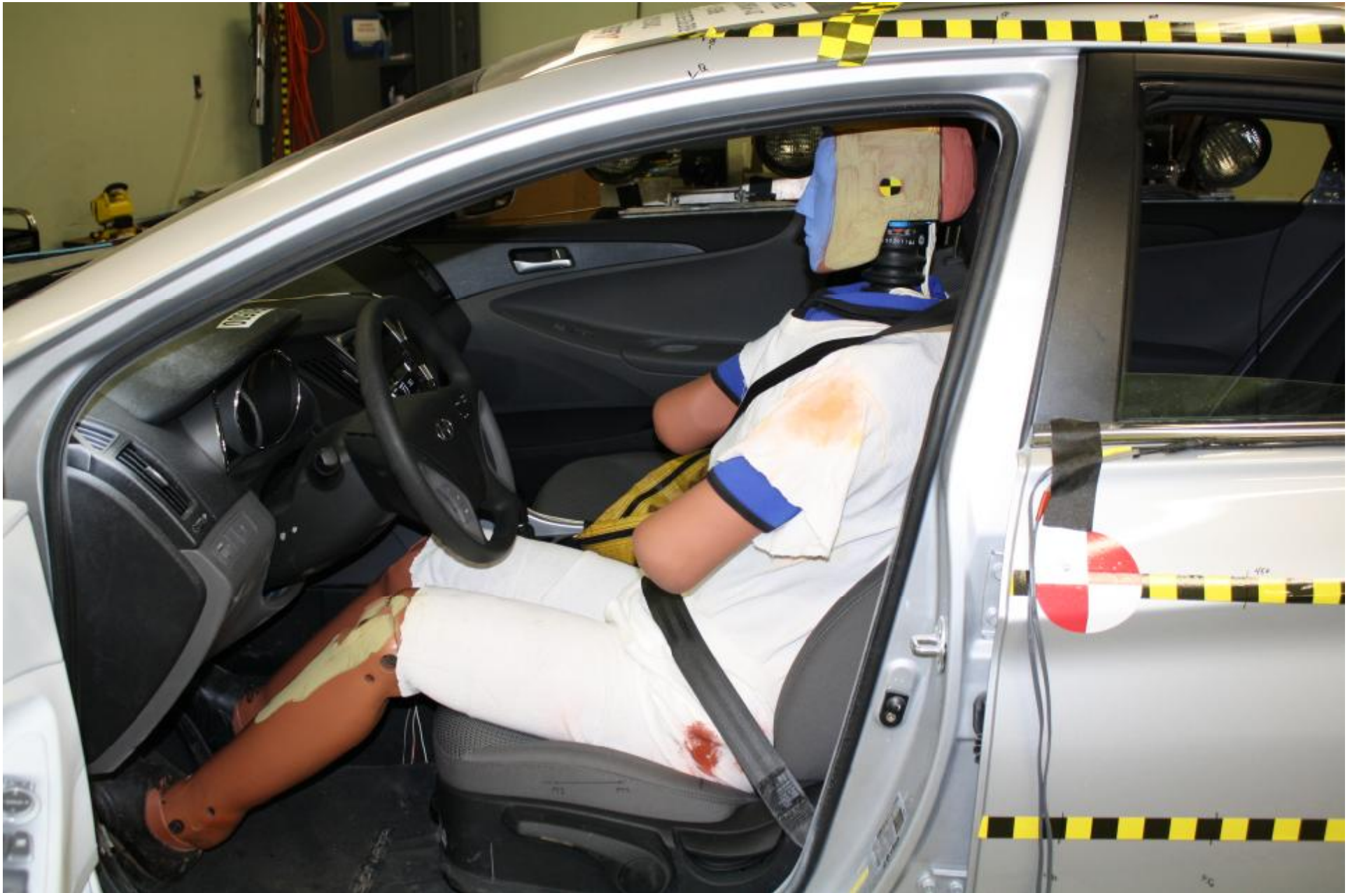
FIGURE A-15 : Pre-Test Dummy Door Open
