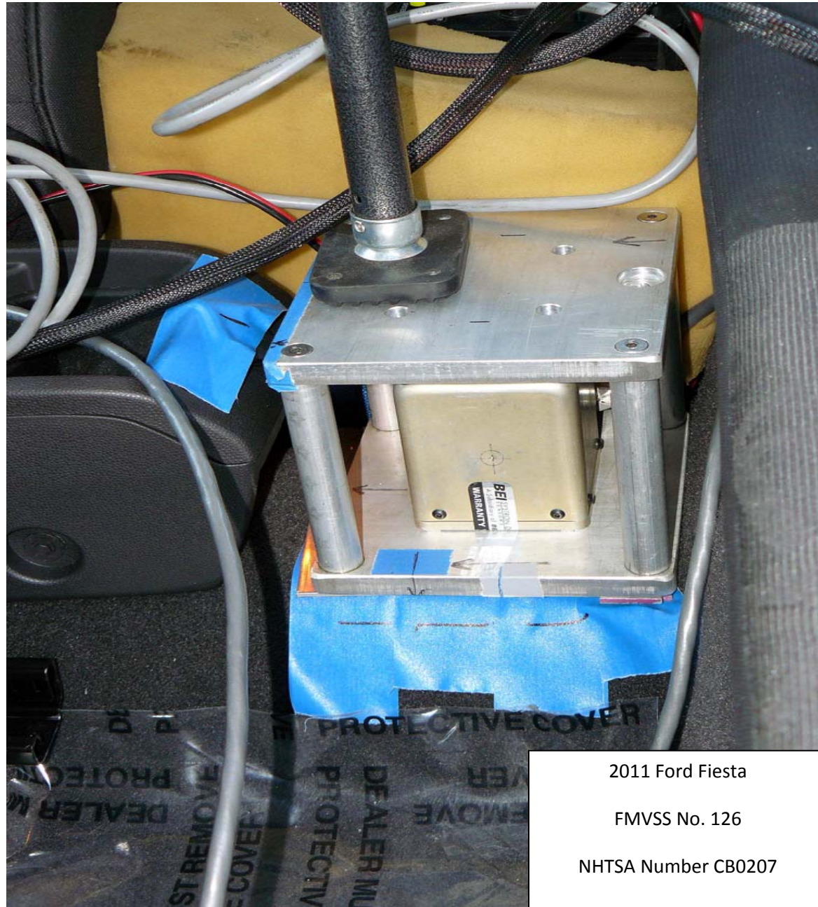
Figure 5.11. Inertial Measurement Unit Mounted in Vehicle
