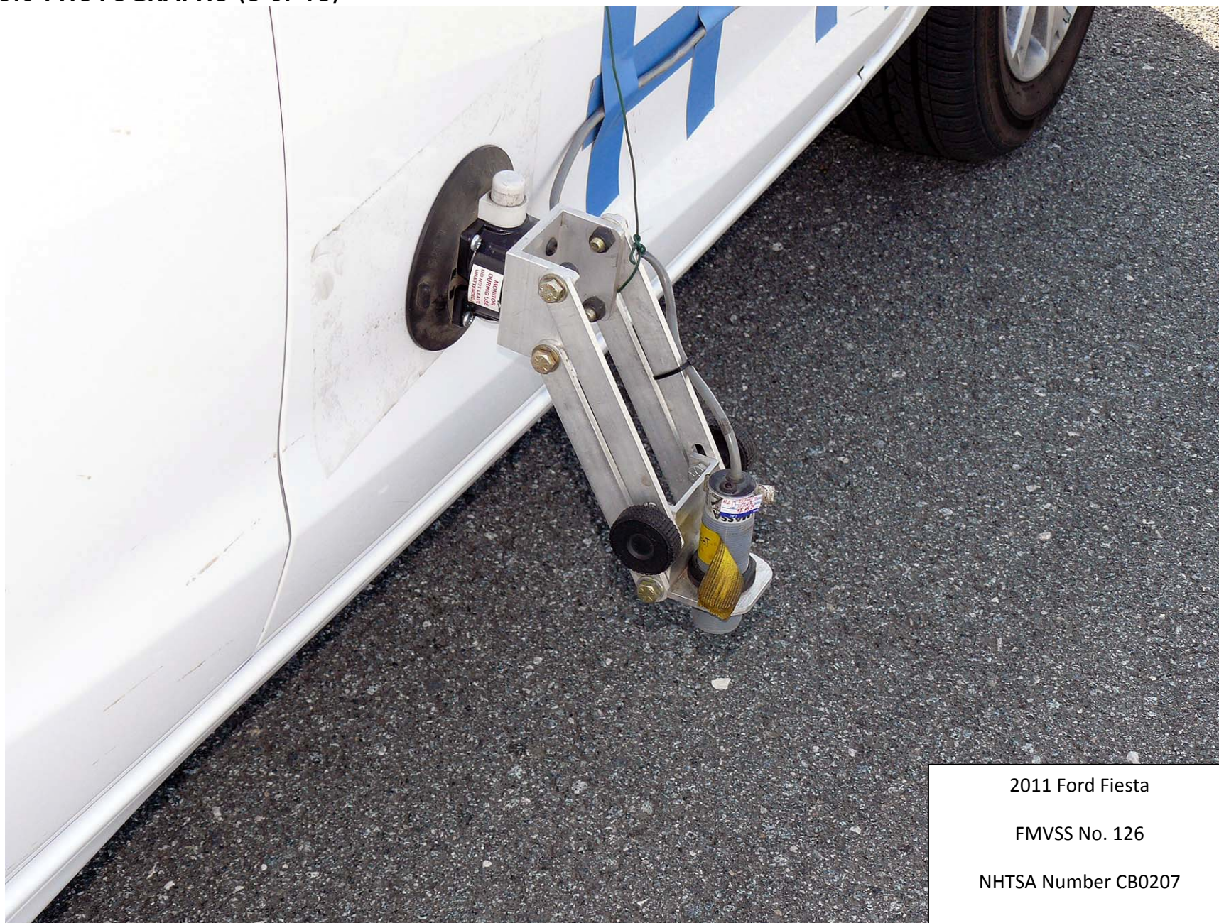
Figure 5.8. Ultrasonic Height Sensor Mounted on Side of Vehicle for Determining Body Roll Angle
