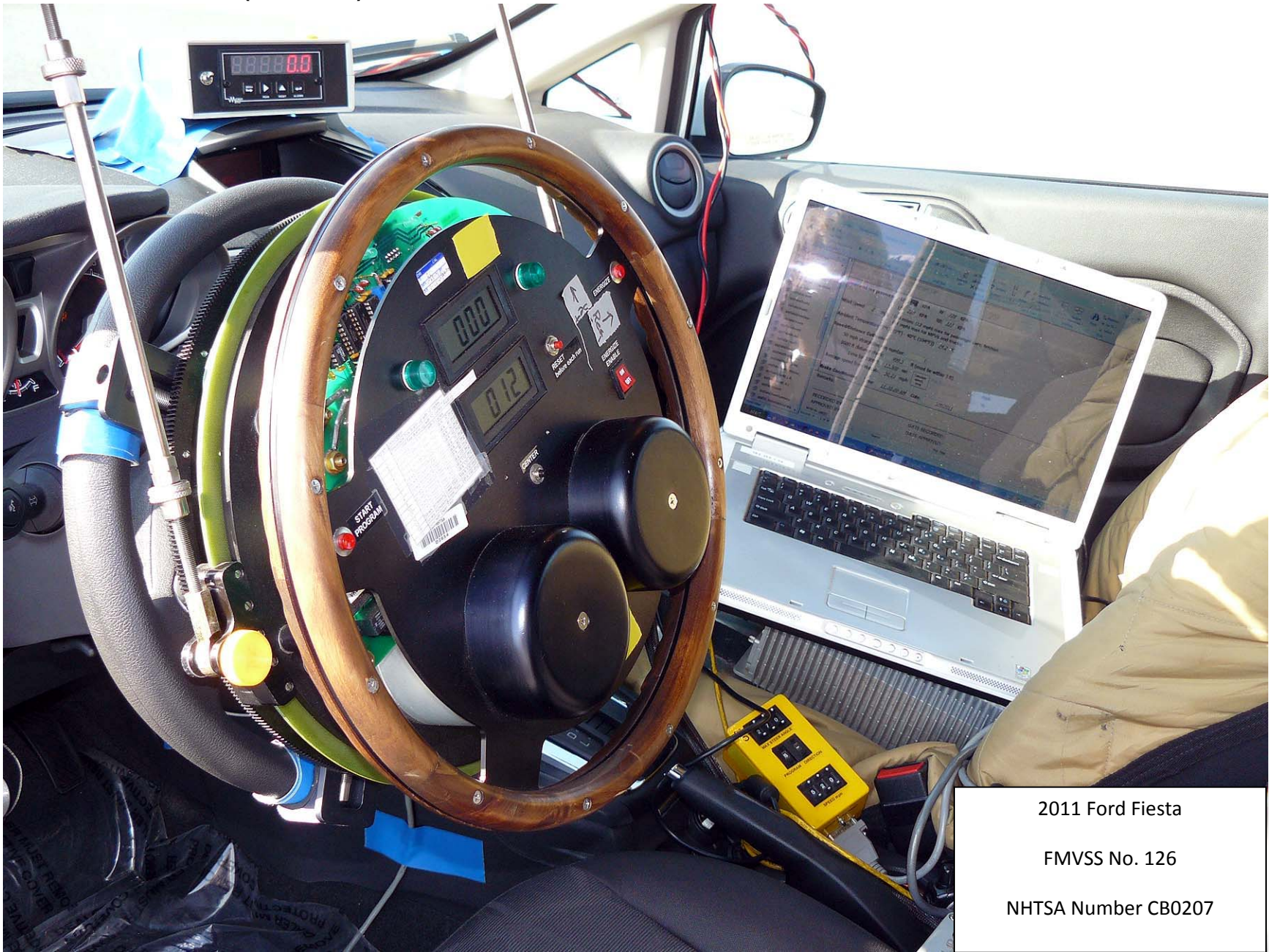
Figure 5.10. Steering Controller and Data Acquisition Computer
