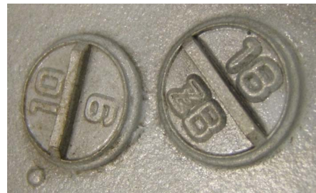
FIGURE 5.10 RIM MARKINGS INCLUDING MANUFACTURE DATE, SIZE, MANUFACTURER'S SYMBOL, DOT SYMBOL, LETTER DESIGNATION FOR SOURCE OF PUBLISHED DIMENSIONS,, AND OTHER RIM MARKINGS
