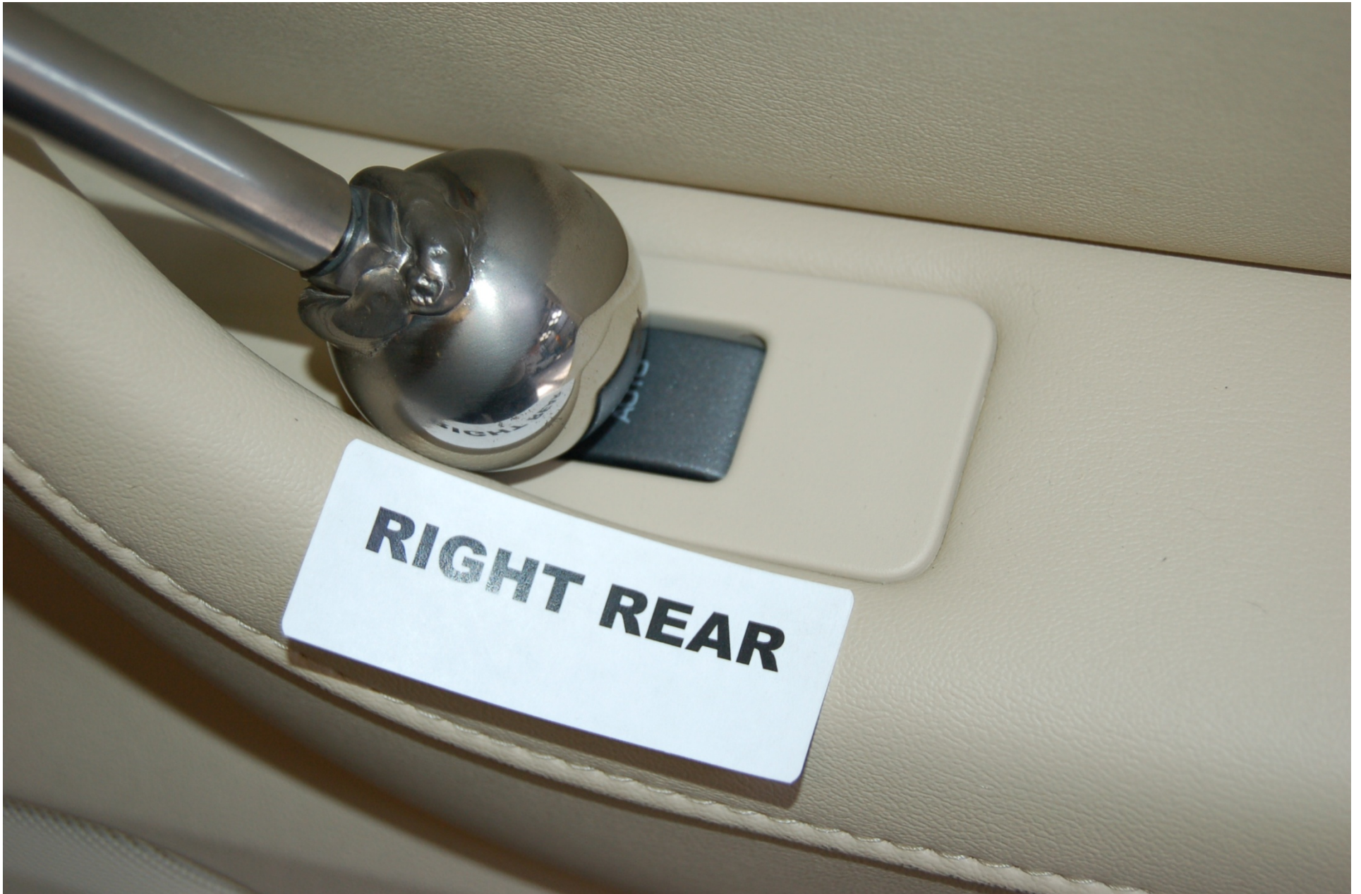
FIGURE 5.13 SPHERE TEST ON RIGHT REAR SWITCH
