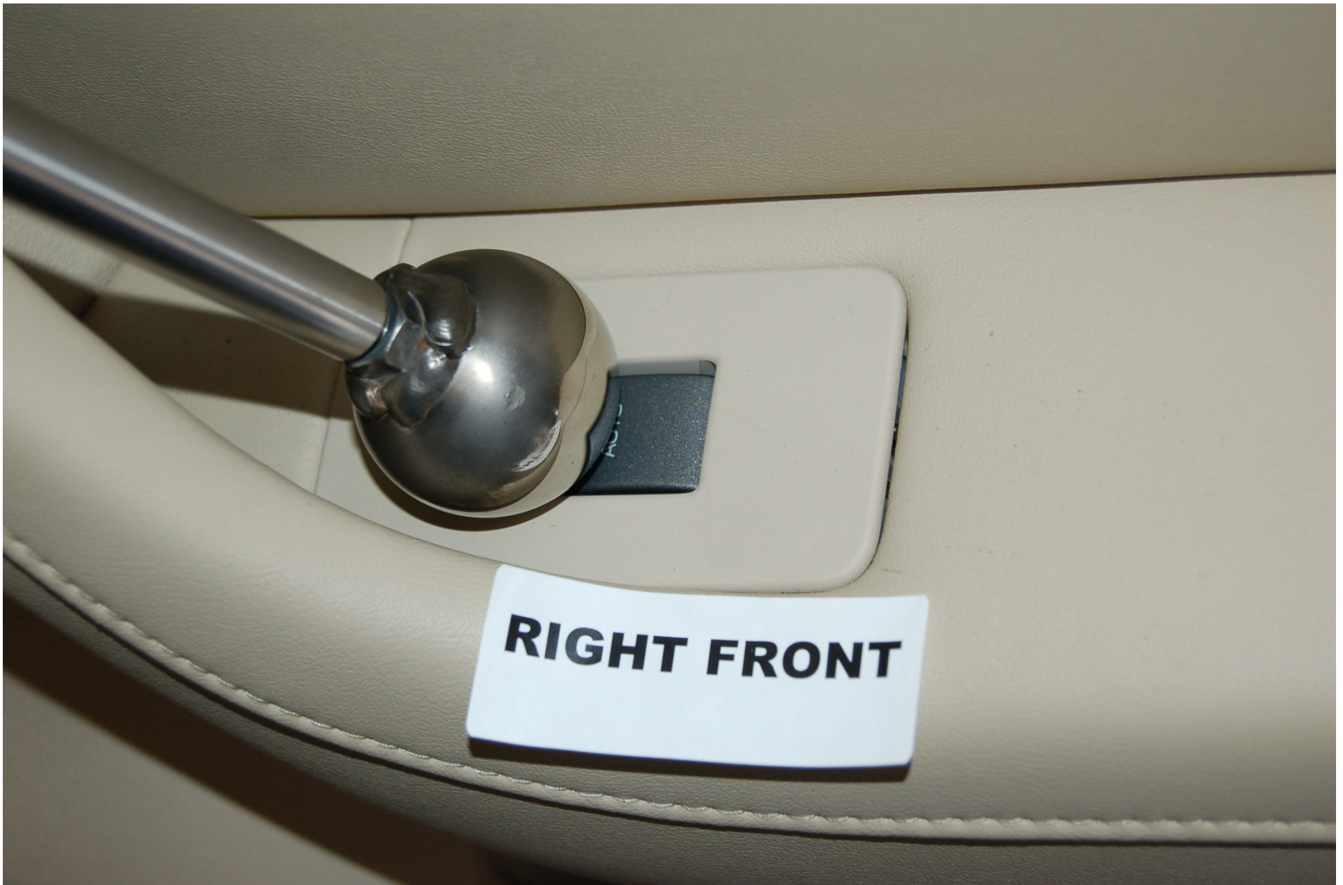
FIGURE 5.11 SPHERE TEST ON RIGHT FRONT SWITCH
