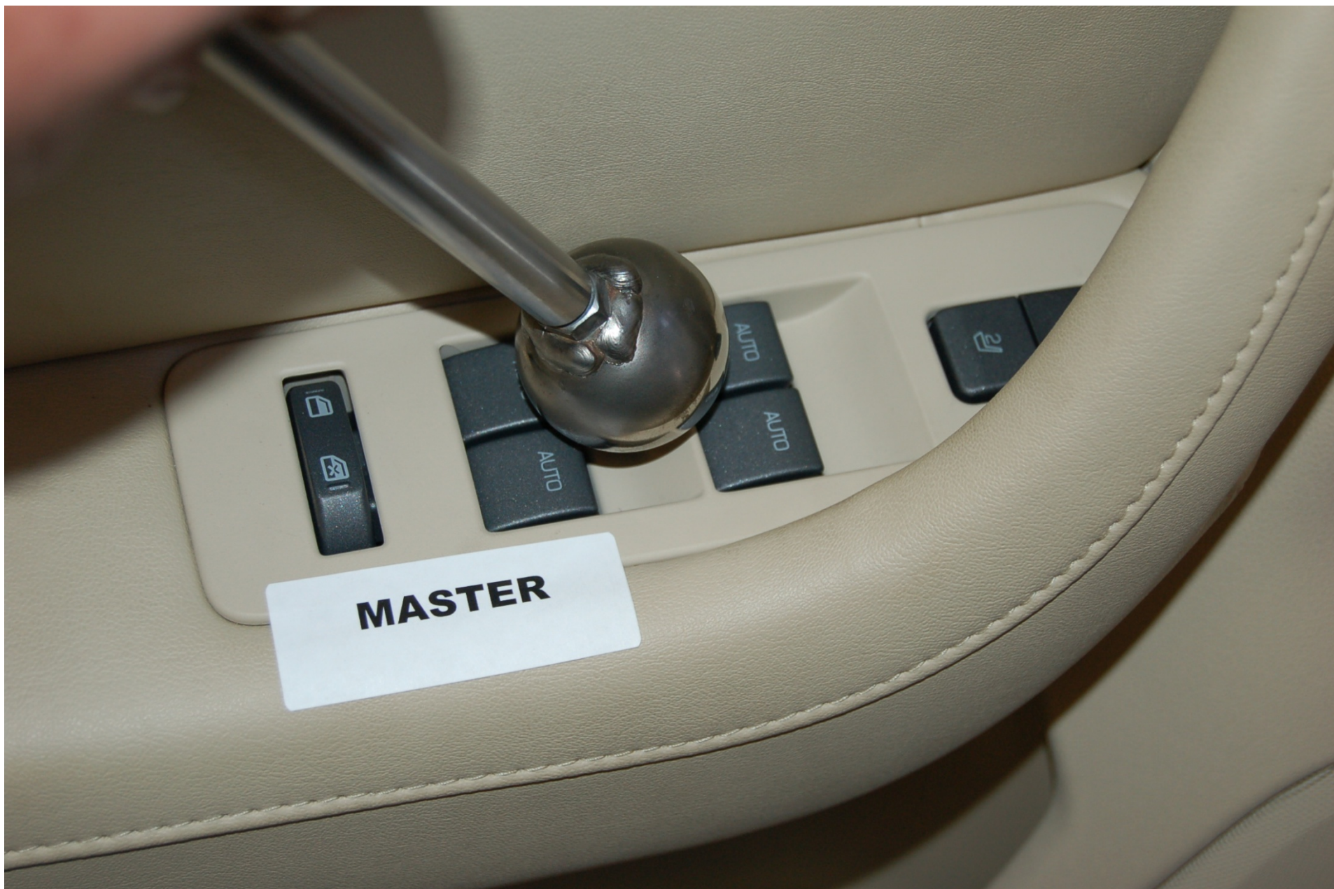
FIGURE 5.10 SPHERE TEST ON MASTER SWITCH
