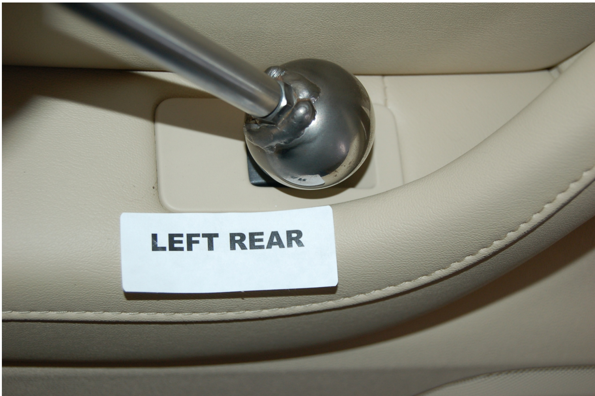
FIGURE 5.12 SPHERE TEST ON LEFT REAR SWITCH
