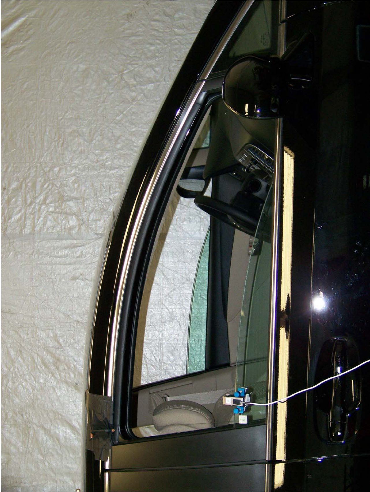
Figure 19: Right Front Window Test Set-Up Rear Edge
