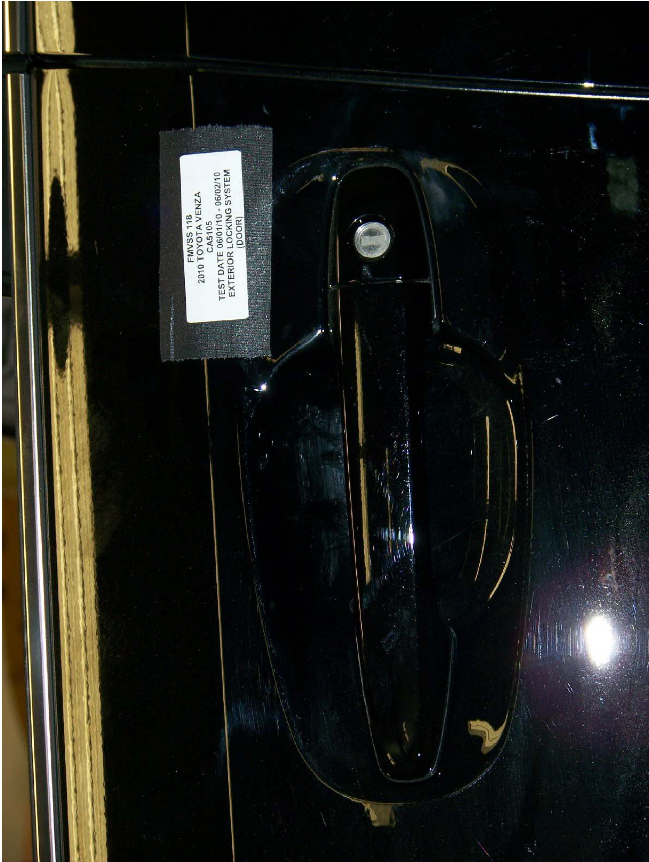
Figure 10: Exterior Locking System (Driver Door)
