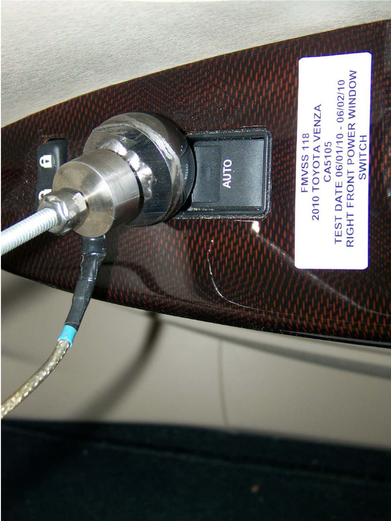
Figure 27: Sphere Test Right Front Window Switch
