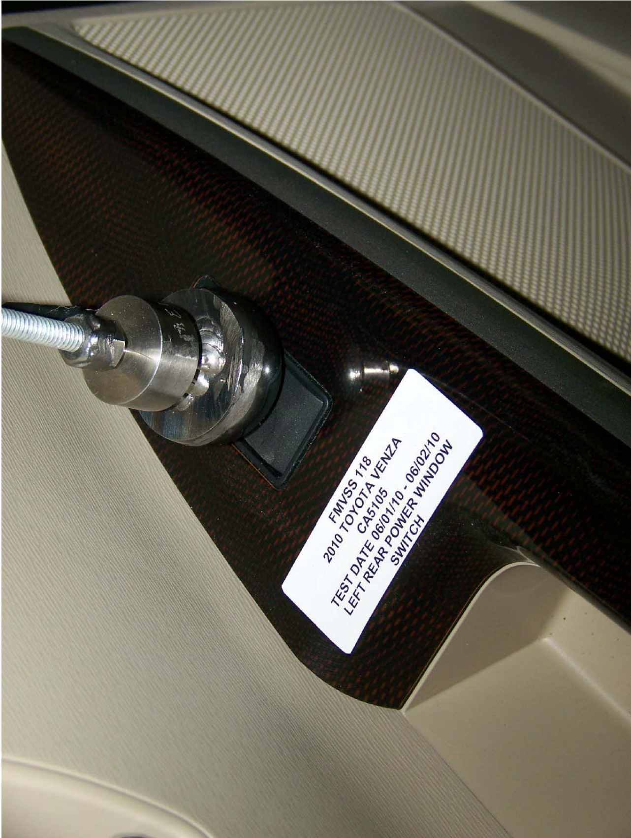
Figure 28: Sphere Test Left Rear Window Switch
