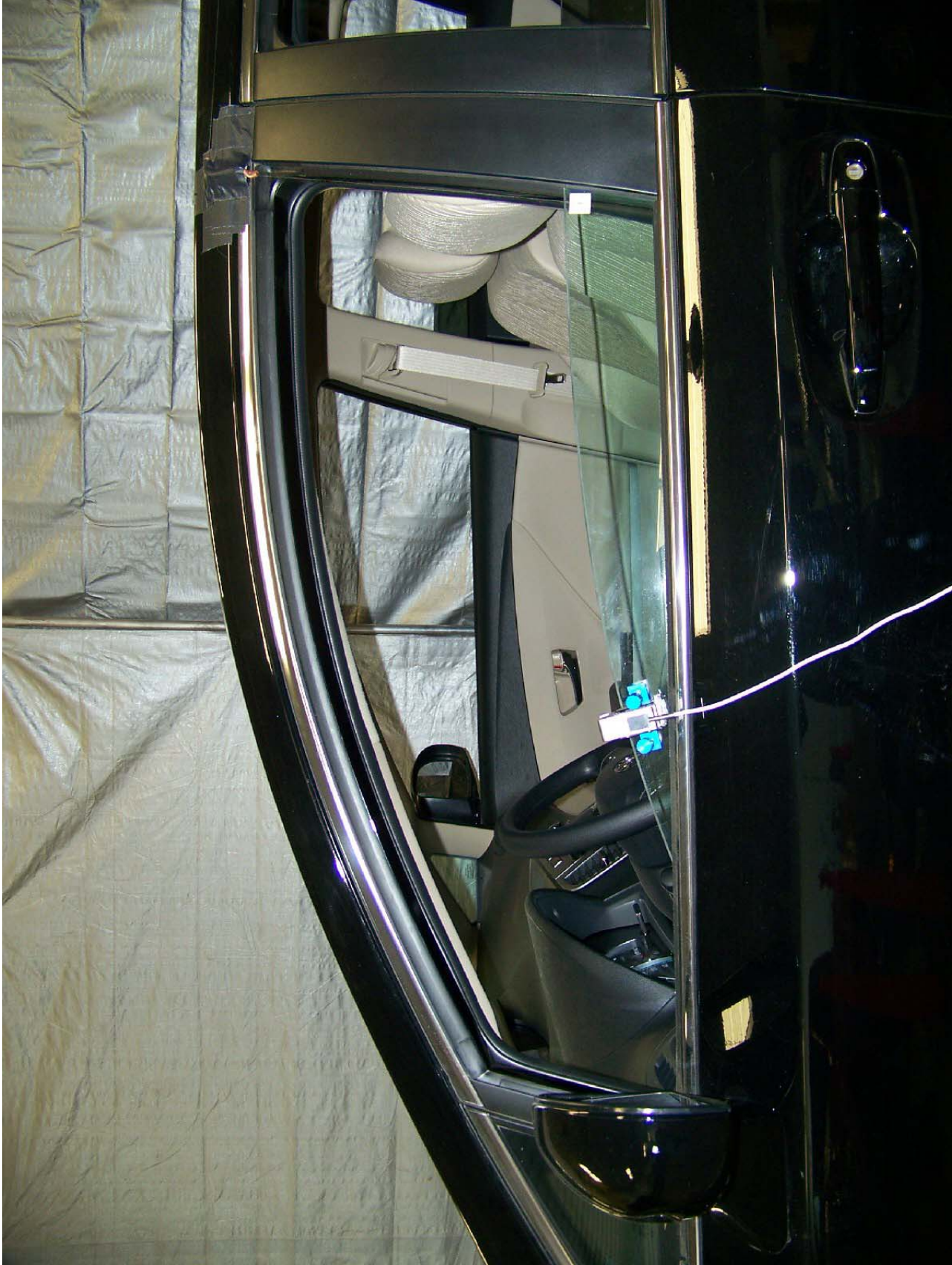
Figure 15: Left Front Window Test Set-Up Leading Edge
