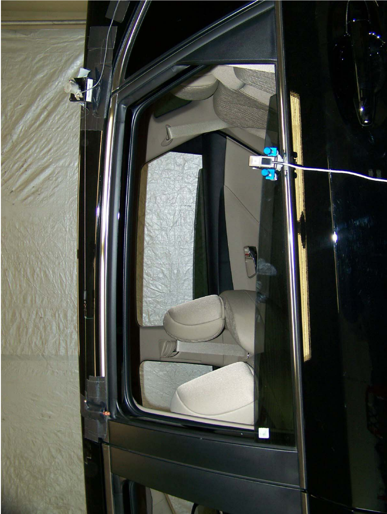
Figure 22: Left Rear Window Test Set-Up Rear Edge
