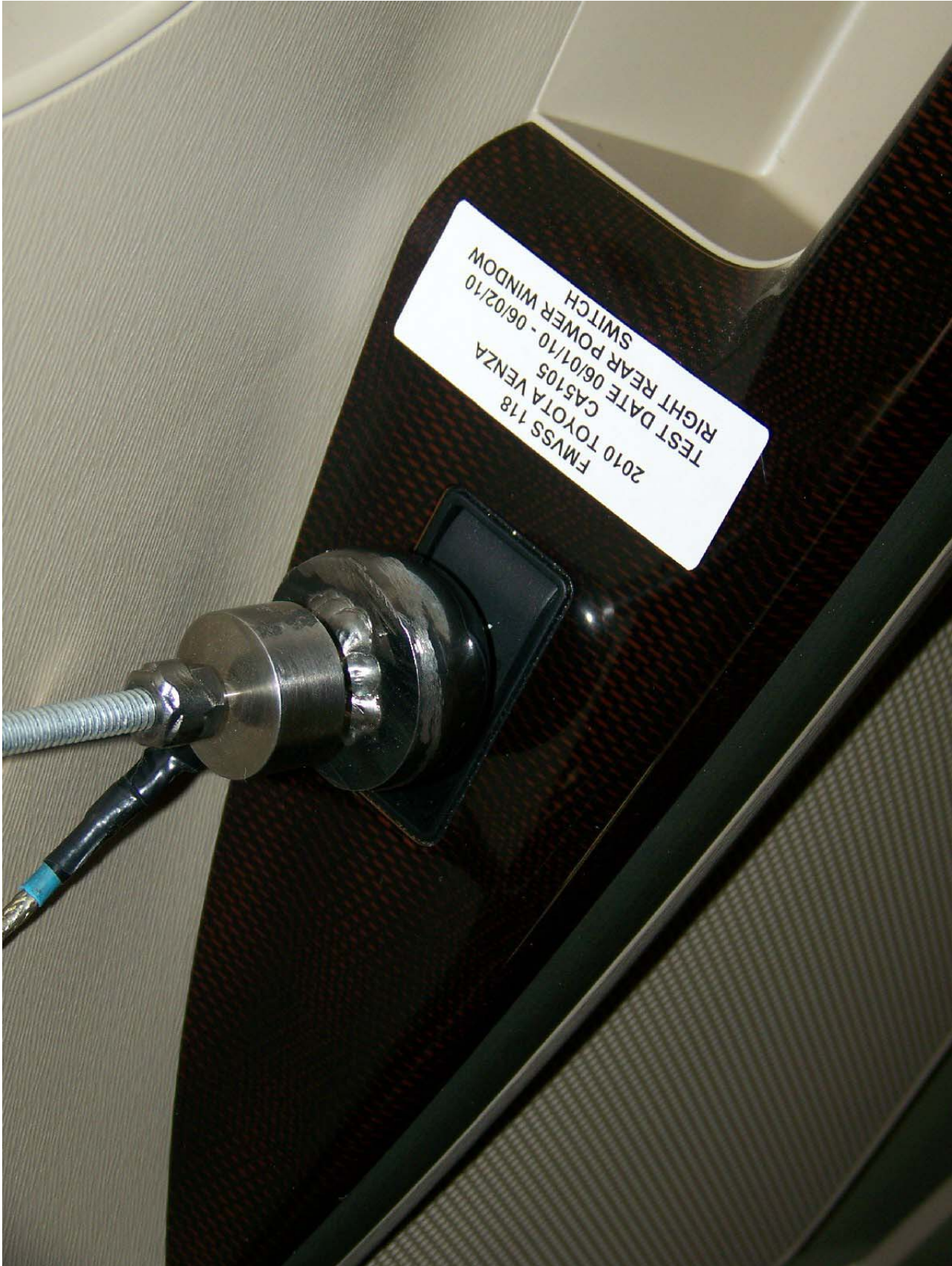
Figure 29: Sphere Test Right Rear Window Switch
