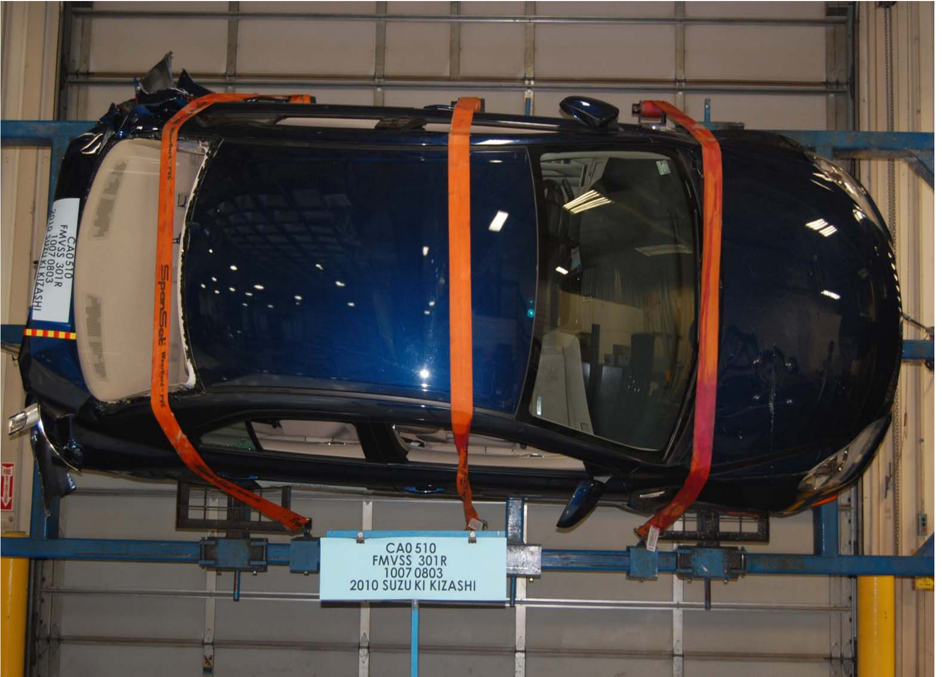
Static Rollover at 270 Degrees
