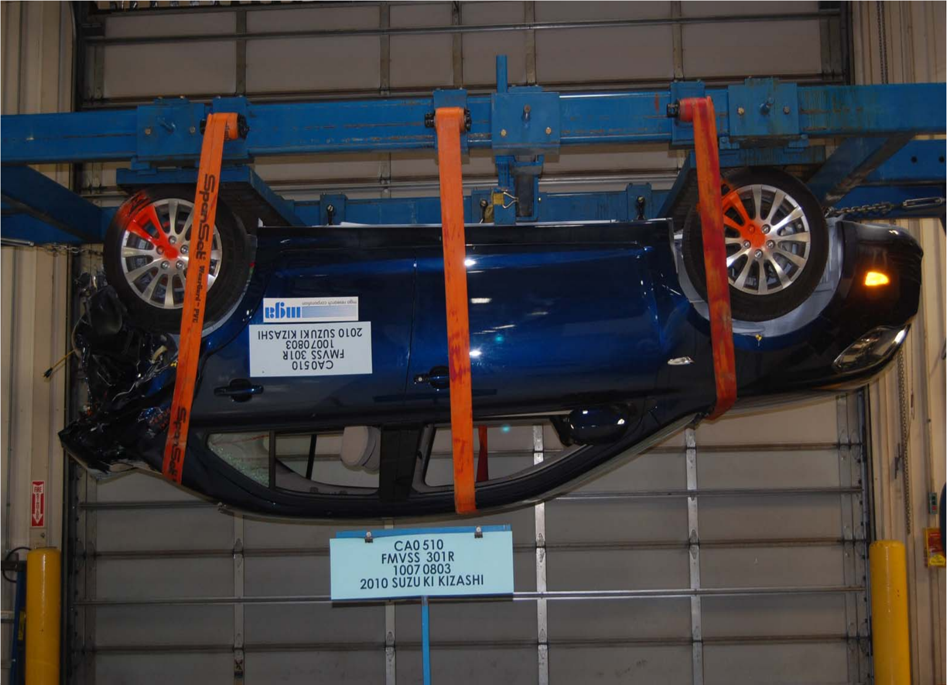
Static Rollover at 180 Degrees
