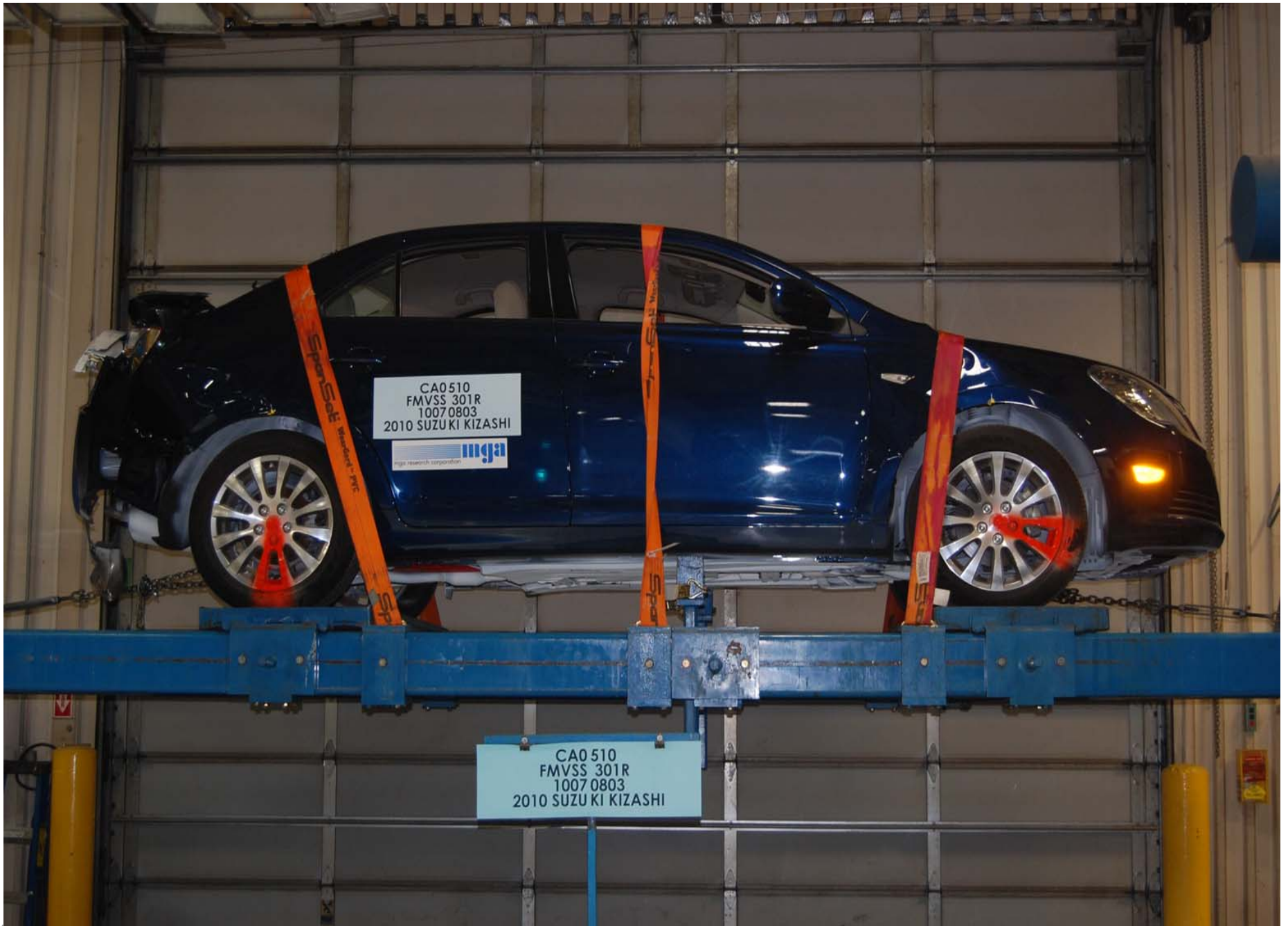
Static Rollover at 360 Degrees
