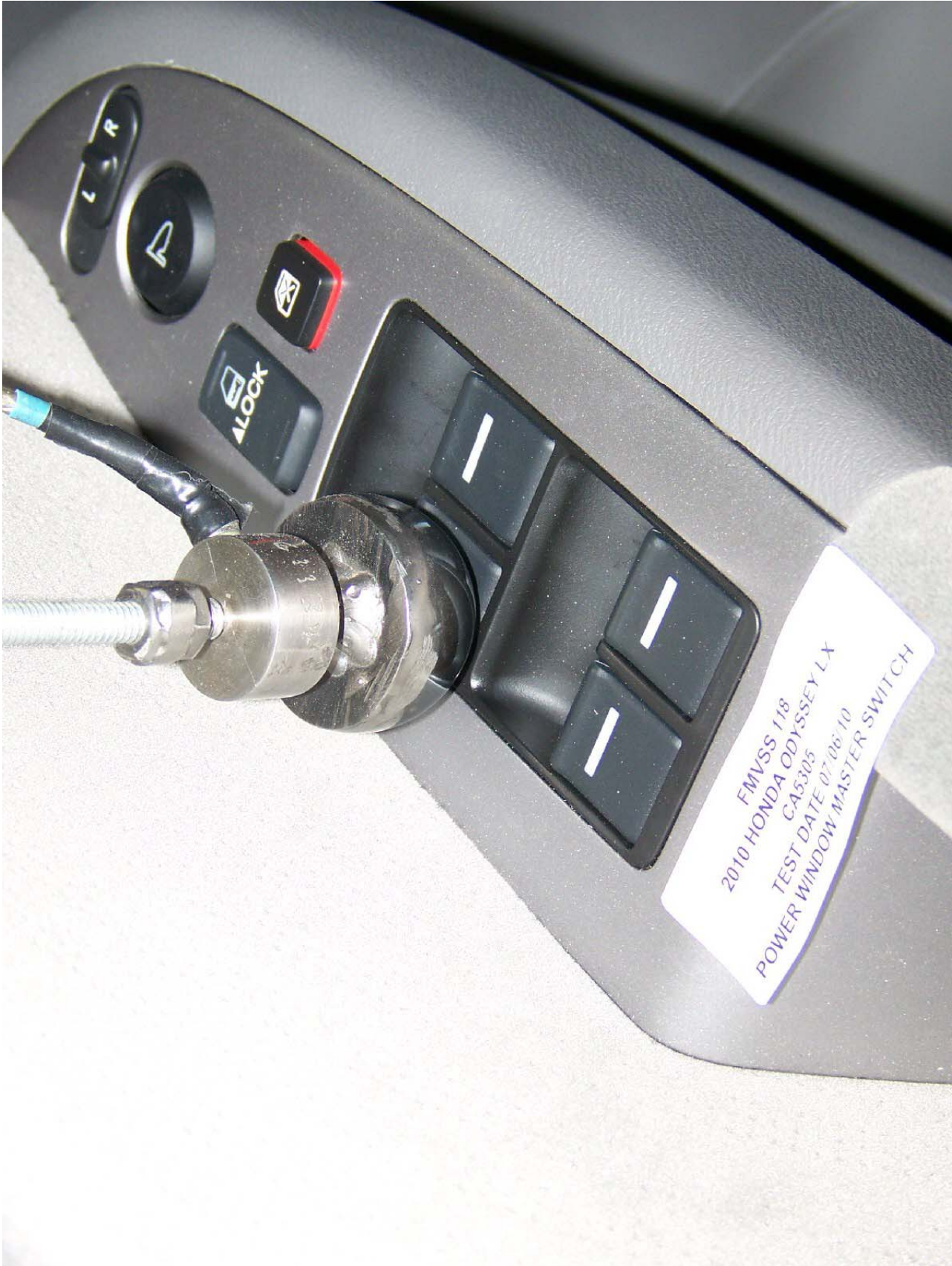
Figure 17: Sphere Test Master Control Panel
