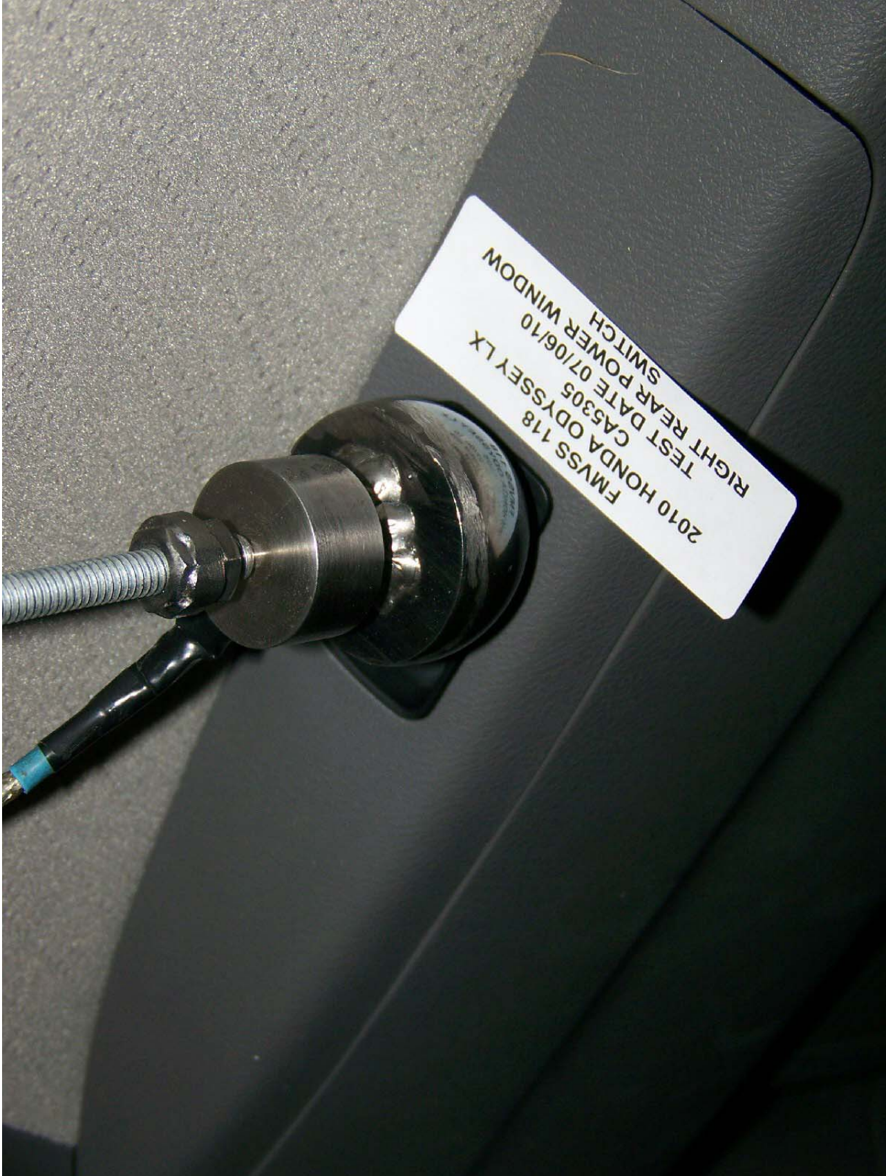
Figure 20: Sphere Test Right Rear Window Switch
