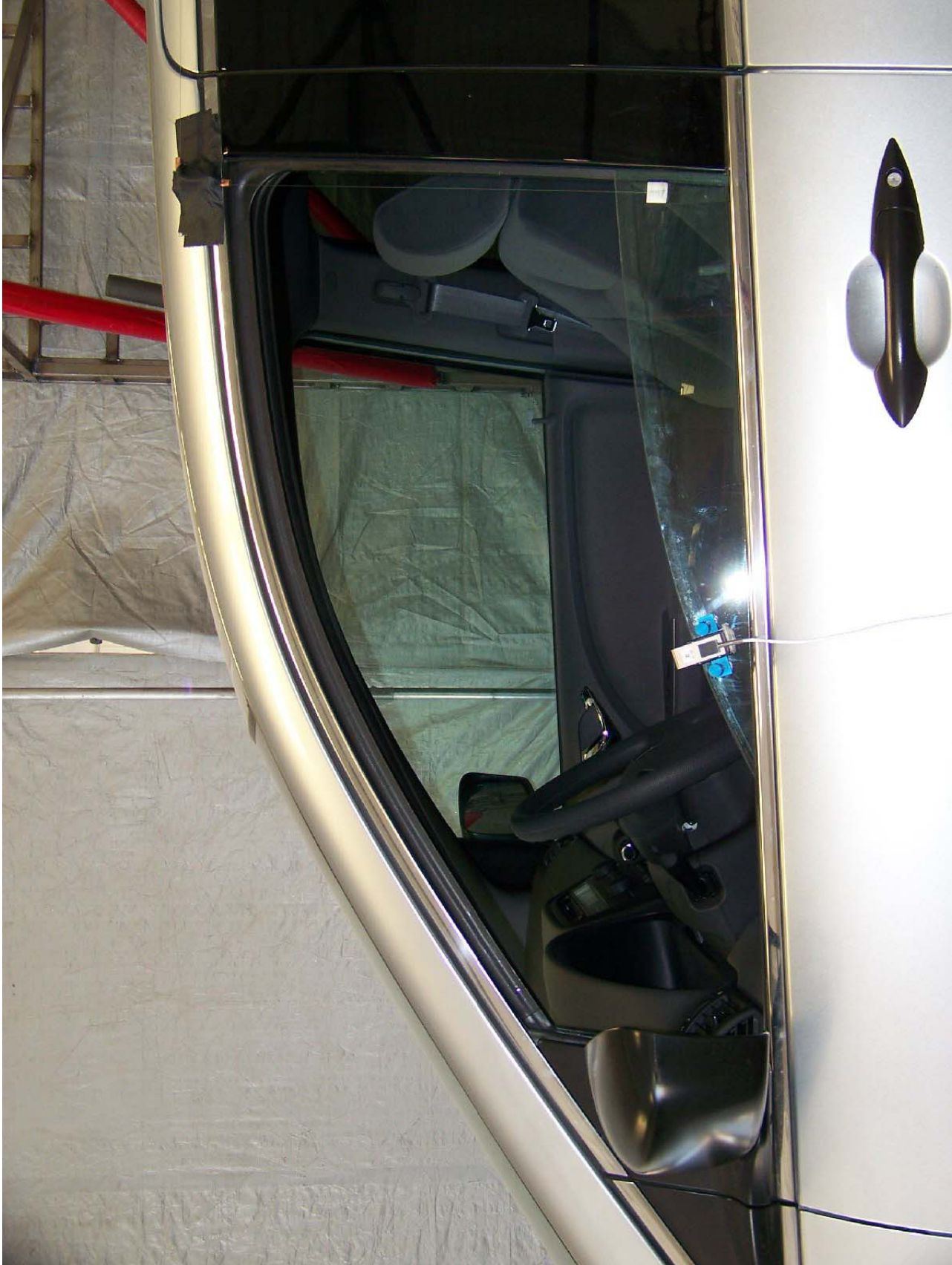
Figure 15: Left Front Window Test Set-Up Leading Edge
