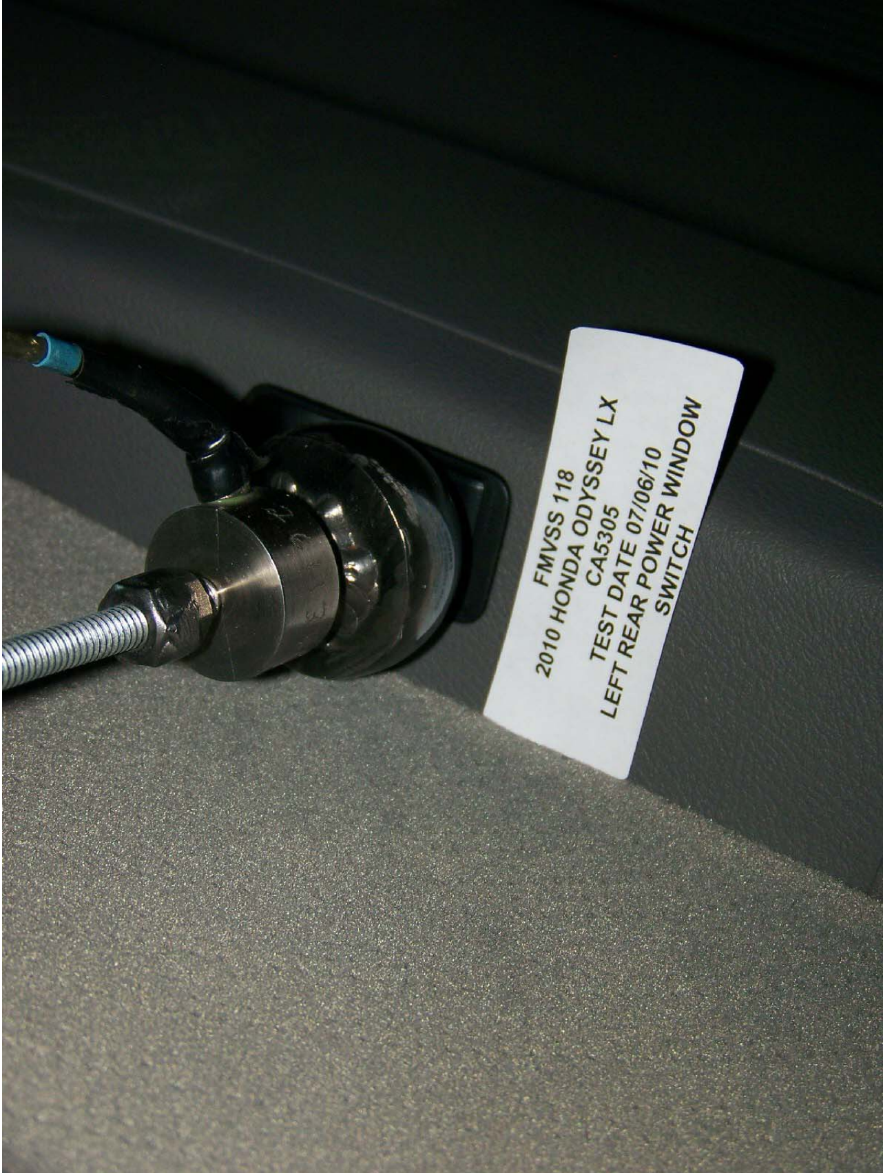
Figure 19: Sphere Test Left Rear Window Switch
