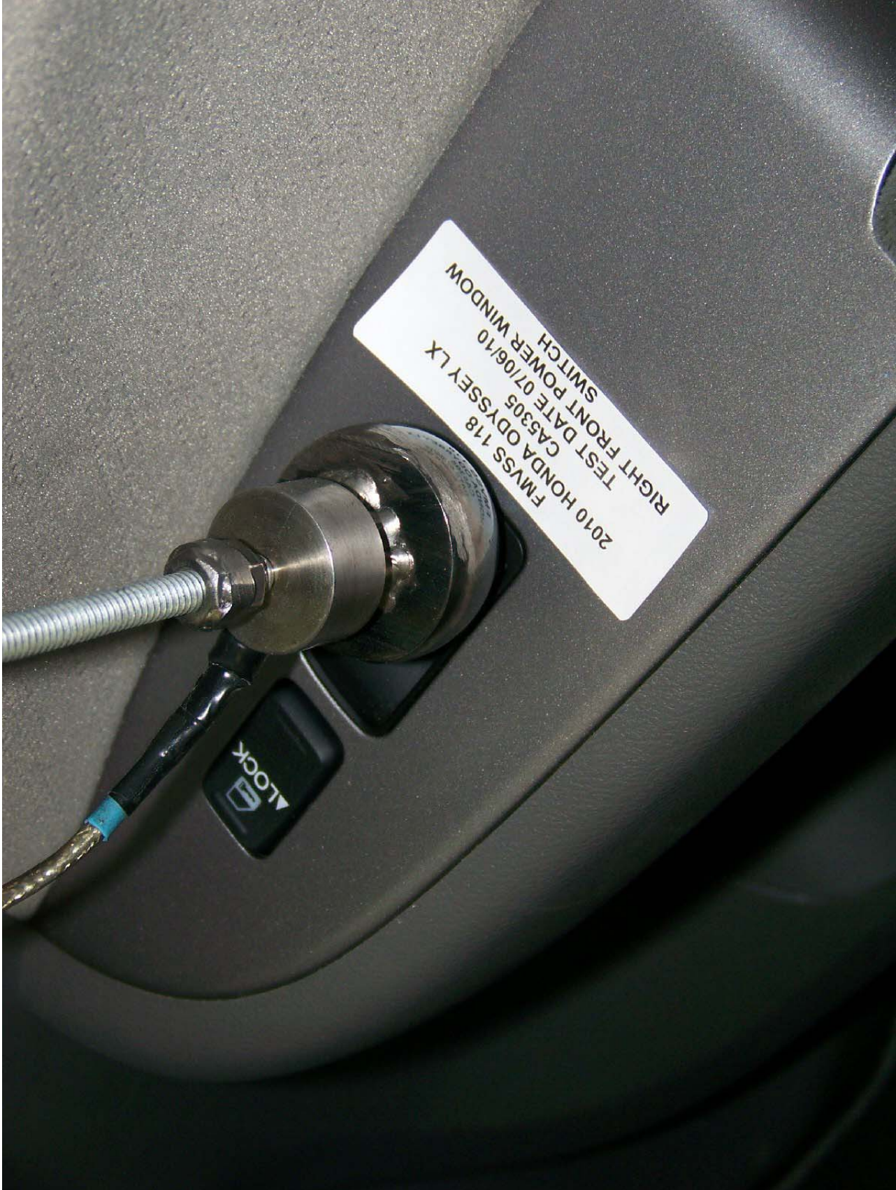
Figure 18: Sphere Test Right Front Window Switch
