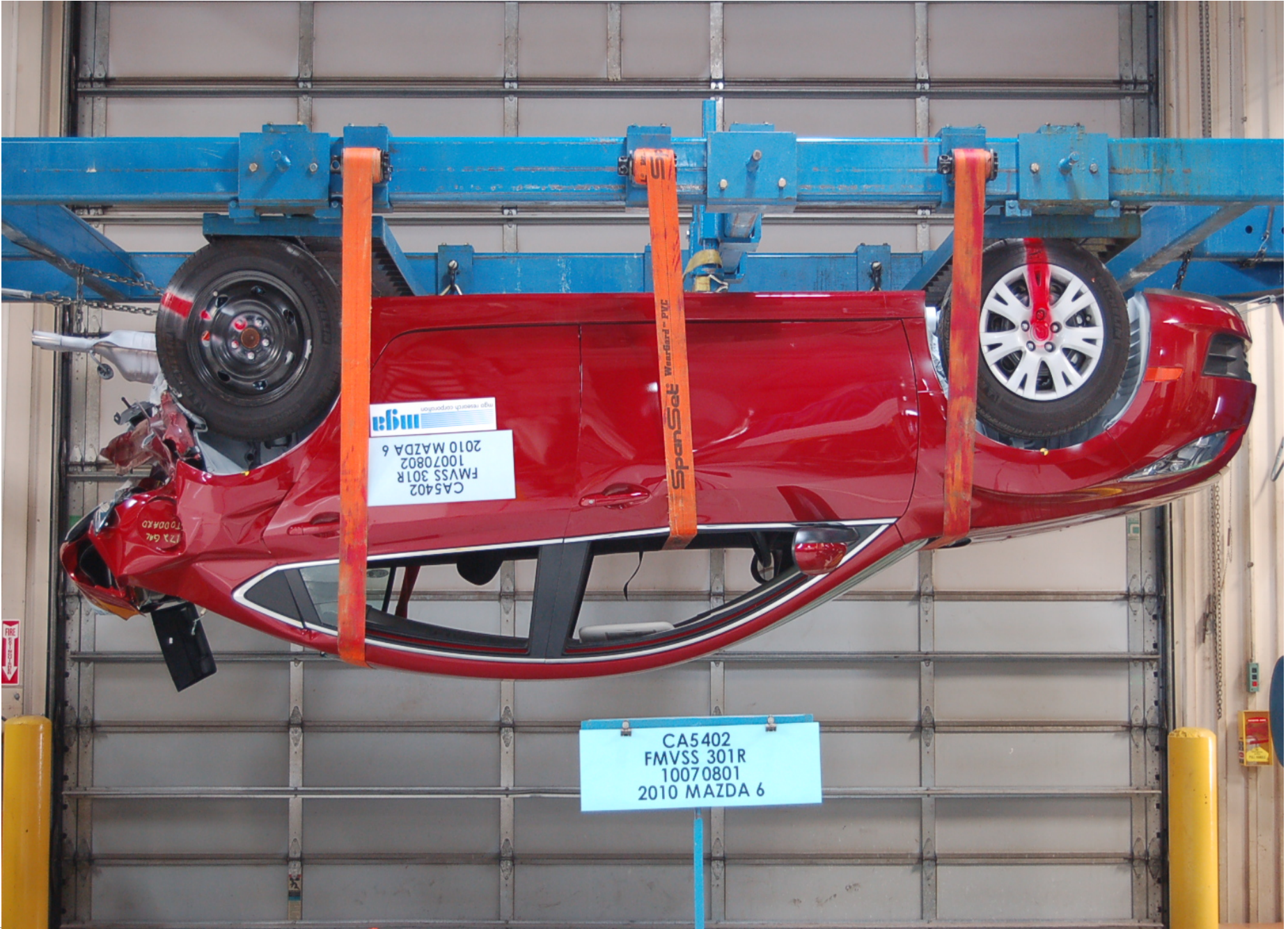
Static Rollover at 180 Degrees
