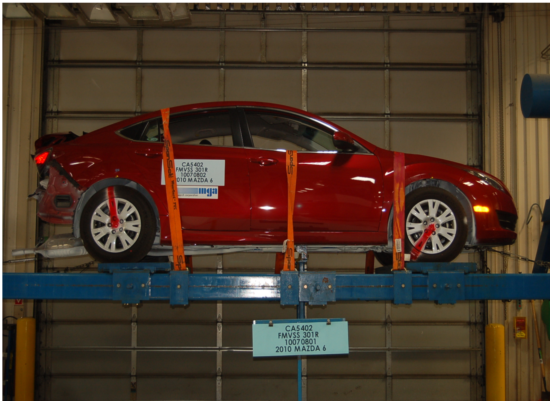
Static Rollover at 360 Degrees
