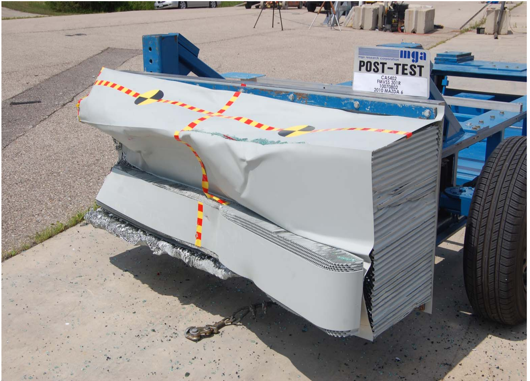
Post-Test \frac{3}{4} Left Side View of MDB
