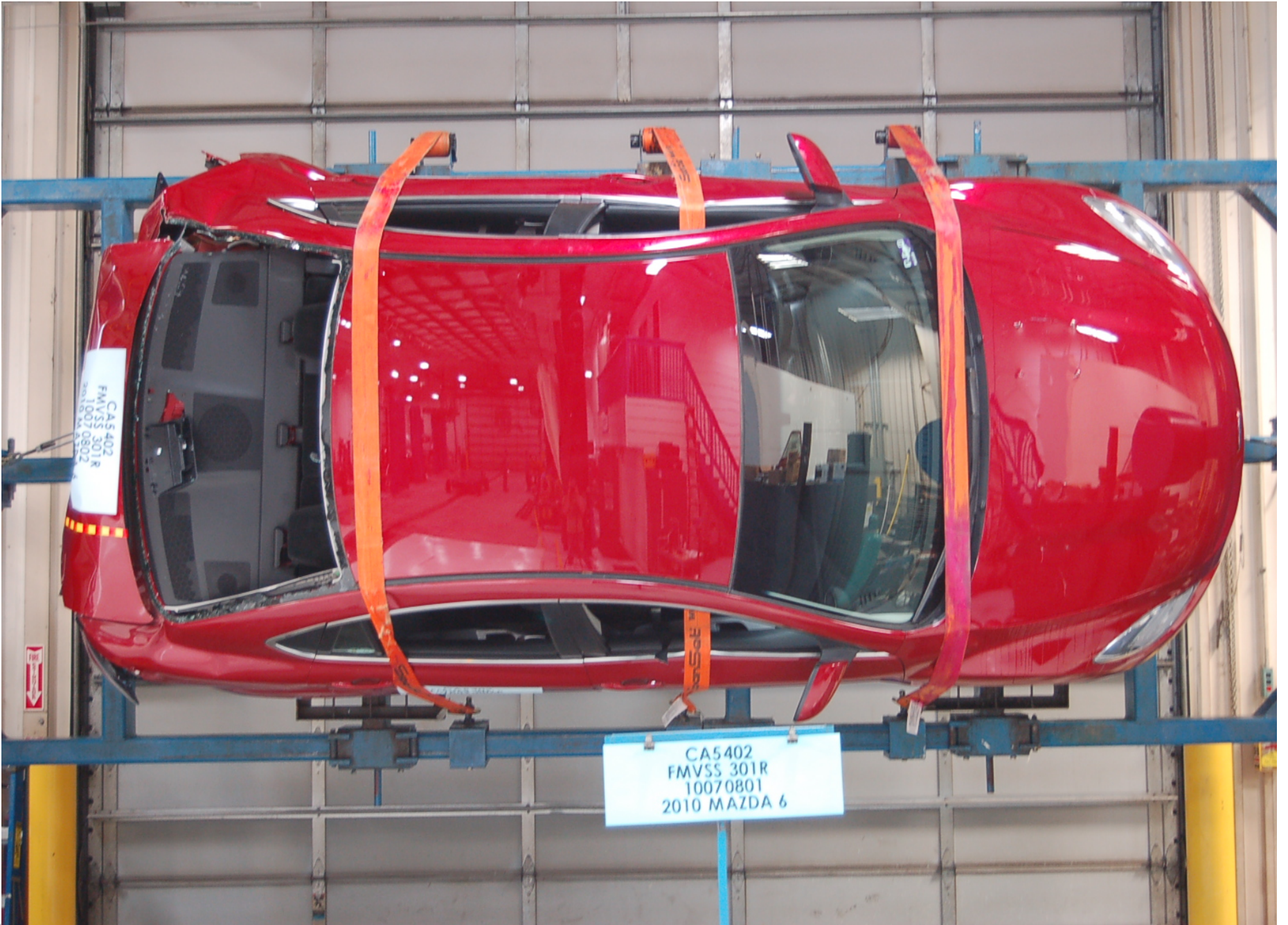
Static Rollover at 90 Degrees
