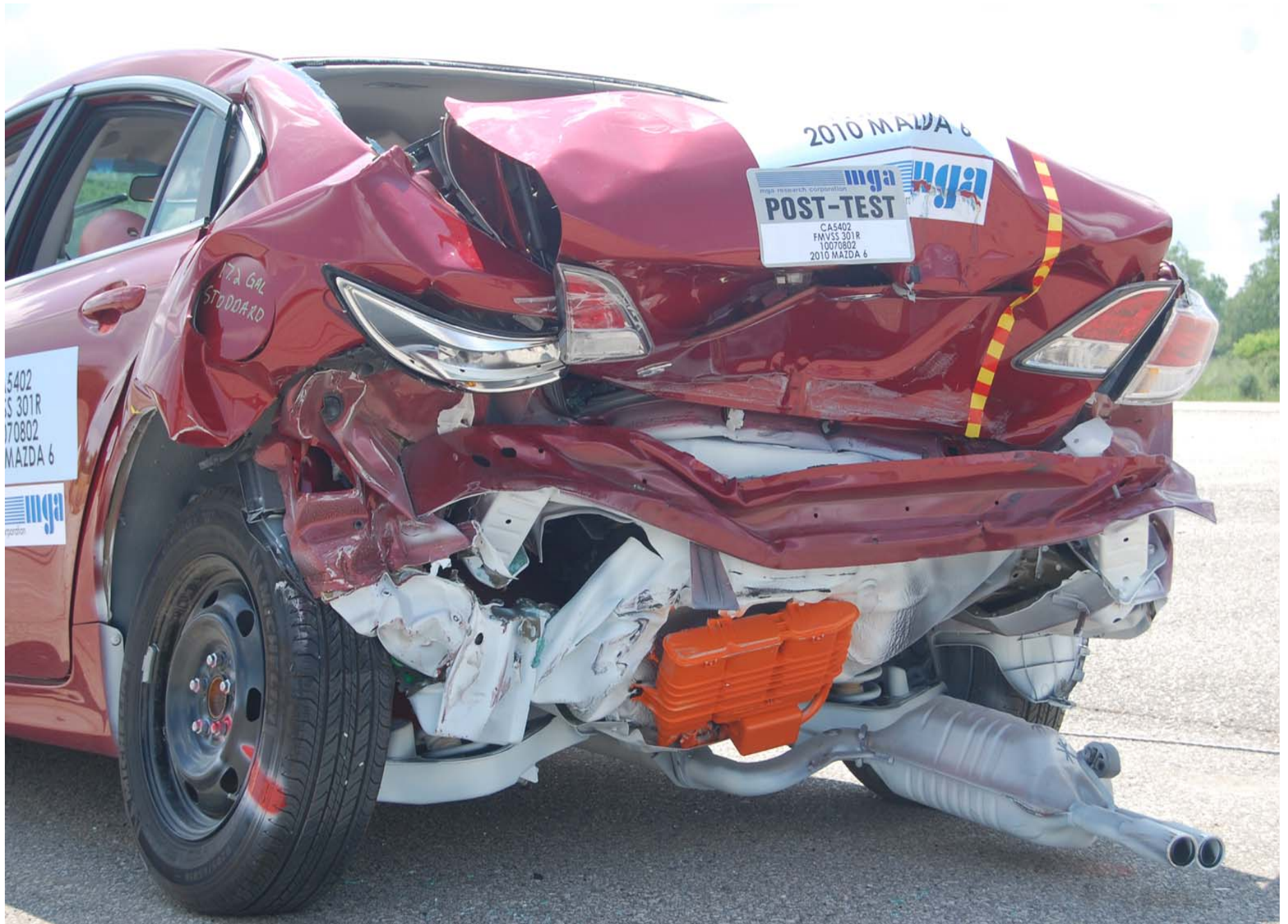
Post-Test Left Rear Close-up View of Vehicle
