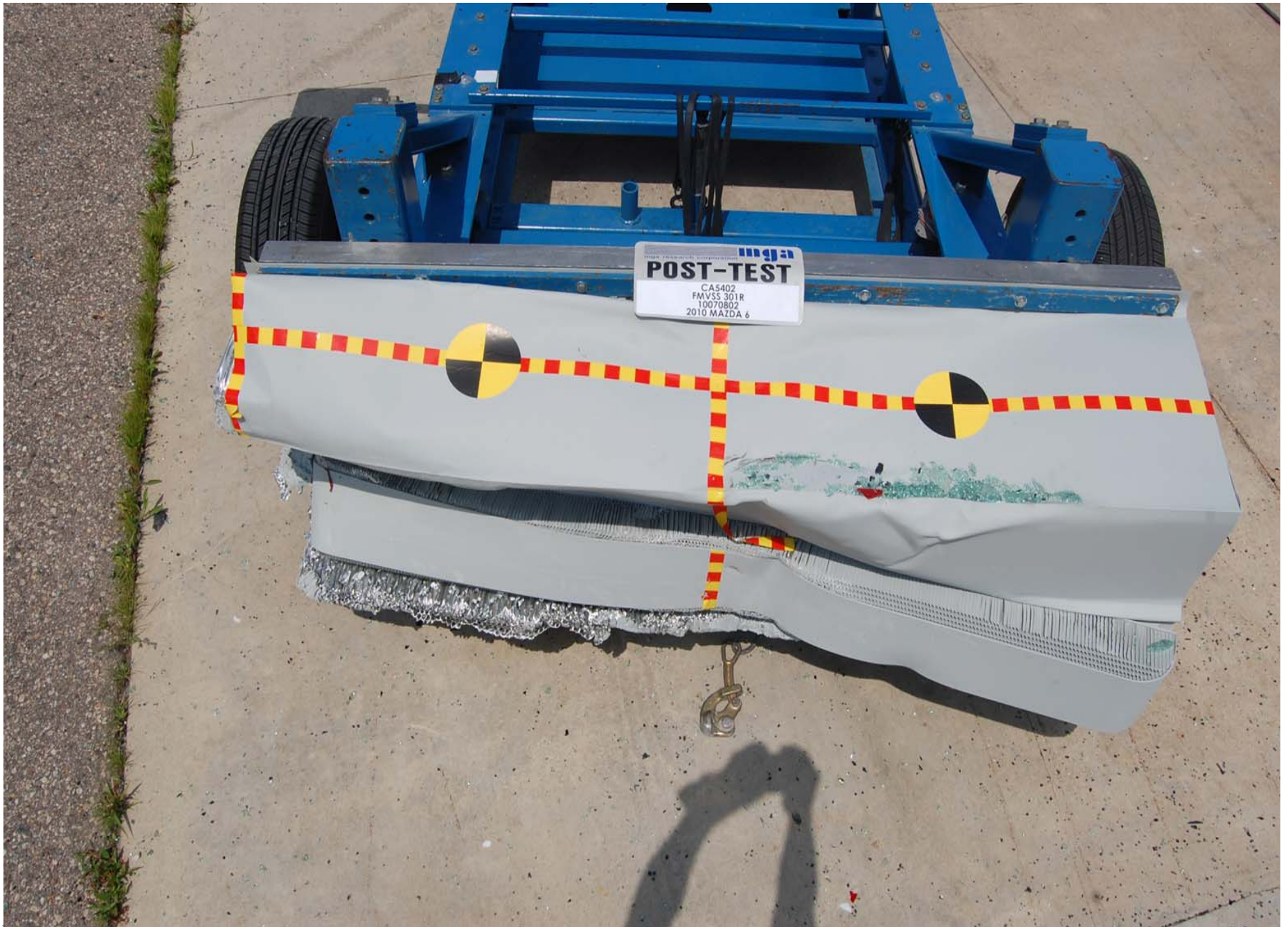
Post-Test Top View of MDB
