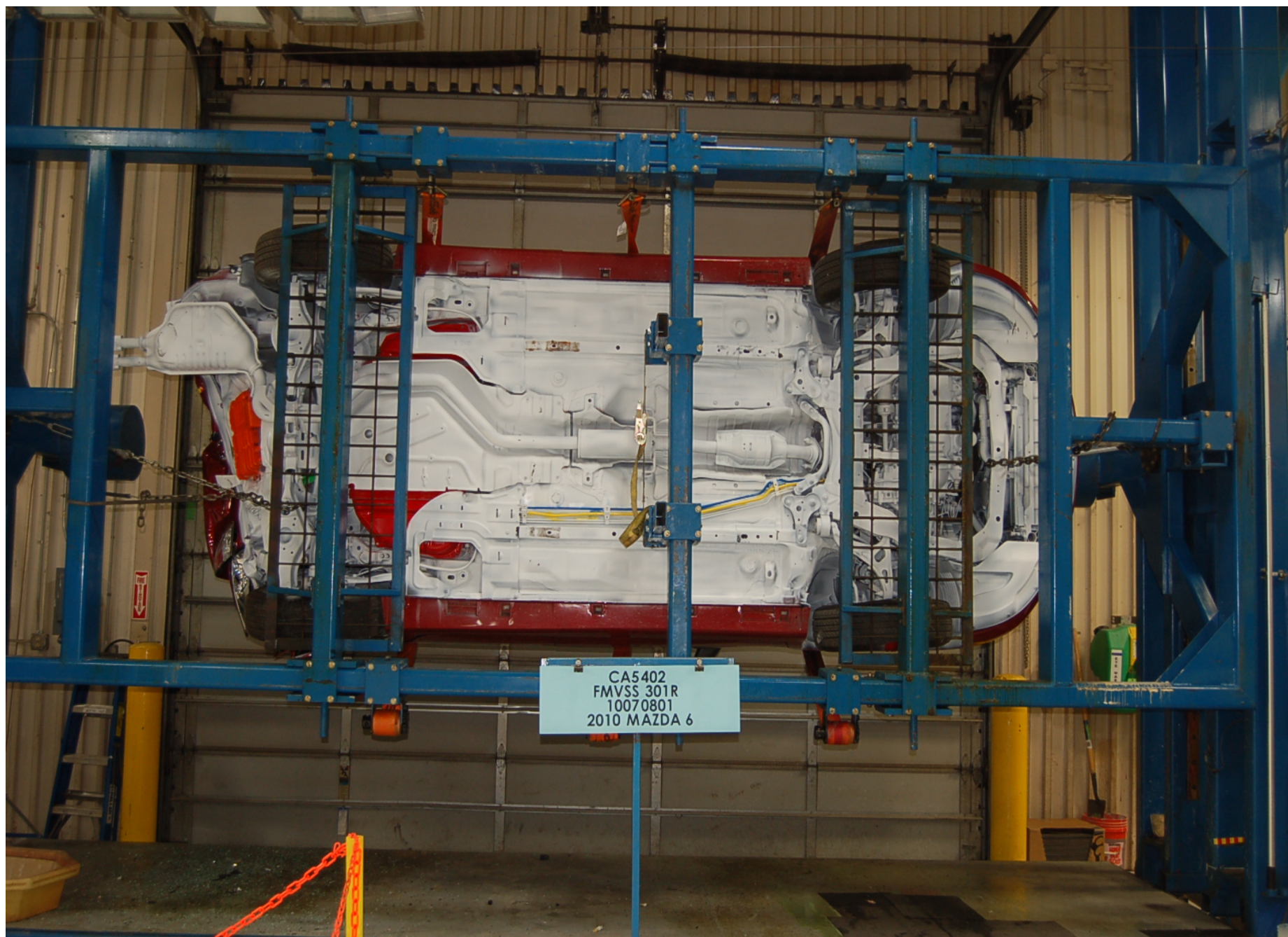
Static Rollover at 270 Degrees
