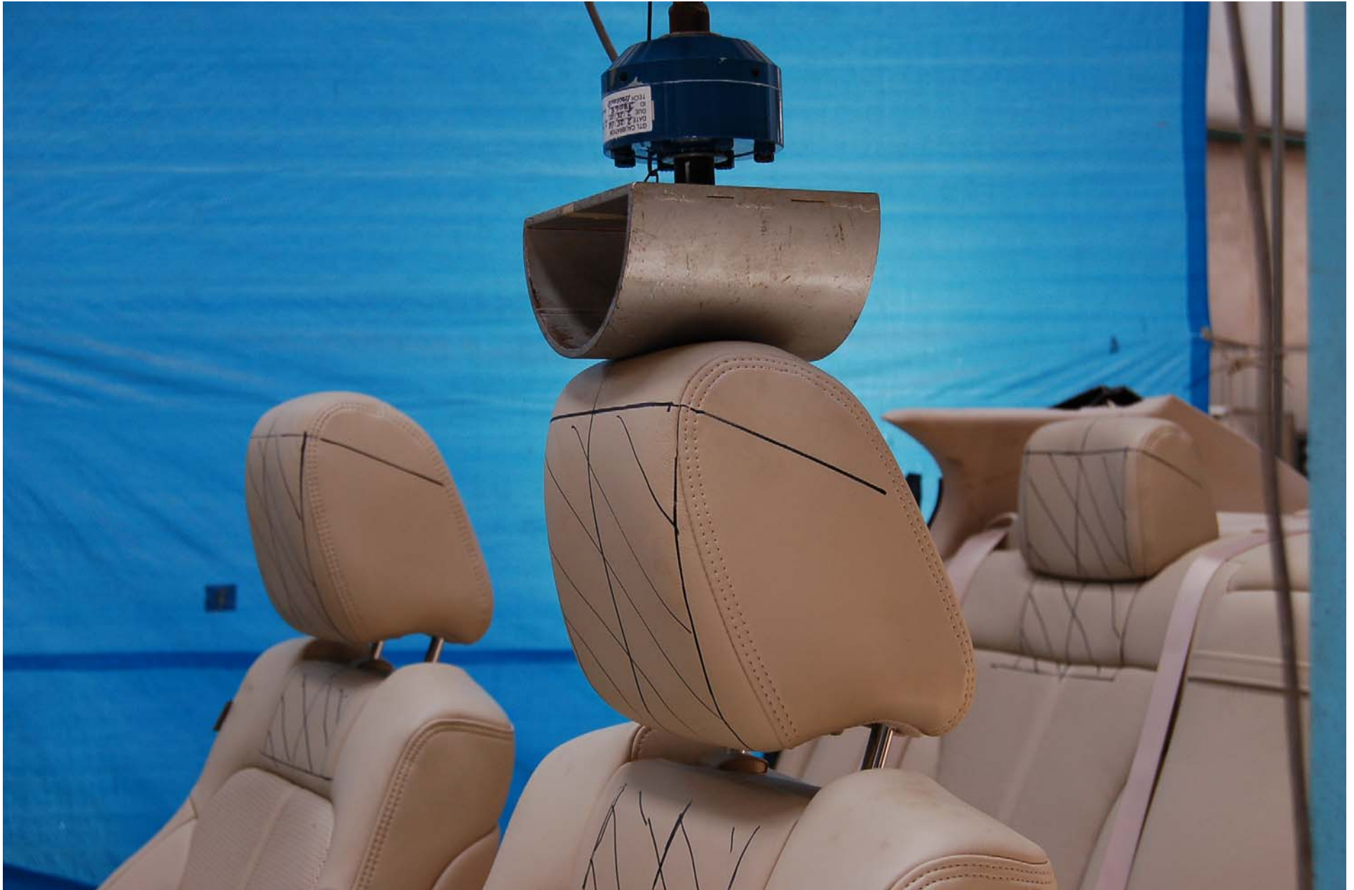
FIGURE 5.32 HEAD FORM AT 10% POST TEST LOAD
