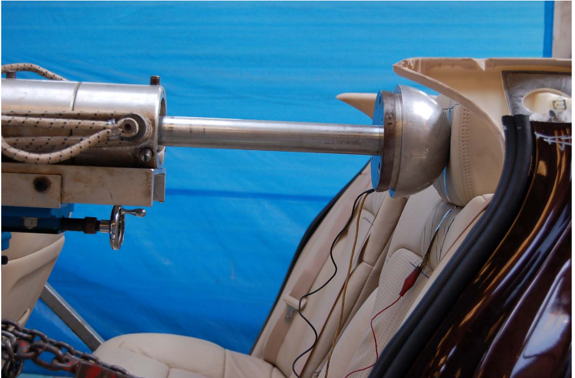
FIGURE 5.42 PRE-TEST SET-UP FOR ENERGY ABSORPTION TEST
