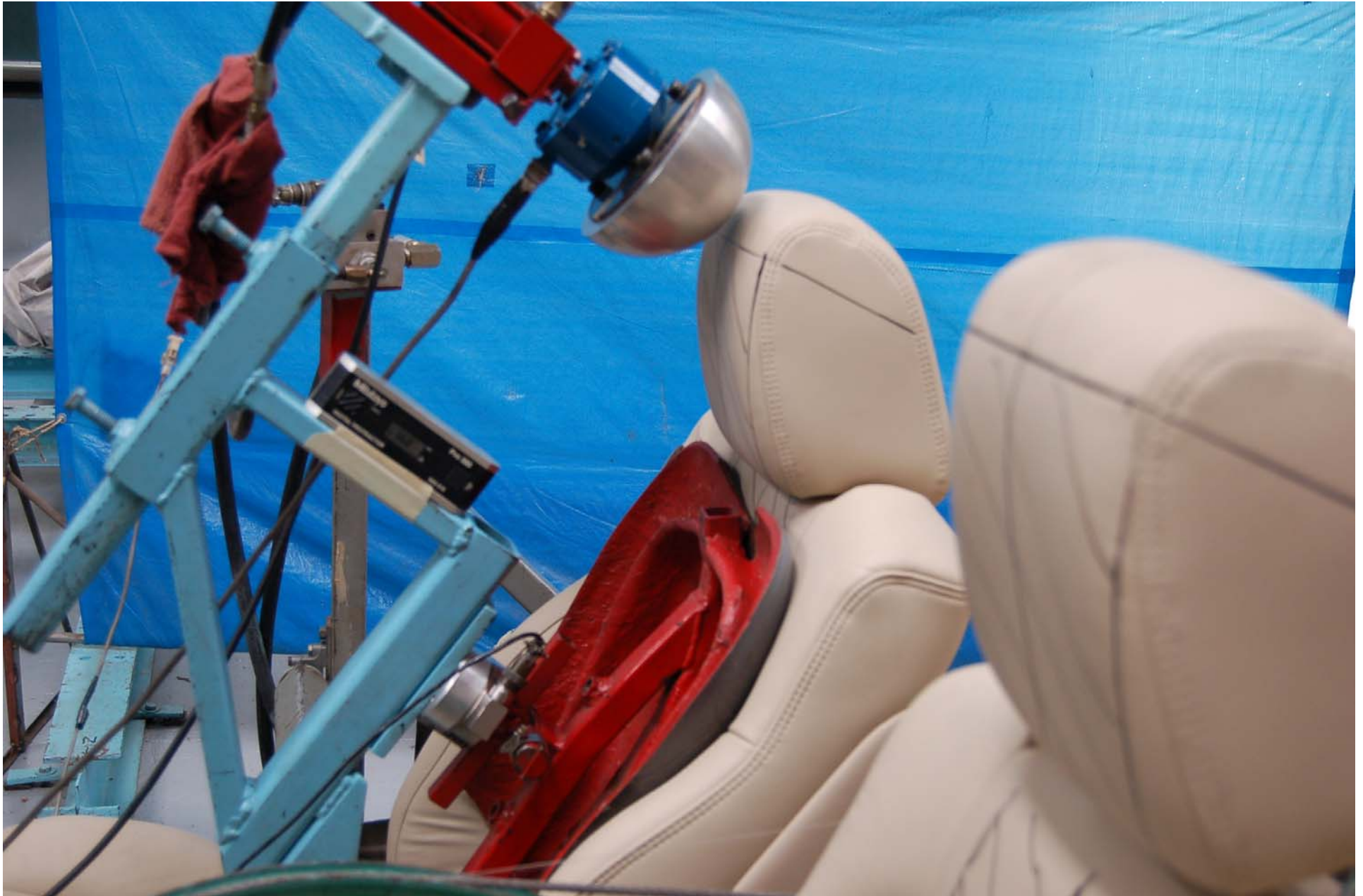
FIGURE 5.34 BACK PAN AT 373 Nm LOAD
