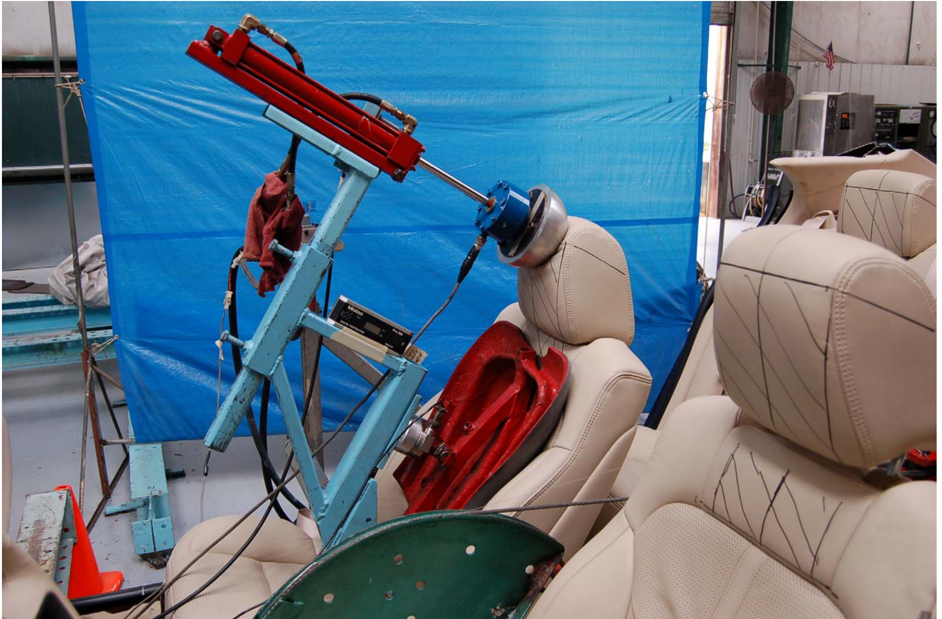
FIGURE 5.39 HEAD RESTRAINT WITH 895 N LOAD APPLIED
