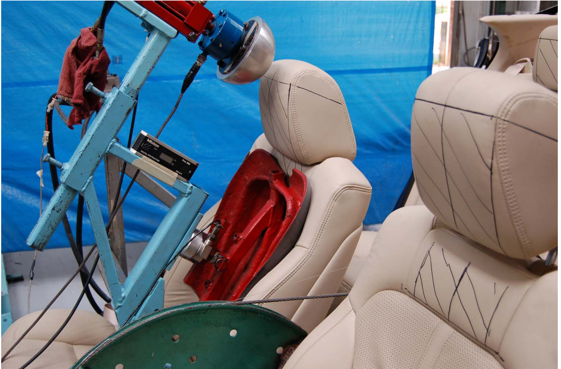
FIGURE 5.41 HEAD RESTRAINT POST TEST
