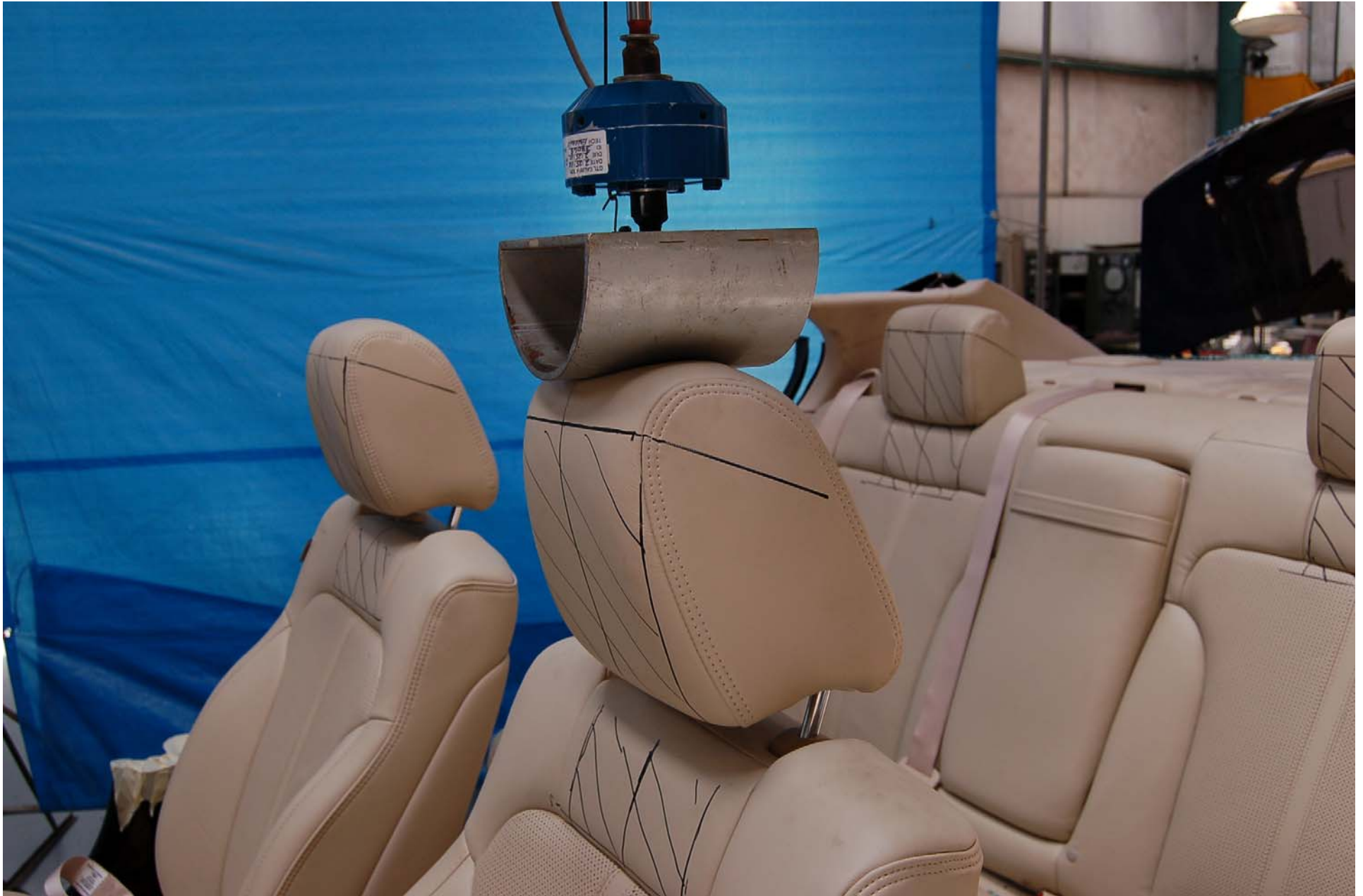
FIGURE 5.30 HEAD FORM CONTACT AT FULL LOAD
