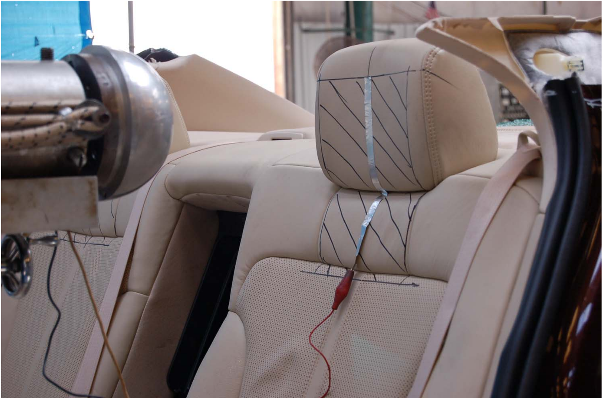
FIGURE 5.43 PRE-TEST HEAD RESTRAINT FOR ENERGY ABSORPTION
