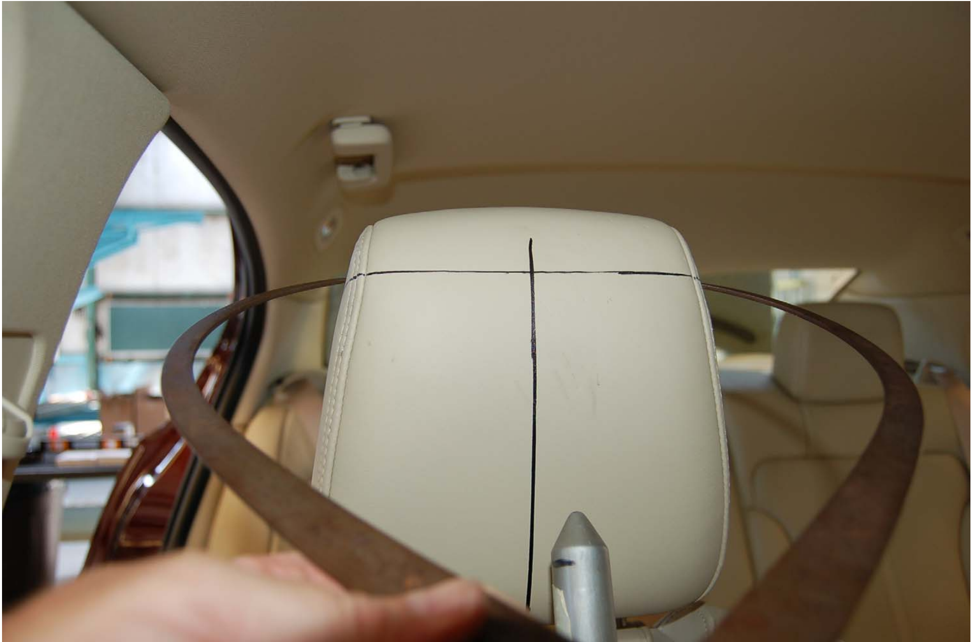
FIGURE 5.13 WIDTH MEASUREMENT OF FRONT HEAD RESTRAINT
