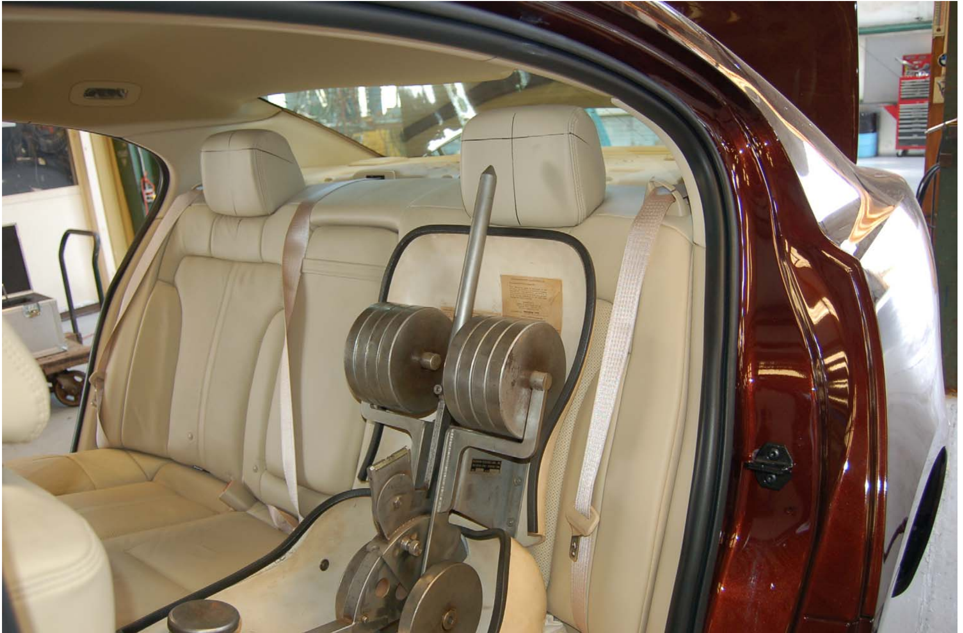
FIGURE 5.24 SAE J826 MANIKIN IN REAR DRIVER SEAT
