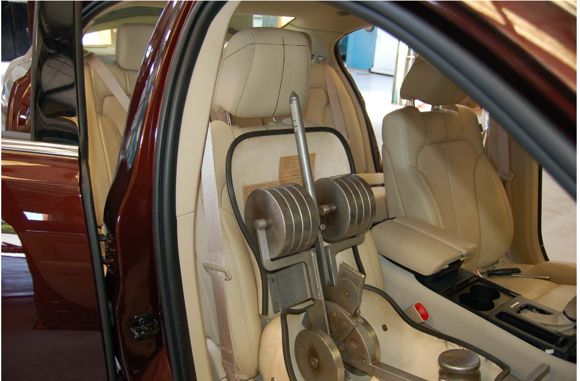
FIGURE 5.18 SAE J826 MANIKIN IN FRONT PASSENGER SEAT
