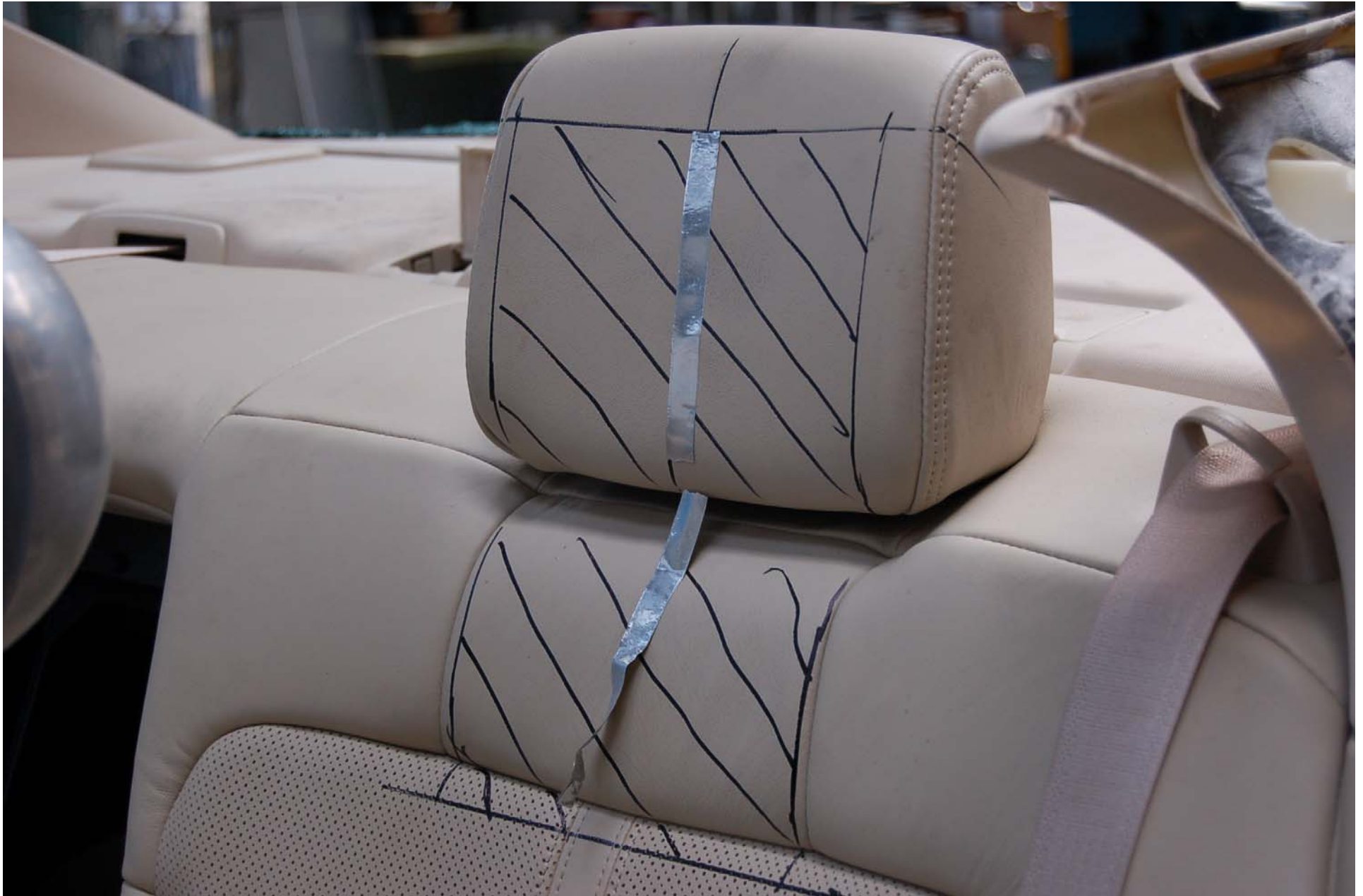
FIGURE 5.44 POST TEST HEAD RESTRAINT FOR ENERGY ABSORPTION
