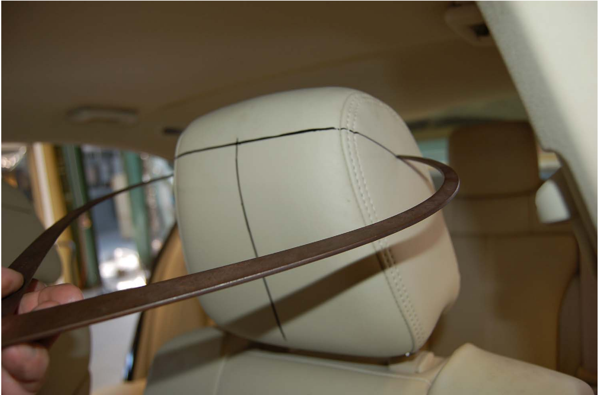
FIGURE 5.14 WIDTH MEASUREMENT OF DRIVER HEAD RESTRAINT
