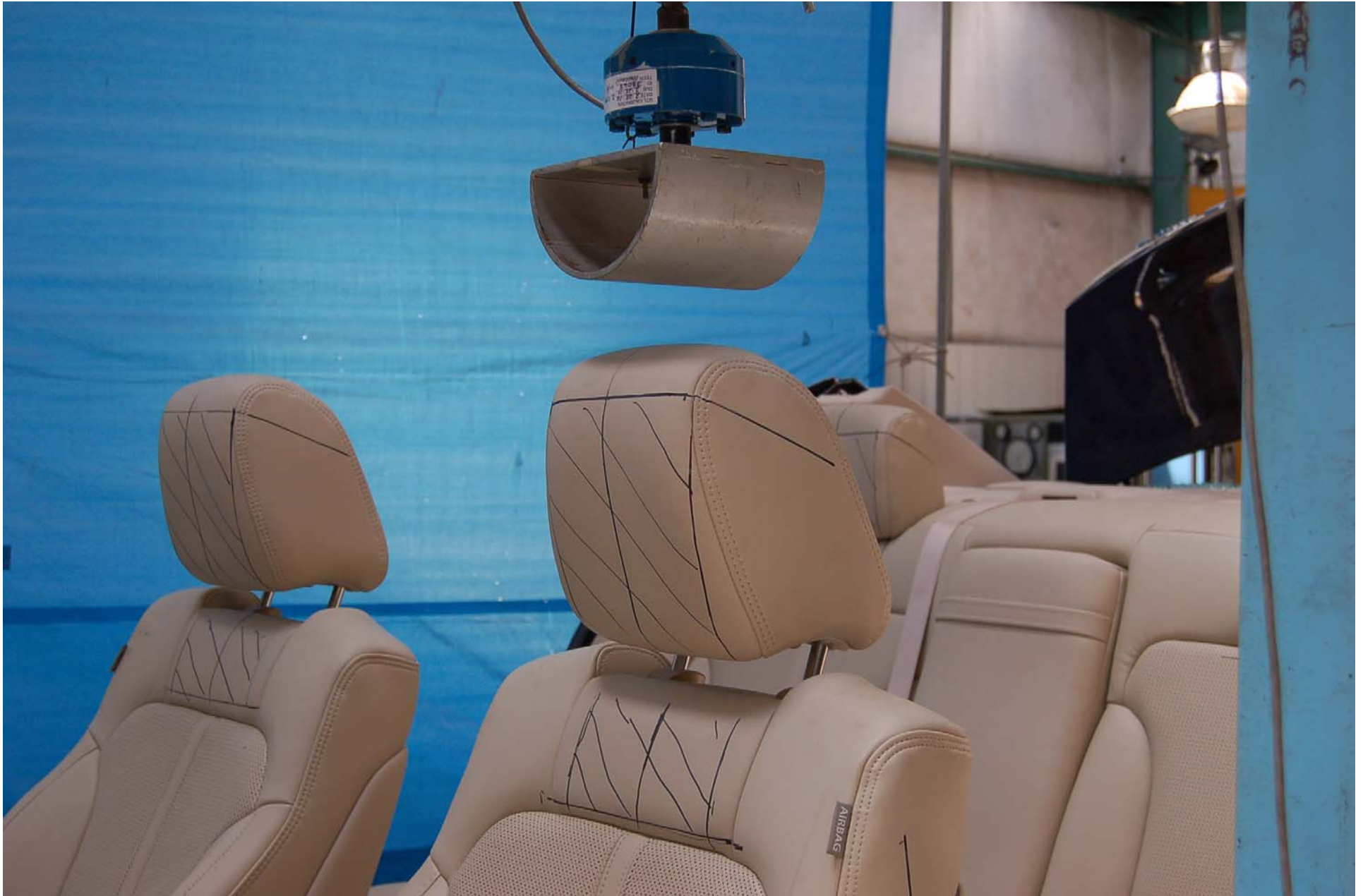
FIGURE 5.27 PRE-TEST SET-UP FOR HEIGHT RETENTION
