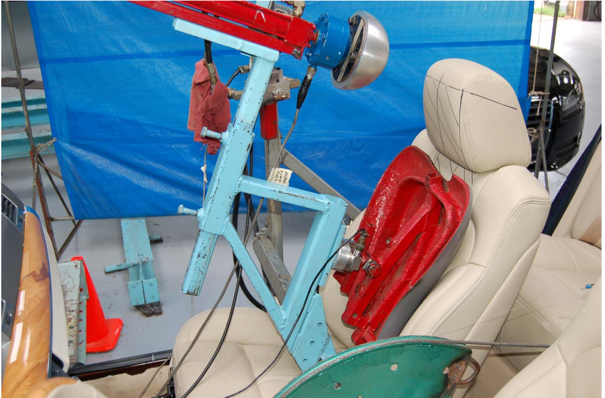
FIGURE 5.33 PRE-TEST SET-UP FOR BACKSET RETENTION
