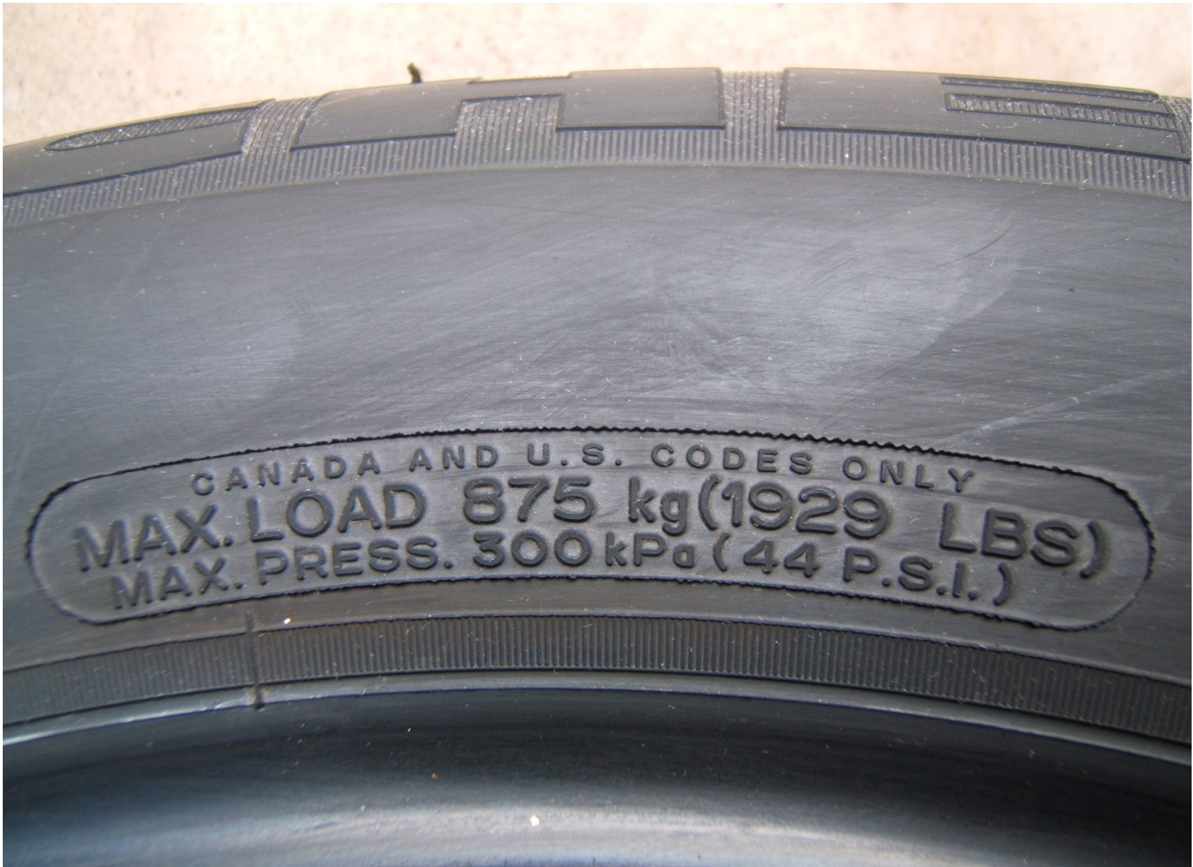
FIGURE 5.8 TIRE SHOWING MAX LOAD RATING AND MAX INFLATION PRESSURE
