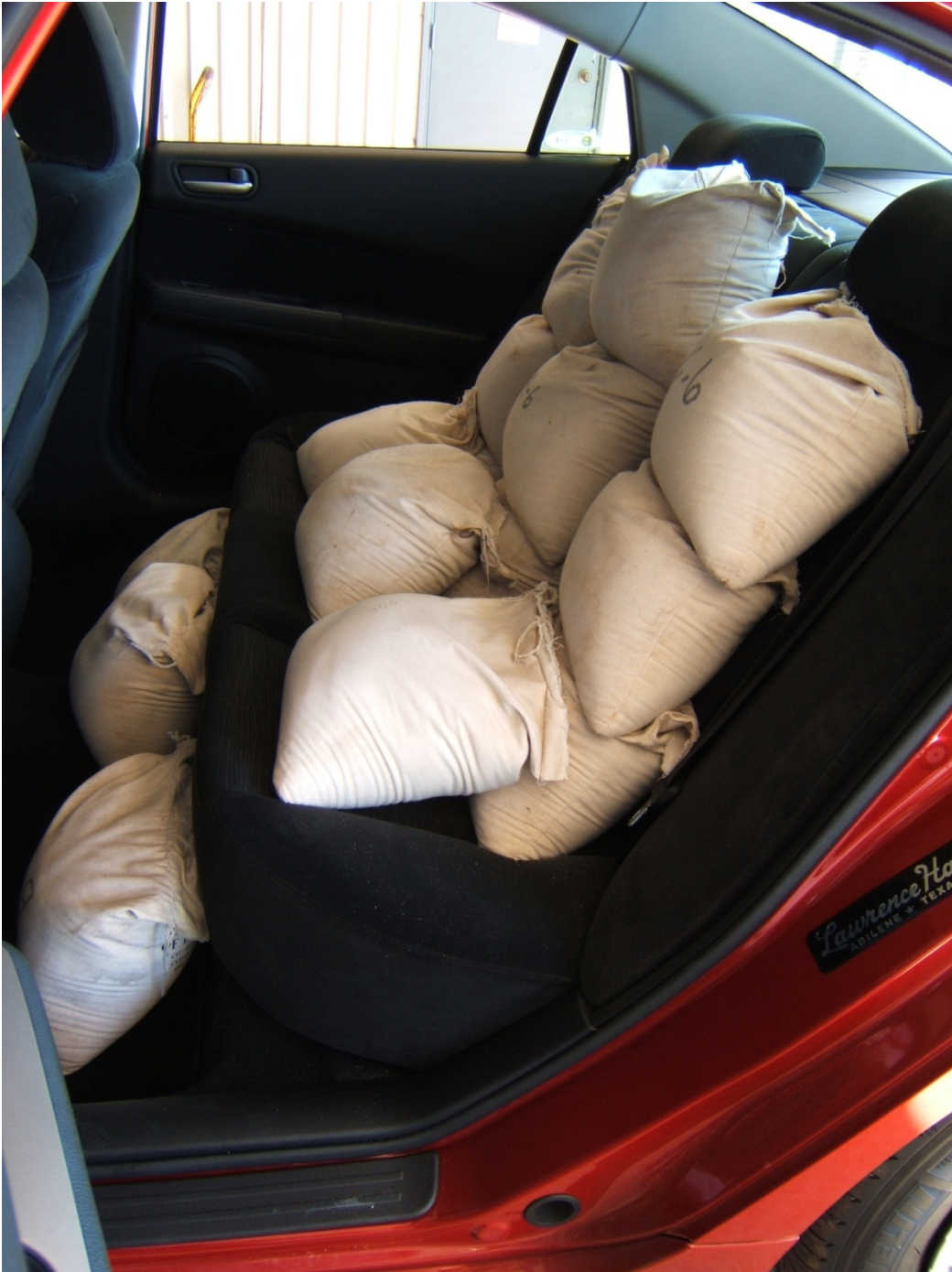
FIGURE 5.13 VEHICLE REAR SEAT BALLASTED FOR FULL AND MAXIMUM LOADS
