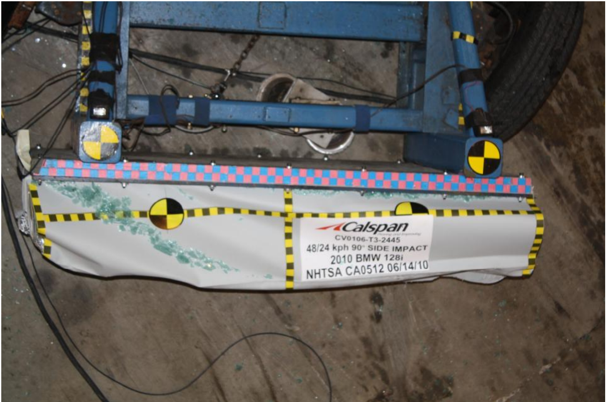
Figure A-14 Post-Test Top View of MDB Impactor Face
