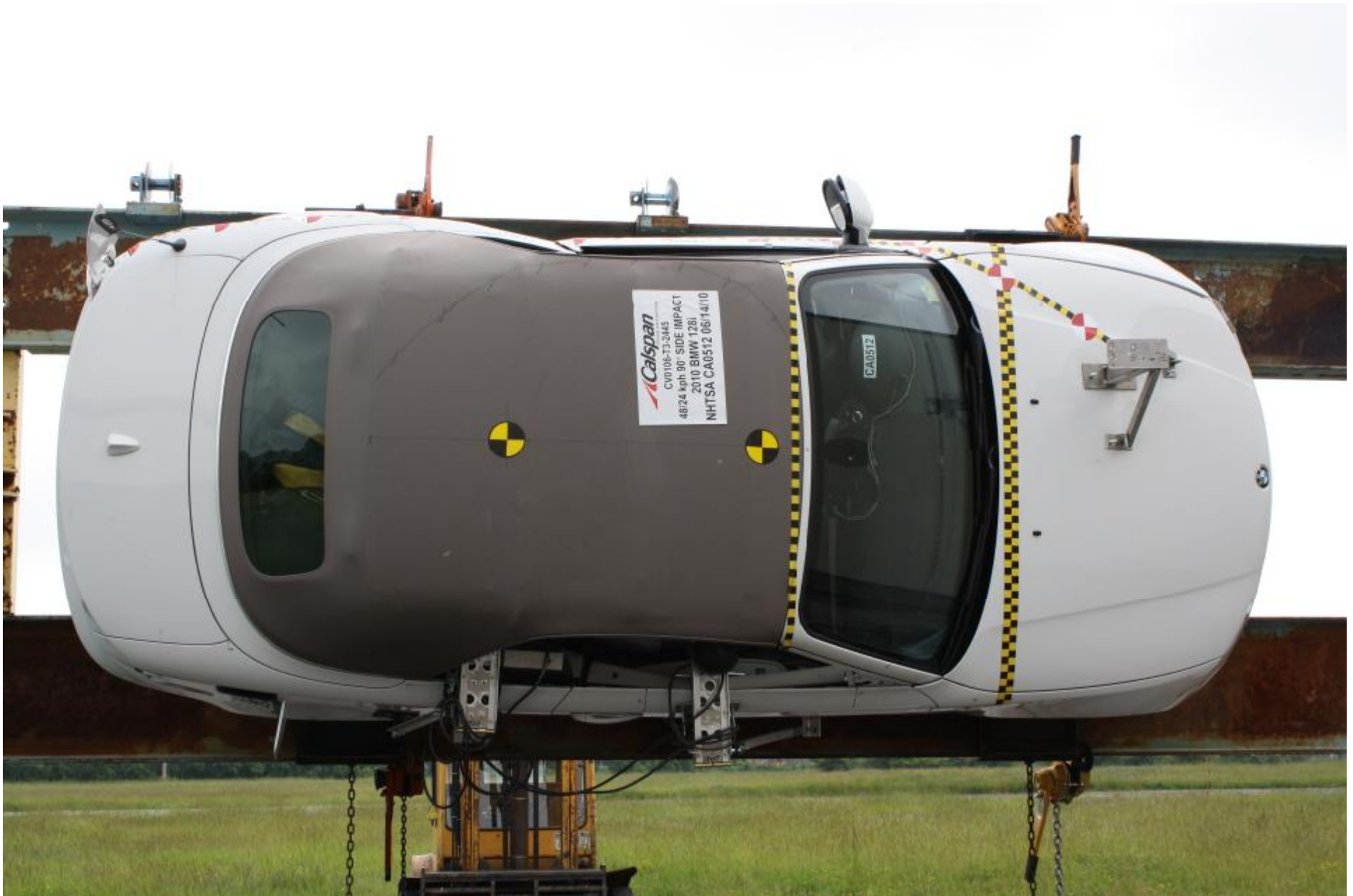
Figure A-28 Rollover 90 Degrees
