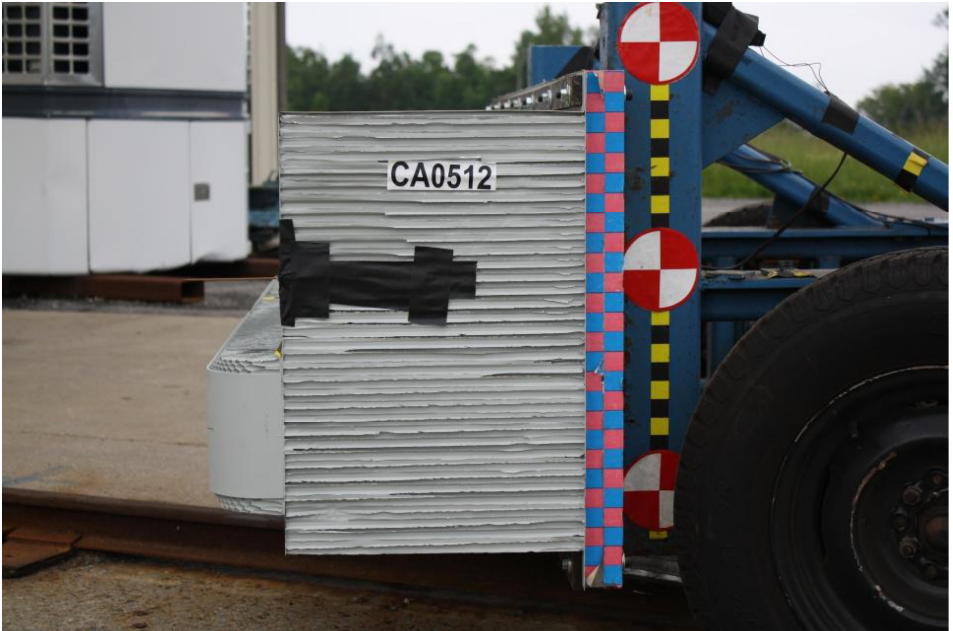
Figure A-9 Pre-Test Left Side View of MDB Impactor Face
