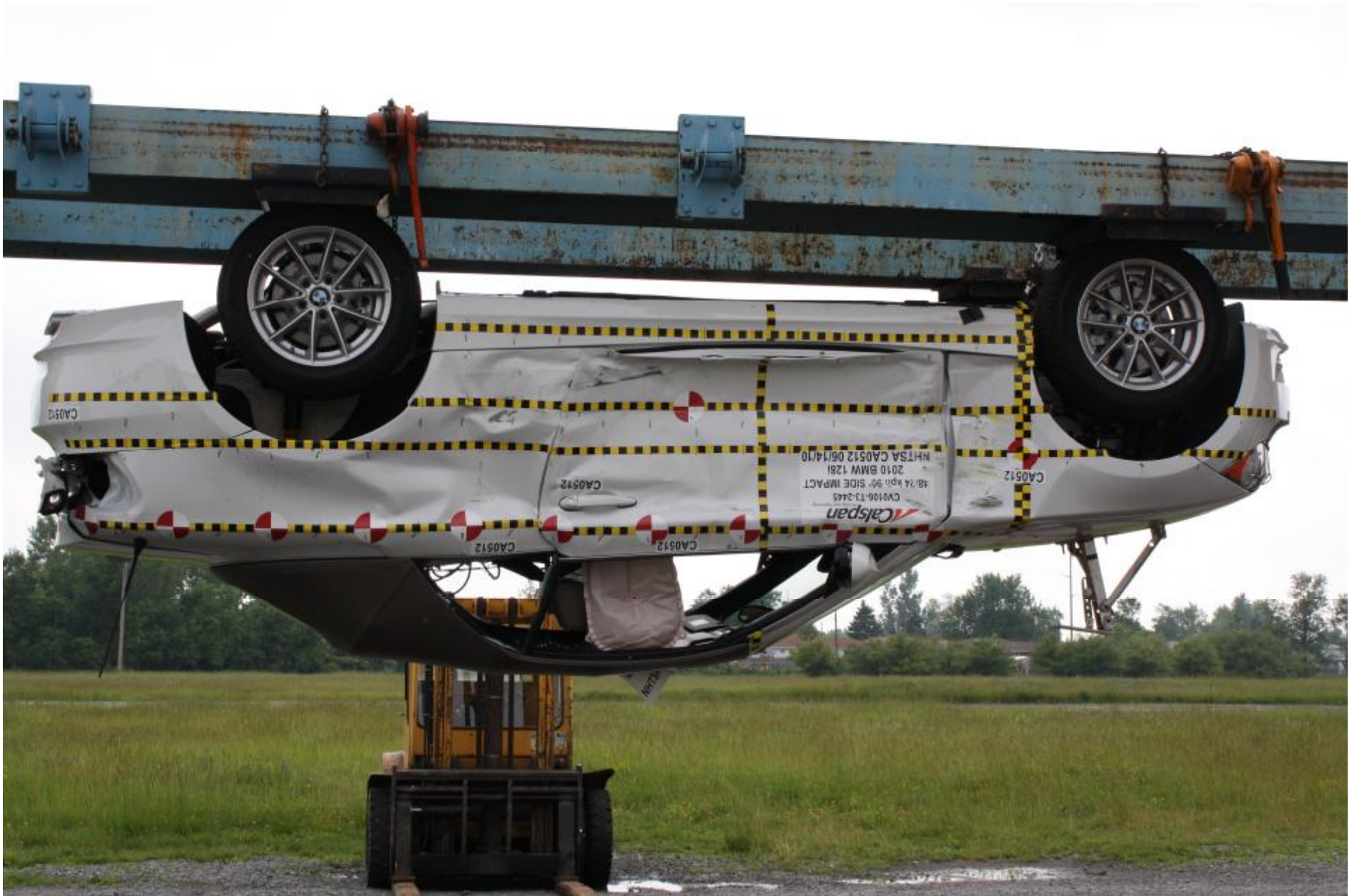
Figure A-29 Rollover 180 Degrees
