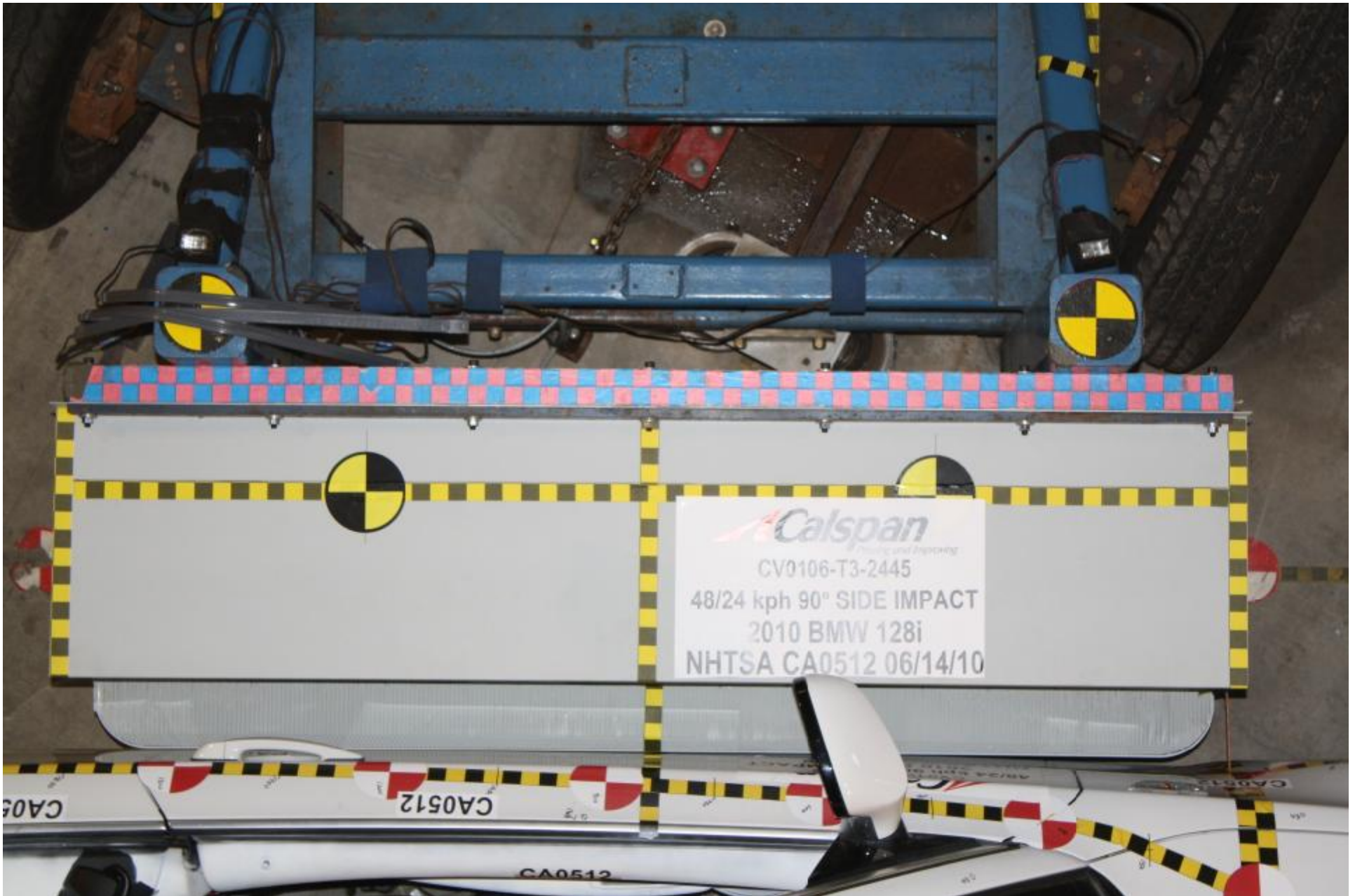
Figure A-13 Pre-Test Top View of MDB Impactor Face
