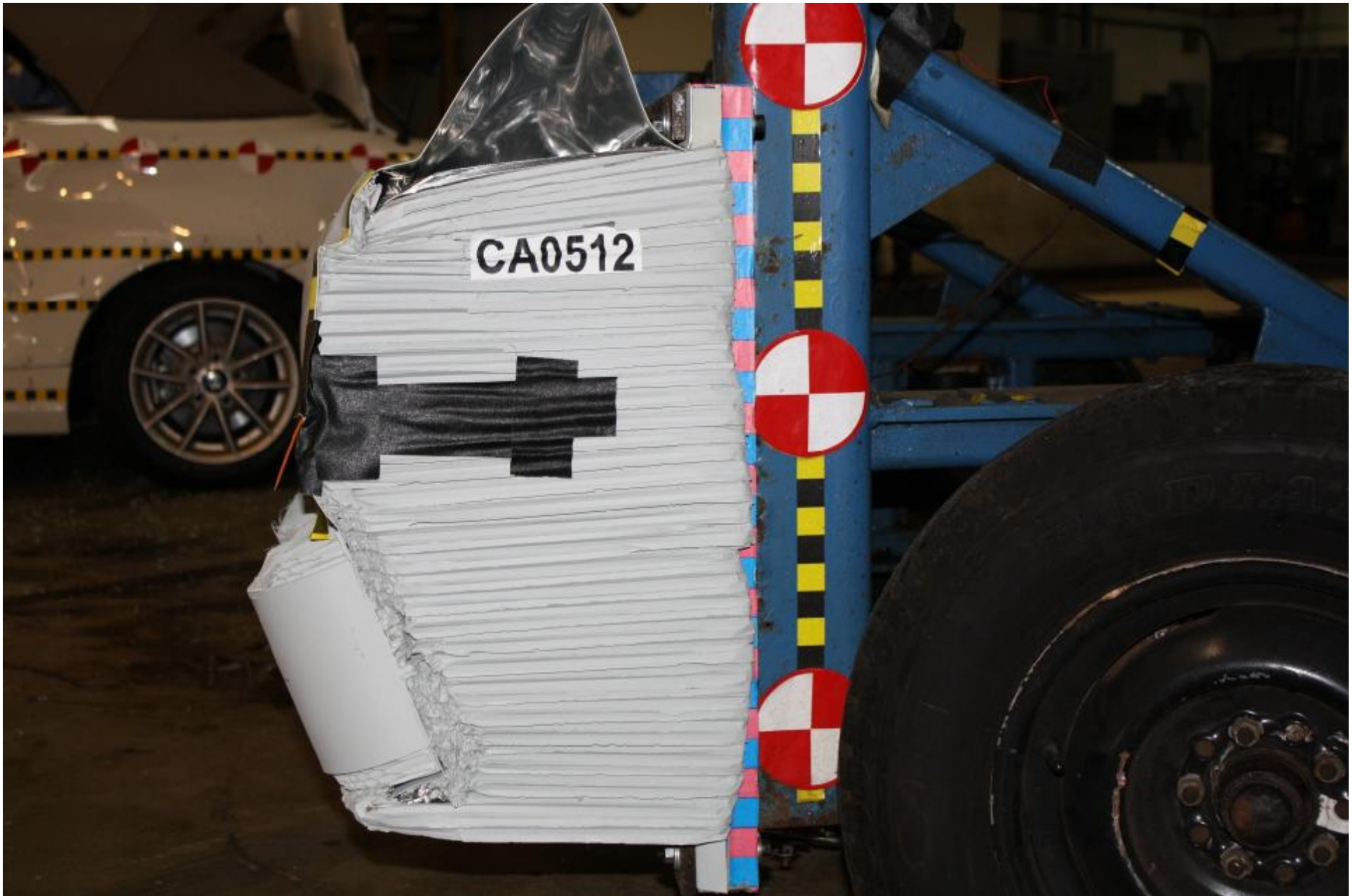
Figure A-10 Post-Test Left Side View of MDB Impactor Face
