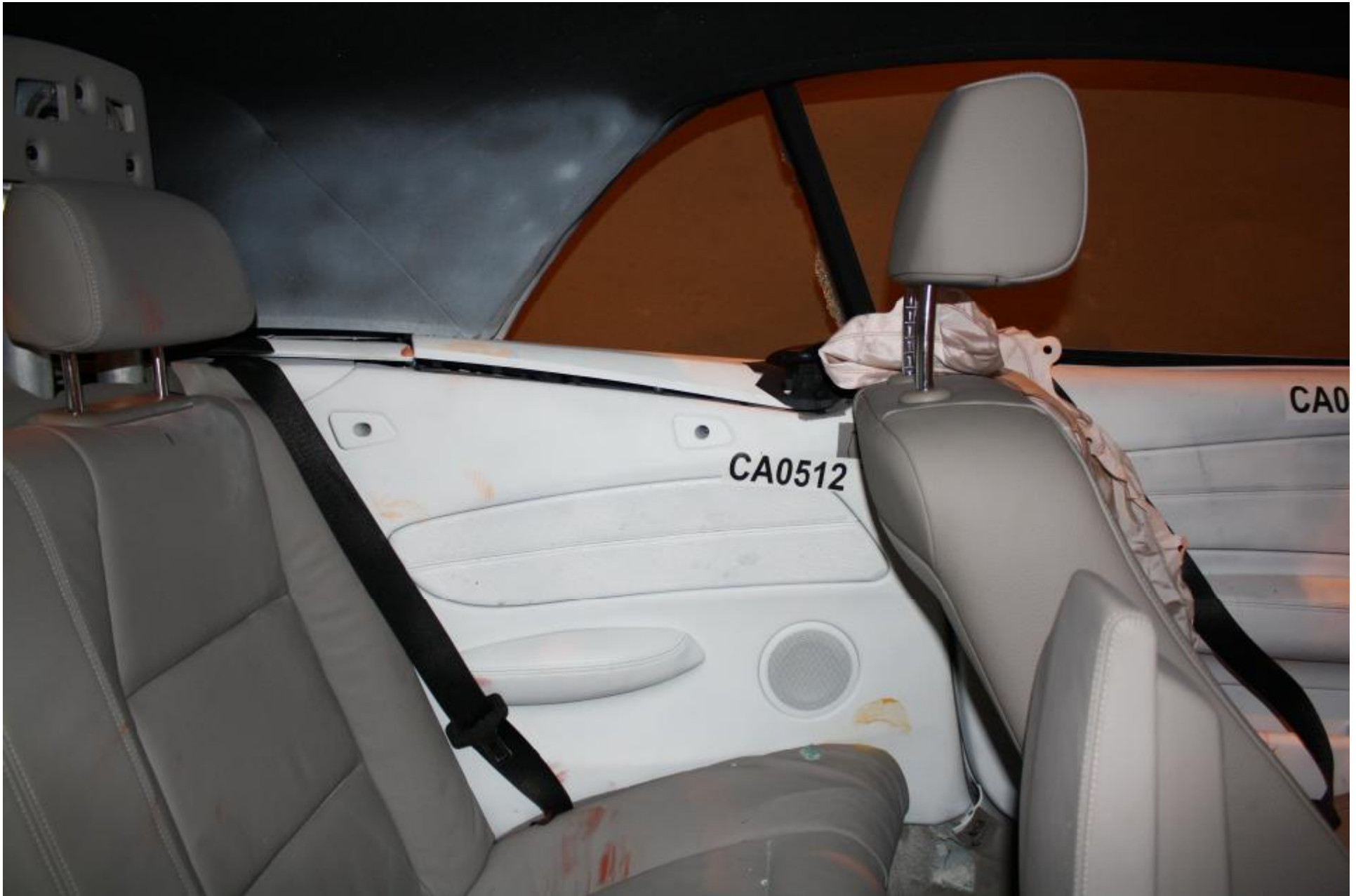
Figure A-21 Post-Test Left Rear Door Interior Trim Showing SID Impact Locations
