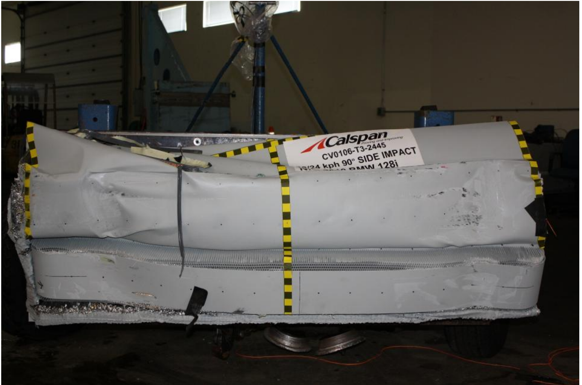
Figure A-8 Post-Test Frontal View of MDB Impactor Face
