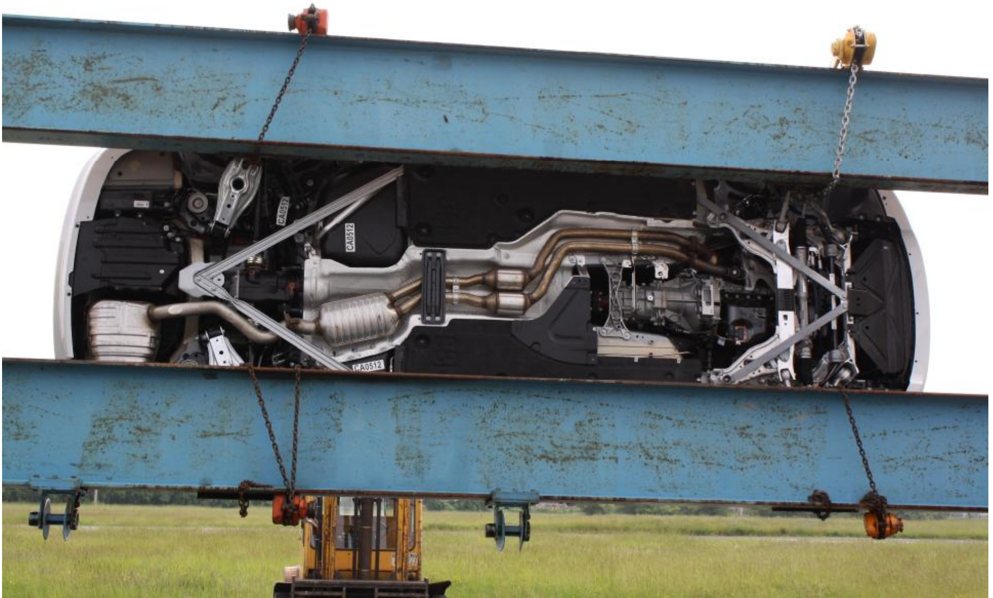
Figure A-30 Rollover 270 Degrees
