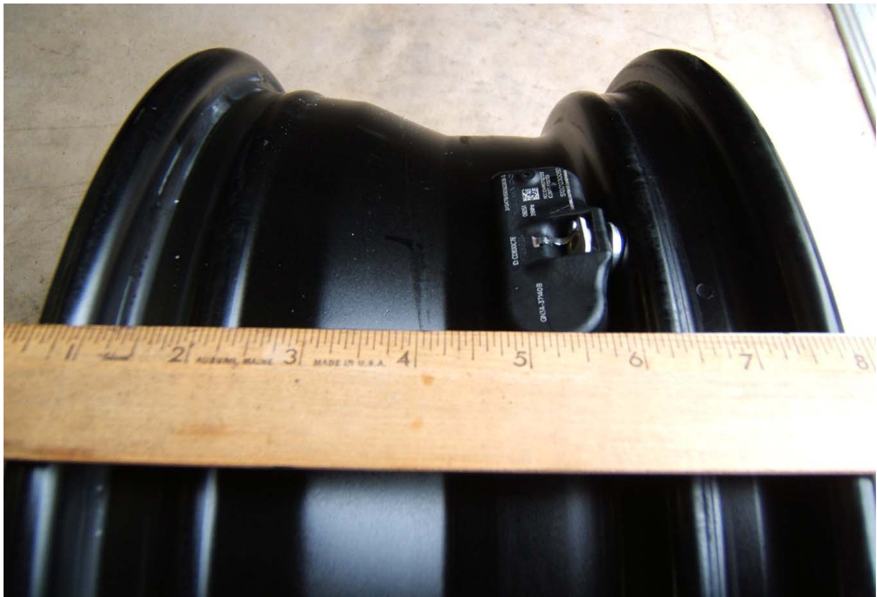
FIGURE 5.9 RIM SHOWING TPMS SENSOR AND RIM CONTOUR FOR FULL WIDTH OF CROSS SECTION
