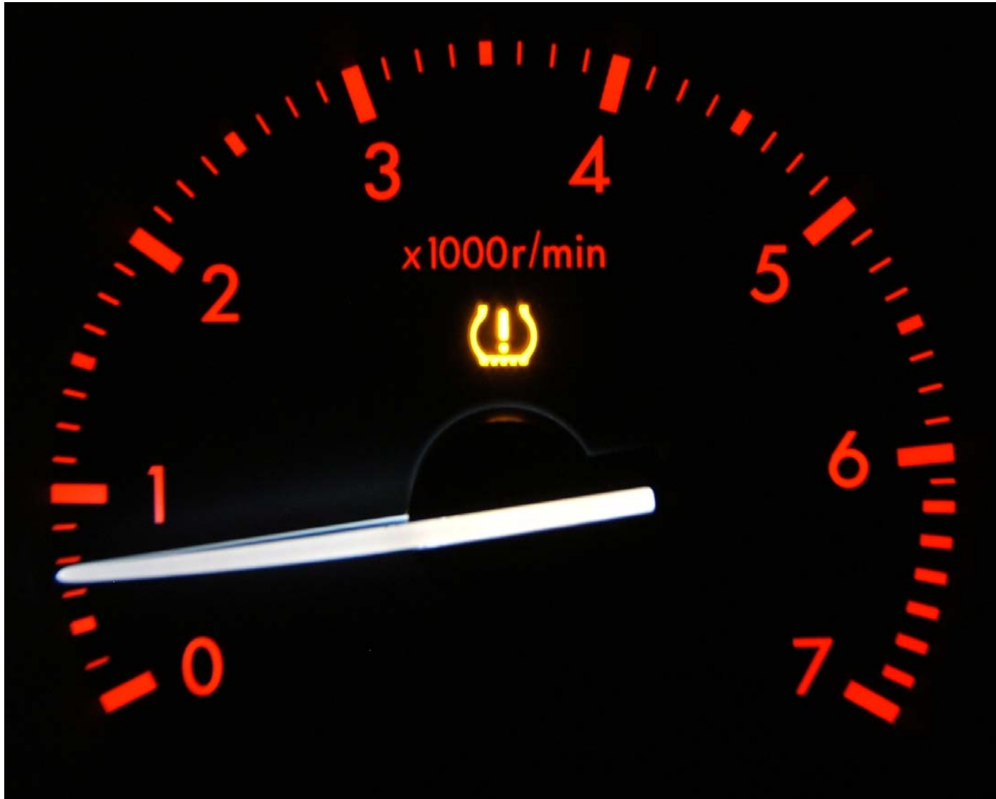
FIGURE 5.10 DISPLAY SHOWING COMBINATION LOW TIRE PRESSURE WARNING/TPMS MALFUNCTION WARNING TELLTALE
