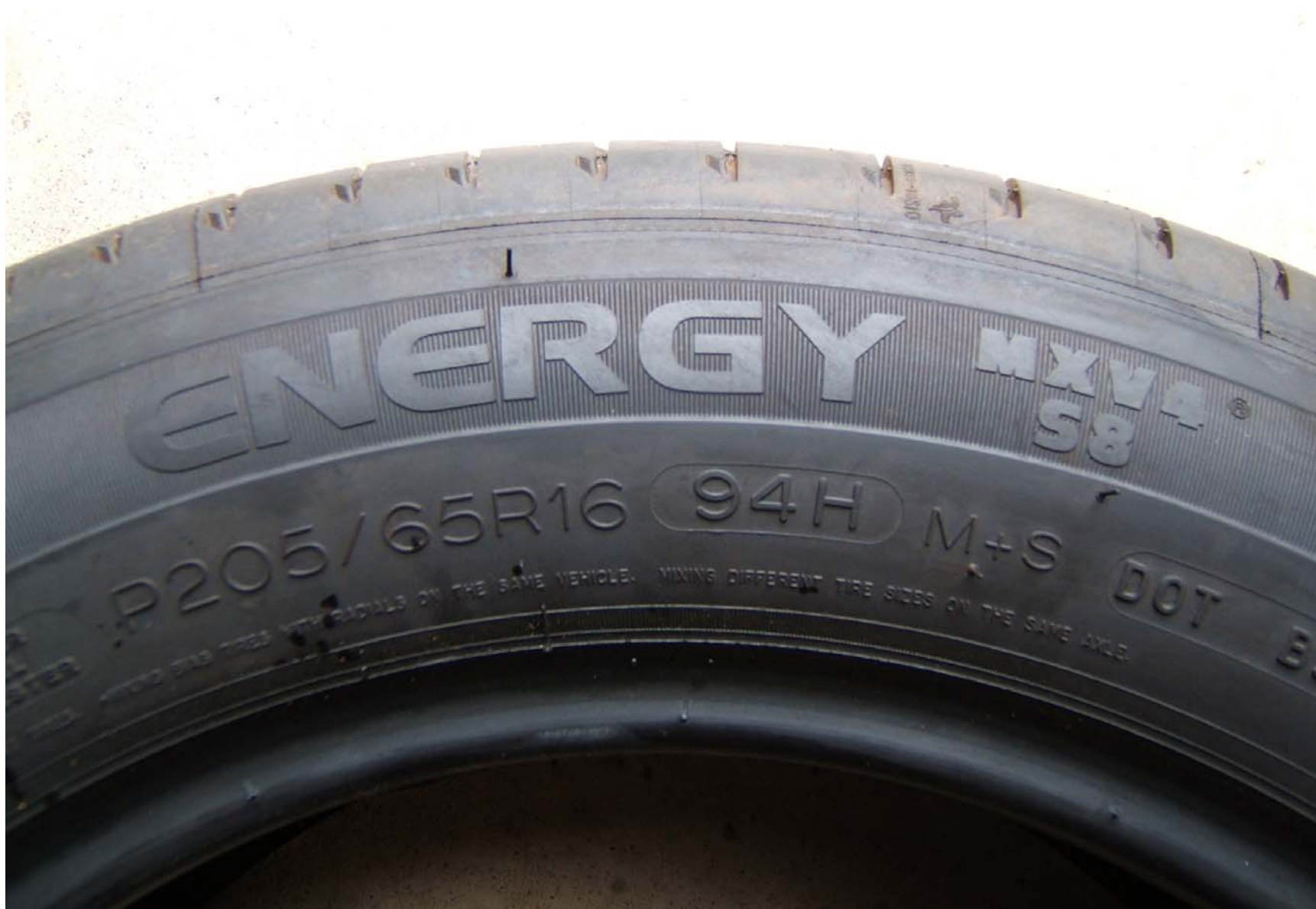
FIGURE 5.5 TIRE SHOWING MODEL, SIZE, AND LOAD INDEX / SPEED RATING
