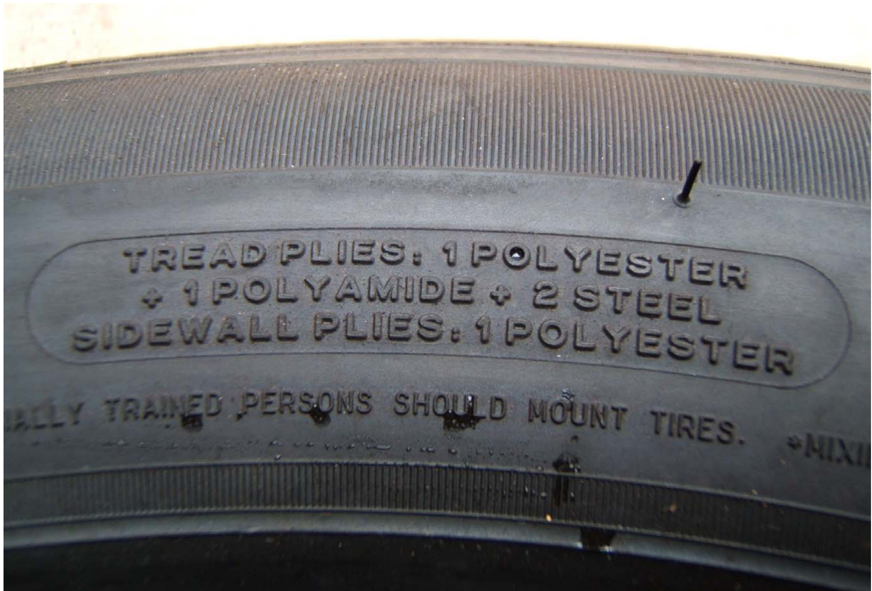
FIGURE 5.8 TIRE SHOWING SIDEWALL / TREAD CONSTRUCTION
