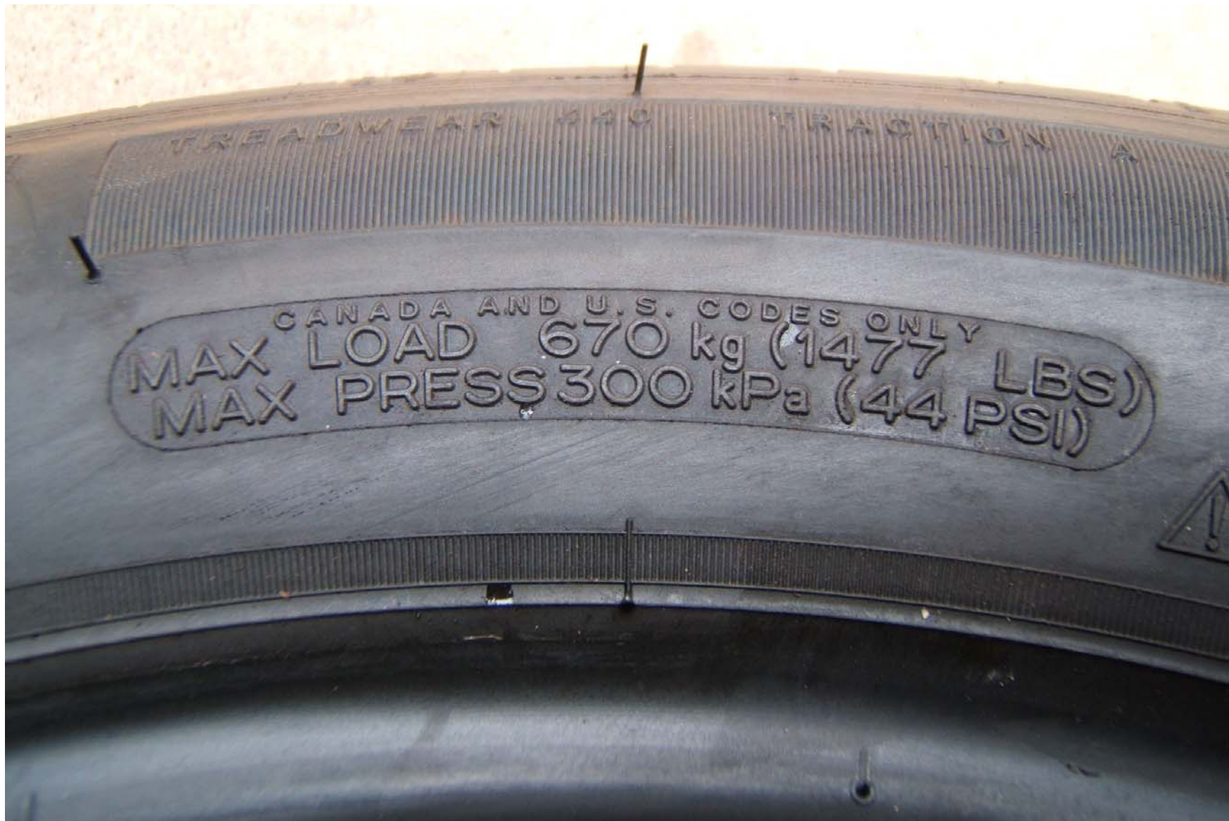
FIGURE 5.7 TIRE SHOWING MAX LOAD RATING AND MAX COLD INFLATION PRESSURE
