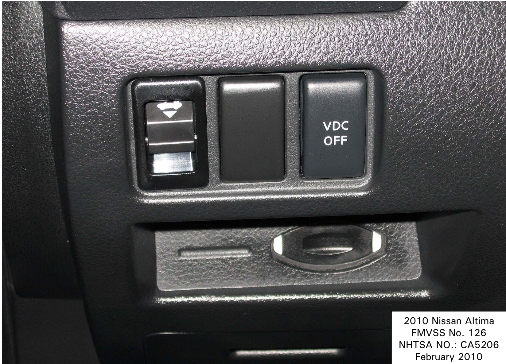
Figure 5.7. ESC Off Control Switch
