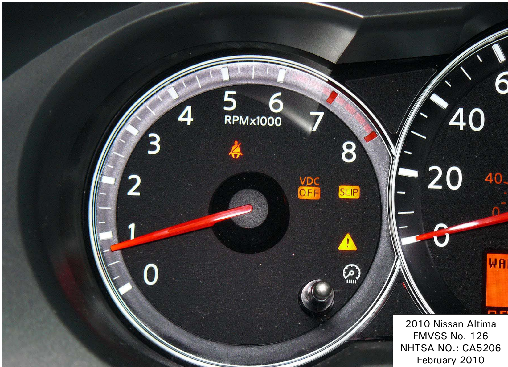
Figure 5.6. Telltale for ESC Malfunction and ESC Off
