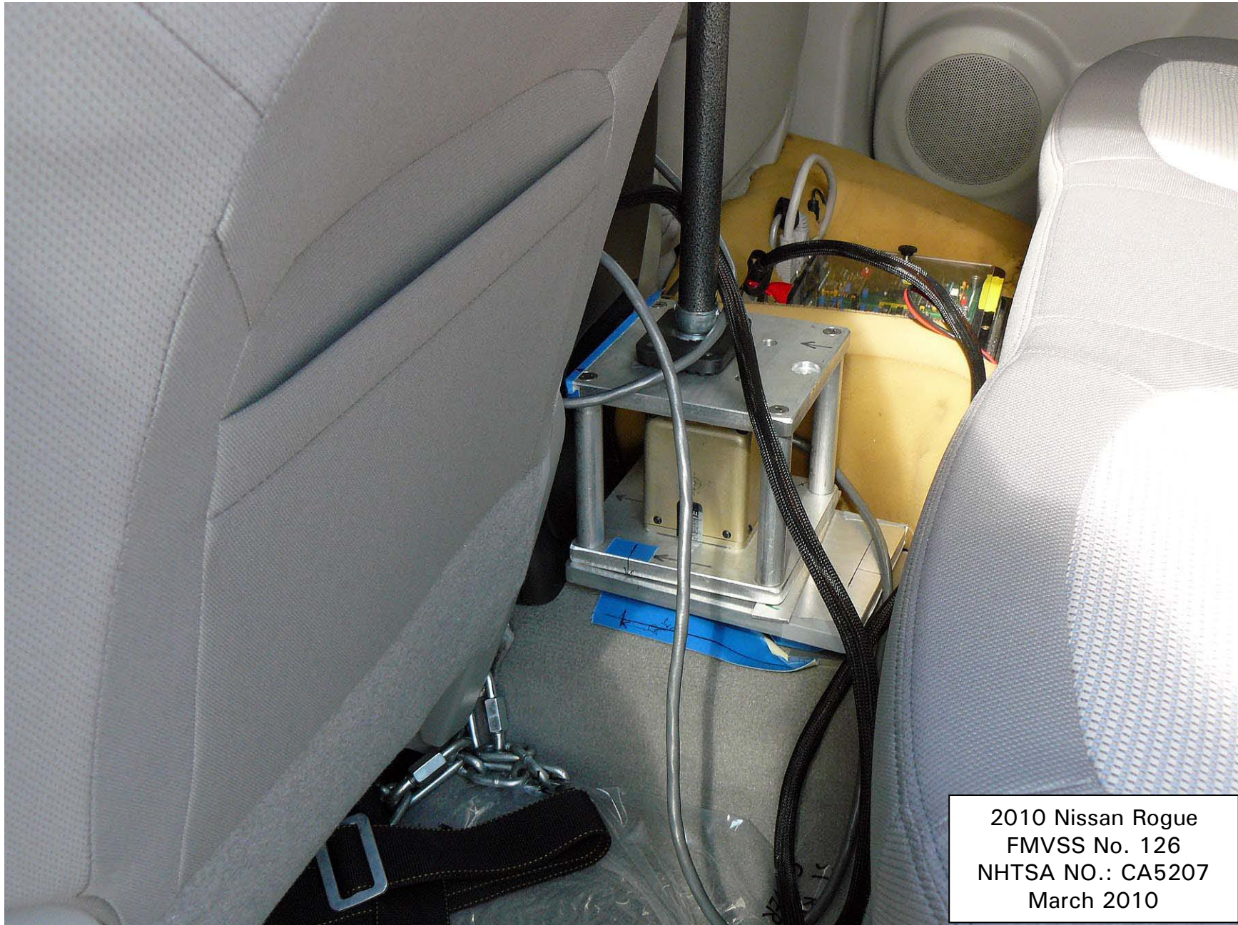
Figure 5.13. Inertial Measurement Unit Mounted in Vehicle
