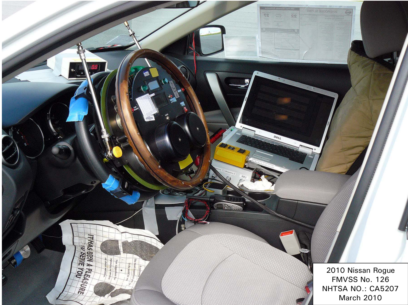
Figure 5.12. Steering Controller and Data Acquisition Computer
