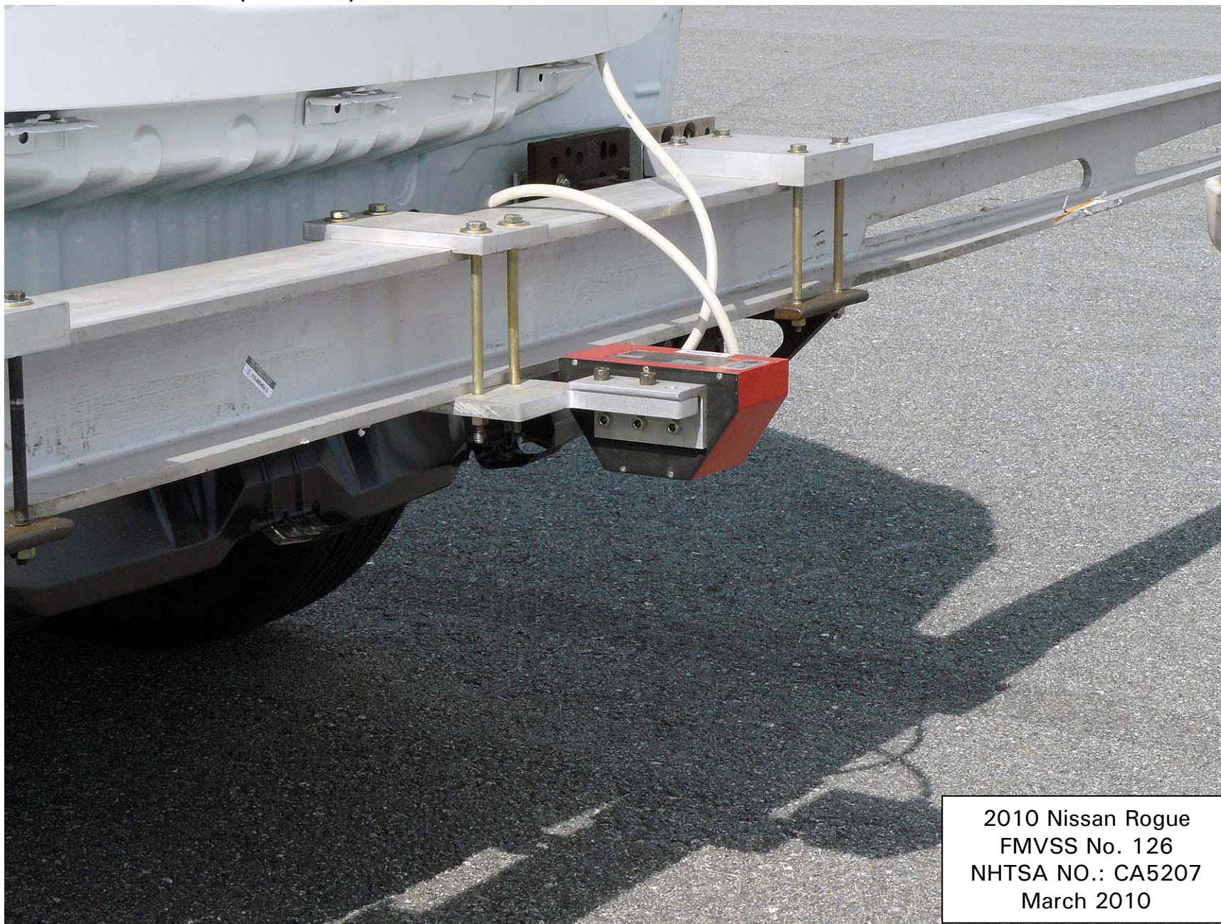
Figure 5.11. Rear Outrigger, Mount and Speed Sensor
