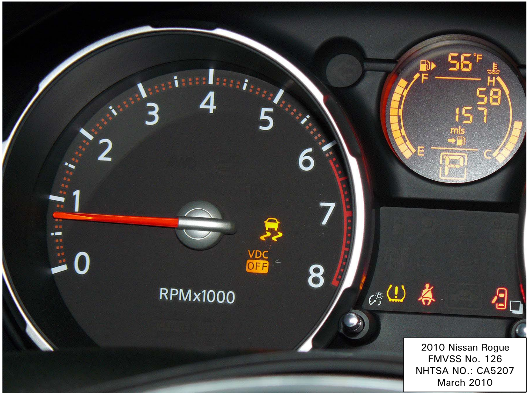
Figure 5.6. Telltale for ESC Malfunction and ESC Off
