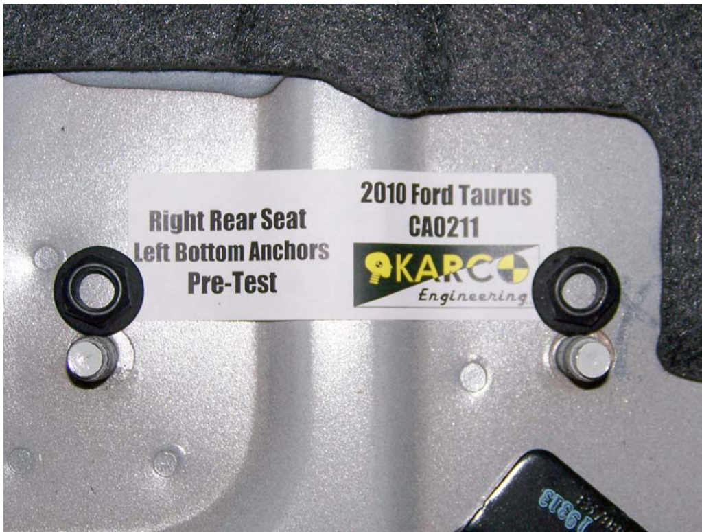
FIGURE 111. Floor Pan Anchor, P3, Pre-Test
