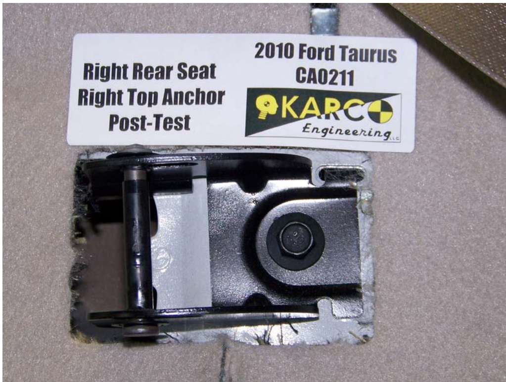
FIGURE 108. Floor Pan Anchor, P3, Post-Test
