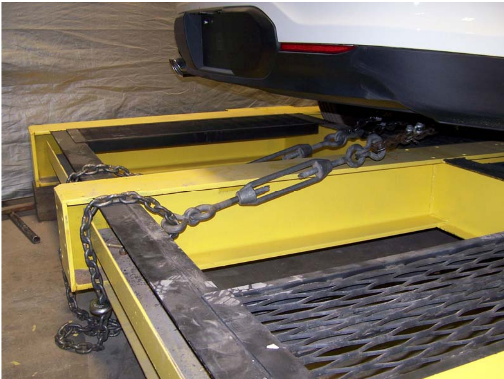
FIGURE 10. Vehicle Mounted in Test Fixture
