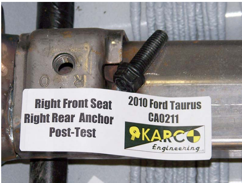
FIGURE 84. Floor Pan Anchor, P2, Post-Test
