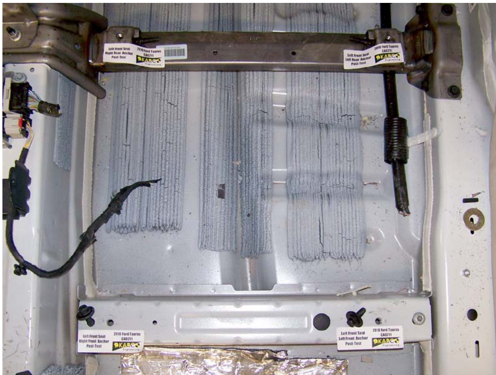
FIGURE 40. Floor Pan Anchors, P1 Overall, Post-Test
