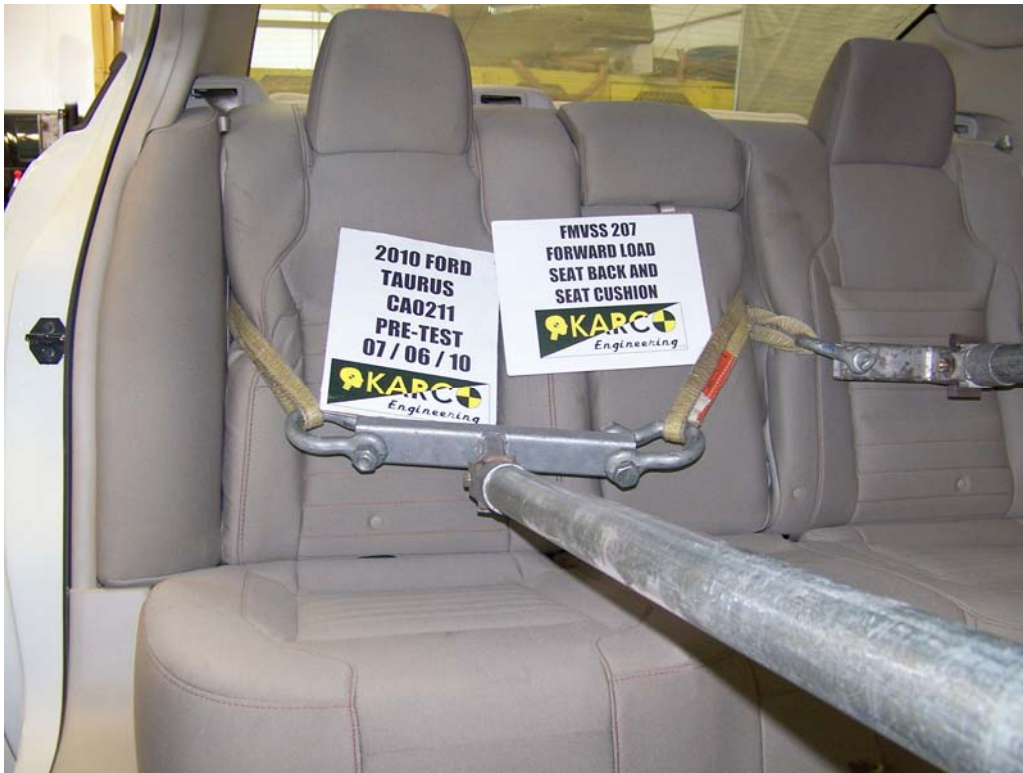
FIGURE 33. Forward Load on Seat Back and Seat Cushion, P3, Pre-Test
