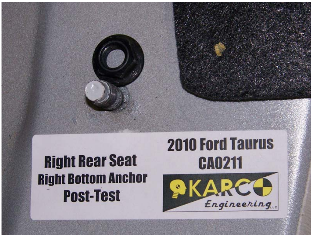
FIGURE 116. Floor Pan Anchor, P3, Post-Test
