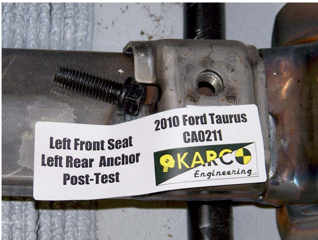
FIGURE 52. Floor Pan Anchor, P1, Post-Test
