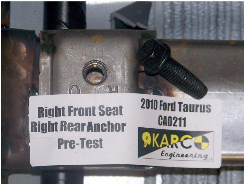
FIGURE 83. Floor Pan Anchor, P2, Pre-Test
