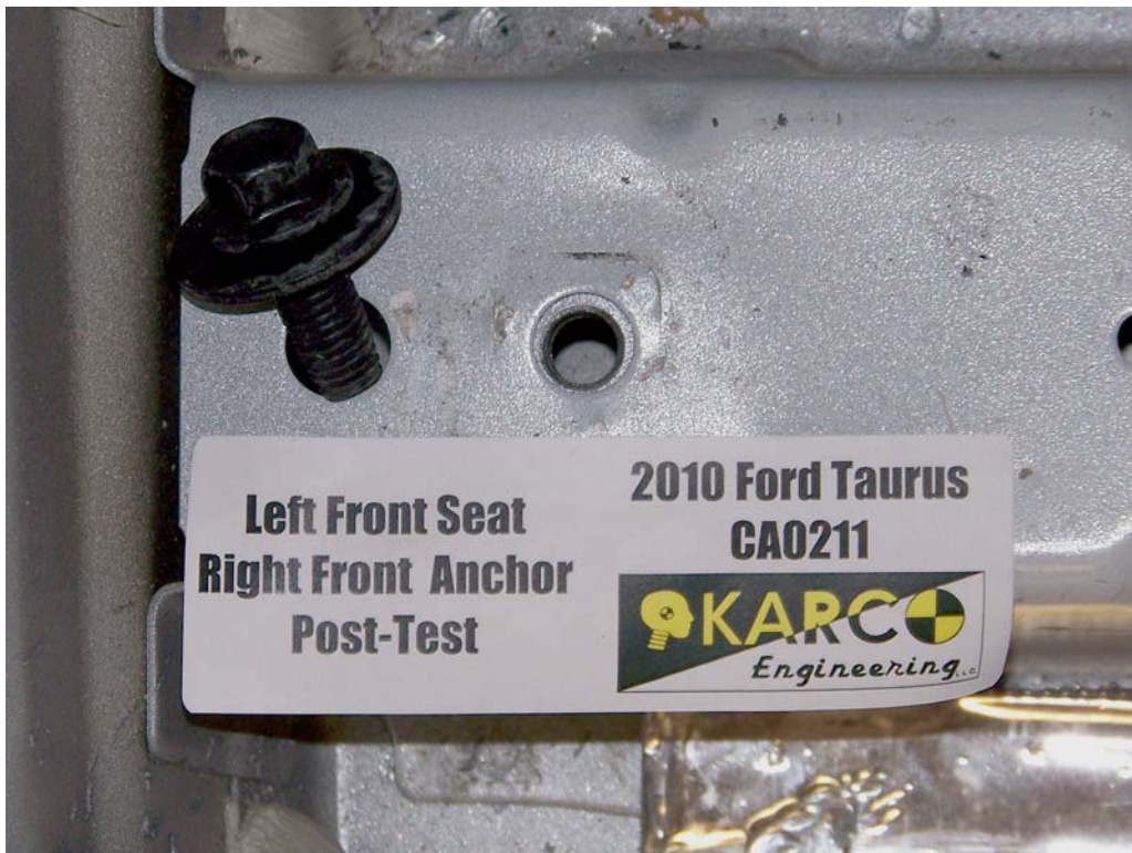
FIGURE 48. Floor Pan Anchor, P1, Post-Test
