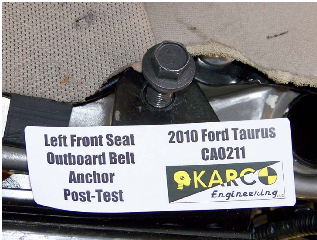
FIGURE 64. Belt Anchor, P1, Post-Test
