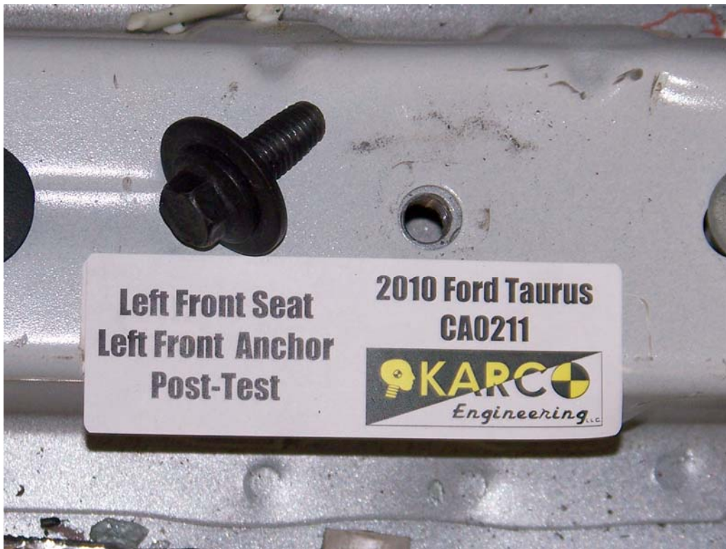
FIGURE 44. . Floor Pan Anchor, P1, Post-Test
