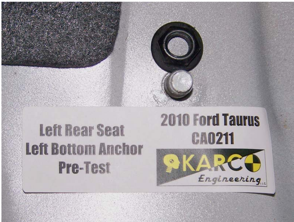
FIGURE 103. Floor Pan Anchor, P4, Pre-Test
