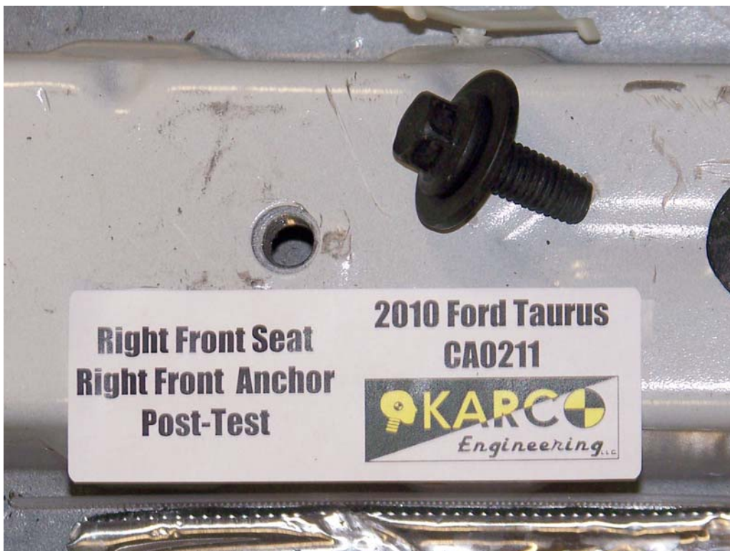
FIGURE 76. Floor Pan Anchor, P2, Post-Test
