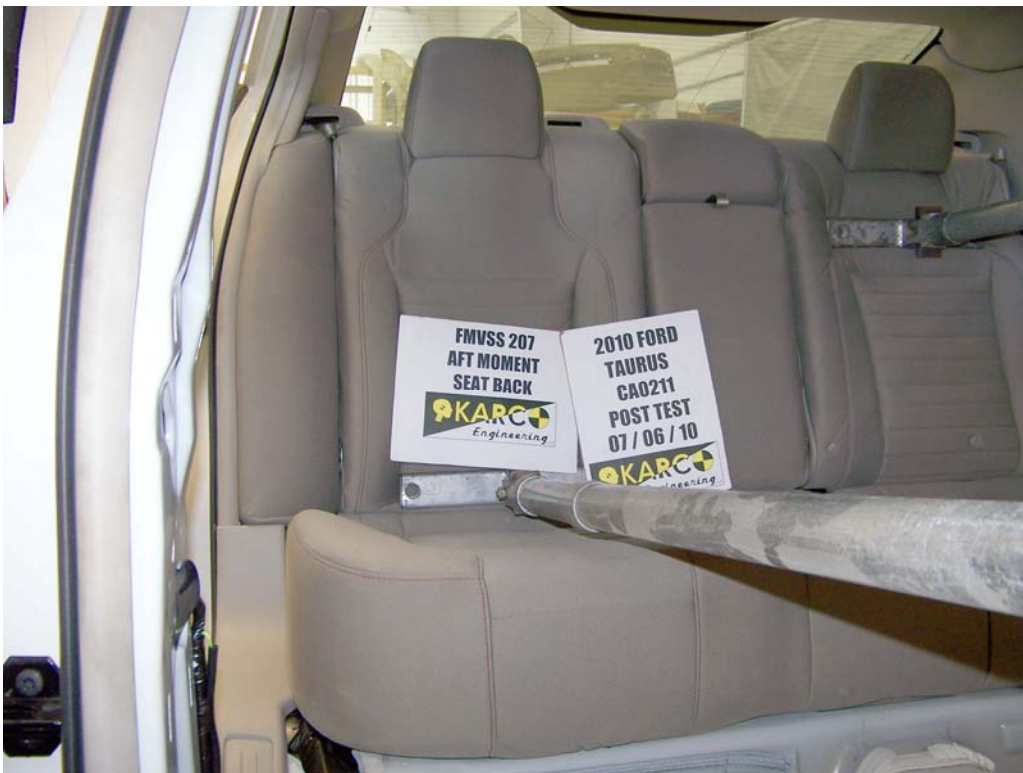
FIGURE 30. Aft Moment on Seat Back, P3, Post-Test
