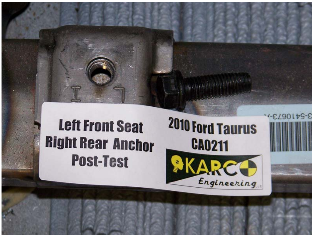
FIGURE 56. Floor Pan Anchor, P1, Post-Test
