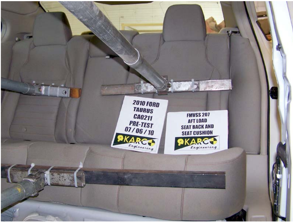
FIGURE 35. Aft Load Seat Back and Seat Cushion, P4, Pre-Test
