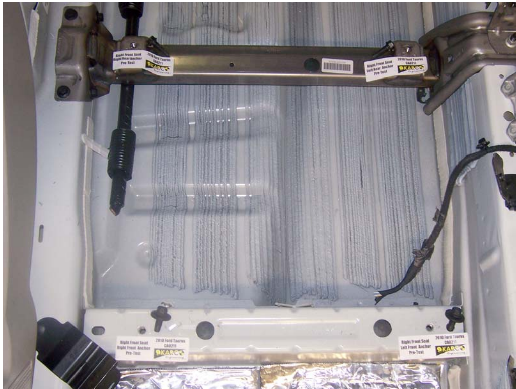
FIGURE 67. Floor Pan Anchors, P2 Overall, Pre-Test
