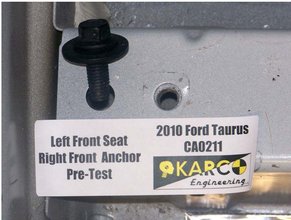
FIGURE 47. Floor Pan Anchor, P1, Pre-Test
