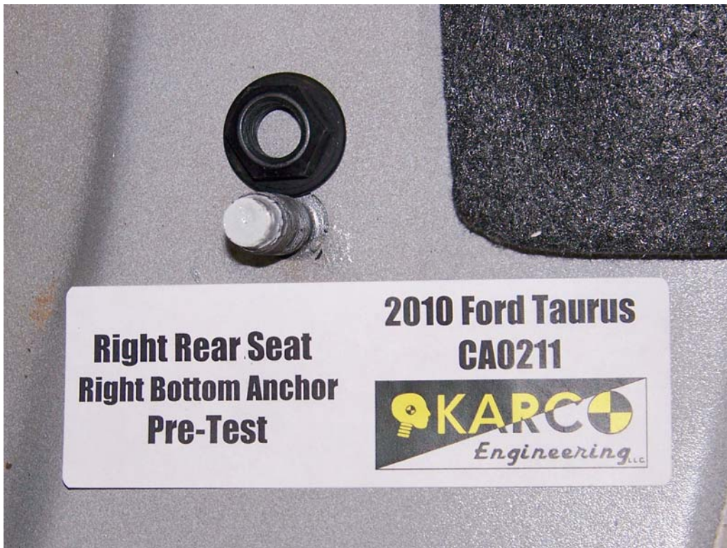
FIGURE 115. Floor Pan Anchor, P3, Pre-Test
