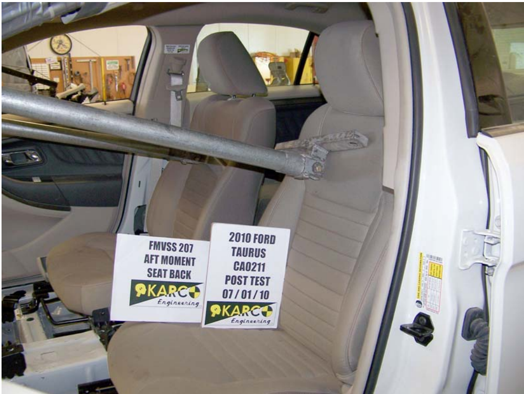
FIGURE 12. Aft Moment on Seat Back, P1, Post-Test
