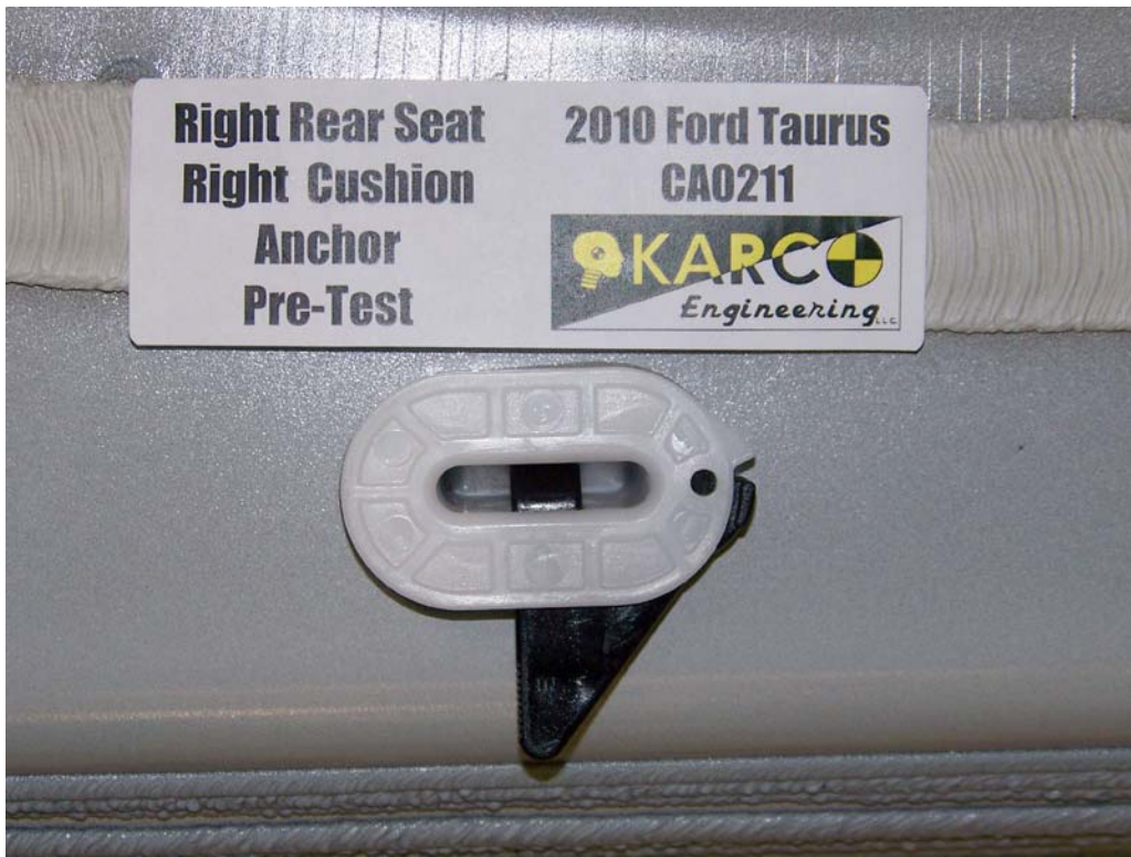
FIGURE 125. Floor Pan Anchor, P3, Pre-Test
