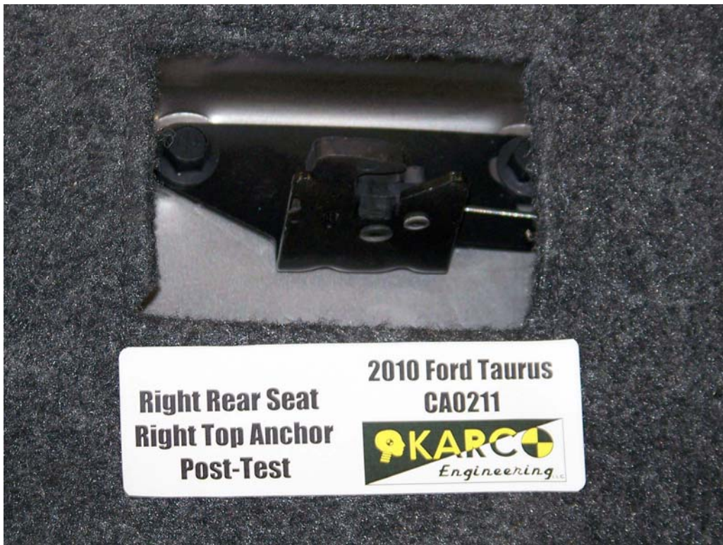
FIGURE 110. Seat Back Anchor, P3, Post-Test
