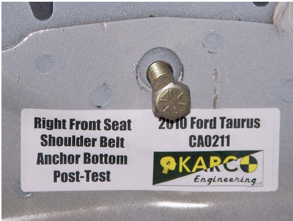
FIGURE 90. Shoulder Belt Anchor, P2, Post-Test
