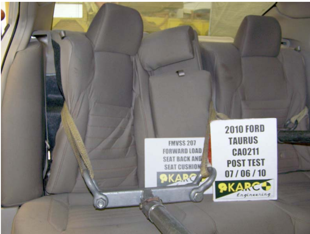
FIGURE 34. Forward Load on Seat Back and Seat Cushion, P3, Post-Test
