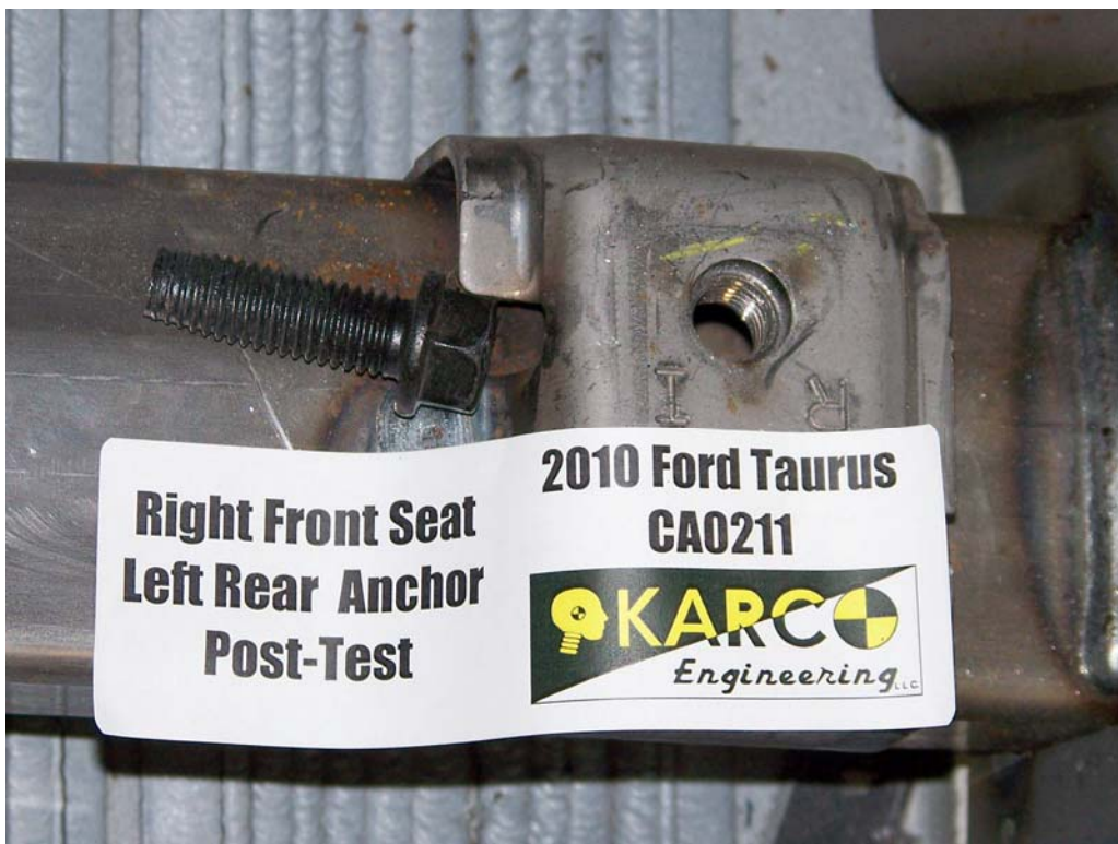
FIGURE 80. Floor Pan Anchor, P2, Post-Test
