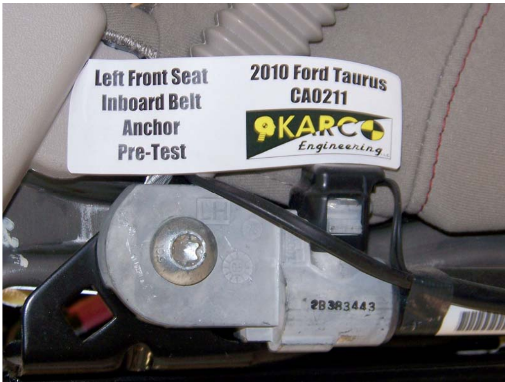
FIGURE 65. Belt Anchor, P1, Pre-Test
