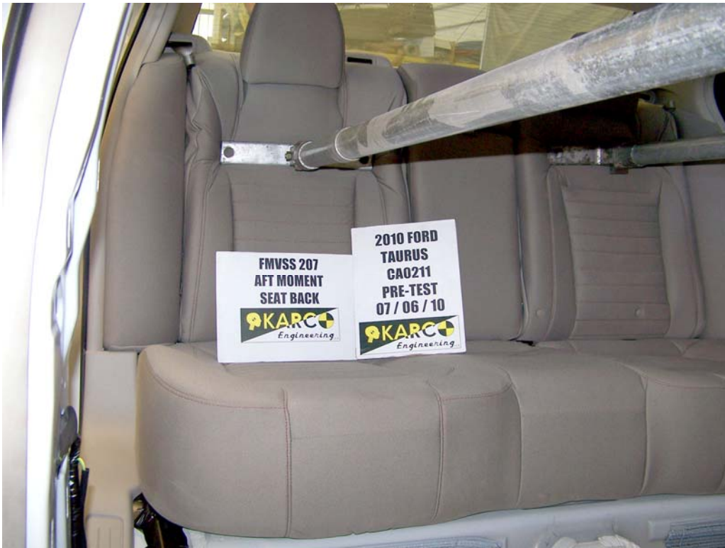
FIGURE 29. Aft Moment on Seat Back, P3, Pre-Test
