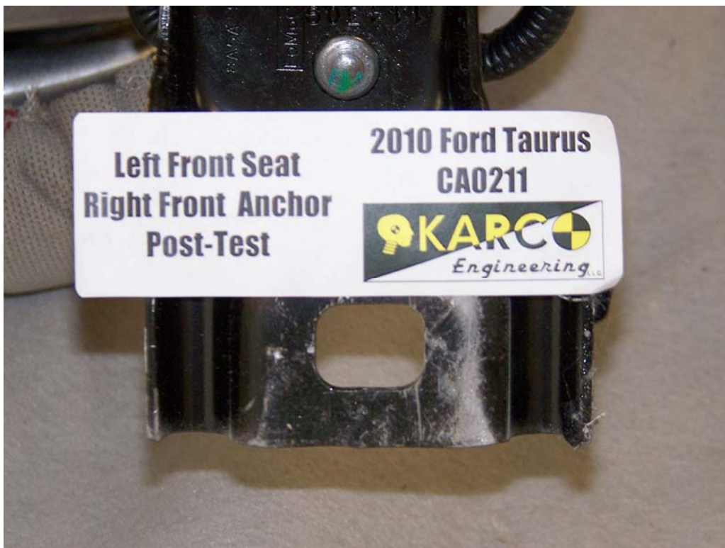
FIGURE 50. Seat Anchor, P1, Post-Test
