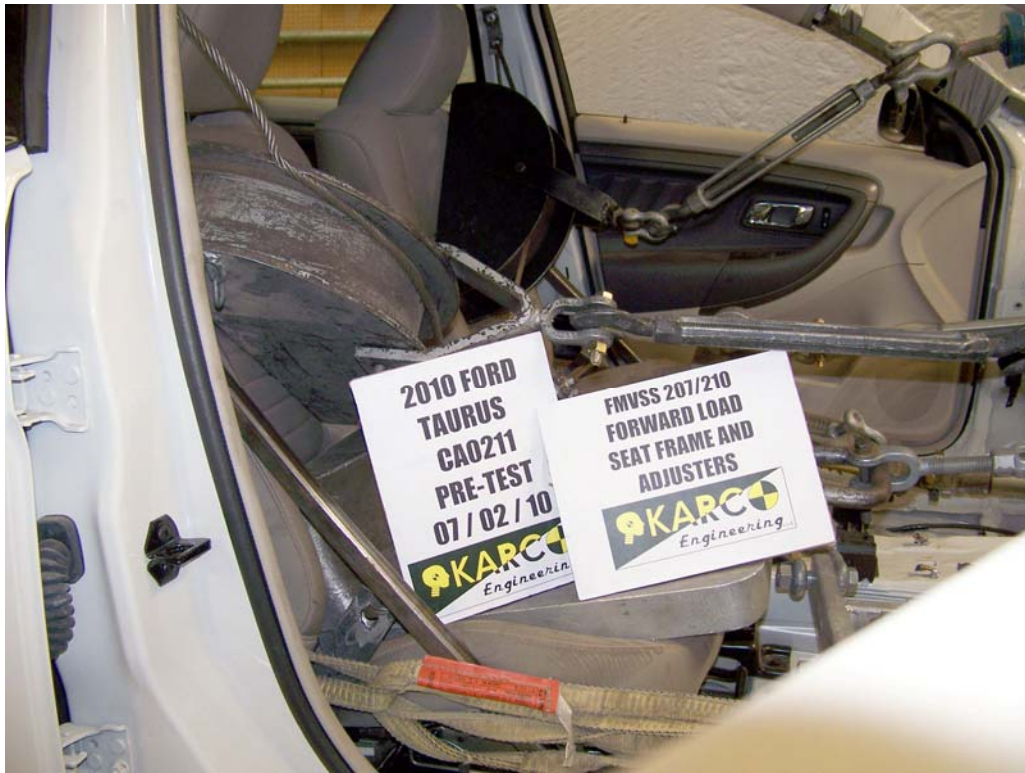
FIGURE 25. 207/210 Forward Load on Seat Frame and Adjusters, P2, Pre-Test
