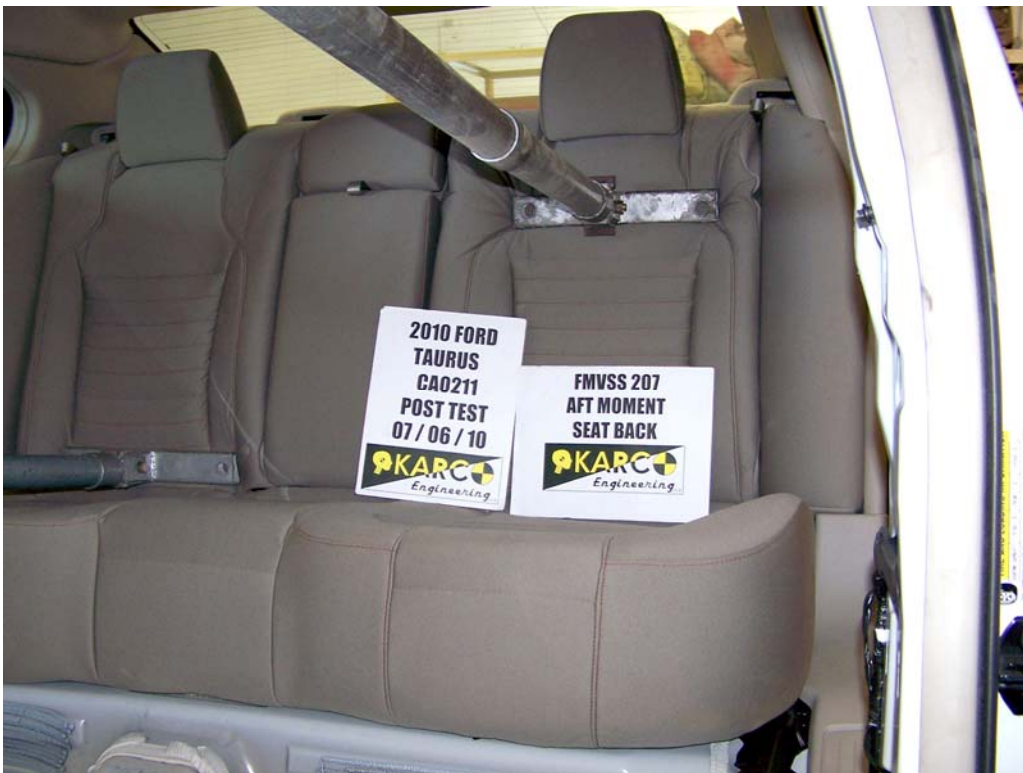
FIGURE 28. Aft Moment on Seat Back, P4, Post-Test
