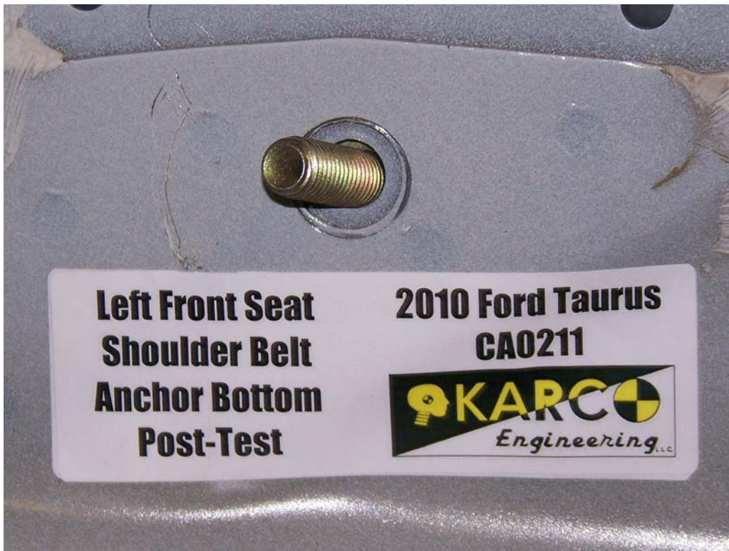
FIGURE 62. Shoulder Belt Anchor, P1, Post-Test
