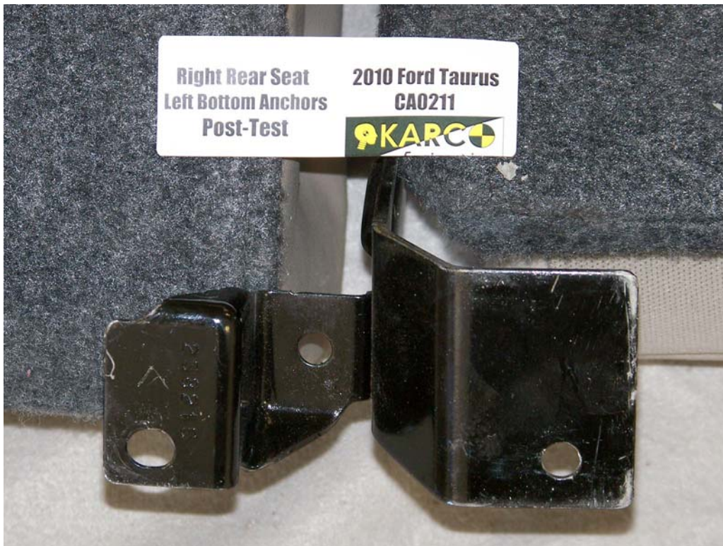
FIGURE 114. Seat Back Anchor, P3, Post-Test
