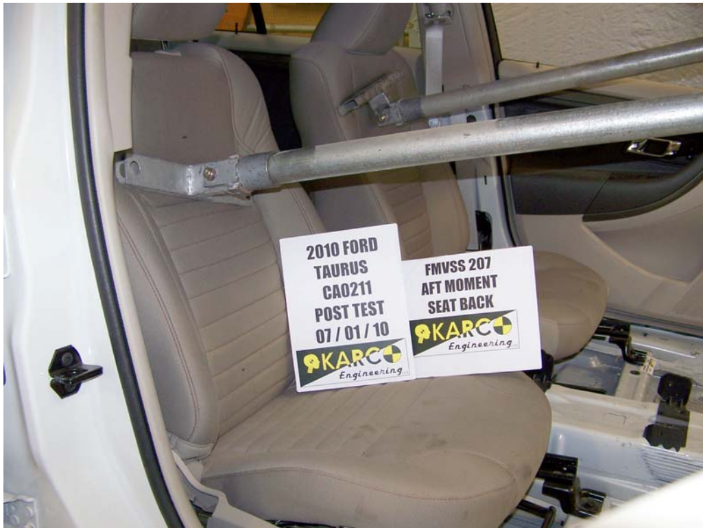
FIGURE 14. Aft Moment on Seat Back, P2, Post-Test
