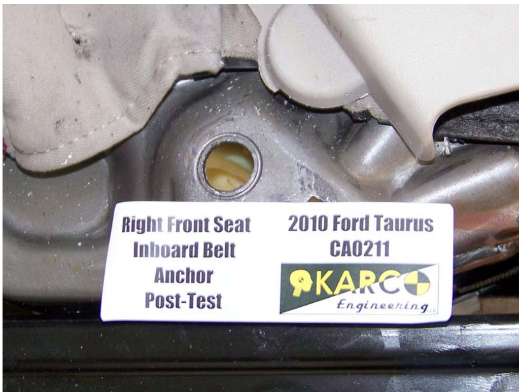
FIGURE 94. Belt Anchor, P2, Post-Test
