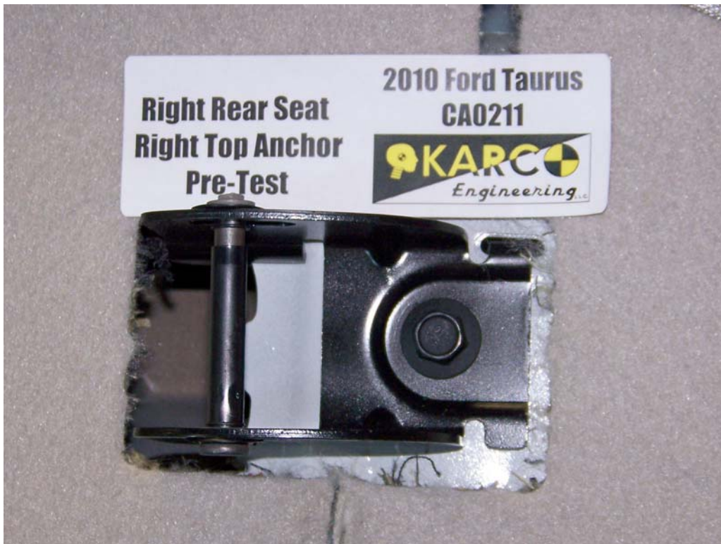
FIGURE 107. Floor Pan Anchor, P3, Pre-Test
