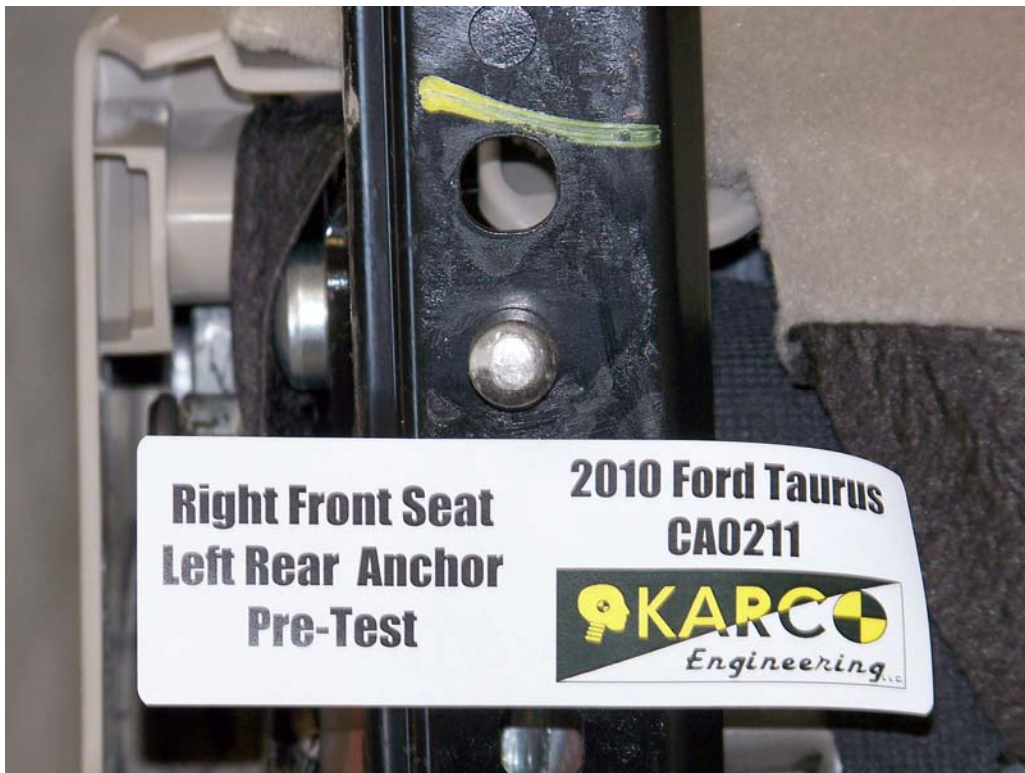
FIGURE 81. Seat Anchor, P2, Pre-Test
