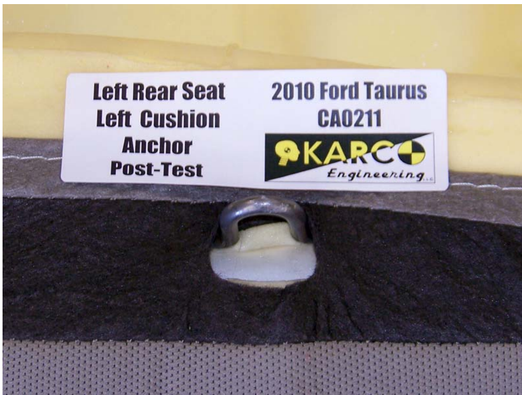
FIGURE 124. Seat Cushion Anchor, P4, Post-Test
