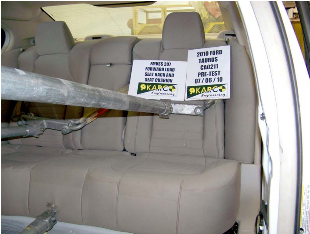
FIGURE 31. Forward Load on Seat Back and Seat Cushion, P4, Pre-Test
