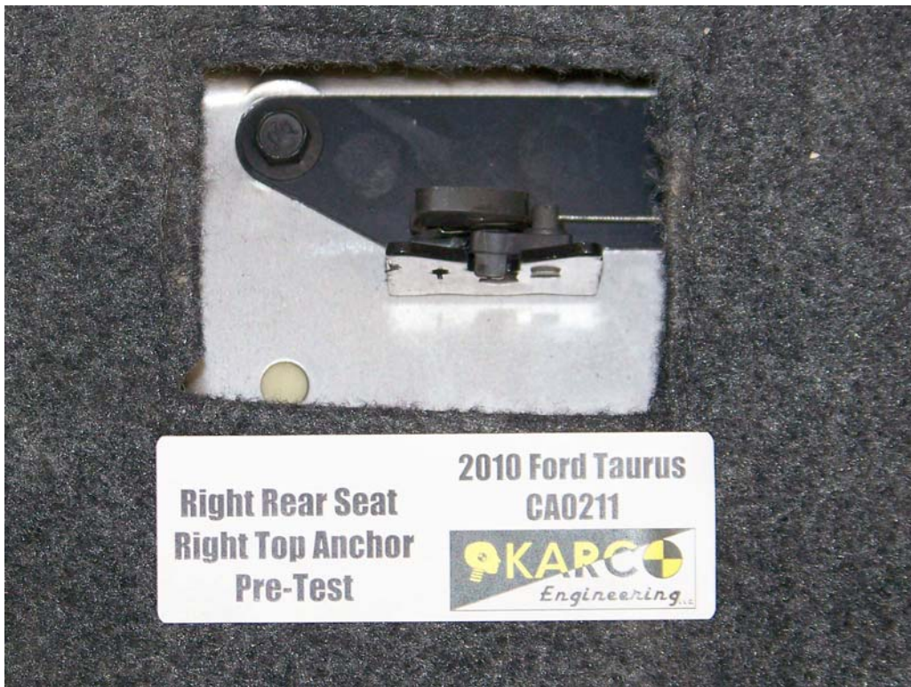
FIGURE 109. Seat Back Anchor, P3, Pre-Test
