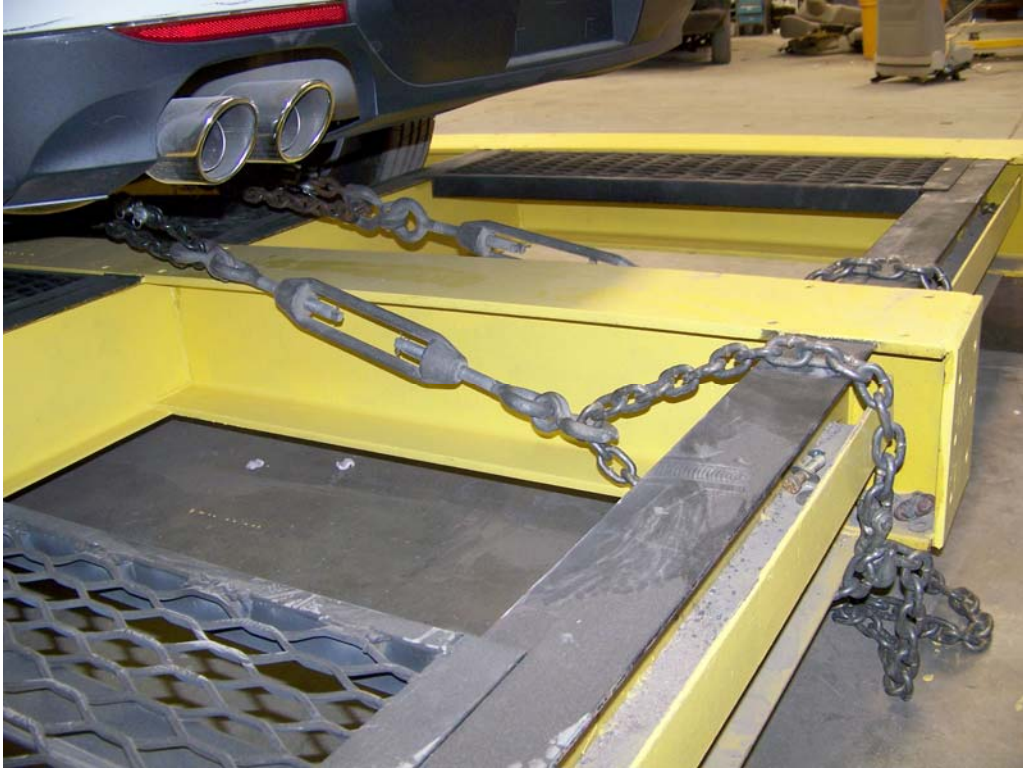
FIGURE 9. Vehicle Mounted in Test Fixture
