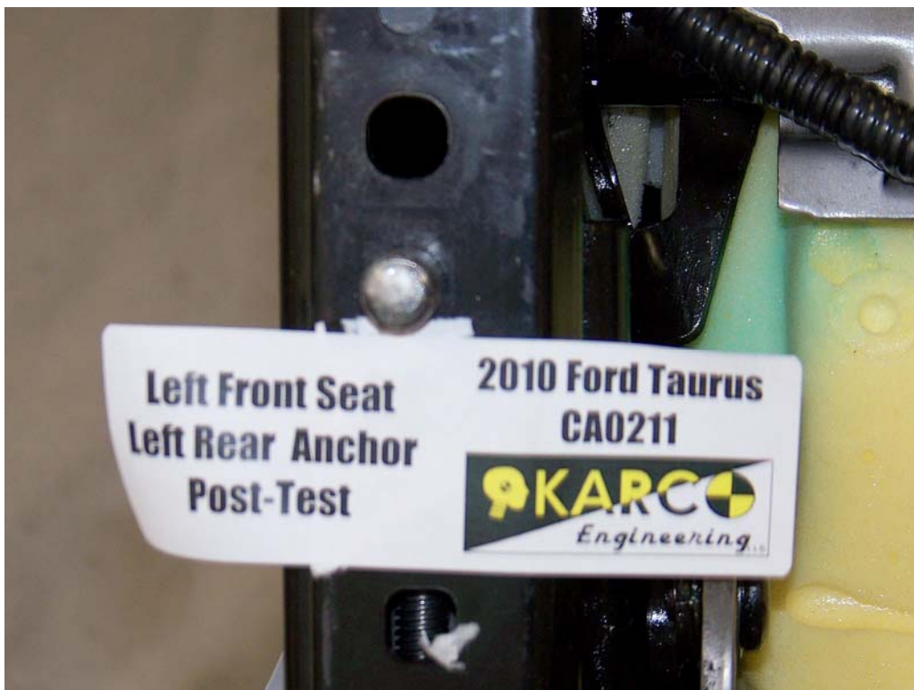
FIGURE 54. Seat Anchor, P1, Post-Test
