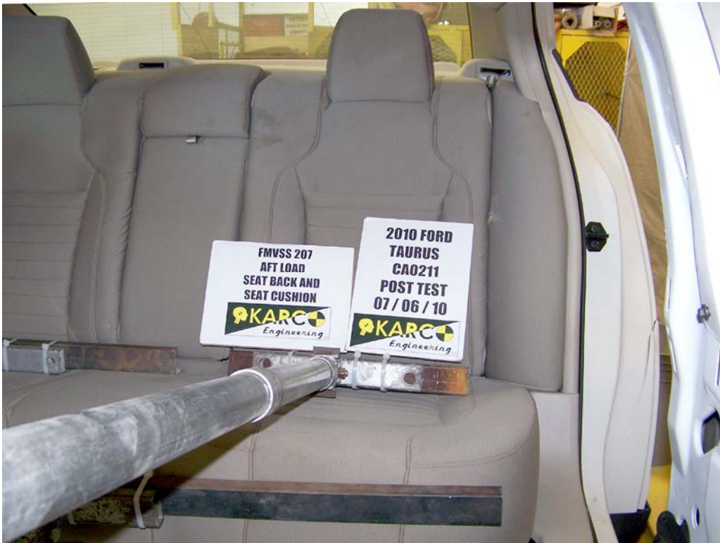
FIGURE 36. Aft Load on Seat Back and Seat Cushion, P4, Post-Test
