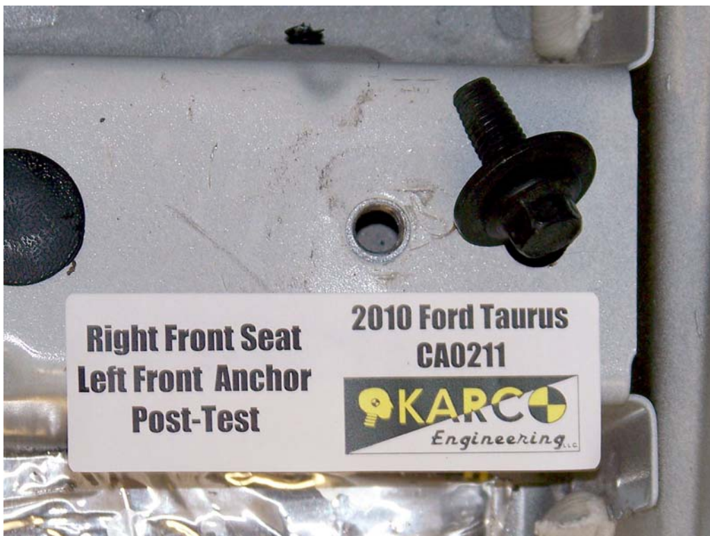
FIGURE 72. Floor Pan Anchor, P2, Post-Test
