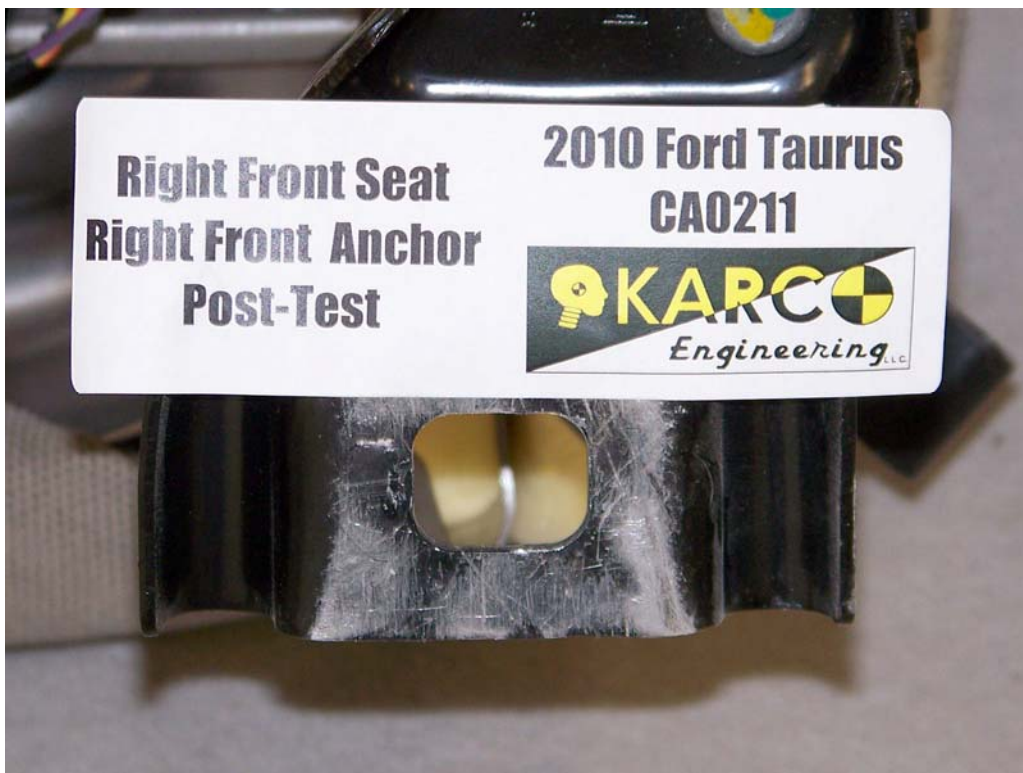
FIGURE 78. Seat Anchor, P2, Post-Test
