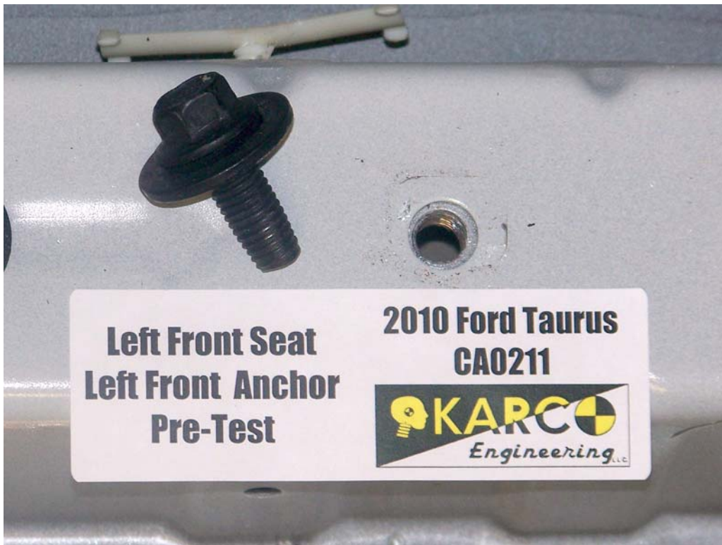
FIGURE 43. Floor Pan Anchor, P1, Pre-Test
