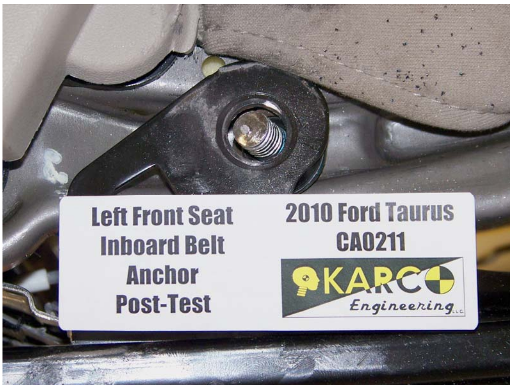
FIGURE 66. Belt Anchor, P1, Post-Test
