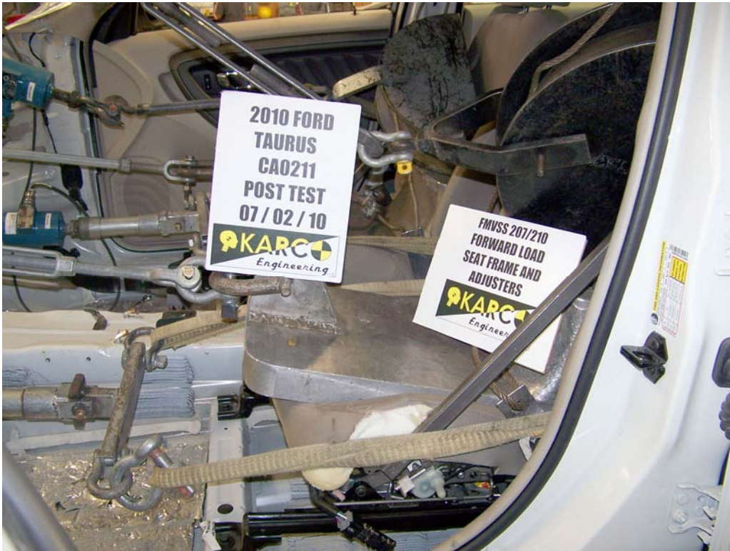
FIGURE 24. 207/210 Forward Load on Seat Frame and Adjusters, P1, Post-Test
