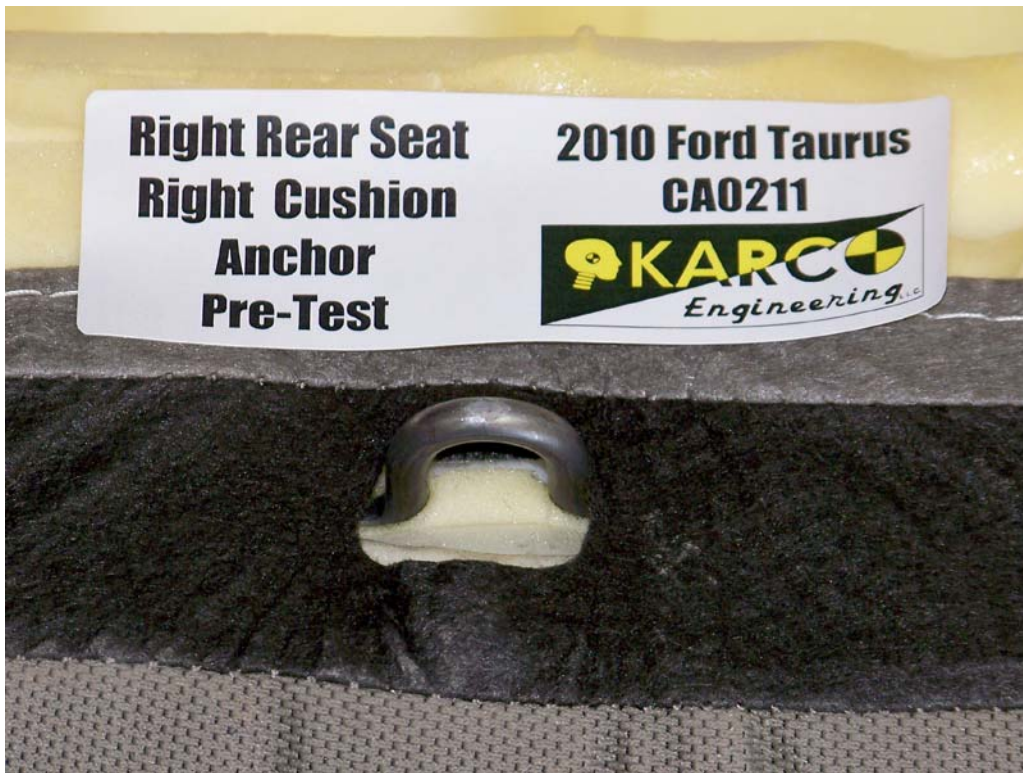
FIGURE 127. Seat Cushion Anchor, P3, Pre-Test
