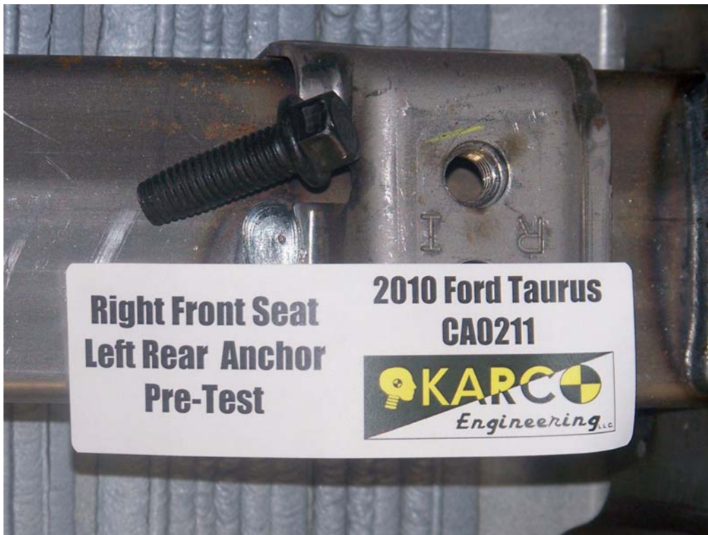
FIGURE 79. Floor Pan Anchor, P2, Pre-Test
