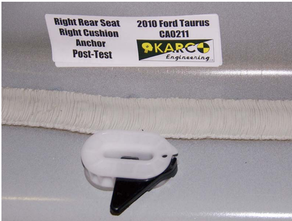
FIGURE 126. Floor Pan Anchor, P3, Post-Test
