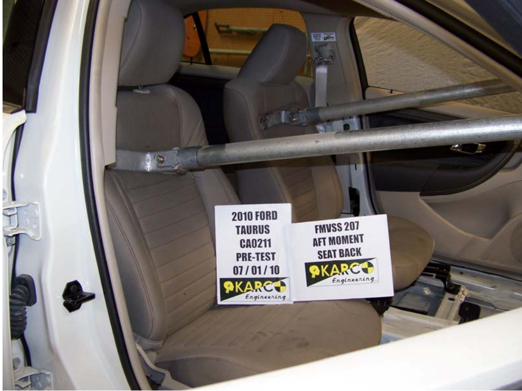
FIGURE 13. Aft Moment on Seat Back, P2, Pre-Test
