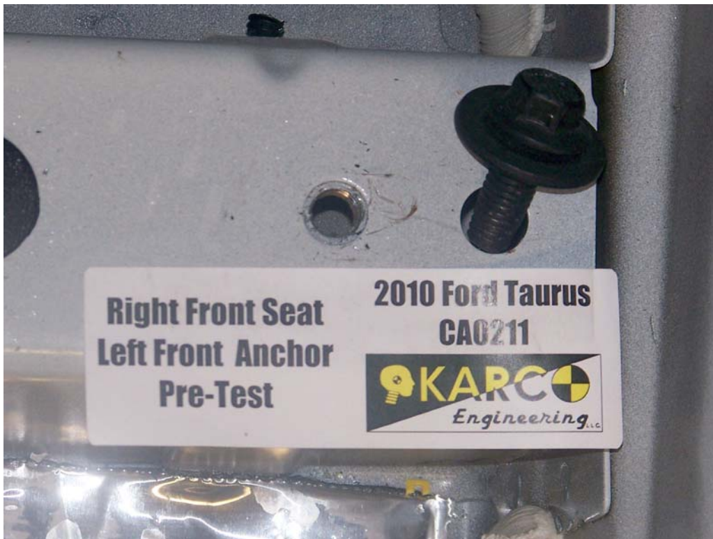
FIGURE 71. Floor Pan Anchor, P2, Pre-Test
