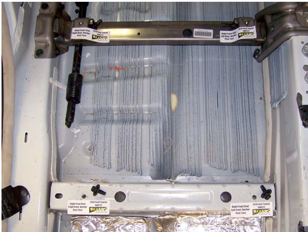
FIGURE 68. Floor Pan Anchors, P2 Overall, Post-Test
