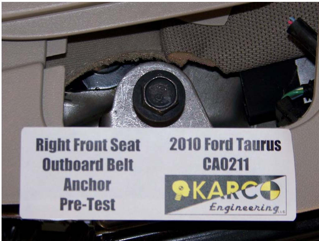
FIGURE 91. Belt Anchor, P2, Pre-Test
