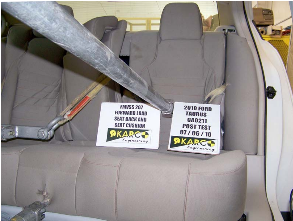
FIGURE 32. Forward Load on Seat Back and Seat Cushion, P4, Post-Test
