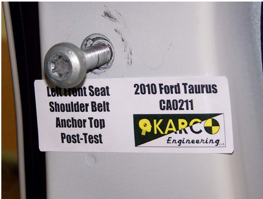
FIGURE 60. Shoulder Belt Anchor, P1, Post-Test
