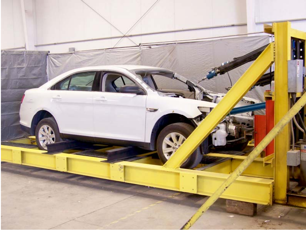
FIGURE 7. Vehicle Mounted in Test Fixture
