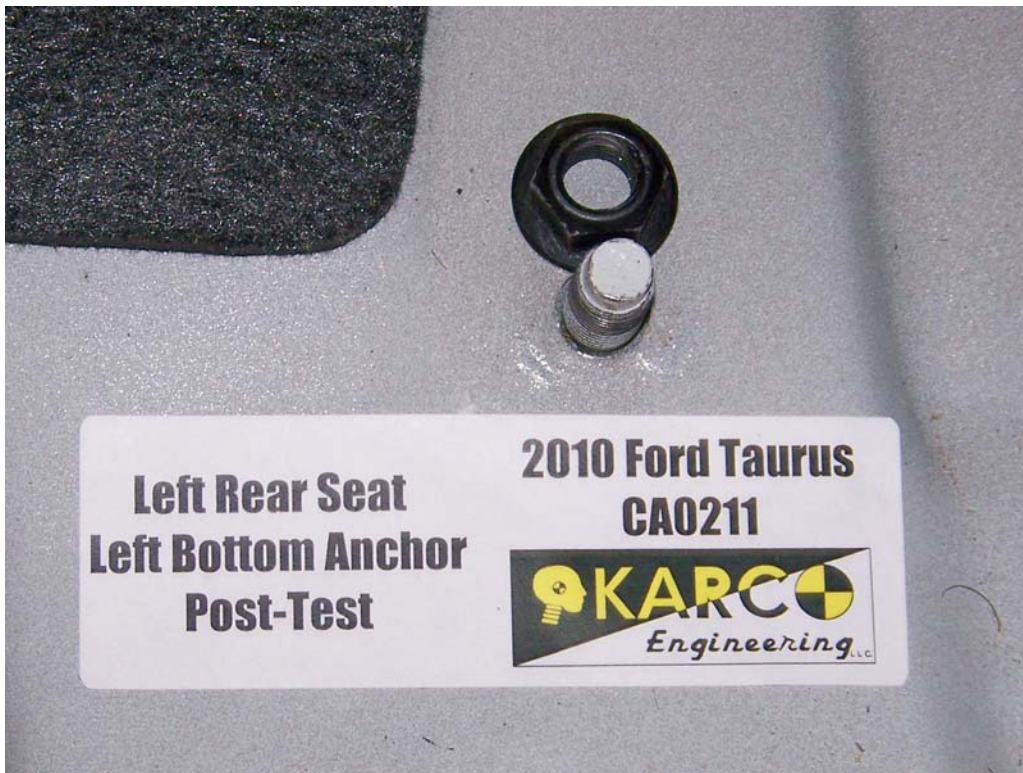
FIGURE 104. Floor Pan Anchor, P4, Post-Test
