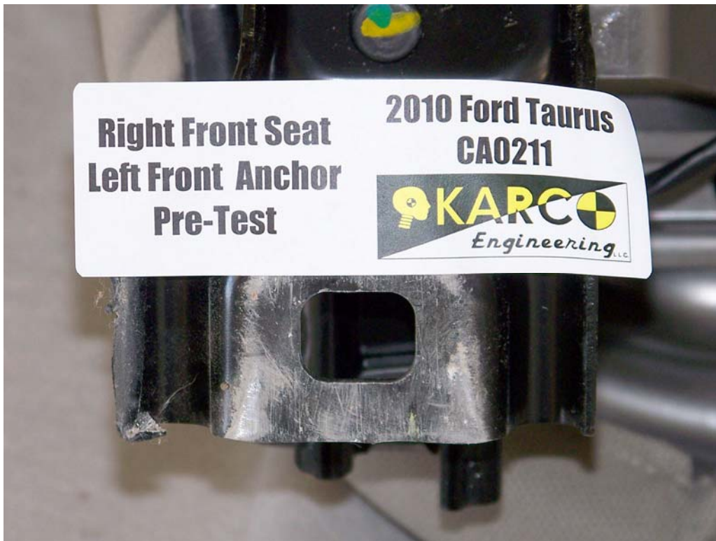
FIGURE 73. Seat Anchor, P2, Pre-Test
