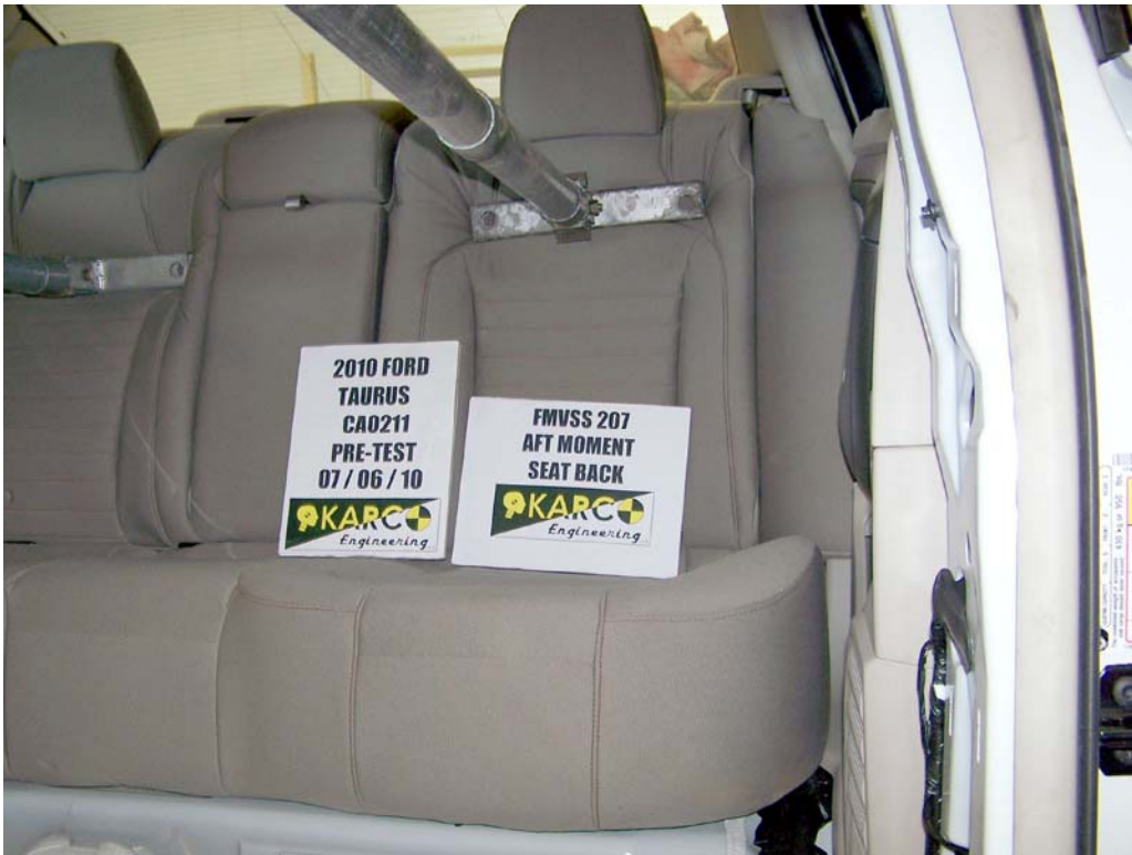
FIGURE 27. Aft Moment on Seat Back, P4, Pre-Test
