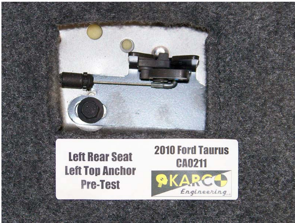
FIGURE 101. Seat Back Anchor, P4, Pre-Test
