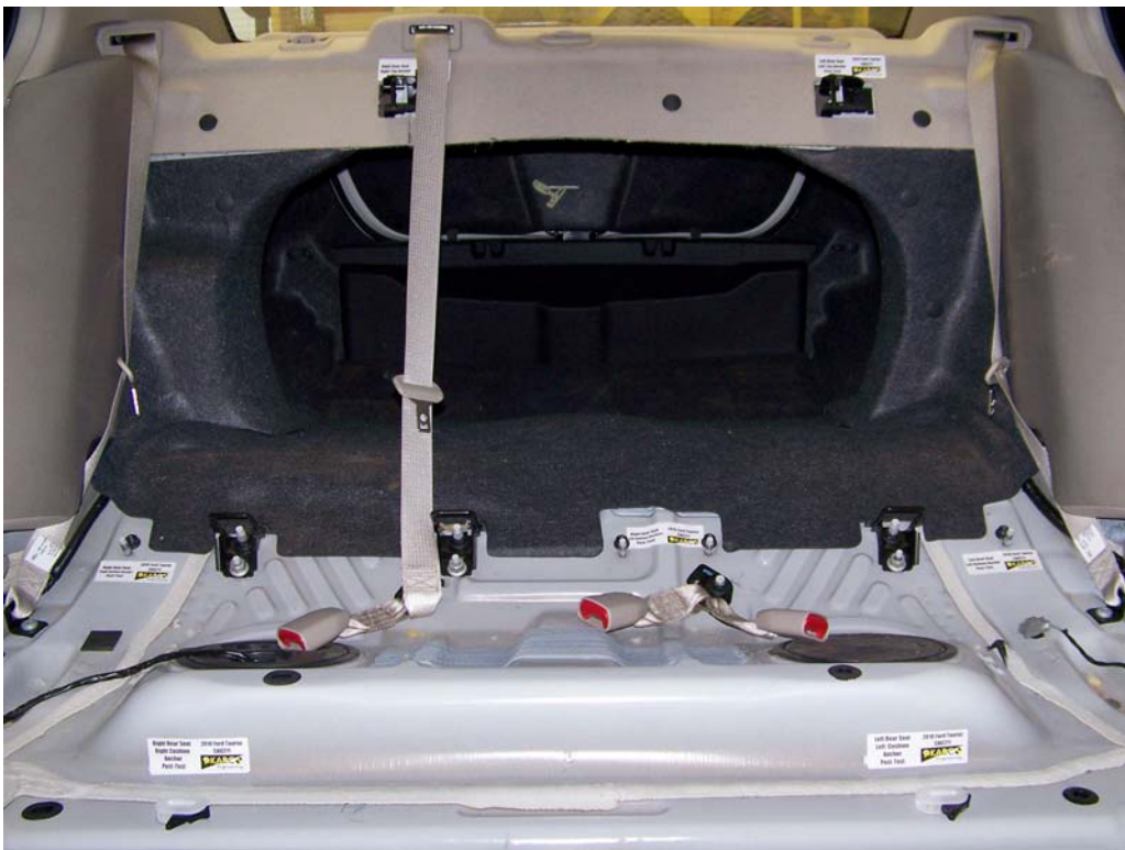
FIGURE 96. Floor Pan Anchors, P3-P4 Overall, Post-Test
