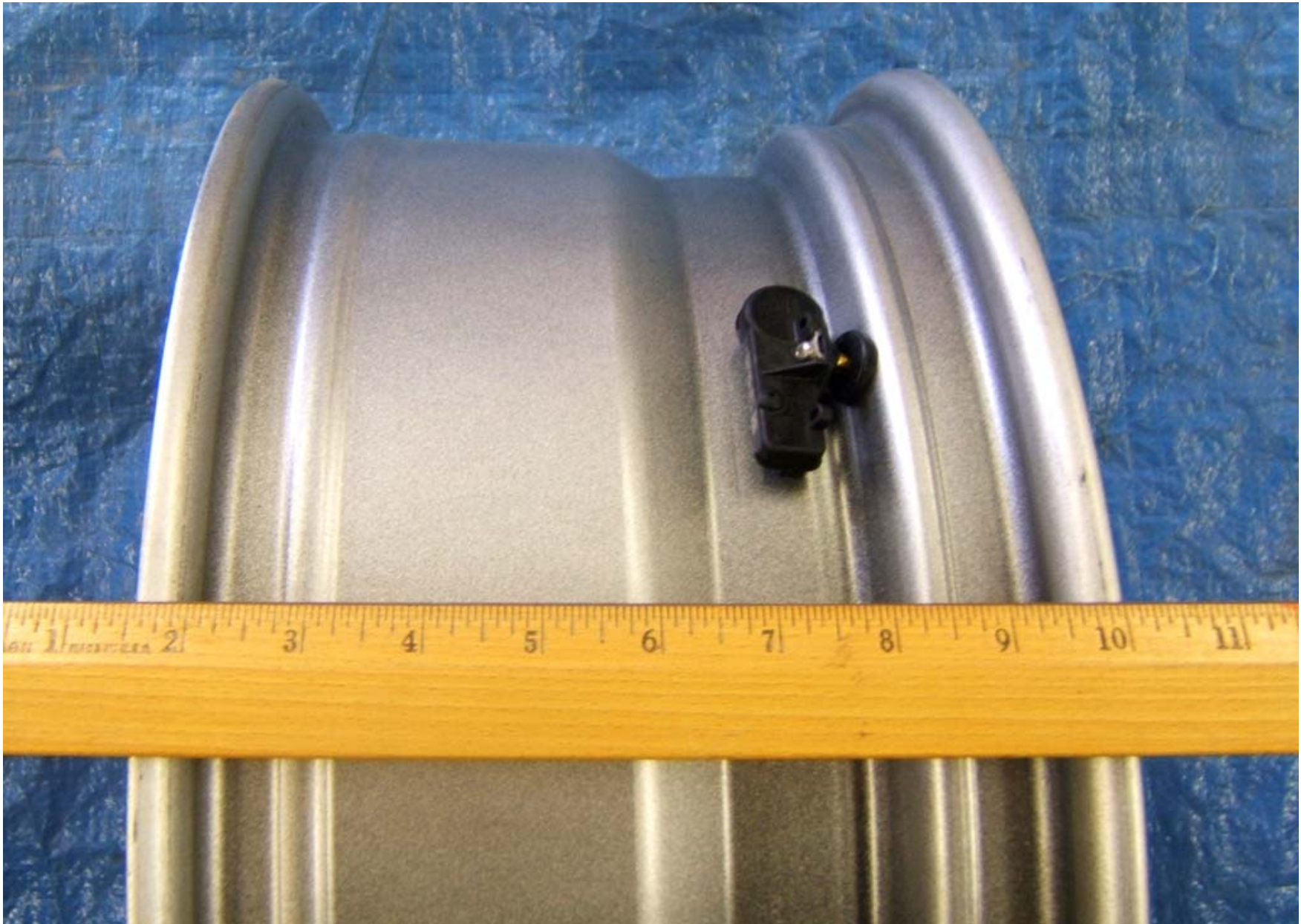
FIGURE 5.12 RIM CONTOUR FOR FULL WIDTH OF CROSS SECTION
