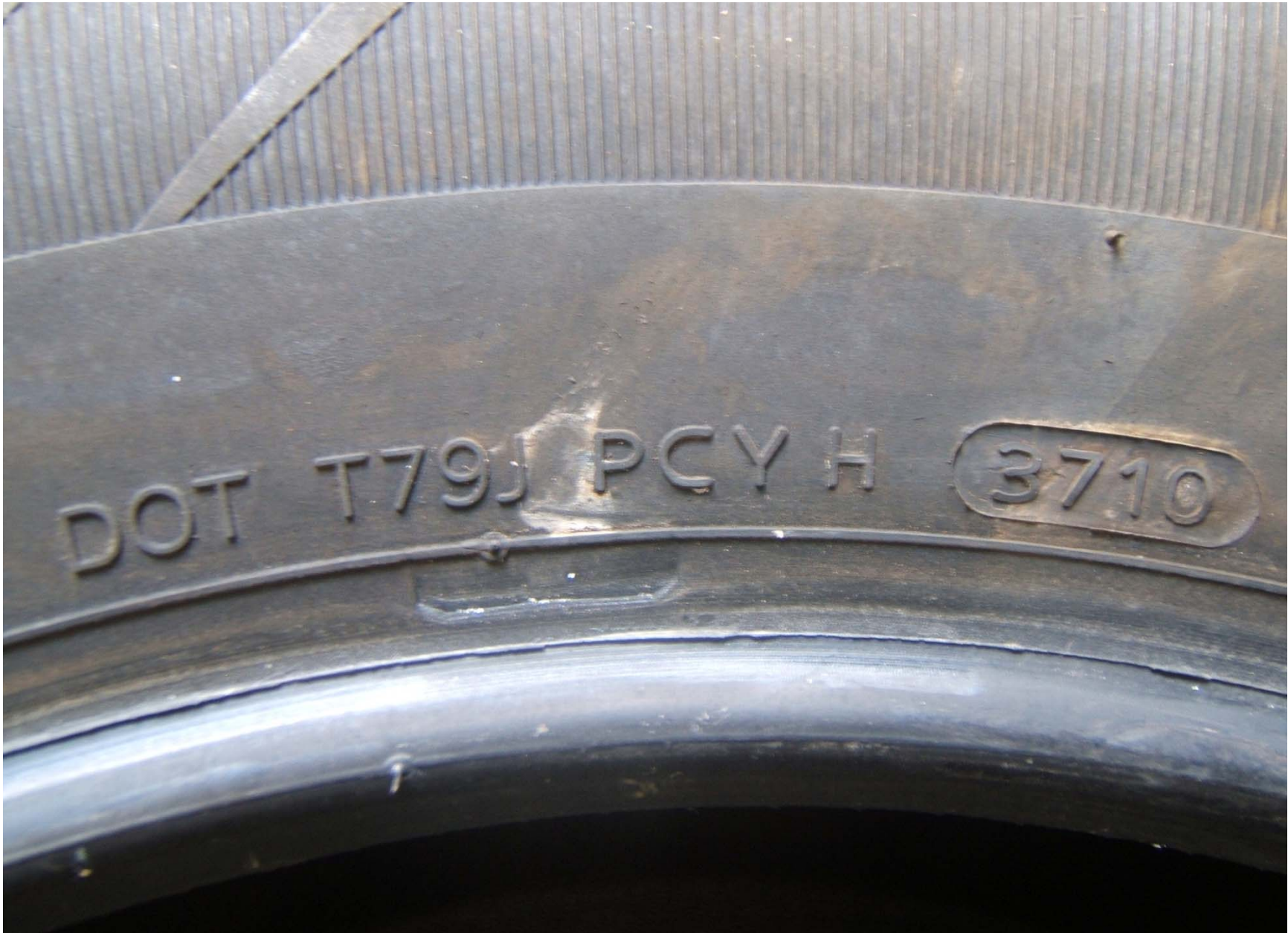
FIGURE 5.9 TIRE SHOWING SERIAL NUMBER
