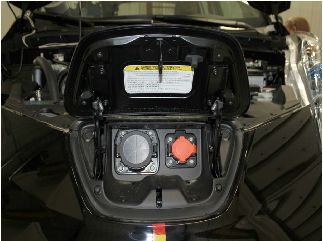
Vehicle Charging Warning Location
