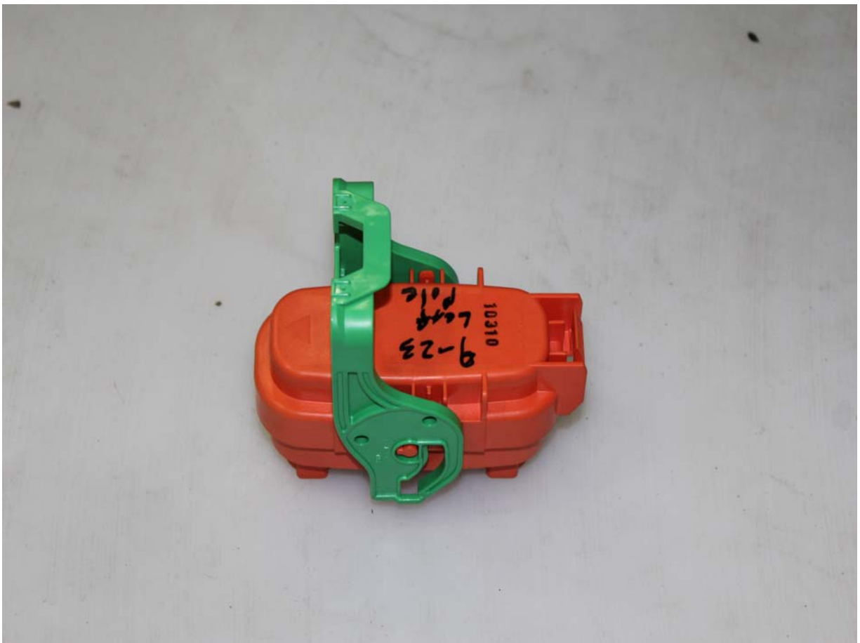
Manual High Voltage Service Disconnect
