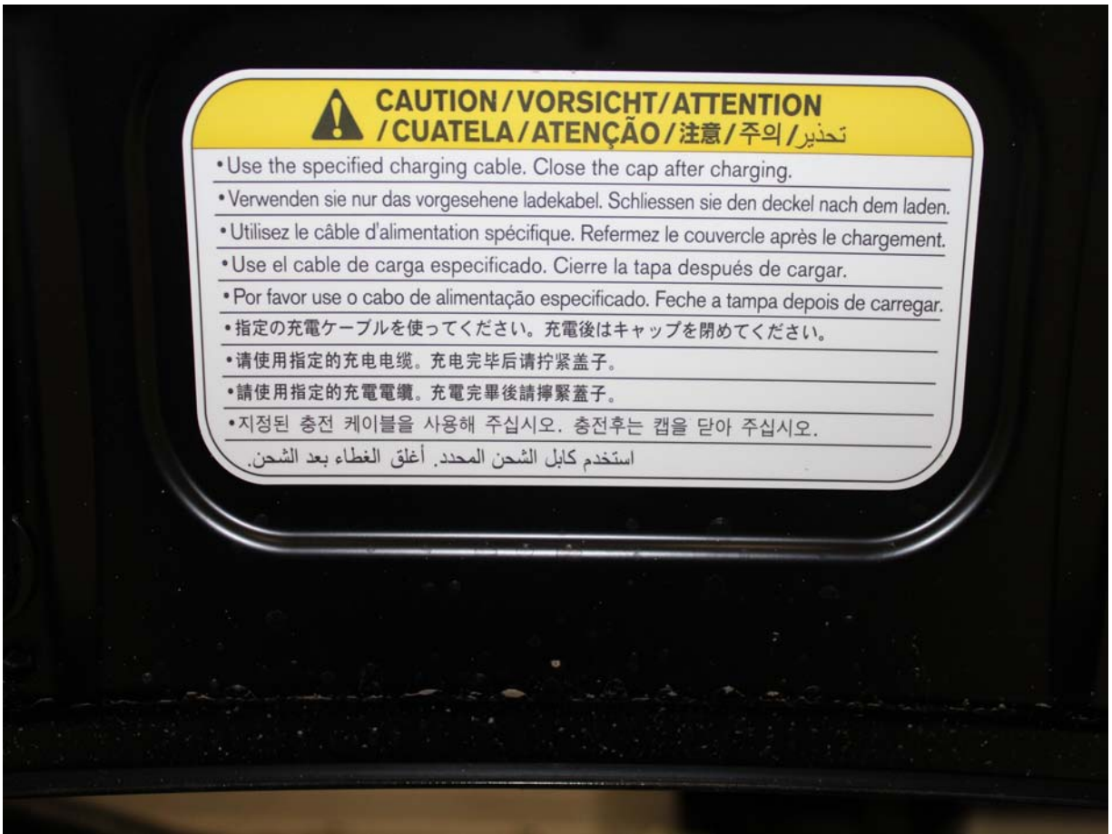
Vehicle Charging Warning Label
