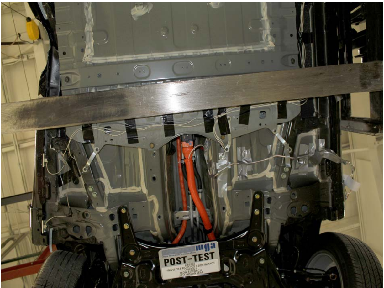
High Voltage Location
