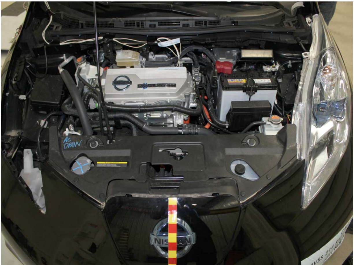
Pre-Test View of Electric Propulsion Drive
