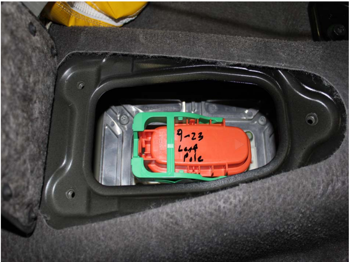
Manual High Voltage Service Disconnect
