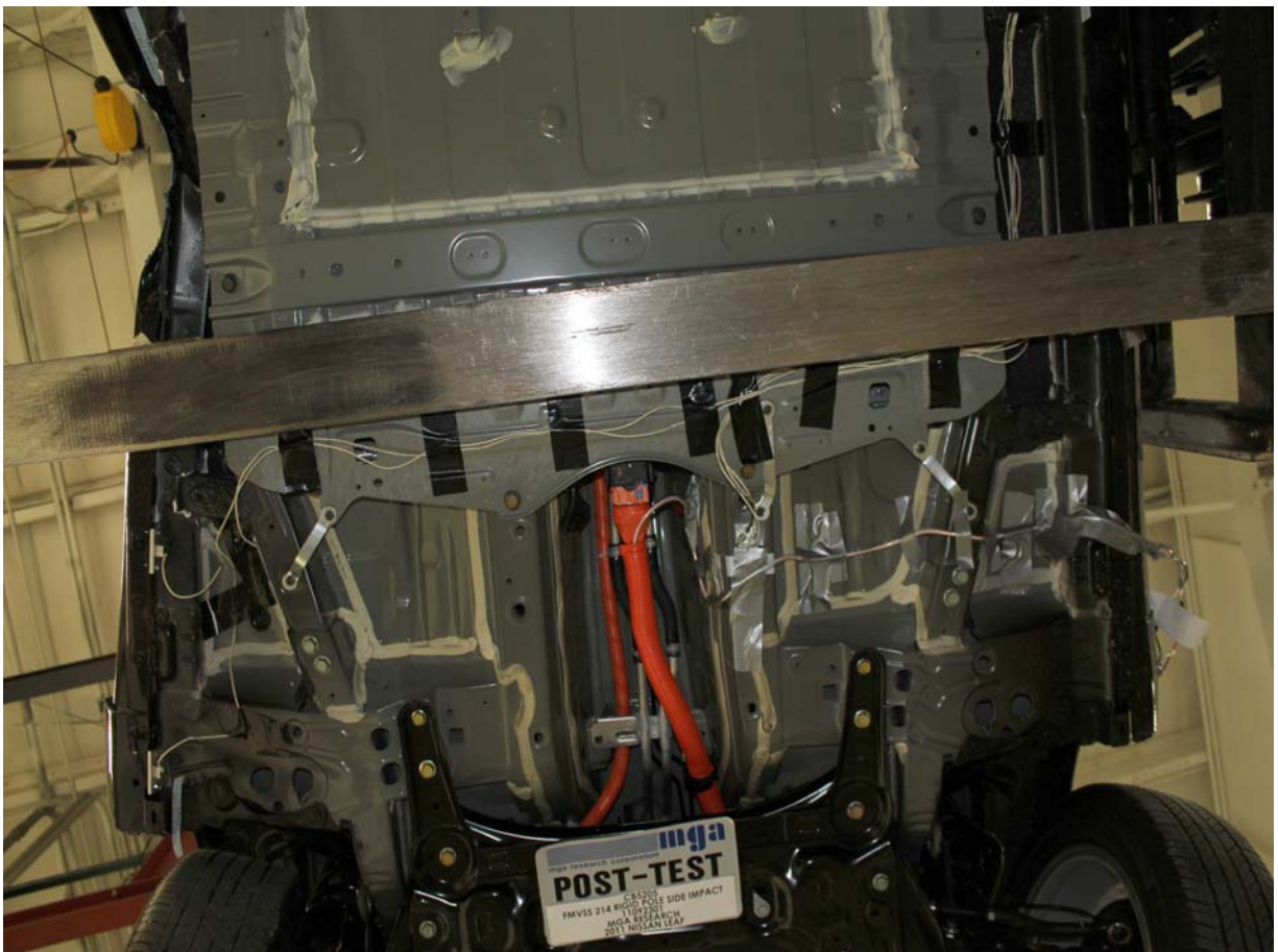
Post-Test View of Propulsion Battery (Front View)
