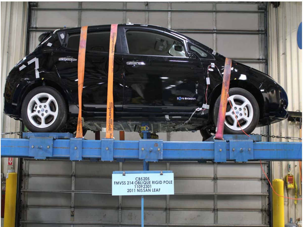
Vehicle at 360 Degrees on Static Rollover Device
