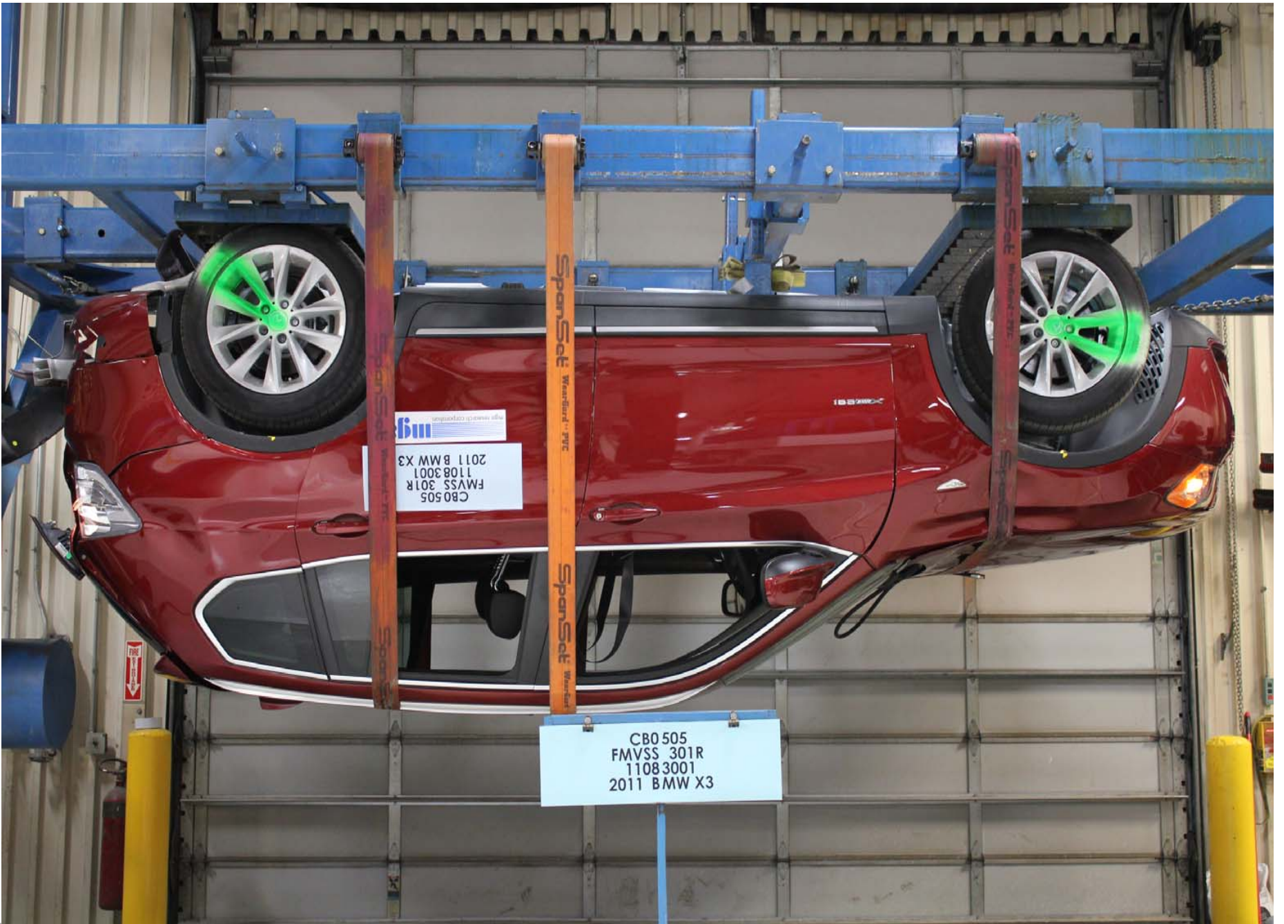
Static Rollover at 180 Degrees
