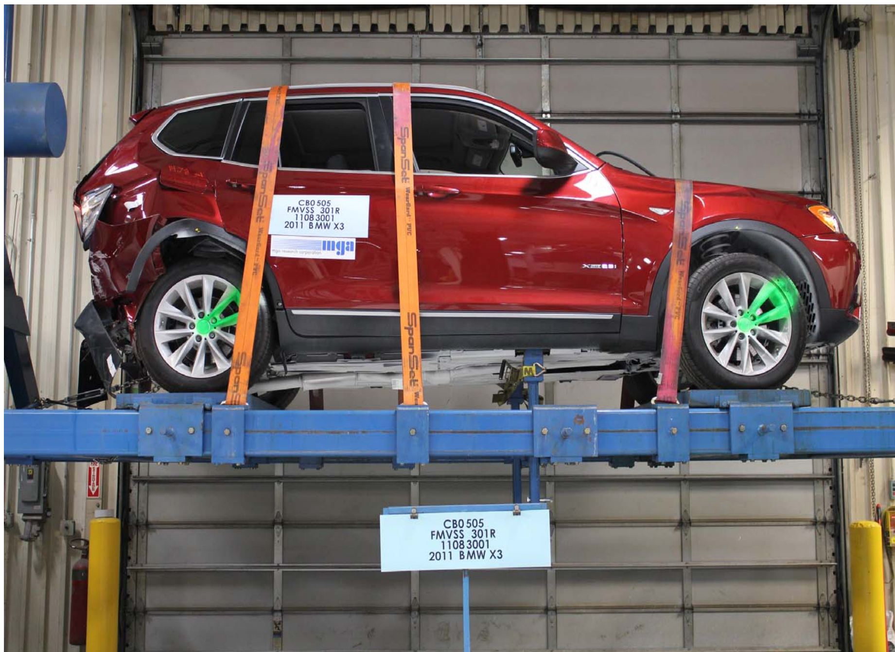
Static Rollover at 360 Degrees
