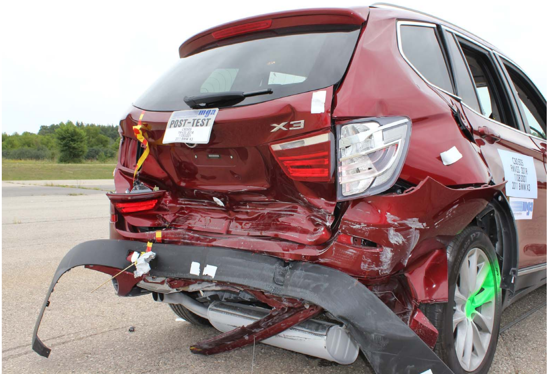
Post-Test Right Rear Close-up View of Vehicle
