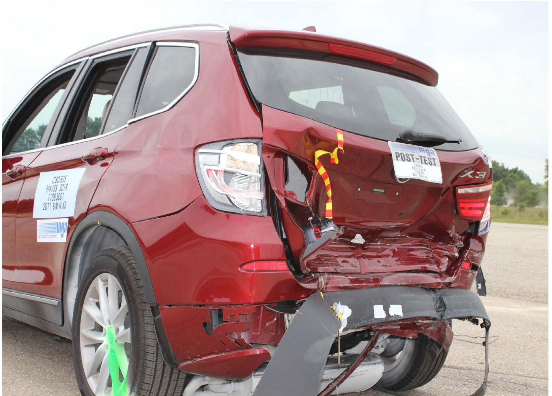
Post-Test Left Rear Close-up View of Vehicle
