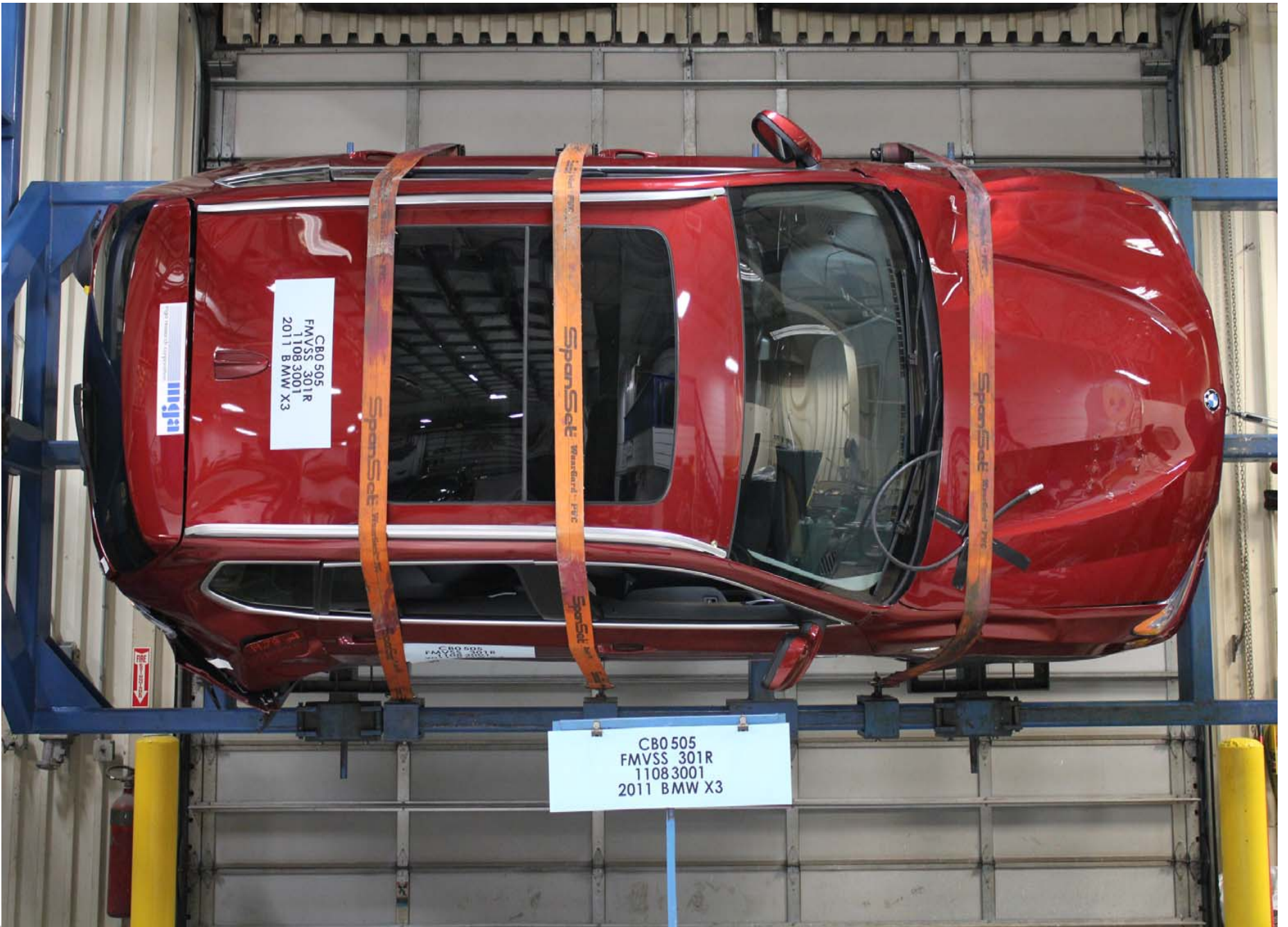
Static Rollover at 90 Degrees
