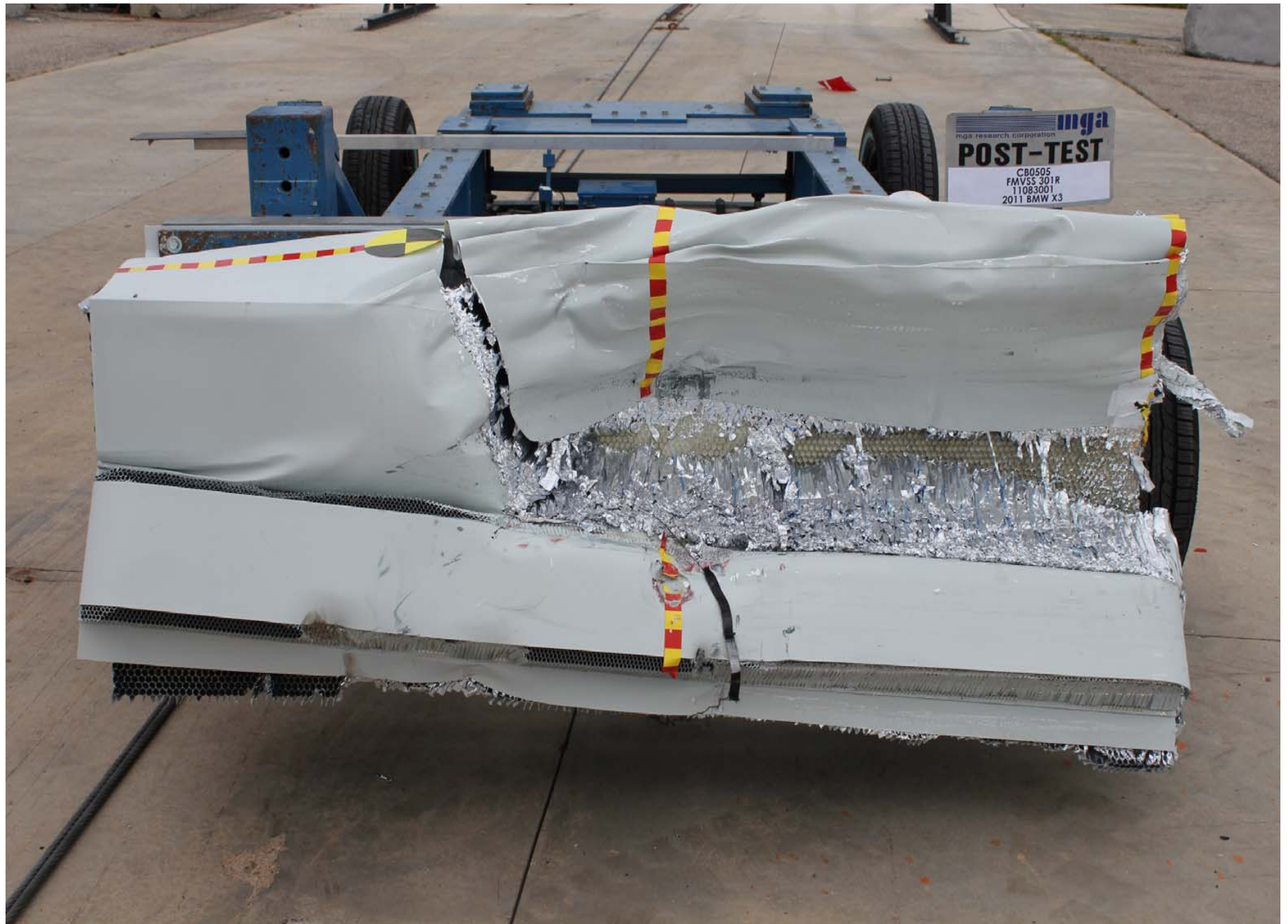
Post-Test Front View of MDB
