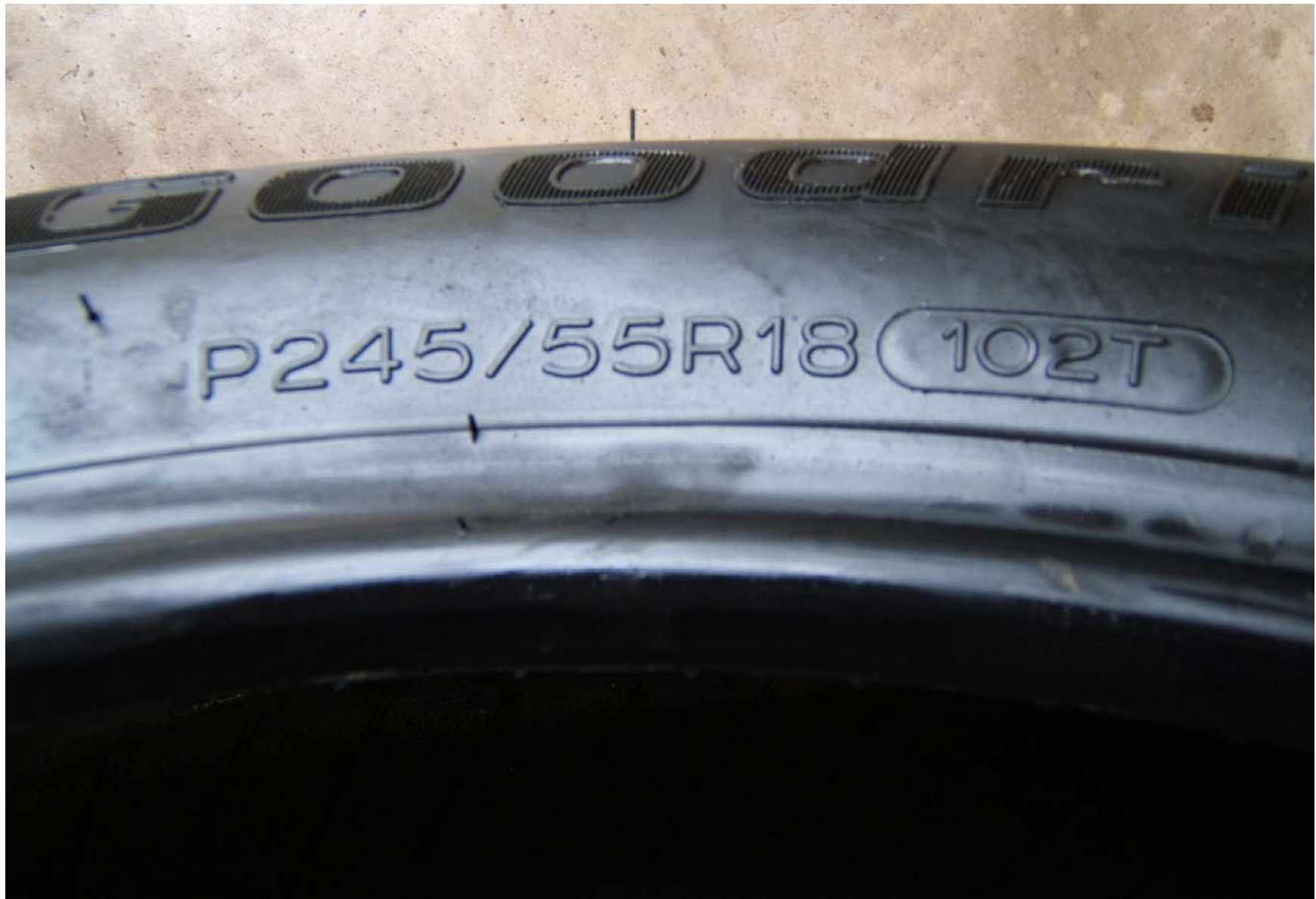
FIGURE 5.6 TIRE SHOWING SIZE AND LOAD INDEX / SPEED RATING
