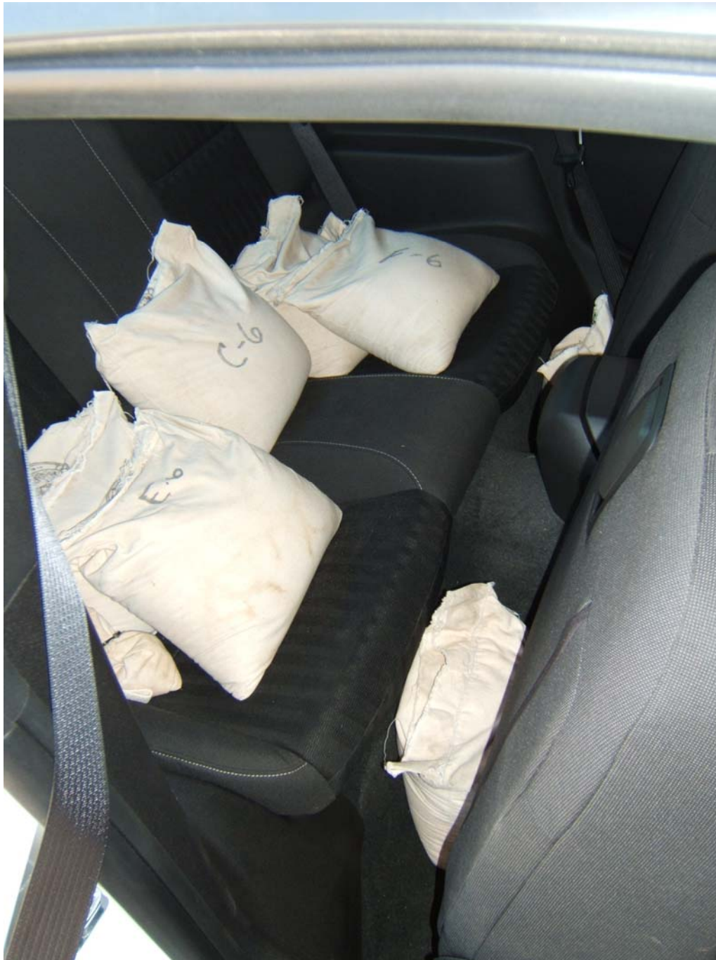
FIGURE 5.16 VEHICLE REAR SEAT BALLAST FOR UVW + VCW LOAD
