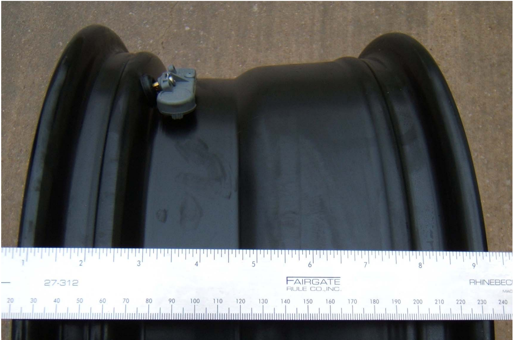
FIGURE 5.10 RIM SHOWING TPMS SENSOR AND RIM CONTOUR FOR FULL WIDTH OF CROSS SECTION
