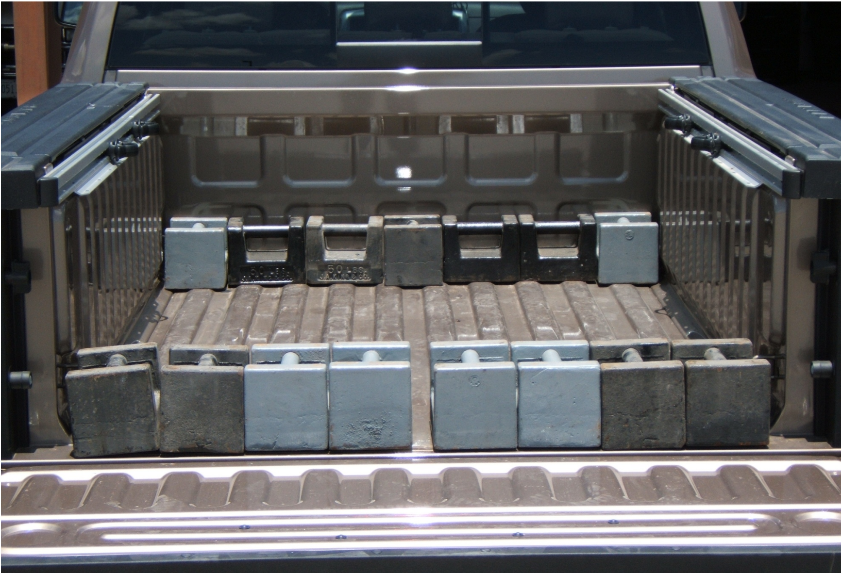
FIGURE 5.15 VEHICLE CARGO AREA BALLAST FOR UVW + VCW LOAD
