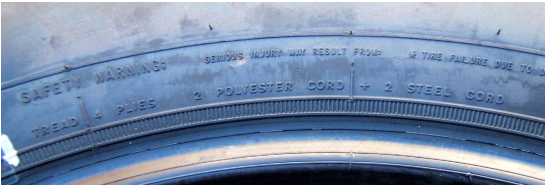
FIGURE 5.10 TIRE SHOWING SIDEWALL / TREAD CONSTRUCTION
