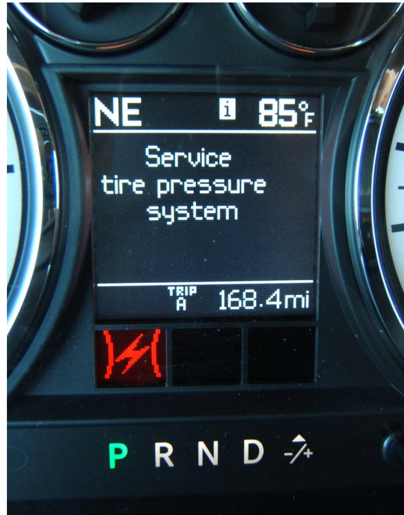
FIGURE 5.18 RECONFIGURABLE DISPLAY SHOWING TPMS MALFUNCTION SCREENS
