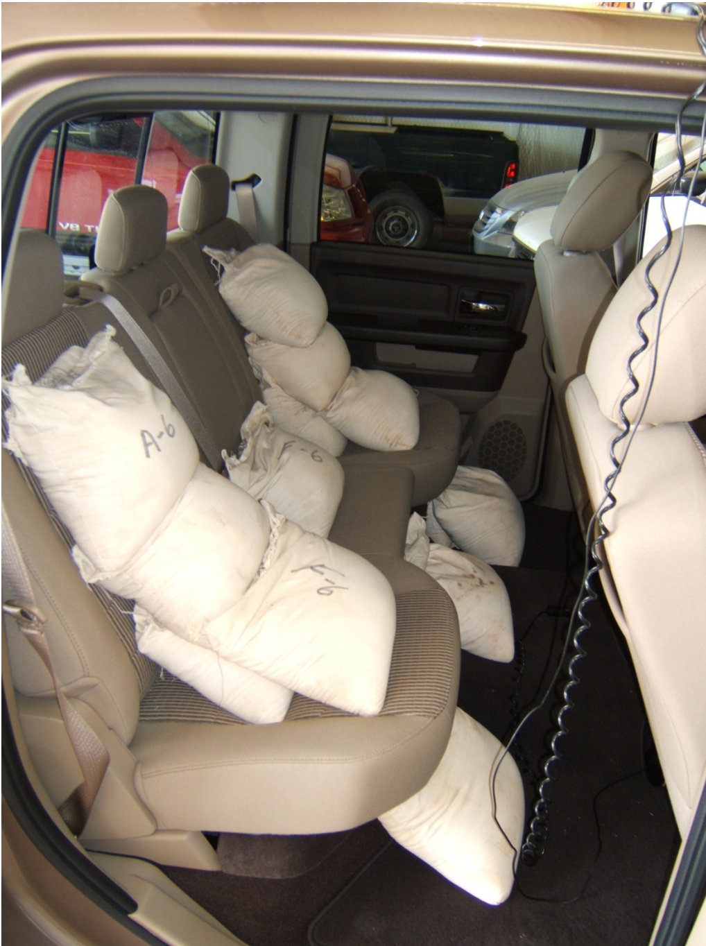
FIGURE 5.14 VEHICLE REAR SEAT BALLAST FOR UVW + VCW LOAD
