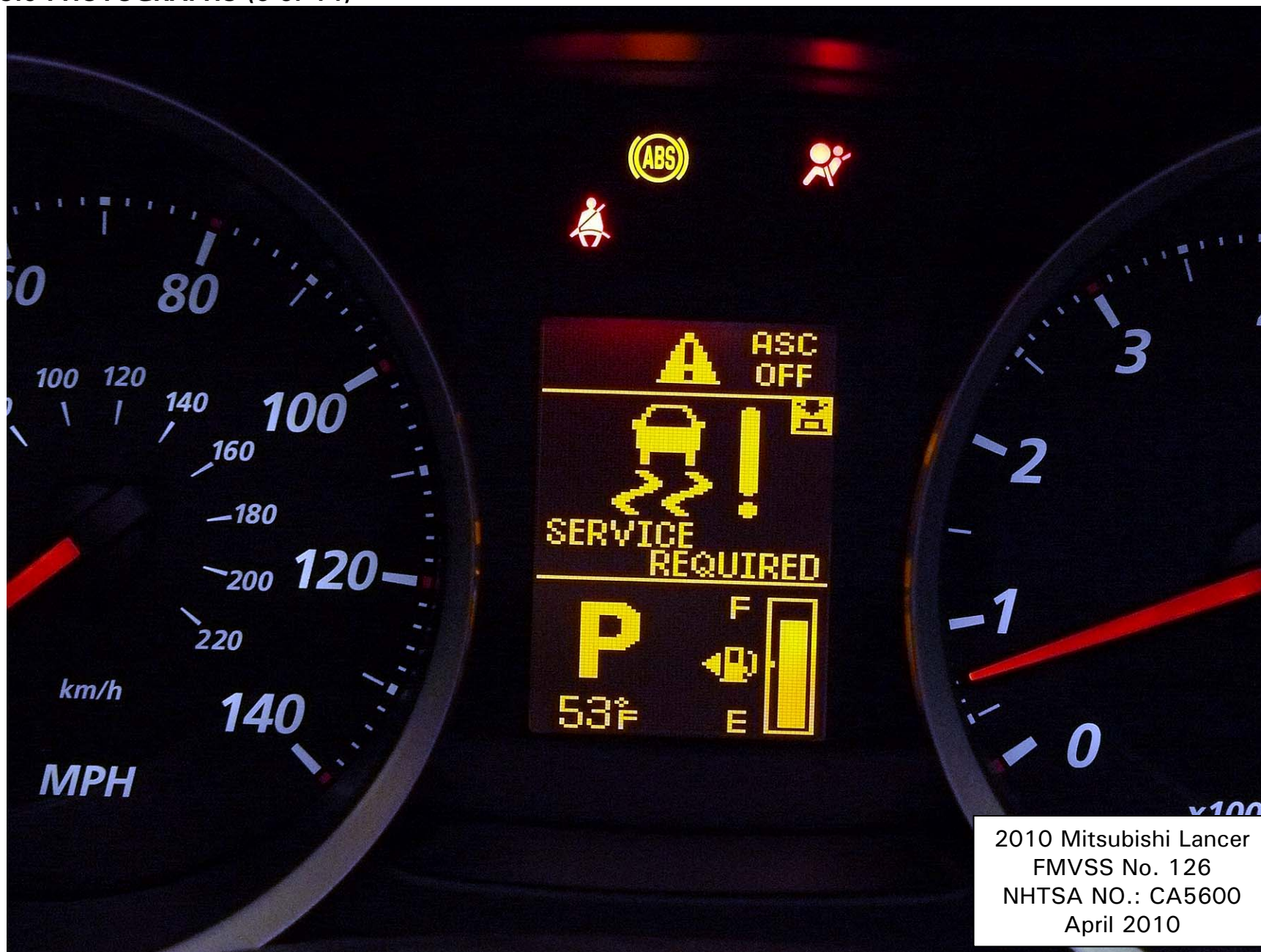
Figure 5.6. Telltale for ESC Malfunction and ESC Off
