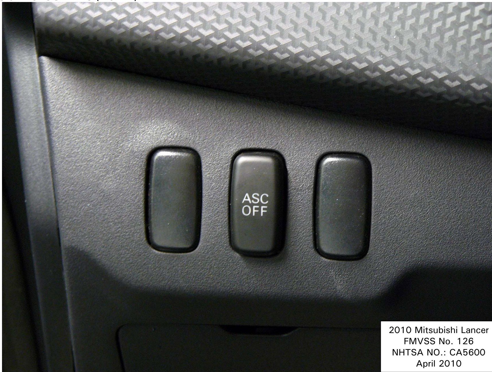
Figure 5.7. ESC Off Control Switch
