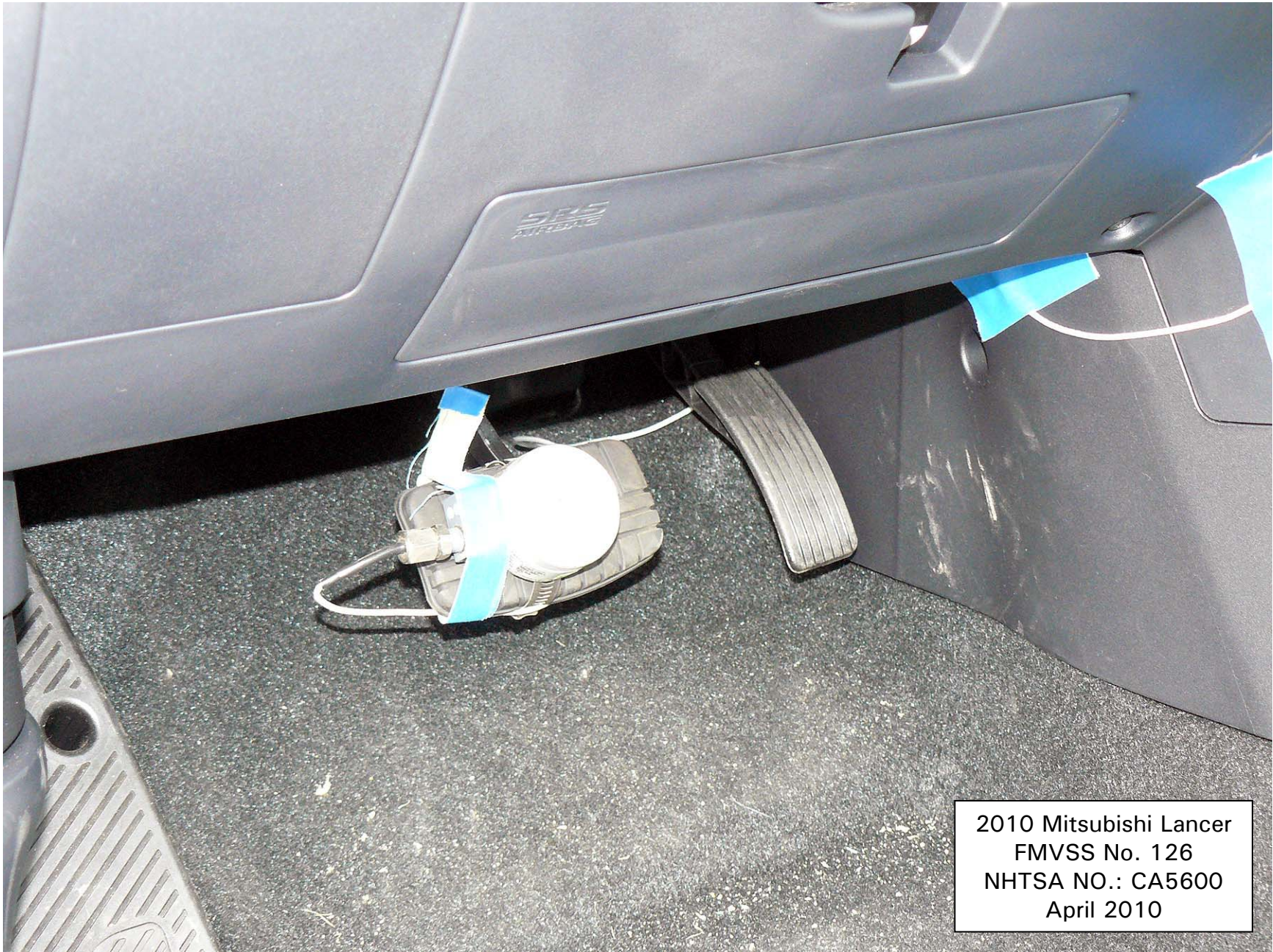
Figure 5.14. Brake Pedal Load Cell
