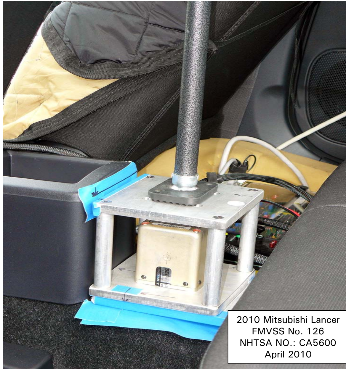
Figure 5.13. Inertial Measurement Unit Mounted in Vehicle
