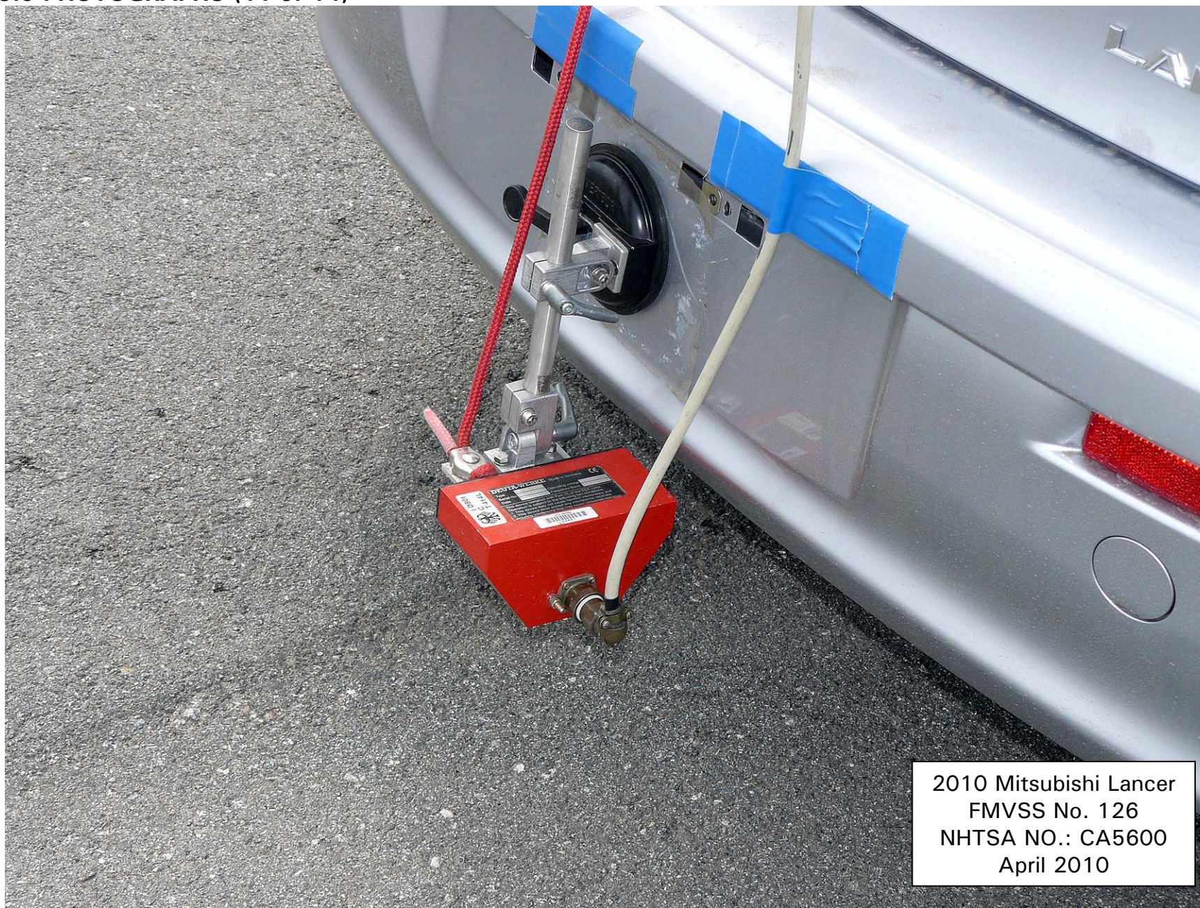
Figure 5.11. Rear Outrigger, Mount and Speed Sensor
