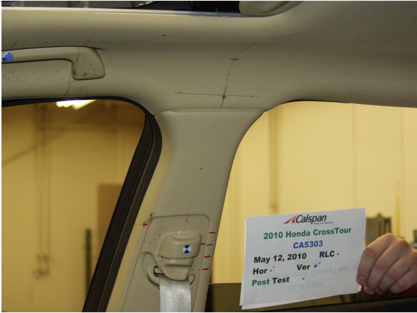
Figure A-28 : POST-TEST PASSENGER SIDE B-PILLAR
