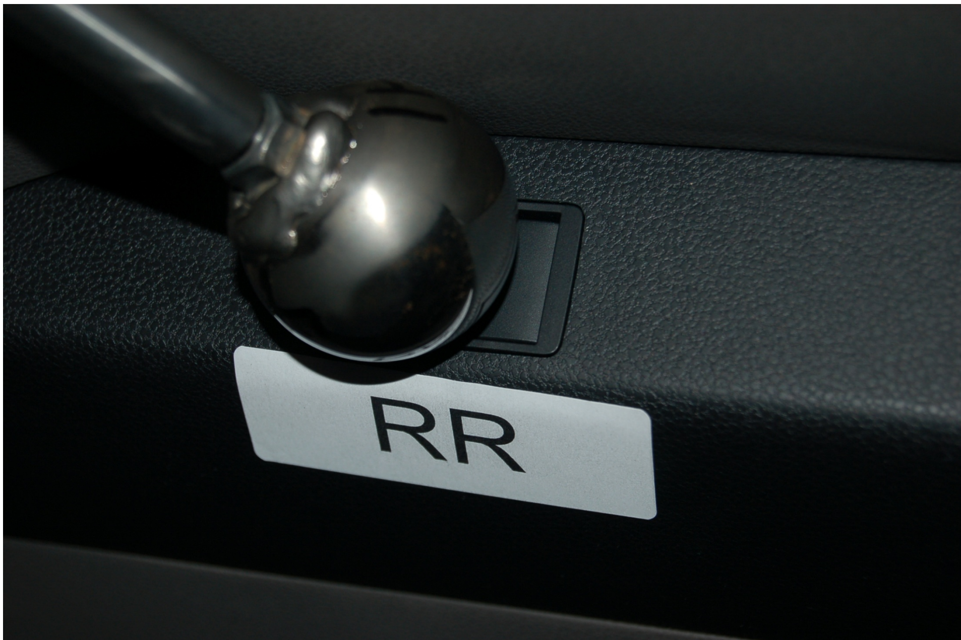
FIGURE 5.14 SPHERE TEST ON RIGHT REAR SWITCH
