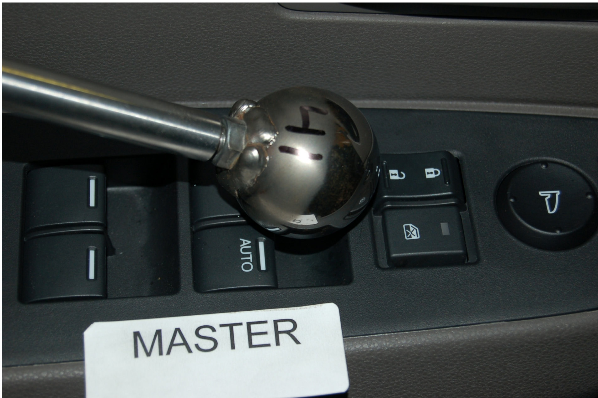
FIGURE 5.11 SPHERE TEST ON MASTER SWITCH
