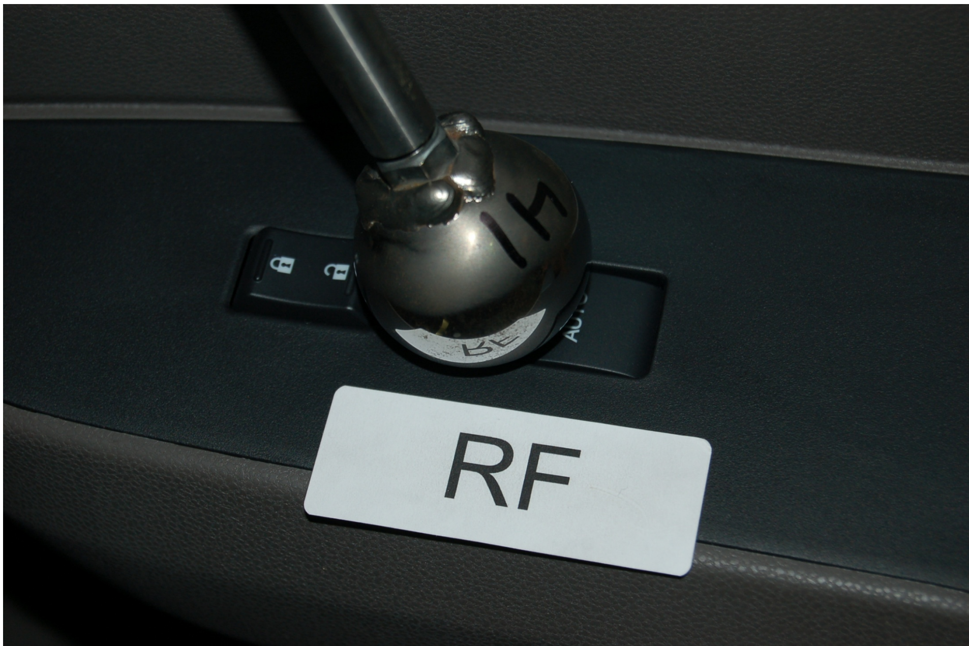
FIGURE 5.12 SPHERE TEST ON RIGHT FRONT SWITCH
