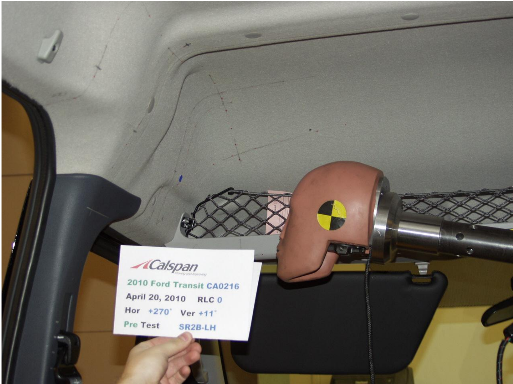
Figure A-10 : PRE-TEST DRIVER SIDE RAIL and B-PILLAR (Pre-impact picture is shown because pre-test pictures were unavailable)
