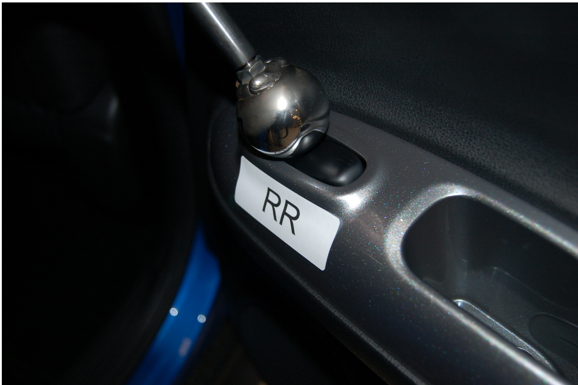
FIGURE 5.15 SPHERE TEST ON RIGHT REAR SWITCH
