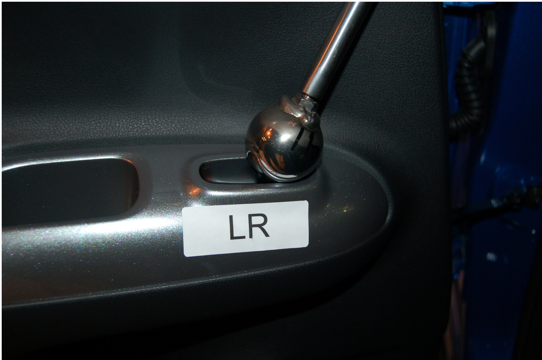
FIGURE 5.14 SPHERE TEST ON LEFT REAR SWITCH
