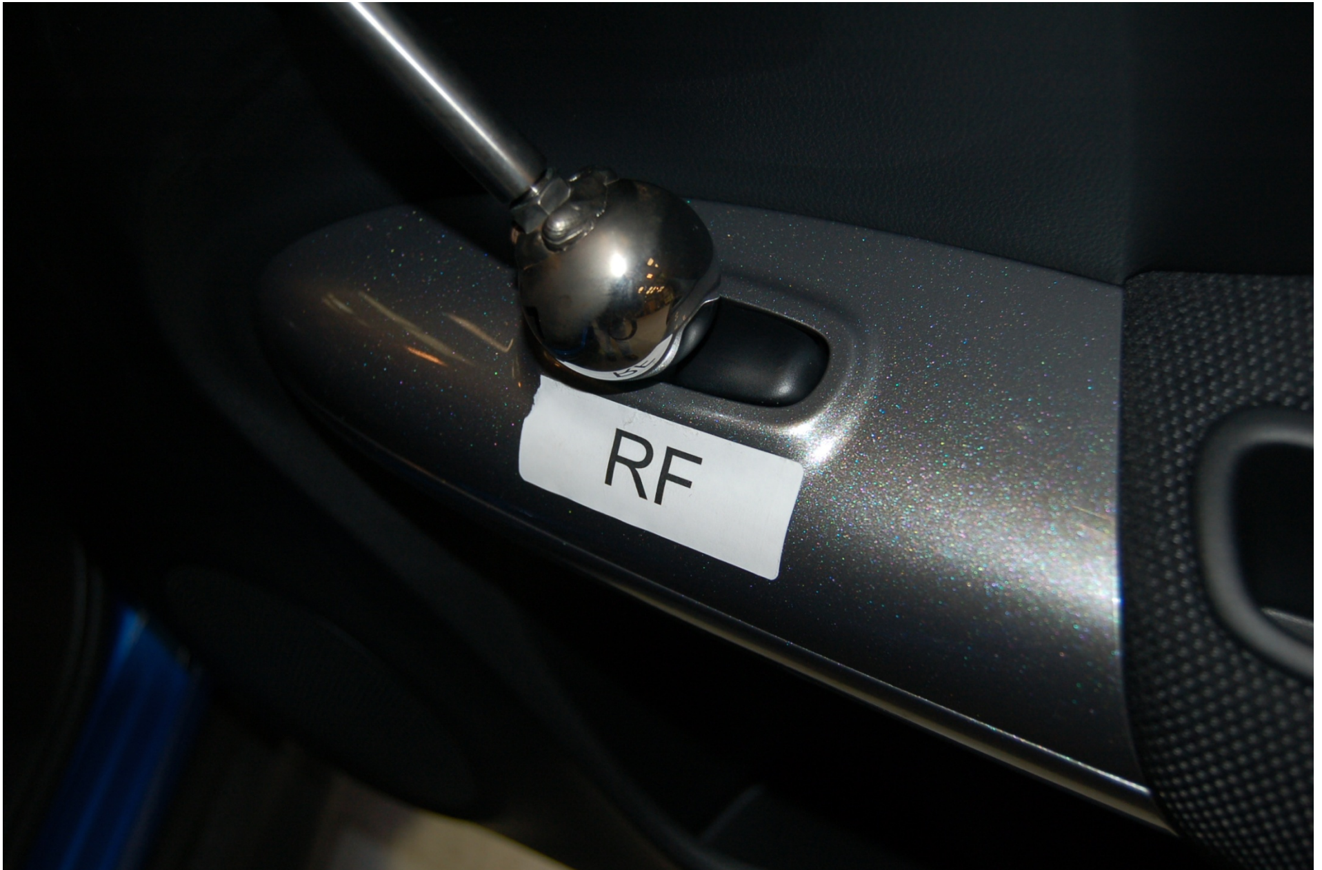
FIGURE 5.13 SPHERE TEST ON RIGHT FRONT SWITCH
