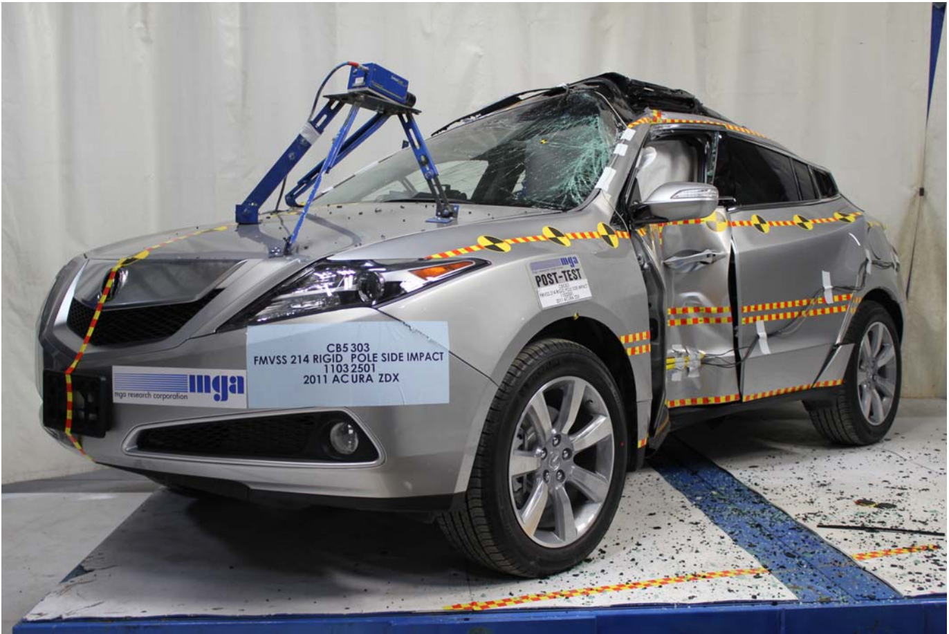
Post-Test \frac{3}{4} Front View of Impact Zone
