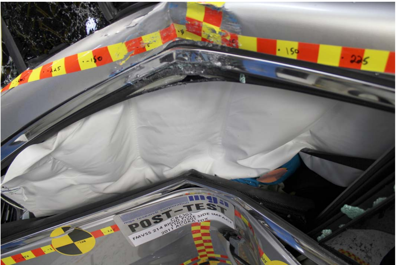
Post-Test Dummy Shoulder and Door Top View
