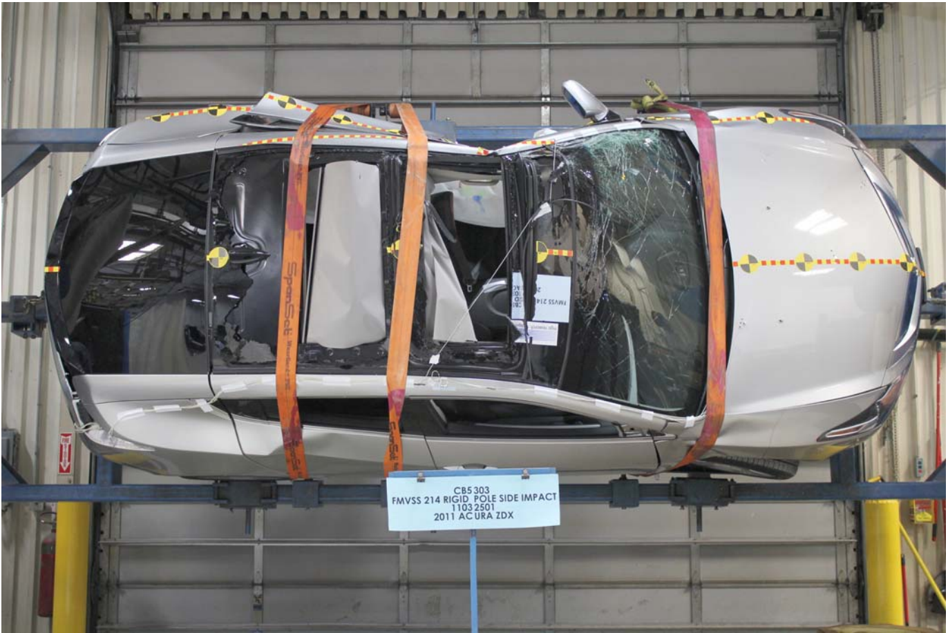
Post-Test Vehicle at 270 Degree Rollover
