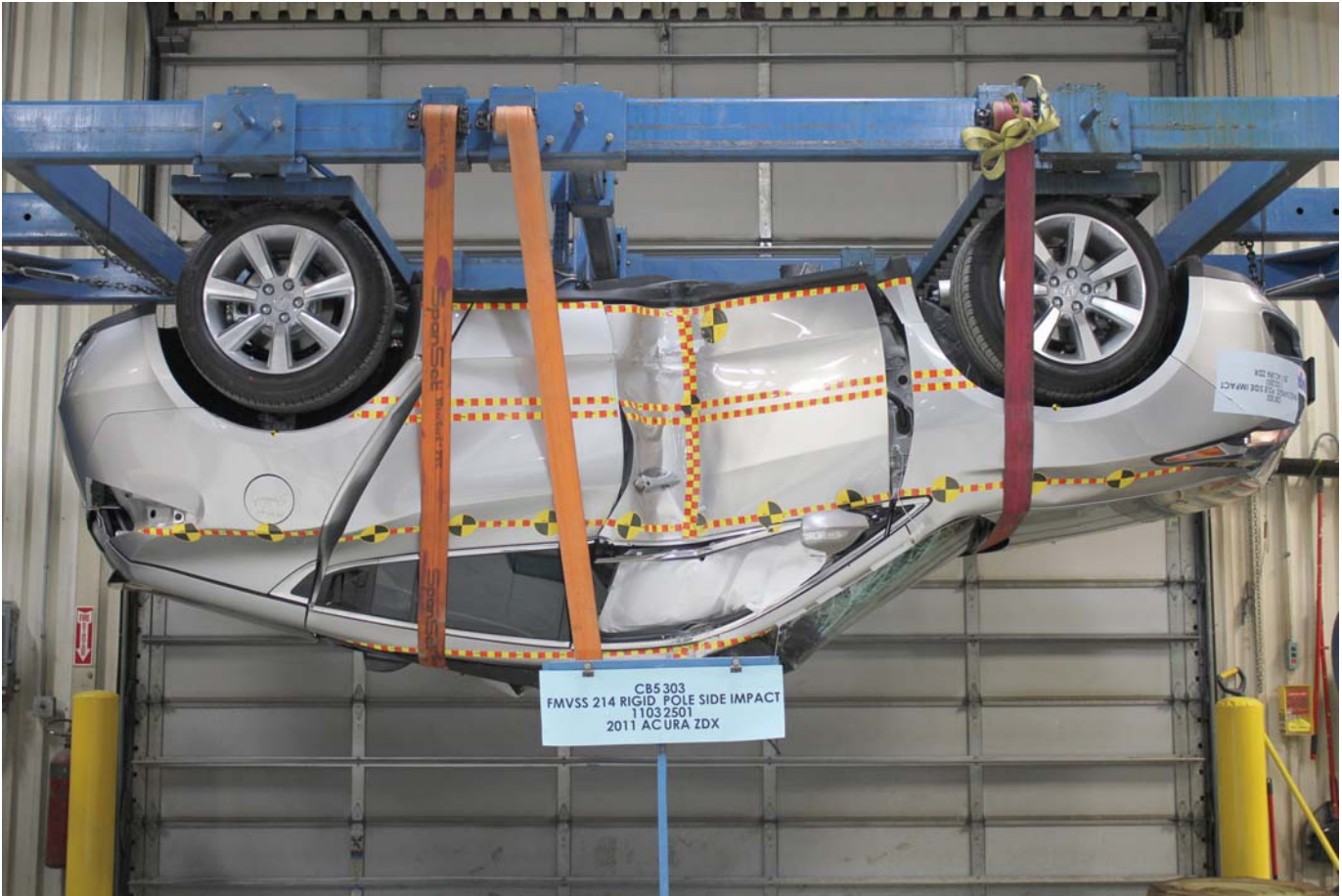
Post-Test Vehicle at 180 Degree Rollover
