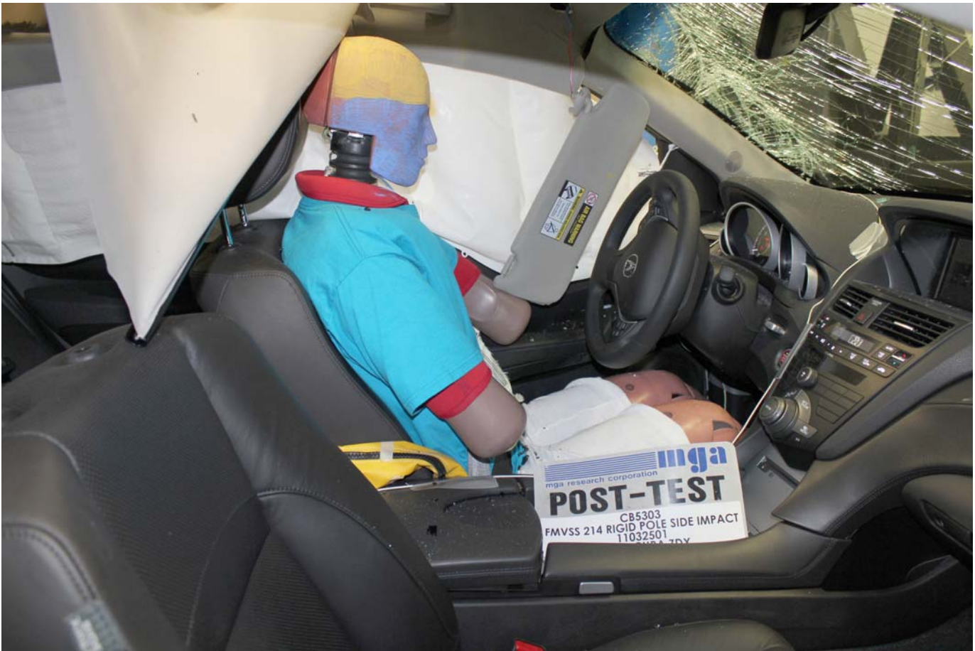
Post-Test Dummy Through Opposite Window
