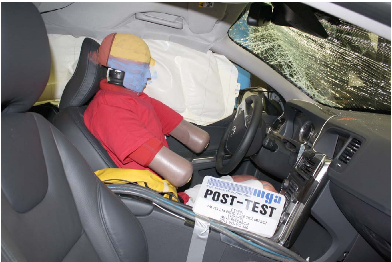
Post-Test Dummy Through Opposite Window
