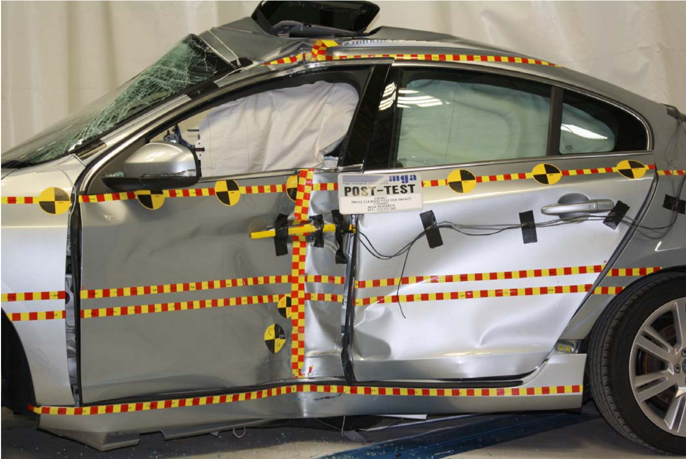
Post-Test Impact Zone Close-up View
