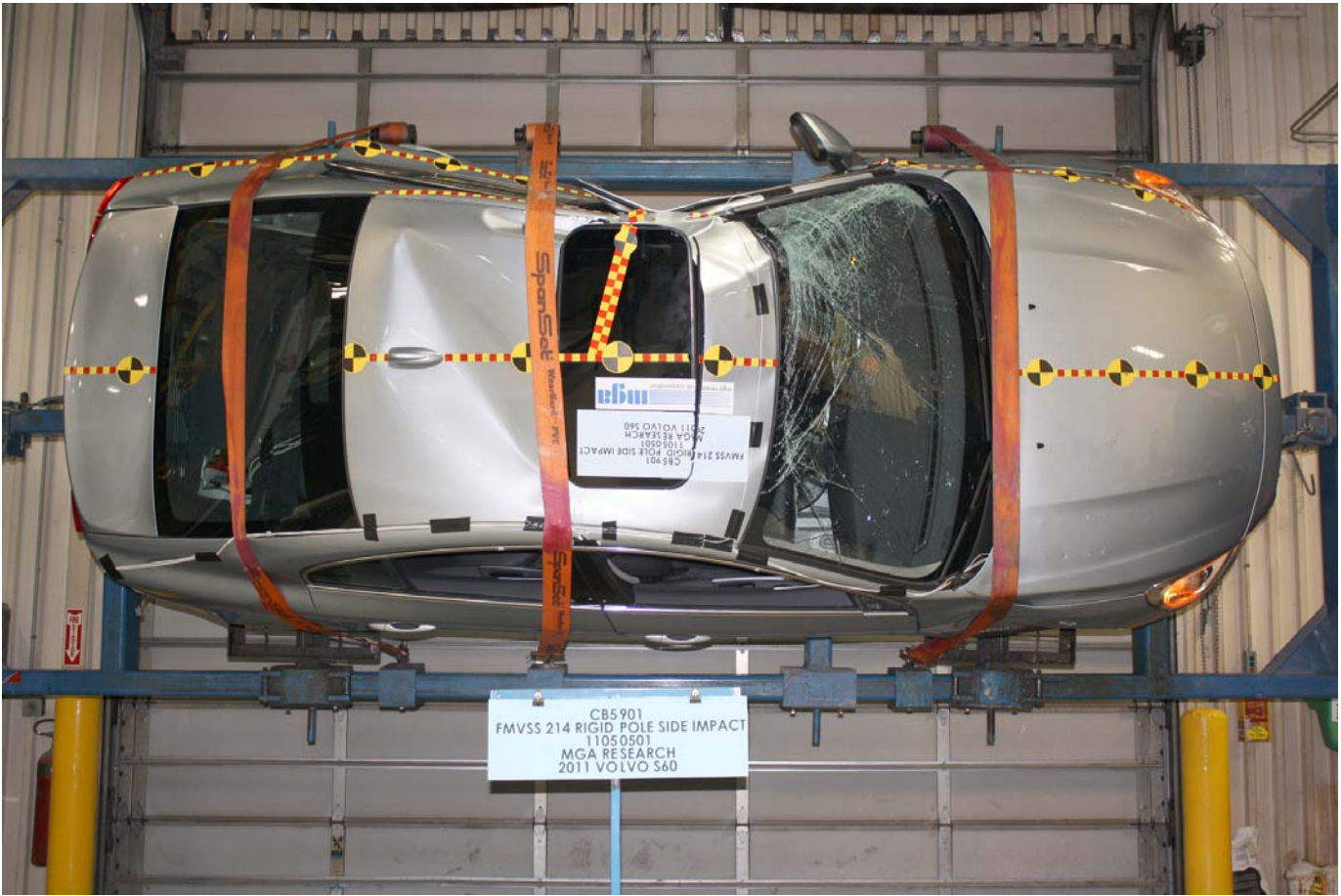
Post-Test Vehicle at 90 Degree Rollover
