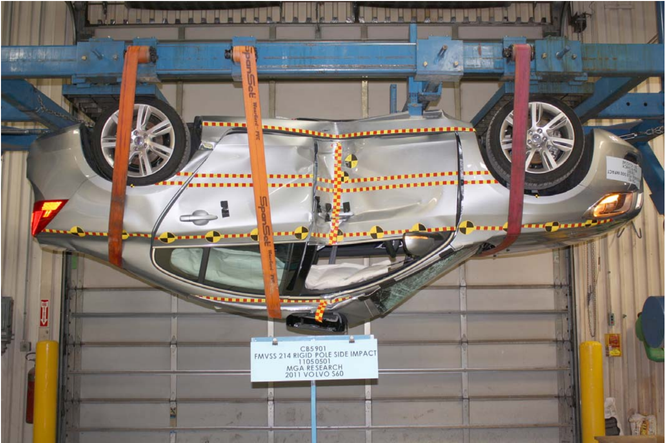
Post-Test Vehicle at 180 Degree Rollover
