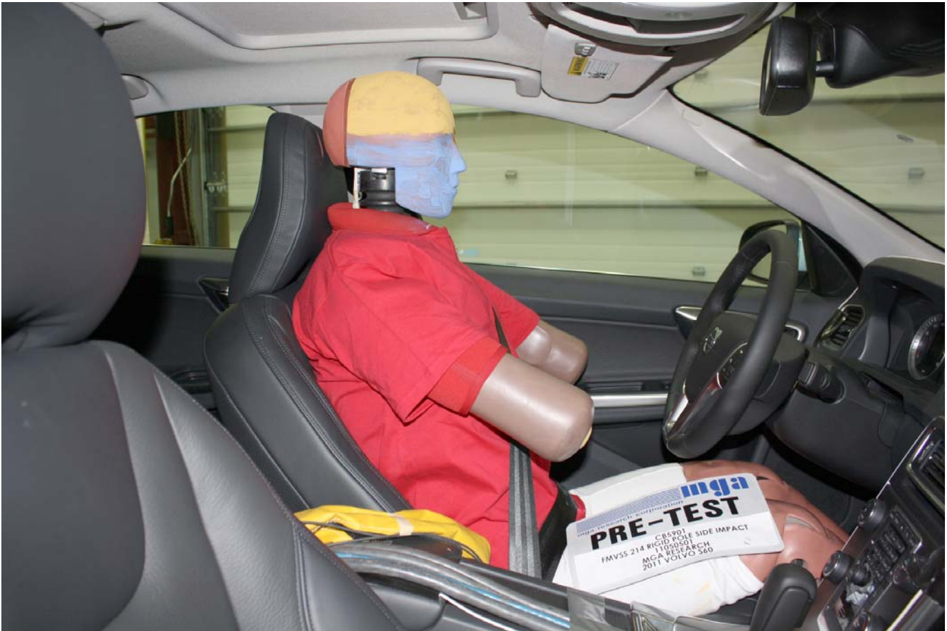
Pre-Test Dummy Through Opposite Window
