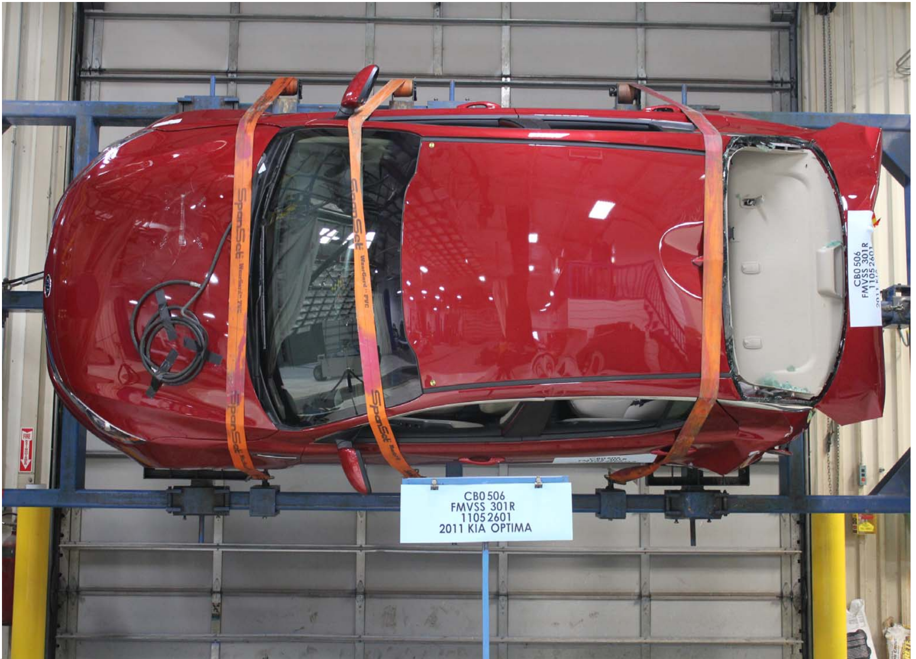
Static Rollover at 90 Degrees
