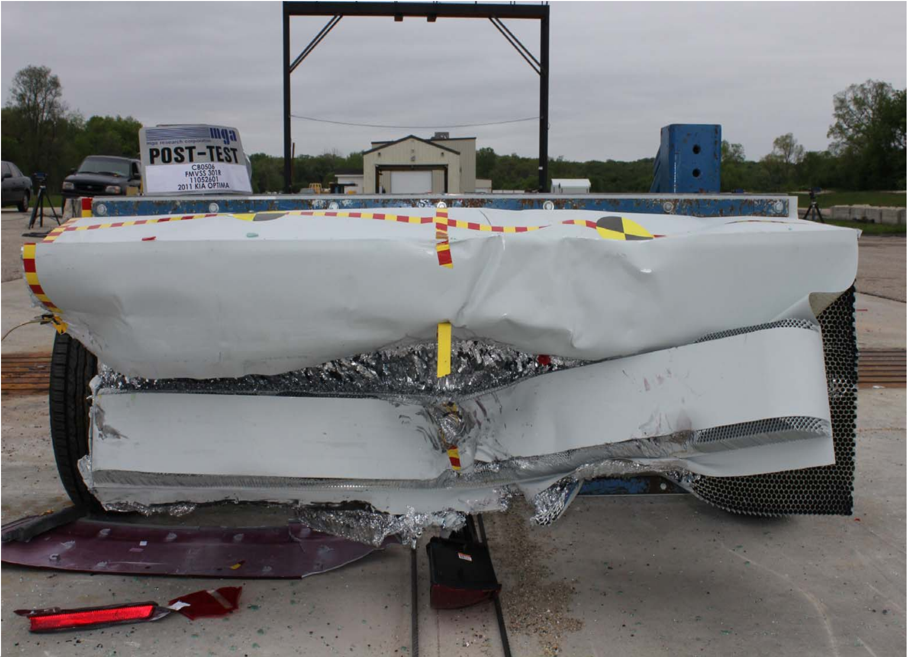
Post-Test Front View of MDB
