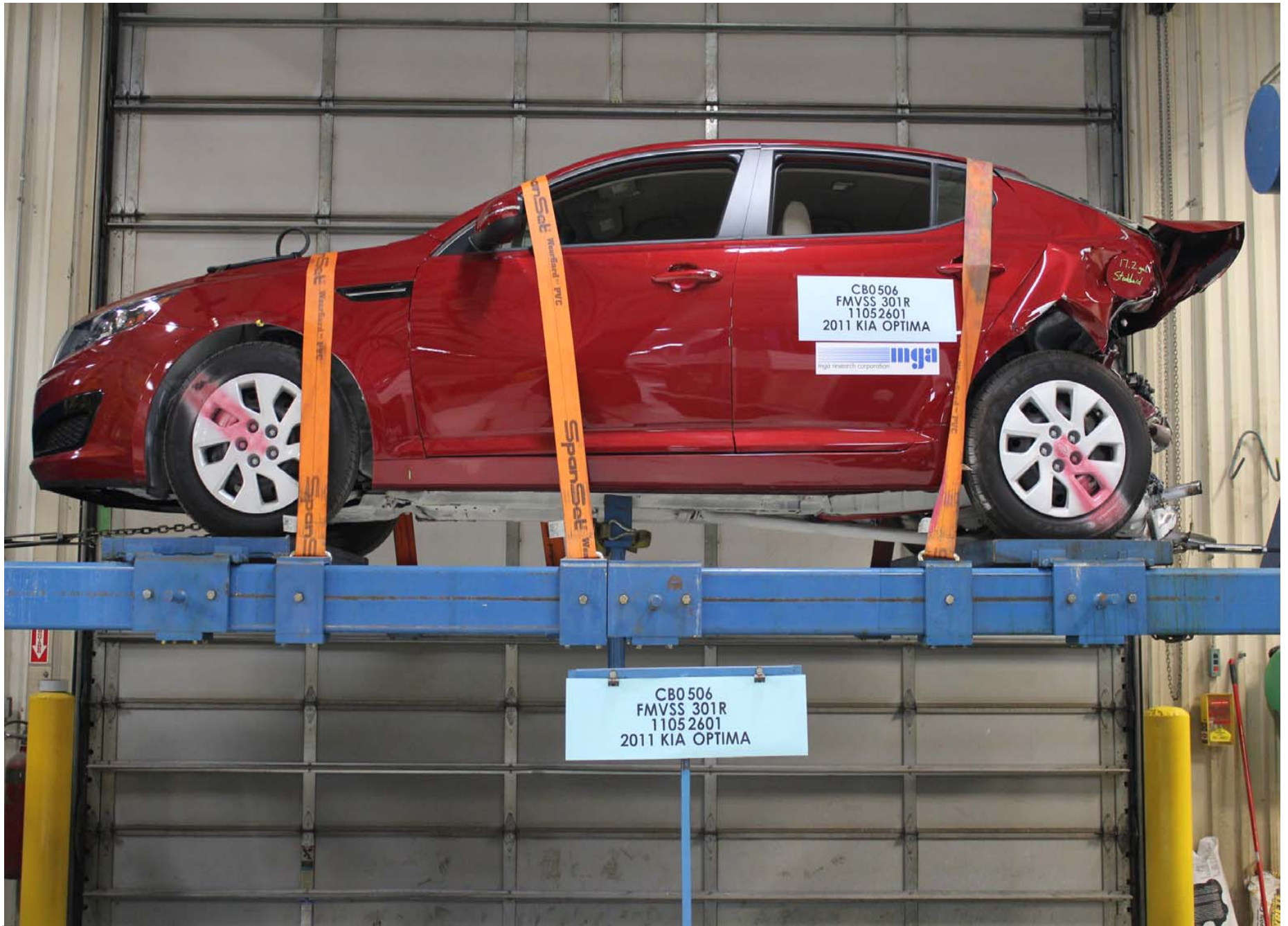
Static Rollover at 360 Degrees
