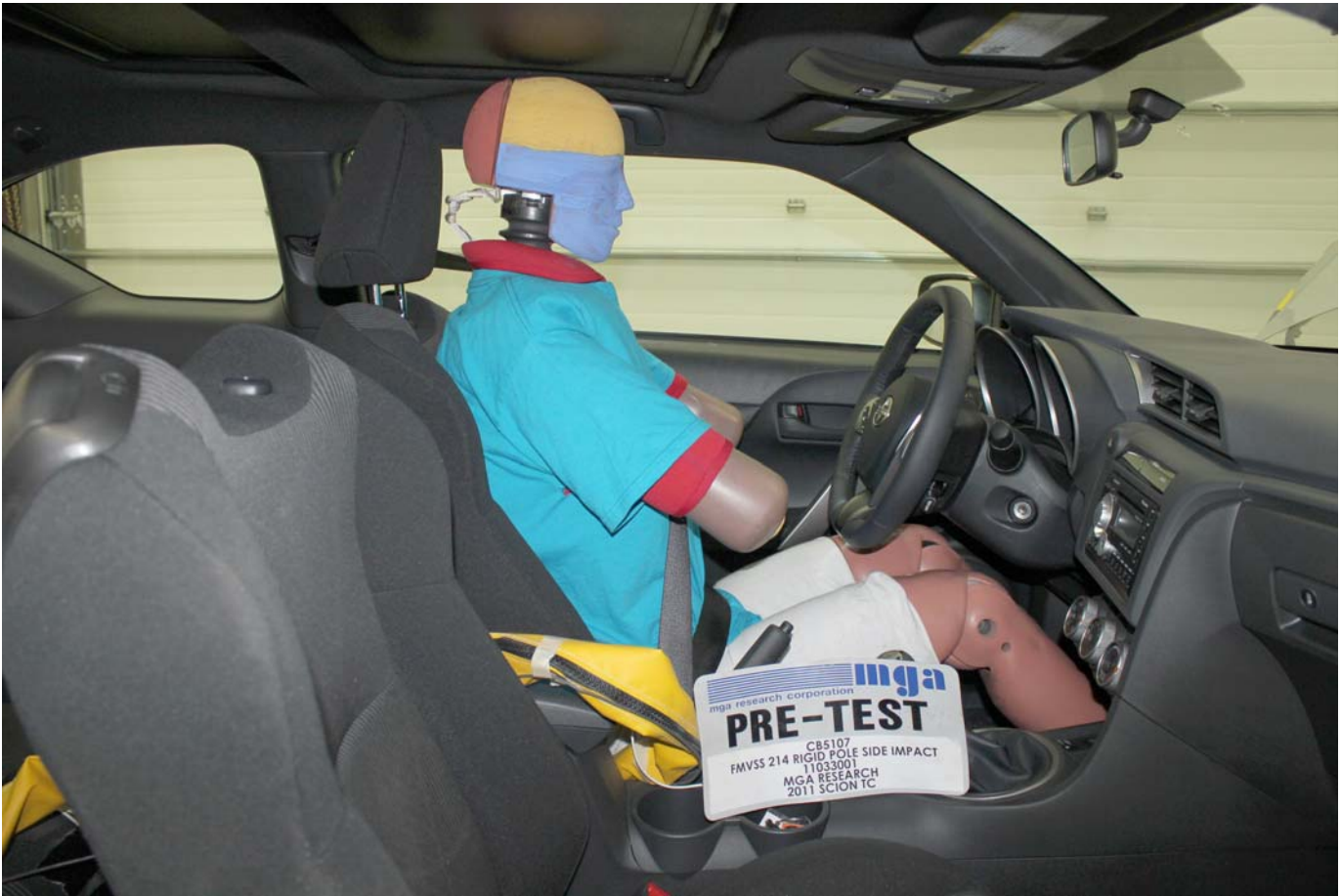
Pre-Test Dummy Through Opposite Window
