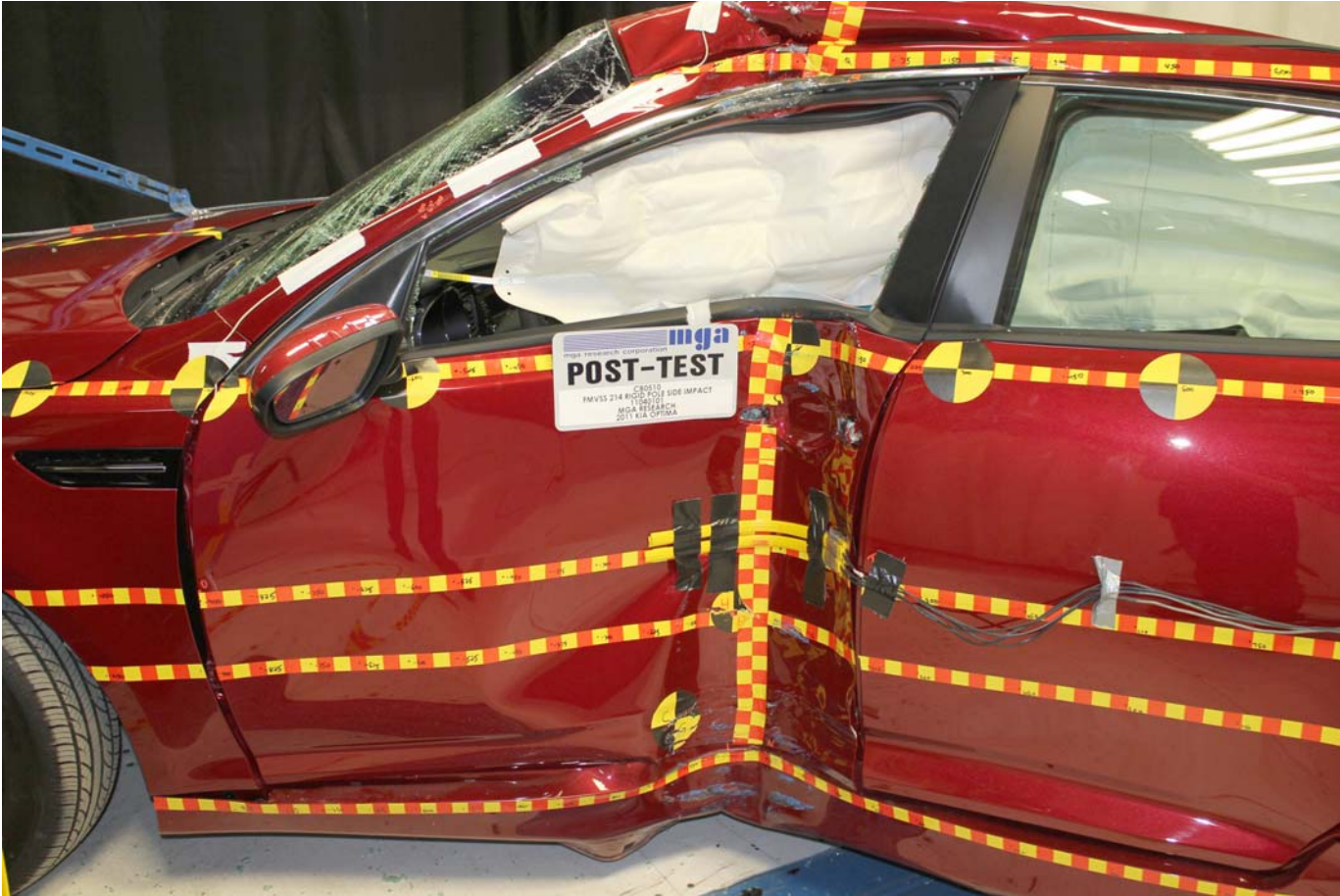
Post-Test Impact Zone Close-up View
