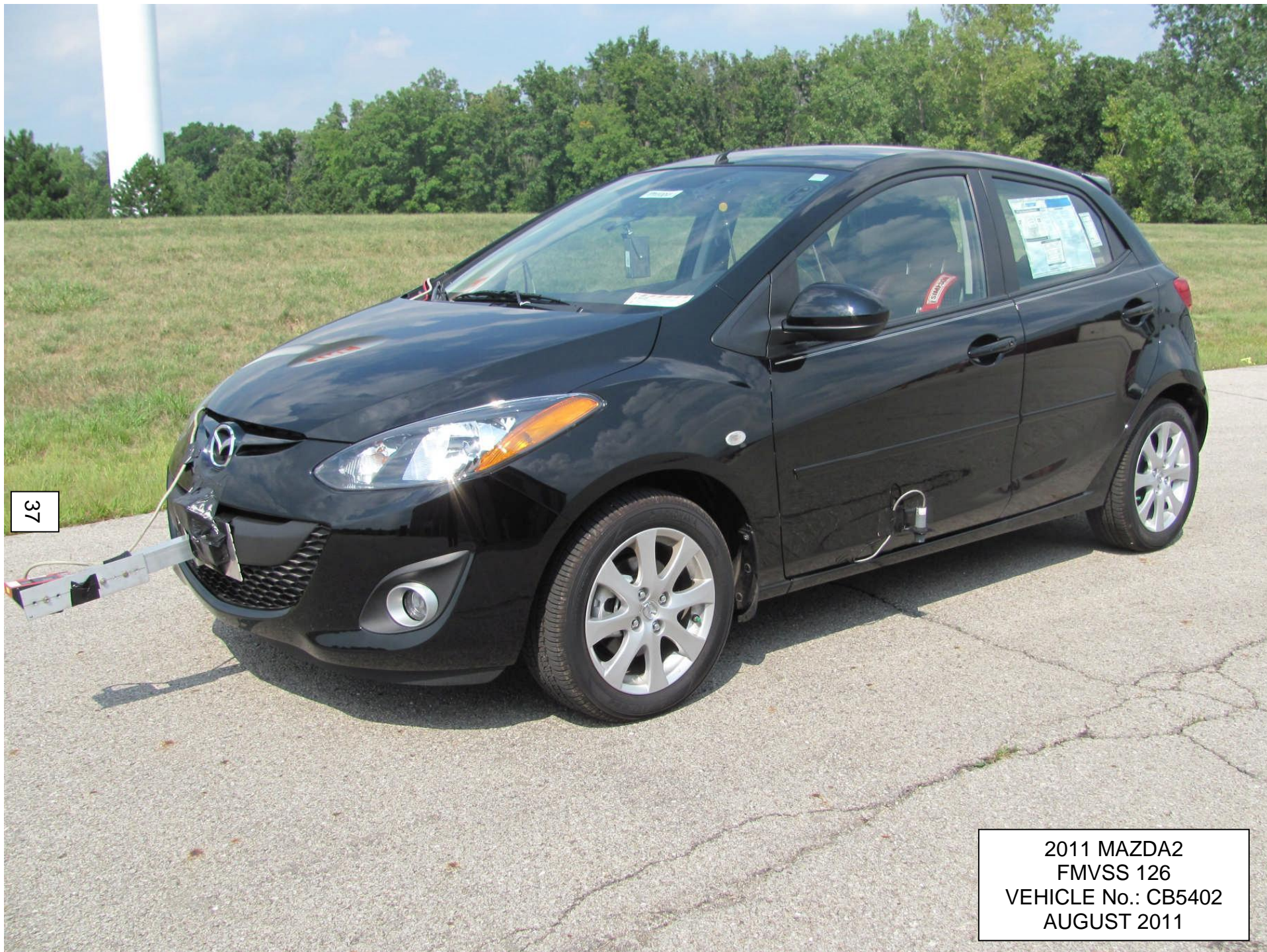
5.9 ¾ FRONT VIEW - TEST VEHICLE INSTRUMENTED
