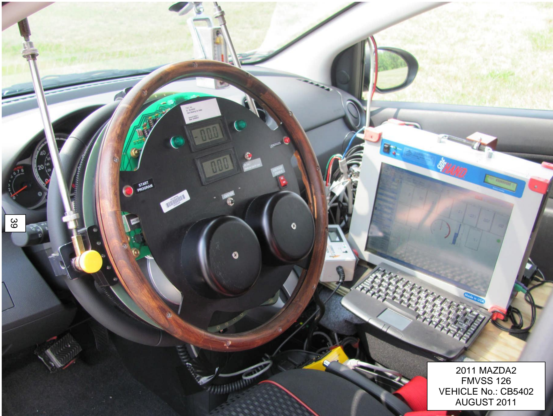
5.11 STEERING WHEEL CONTROLLER AND DATA ACQUISITION SYSTEM
