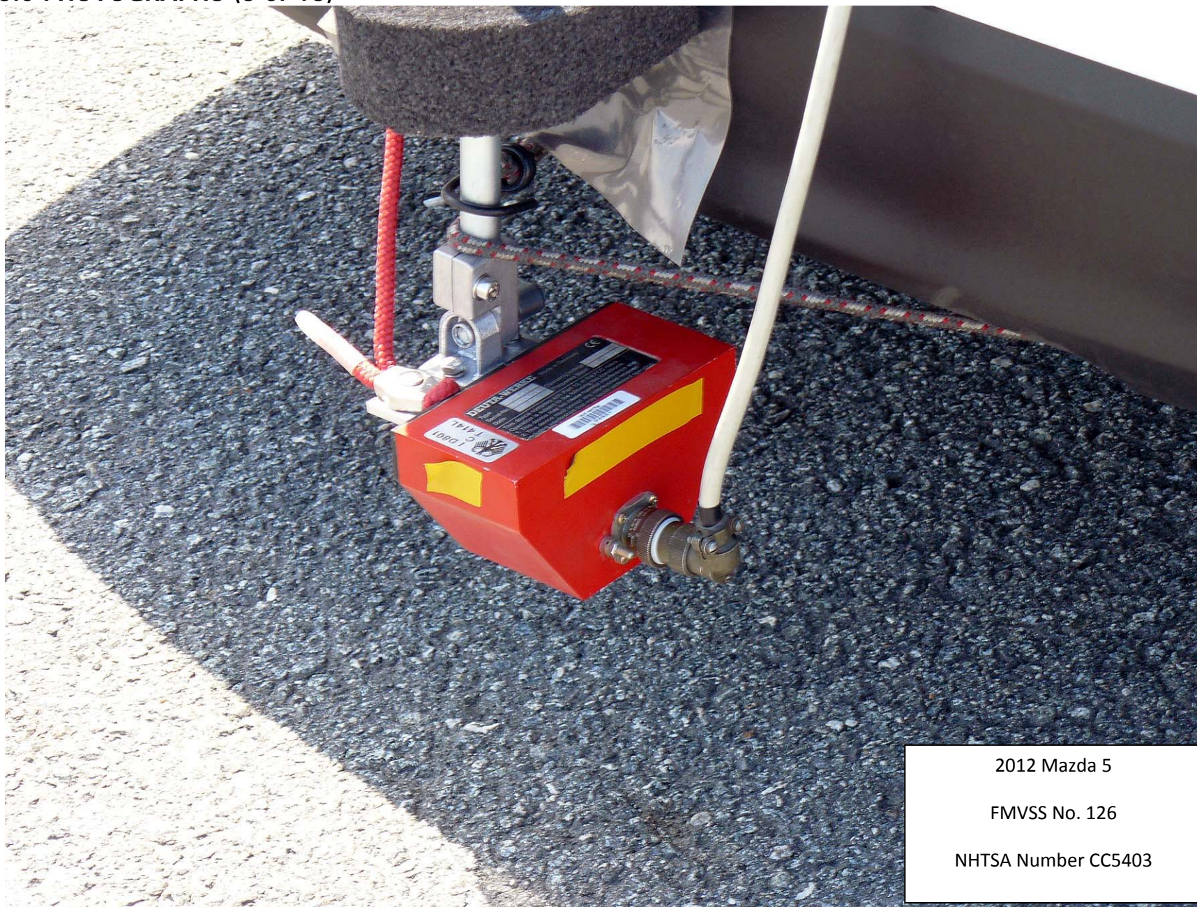
Figure 5.9. Rear Mounted Speed Sensor
