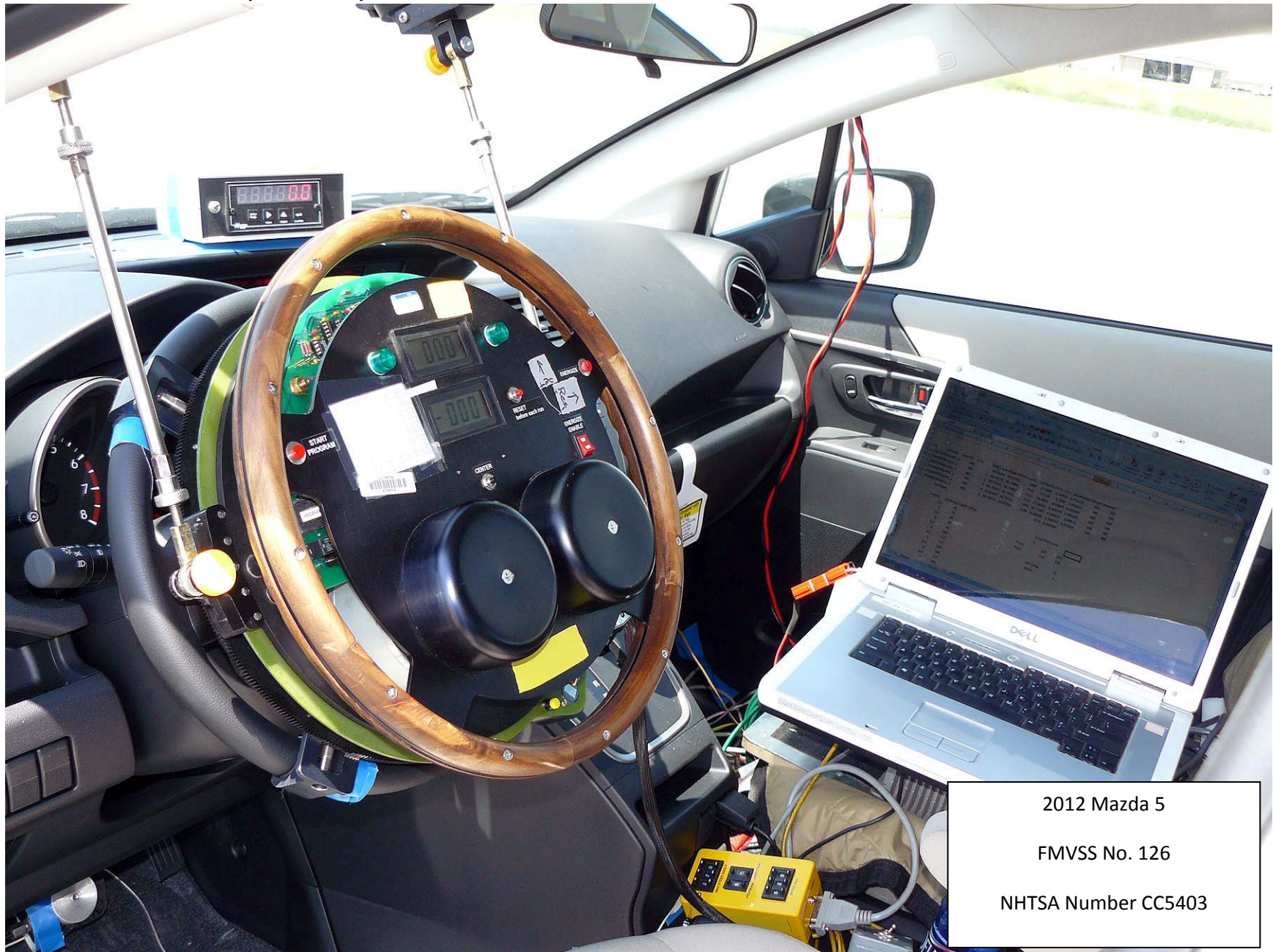
Figure 5.10. Steering Controller and Data Acquisition Computer
