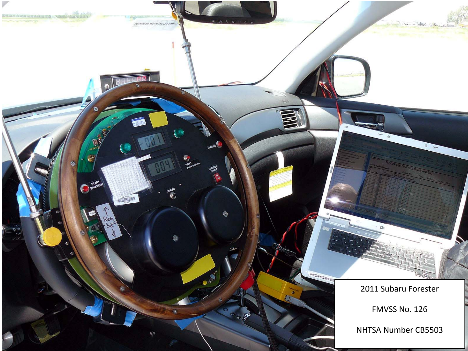
Figure 5.10. Steering Controller and Data Acquisition Computer
