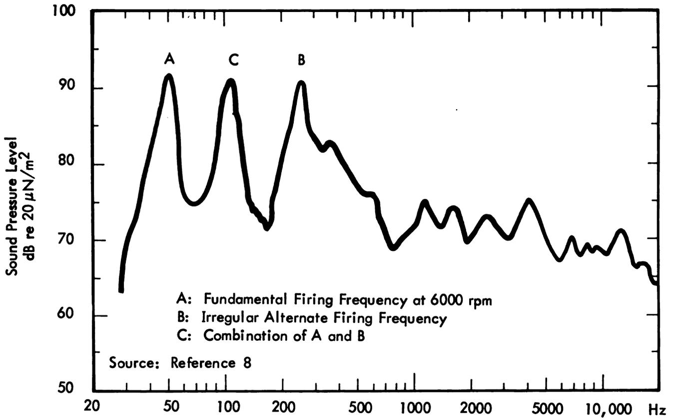
Figure 7. Narrow Band Exhaust Noise Spectrum for >200 cc Muffled Four-Cycle Twin Cylinder Motorcycle – See Text
