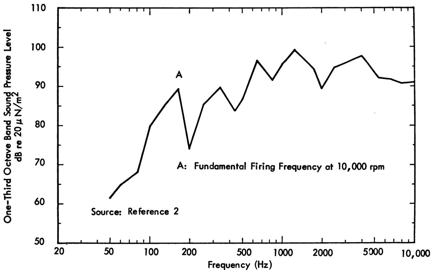
Figure 8. Passby Noise Spectrum for <200 cc Unmuffled Two-Cycle Single Cylinder Motorcycle – See Text
