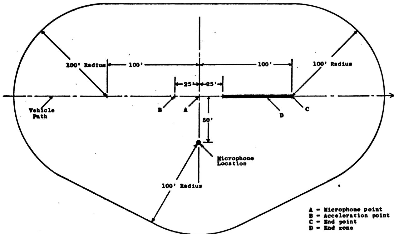
**Test Area Layout.** The test area shall include a vehicle path of sufficient length for safe acceleration, deceleration, and stopping of the vehicle. The vehicle path (shown with only one directional approach in Figure 3 for purposes of clarification) shall be marked with the following zone and points:
