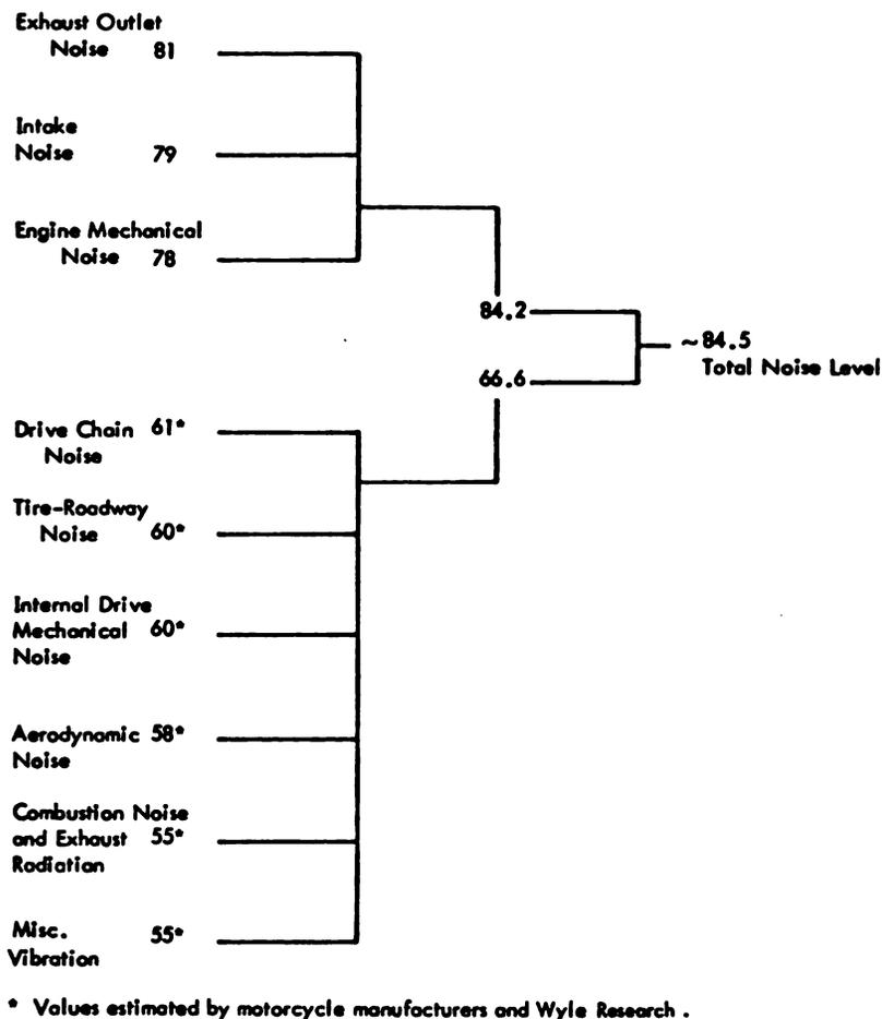
Figure 6. Typical Component Contributions to Total Noise Level When Measured per California Highway Patrol Procedures (dBA at 50 feet) for Typical 1973 Model Motorcycles > 200 cc
