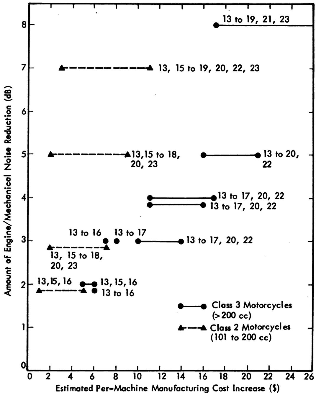
Figure 11. Estimated Costs for Reduction of Motorcycle Engine/Mechanical Noise
